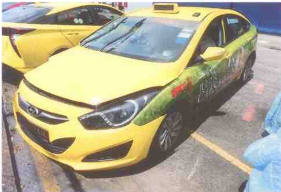
Photo 3 shows a general view of the front left portion of the Motor Taxi at the time of our inspection. The Motor Taxi was observed to have sustained minor impact damage at its front left portion.
