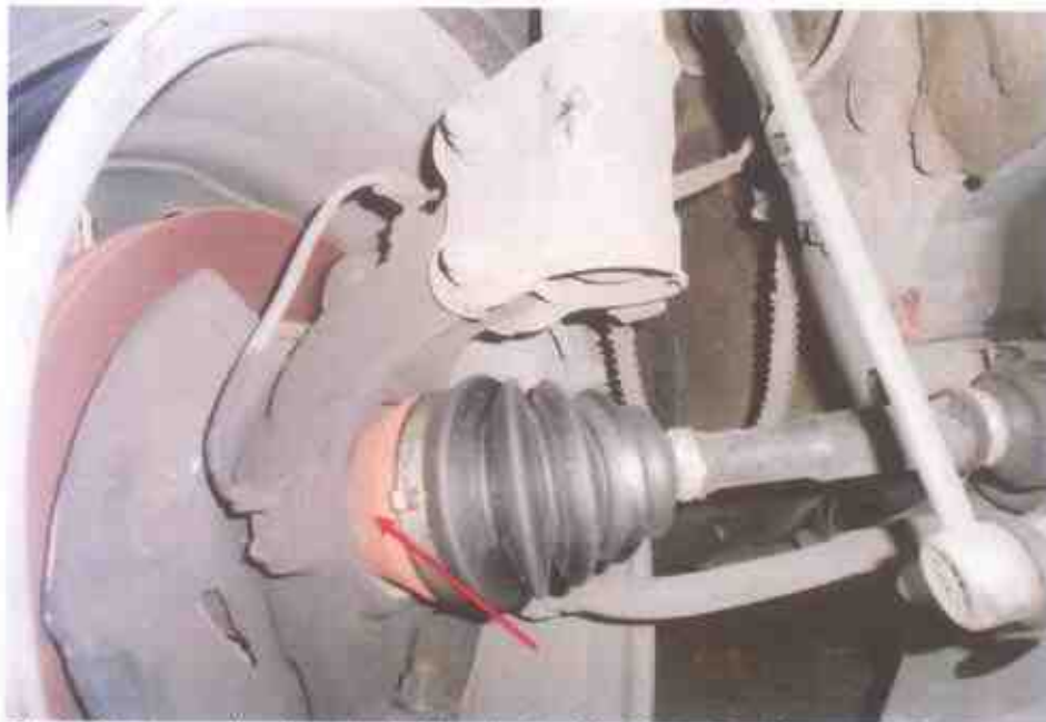
Photo 27 shows the dislodged drive shaft of the Motor Taxi front right wheel as a result of the accident's impact collision.
