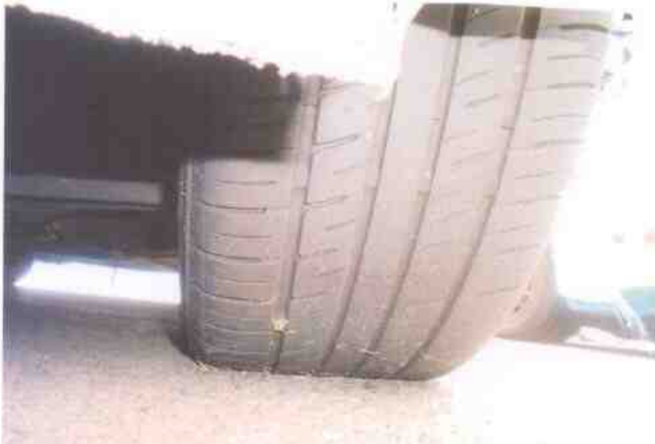
Photo 14 shows the condition of the front left tyre of the Motor Taxi, which was observed to be in serviceable condition with remaining tread depth of approximately 4mm. However, a small cut mark was observed on the outer sidewall of the tyre likely due to the accident.
