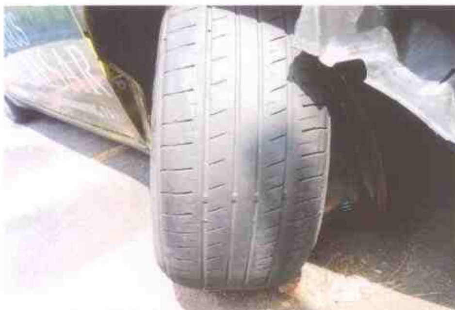
Photo 10 shows the condition of the front right tyre of the Motor Taxi, which was observed to be dislodged as a result of the accident. We did find cut mark on the outer sidewall as well as across the tyre surface which was likely due to the result of the accident.
