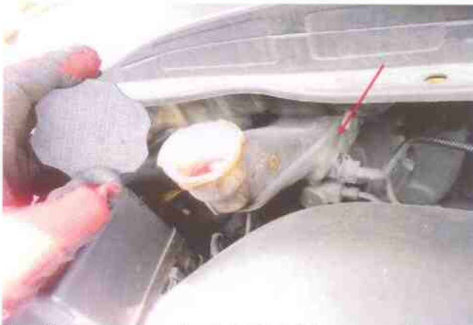
Photo 22 shows the close up view of the brake fluid that was seen with sufficient level not affected by the accident's impact.
