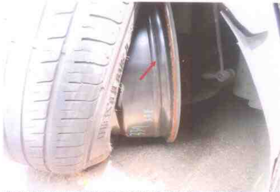
Photo 26 shows the dislodged front right wheel rim of the Motor Taxi as a result of the accident's impact collision.
