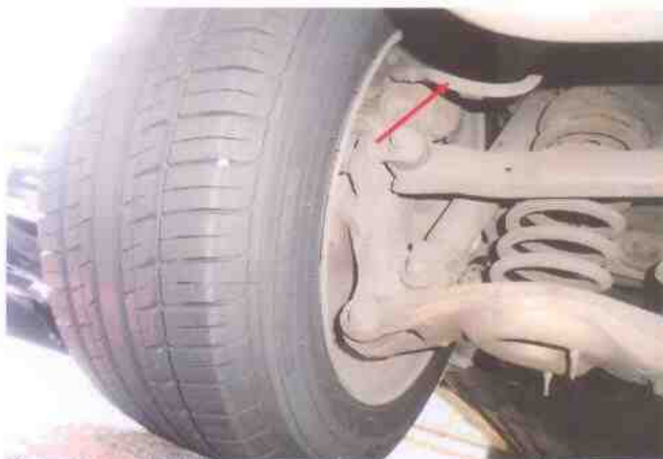
Photo 31 shows the braking components at the rear left wheel of the Motor Taxi. We did not observe any leakage of brake fluid at the time of our inspection of the Motor Taxi.
