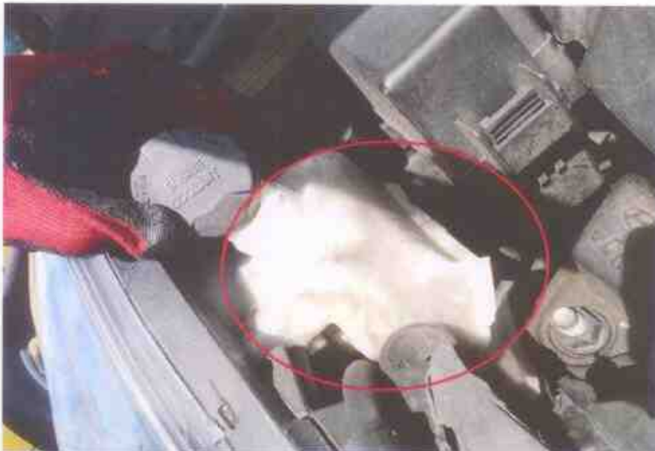
Photo 20 shows the close up view of the engine coolant reservoir that was observed to be damaged (cracked) by the accident's impact
