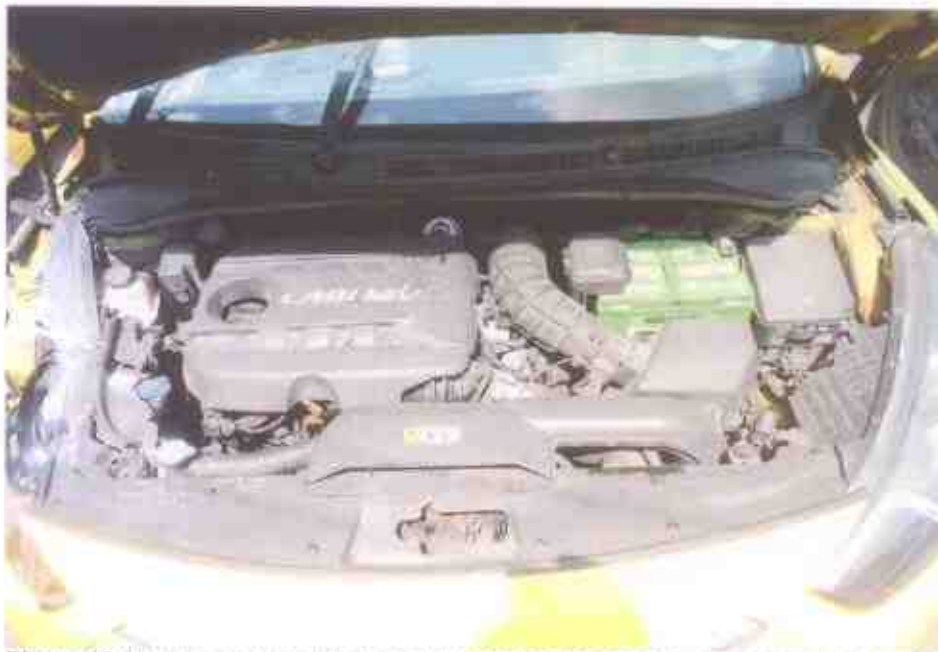
Photo 18 shows a general view of the Motor Car's engine compartment. Most of the various parts and components inside the engine compartment were unaffected by the accident. There was also no sign(s) or indication(s) of fluid leakage and/or fluid stain within the engine compartment.
