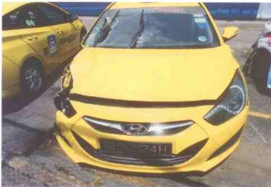
Photo 1 shows a general view of the frontal portion of the Motor Taxi at the time of our inspection. The Motor Taxi was observed to have sustained extensive impact damage at its frontal right portion. The impact force was significant, causing the various parts and components to be damaged as a result of the accident.
