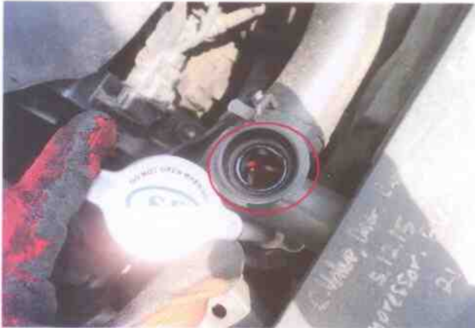
Photo 19 shows the close up view of the engine coolant that was seen with sufficient level not affected by the accident's impact
