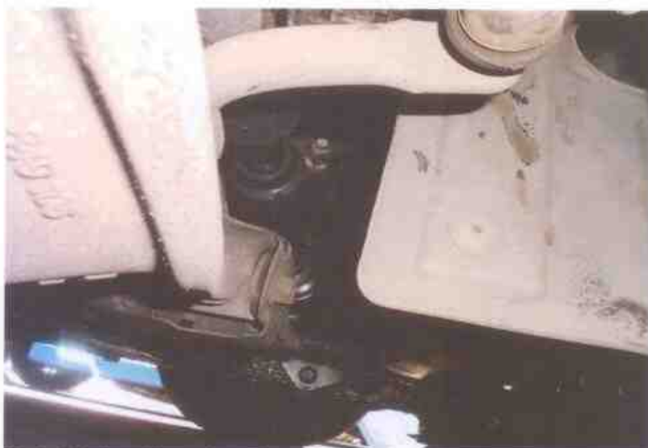
Photo 24 shows the undercarriage of the engine area. It was observed to be unaffected by the accident's impact.
