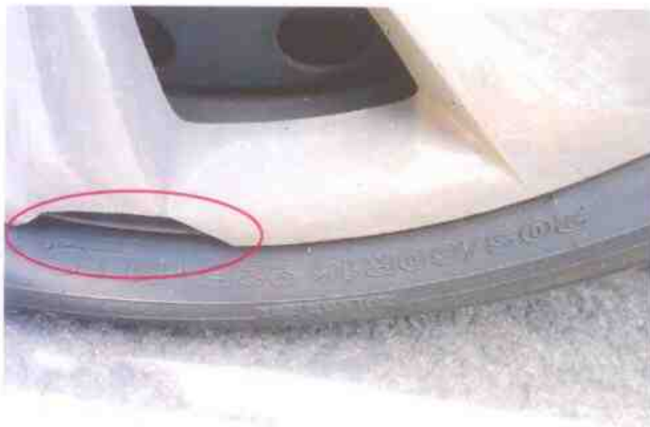
Photo 15 shows the condition of the front left tyre of the Motor Taxi, which was observed to be in serviceable condition with remaining tread depth of approximately 4mm. However, a small cut mark was observed on the outer sidewall of the tyre likely due to the accident.
