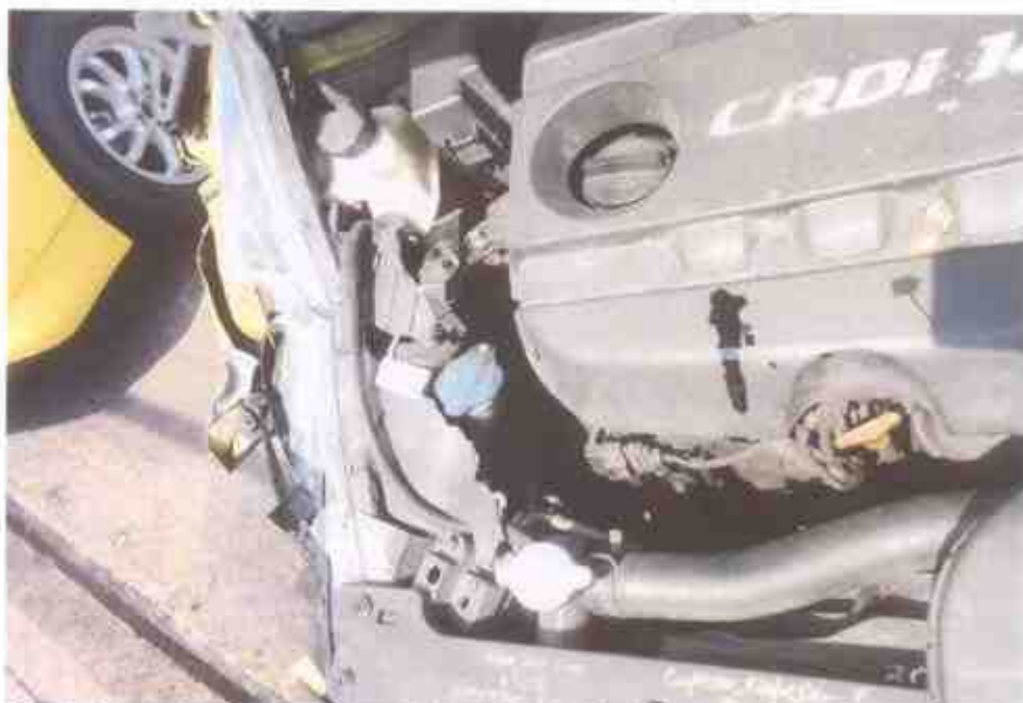
Photo 7 shows a closer view of the damaged engine component. The impact force was significant, causing the engine coolant reservoir to be damaged due to the accident's impact.
