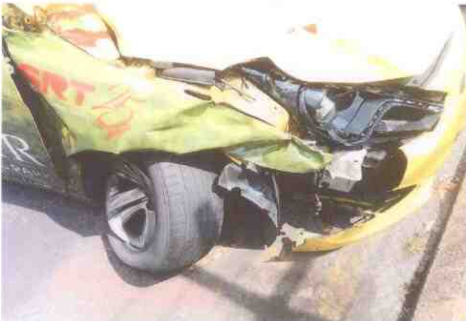
Photo 5 shows a closer view of the damage sustained on the front right of the Motor Taxi. The impact force was significant, causing the various parts and components inside the engine compartment to be damaged, which includes the headlamp, rim & tyre amongst others.
