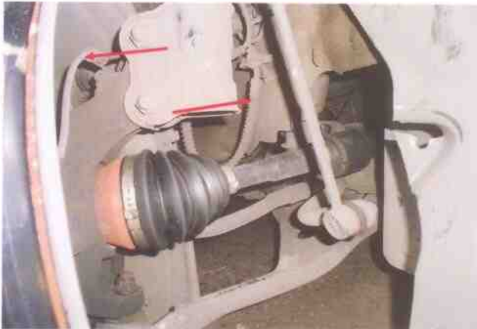
Photo 29 shows the braking components at the front right wheel of the Motor Taxi. We did not observe any leakage of brake fluid at the time of our inspection of the Motor Taxi.
