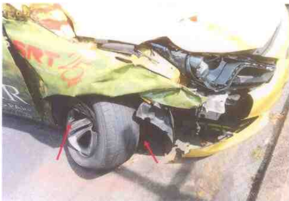
Photo 25 shows the damaged steering system at the front right wheel of the Motor Taxi.
