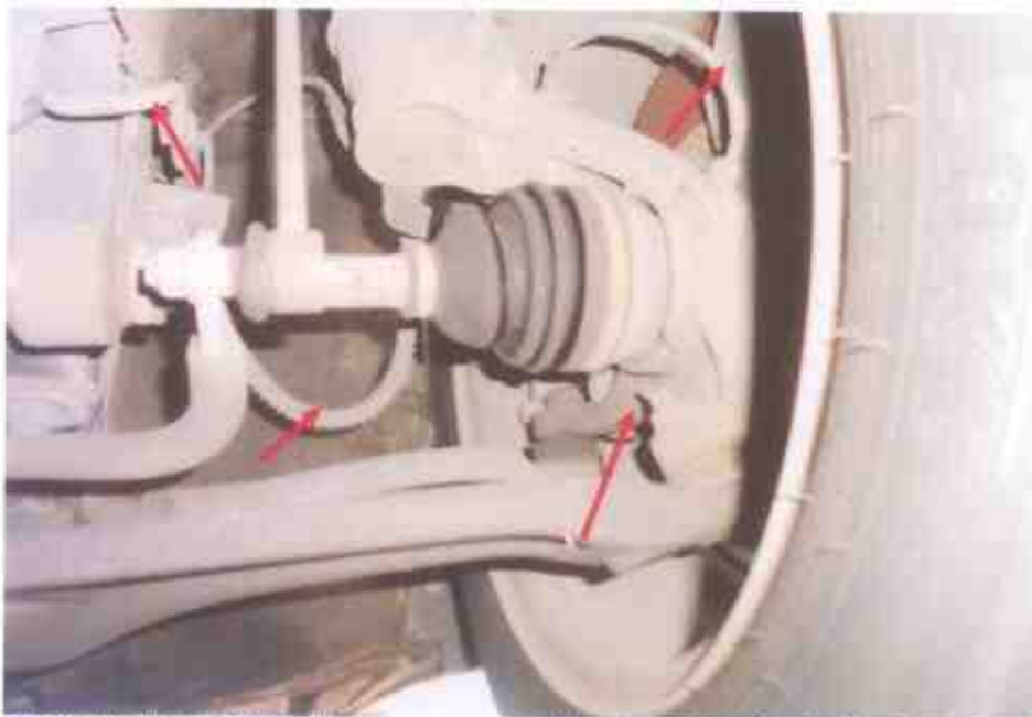
Photo 28 shows the braking components at the front left wheel of the Motor Taxi. We did not observe any leakage of brake fluid at the time of our inspection of the Motor Car.
