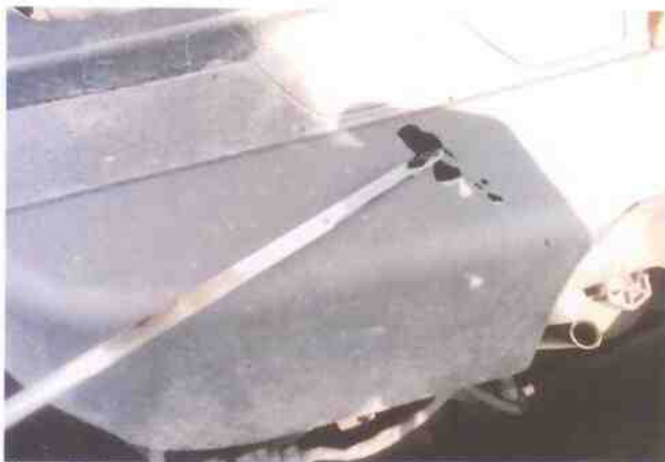
Photo 23 shows the engine oil dip stick of the Motor Taxi at the time of our inspection. The engine oil was observed to be of sufficient level and without any visible contamination.
