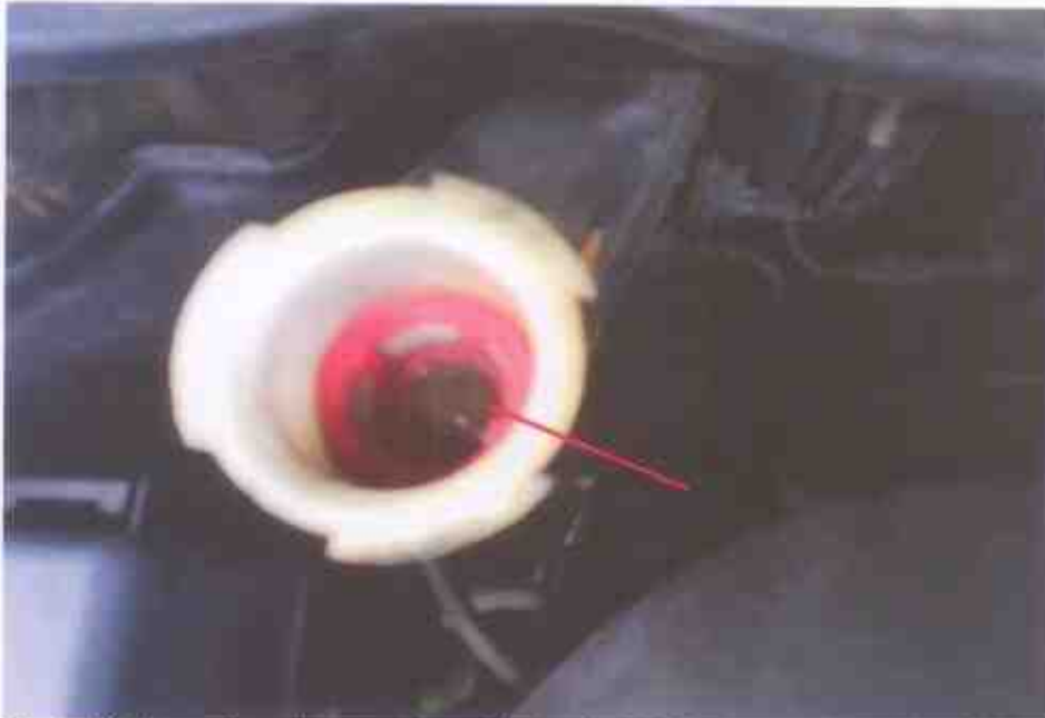
Photo 21 shows the close up view of the brake fluid that was seen with sufficient level not affected by the accident's impact.
