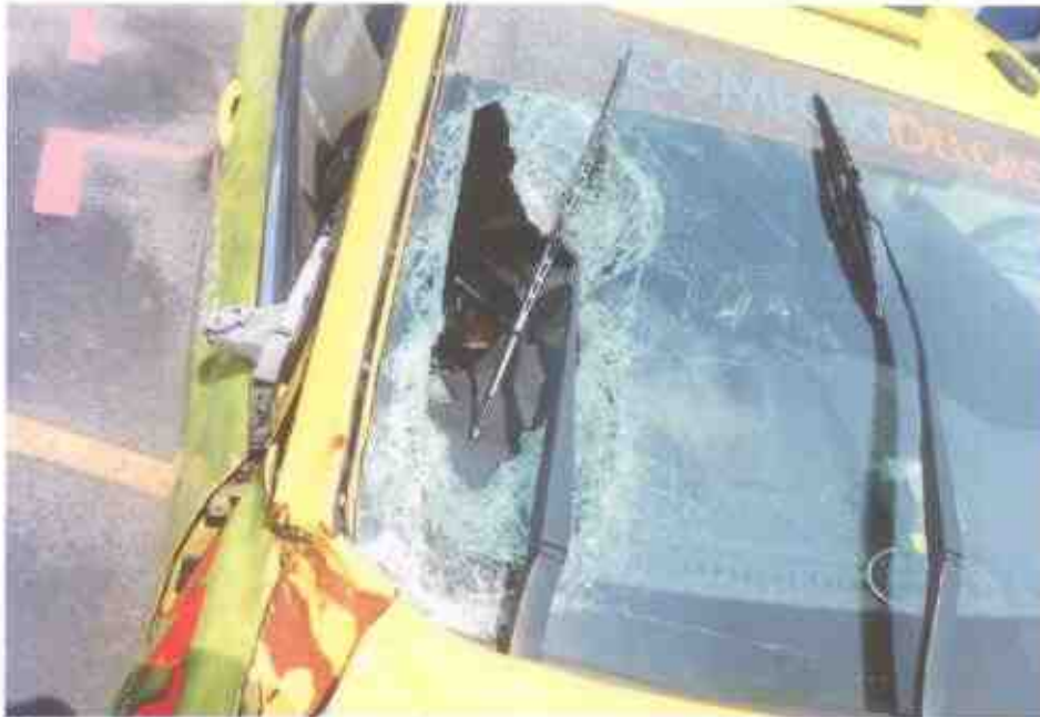
Photo 4 shows a closer view of the damage sustained on the right portion of the Motor Taxi. The impact force was significant, causing the right portion of the windshield to be shattered due to the accident.
