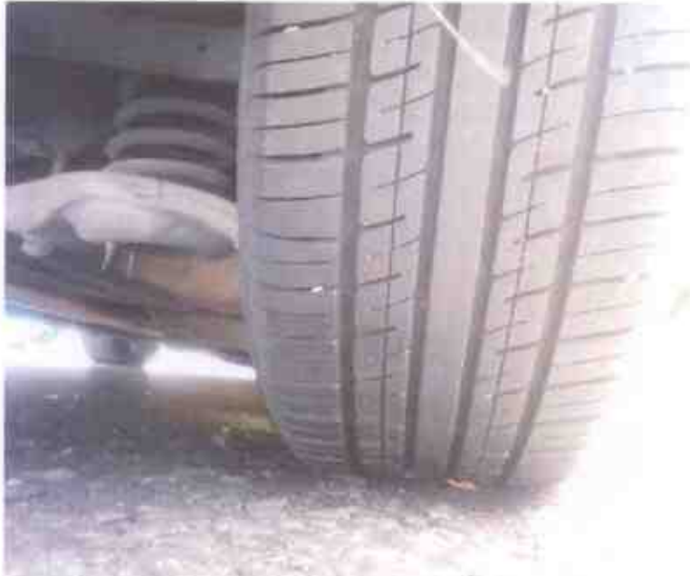
Photo 16 shows the condition of the rear right tyre of the Motor Taxi, which was observed to be in serviceable condition with remaining tread depth of approximately 6mm. There was also no tear, cut or burst mark(s) on the outer and the inner sidewalls as well as across the tread of this tyre.
