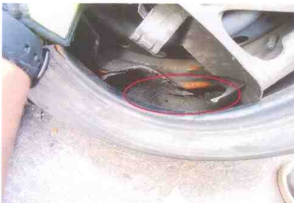
Photo 13 shows the condition of the front right tyre of the Motor Taxi, which was observed to be dislodged as a result of the accident. We did found cut mark on the outer sidewall as well as across the tyre surface which was likely due to the result of the accident.
