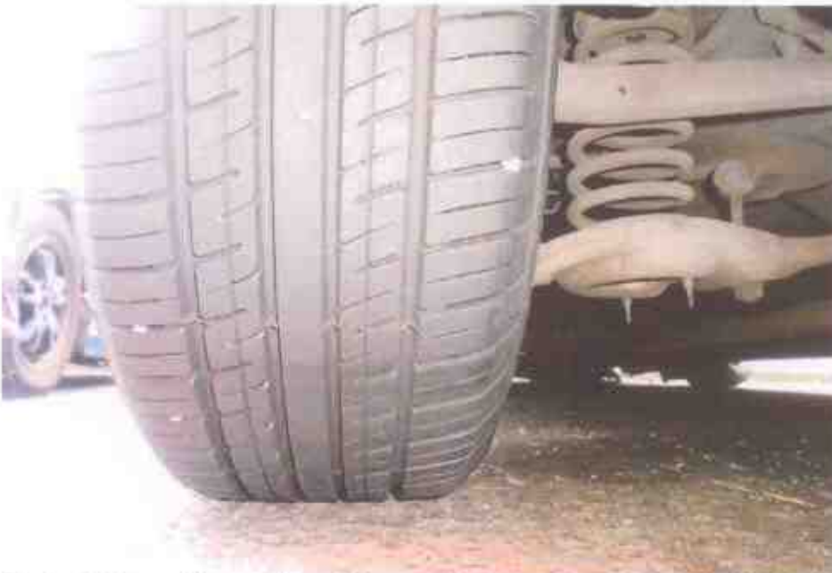
Photo 17 shows the condition of the rear left tyre of the Motor Taxi, which was observed to be in serviceable condition with remaining tread depth of approximately 5mm. There was also no tear, cut or burst mark(s) on the outer and the inner sidewalls as well as across the tread of this tyre.
