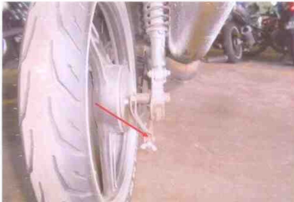
Photo 16 shows our checks on the rear brake component had indicated that the mechanical components were in serviceable condition unaffected by the accident's impact.
