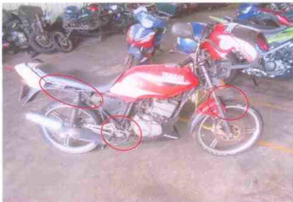
Photo 3 shows a general view of the right body of the Motorcycle at the time of our inspection. The Motorcycle was observed to have sustained damages on the right side fairing, rear brake pedal & mudguard at time of our inspection.
