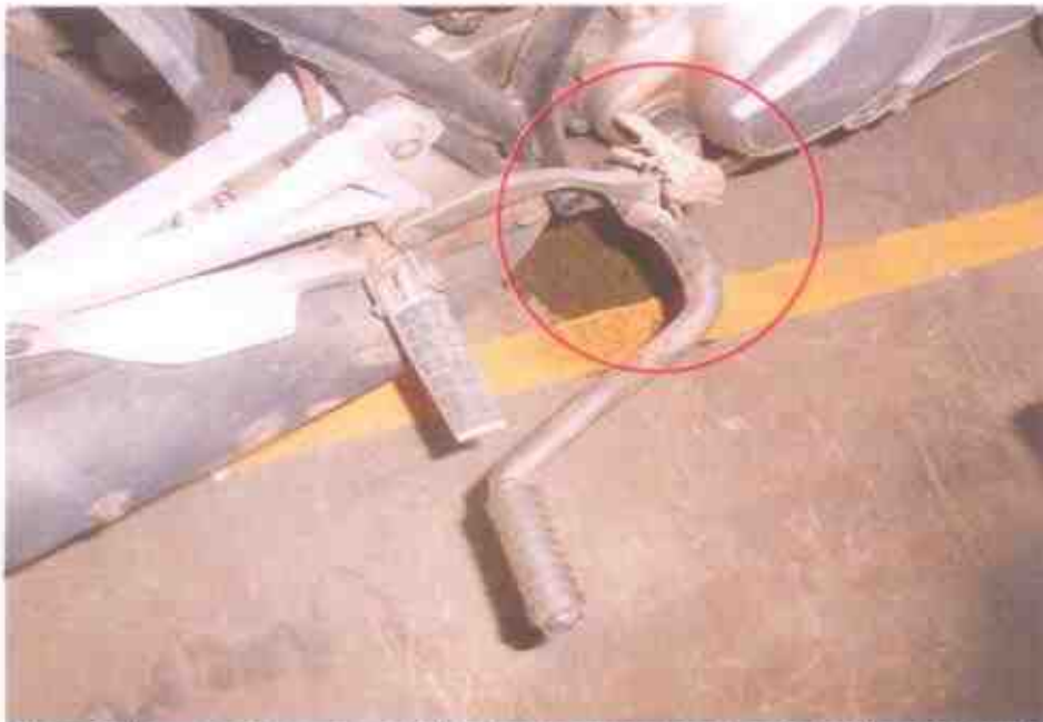
Photo 7 shows a closer view of the damaged rear brake pedal of the Motorcycle at the time of our inspection. The Motorcycle was observed to have sustained with relatively minor damages due to the accident's collision. (Circled)
