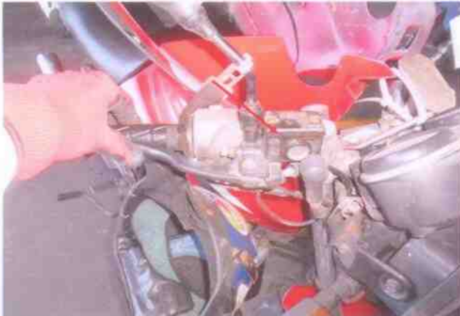
Photo 14 shows our checks on the brake fluid (front) reservoir. It was observed to sustained fluid leakage at the brake fluid reservoir cover. There was no spongy feeling when depressing the brake lever.
