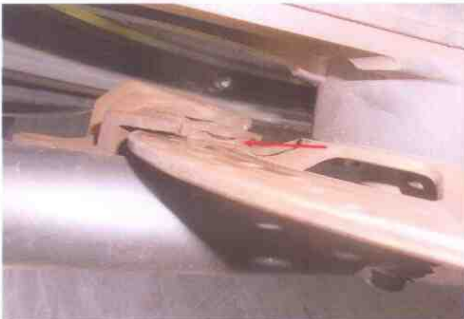
Photo 15 shows the front brake pad at time of our inspection. The frictional material was observed to be sufficient for operational purposes.
