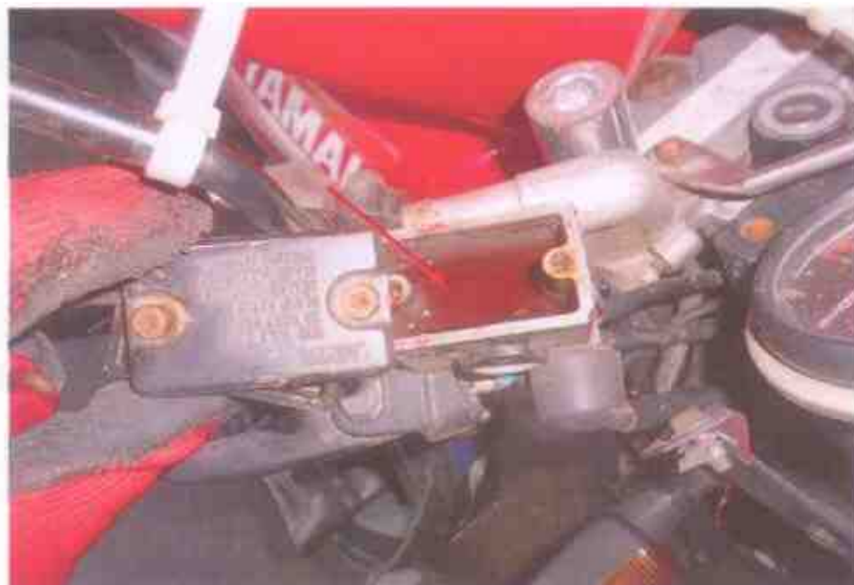
Photo 13 shows our checks on the brake fluid (front) reservoir had indicated that the brake fluid was of sufficient level for operational purposes, and without contamination.
