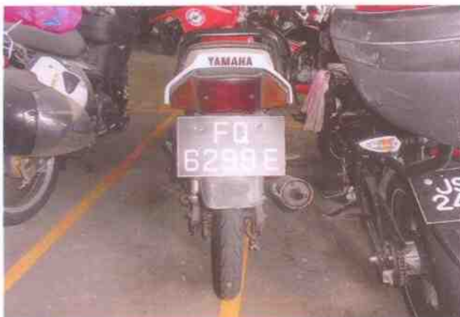
Photo 4 shows a general view of the rear body of the Motorcycle at the time of our inspection. The Motorcycle was observed to be in good condition unaffected by the accident.
