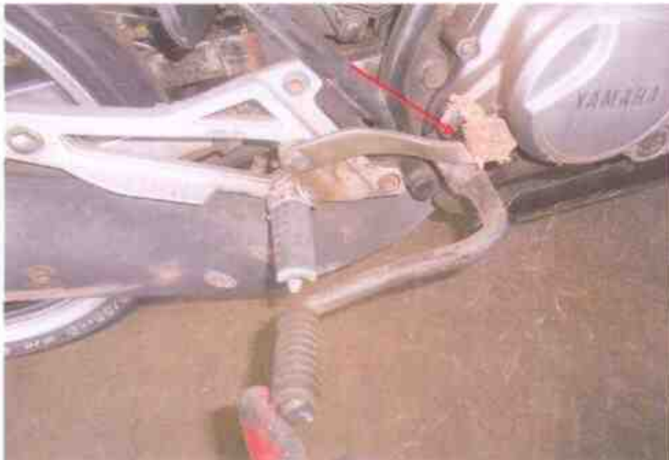
Photo 17 shows the rear brake pedal was stuck likely due to the accident's impact collision.
