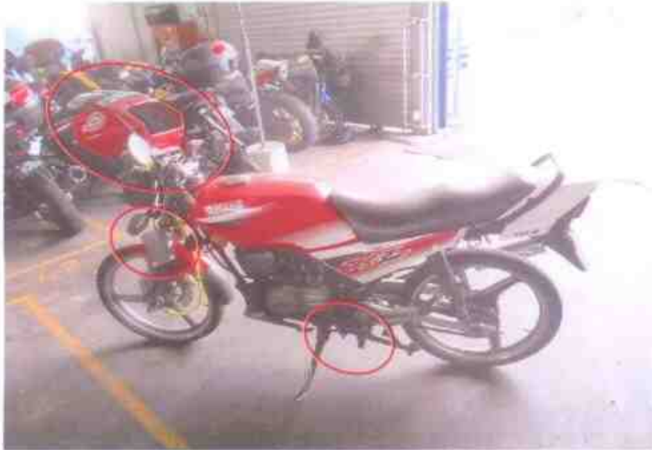
Photo 5 shows a general view of the left body of the Motorcycle at the time of our inspection. The Motorcycle was observed to have sustained damages on the front fairing, IU & foot rest amongst others at time of our inspection.
