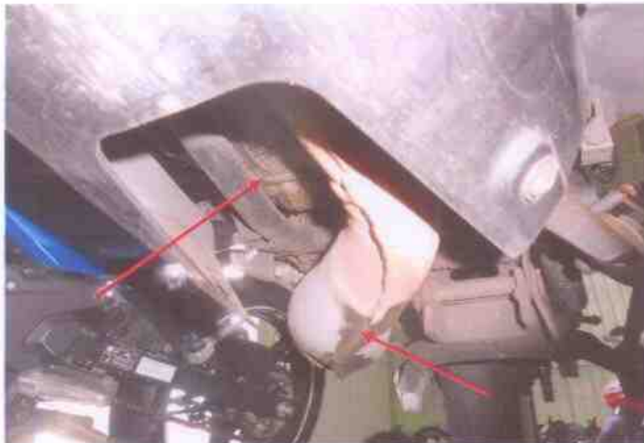
Photo 10 shows sign(s) or indication(s) of fluid leak observed around the underside of the engine area of the Motorcycle. Traces of fluid leakage was also observed on the exhaust pipe.
