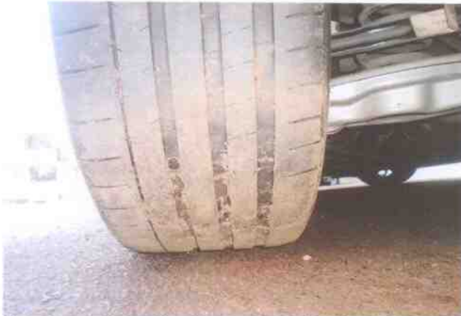
Photo 10 shows the condition of the rear left tyre of the Motor Car, which was observed to be in serviceable condition with remaining tread depth of approximately 4mm.
