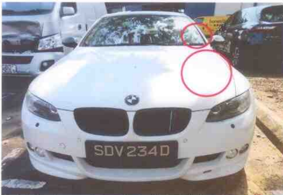
Photo 2 shows a general view of the front body of the Motor Car at the time of our inspection. The Motor Car was observed to have sustained a relatively minor impact damages that was confined to its frontal portion. Its front left bonnet was corrugated & its shattered windshield was observed to be affected likely due to the accident.
