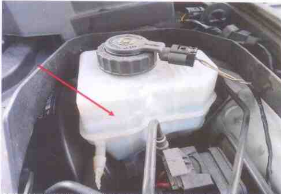
Photo 13 shows the brake fluid reservoir of the Motor Car at the time of our inspection. The brake fluid was observed to be of sufficient level (arrowed) and without any visible contamination.
