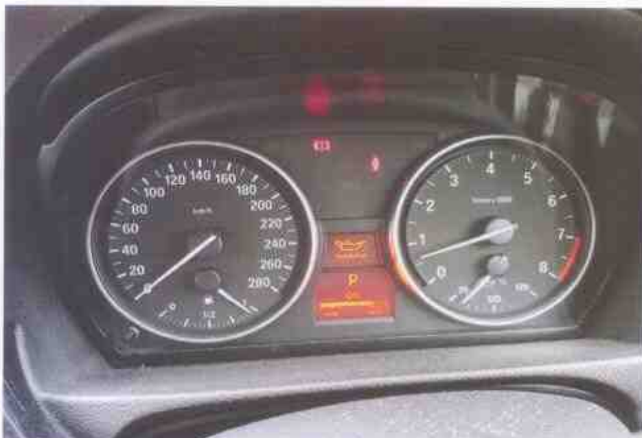
Photo 16 shows the engine fluid indication on the system of the Motor Car at the time of our inspection. The engine oil was observed to be of sufficient level from the system reading.
