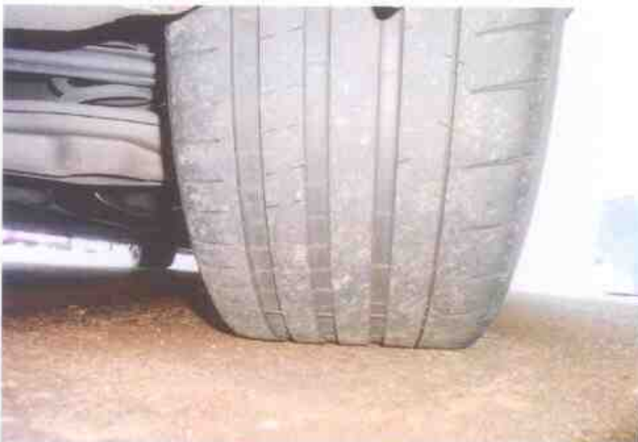
Photo 11 shows the condition of the rear right tyre of the Motor Car, which was observed to be in serviceable condition with remaining tread depth of approximately 4mm.
