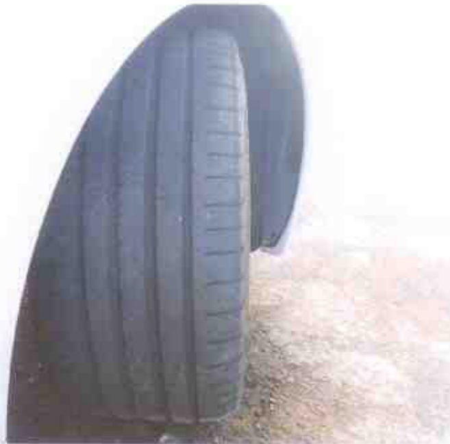
Photo 8 shows the condition of the front right tyre of the Motor Car, which was observed to be in serviceable condition with remaining tread depth of approximately 6mm. The tyre, which was wrapped around alloy wheel rim, was also observed to be sufficiently inflated for vehicular operation.
