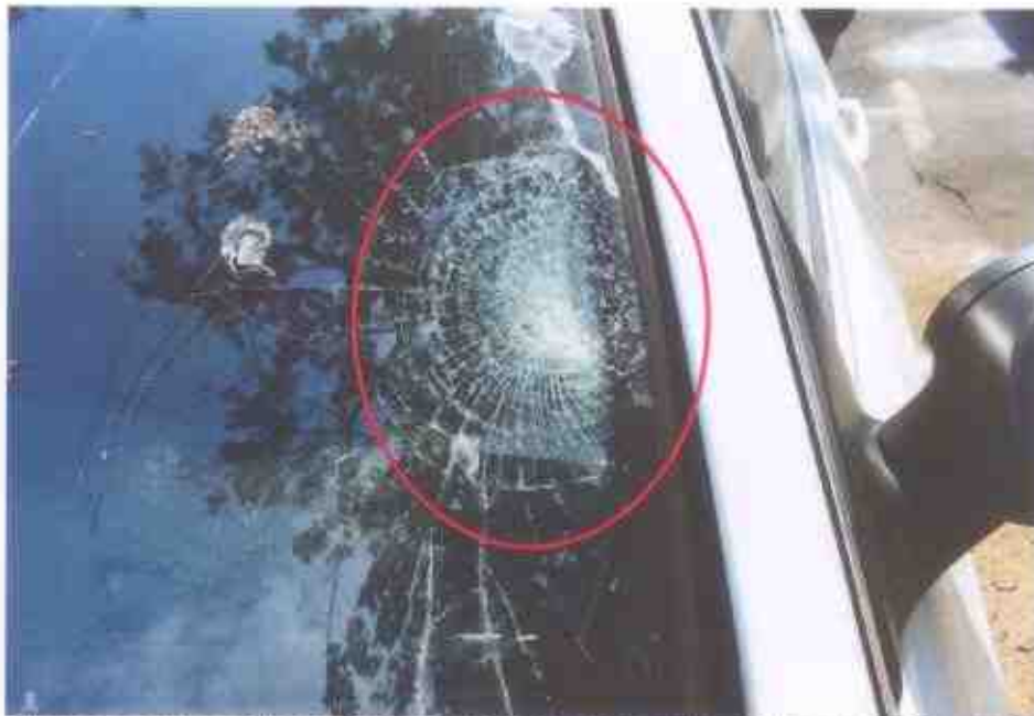
Photo 7 shows a close up view of the front left portion of the Motor Car at the time of our inspection. The Motor Car had sustained shattering cracked at the front left portion of the Motor Car.
