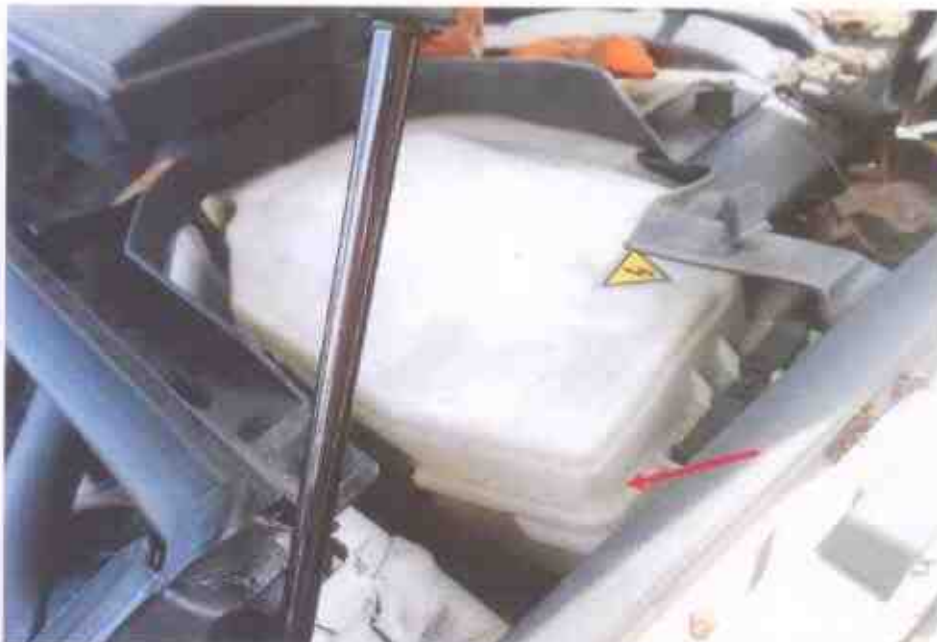
Photo 14 shows the engine coolant fluid reservoir of the Motor Car at the time of our inspection. The engine coolant fluid was observed to be of sufficient level and without any visible contamination.
