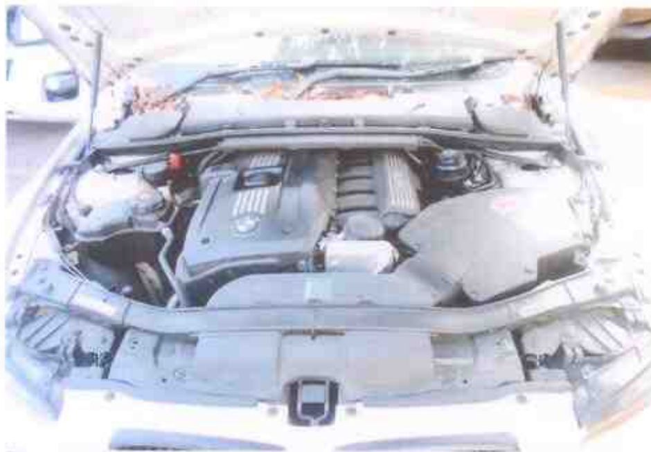
Photo 12 shows a general view of the Motor Car's engine compartment. The various parts and components inside the engine compartment were unaffected by the accident. There was also no sign(s) or indication(s) of fresh fluid leakage and/or fluid stain within the engine compartment.
