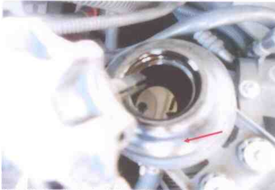
Photo 15 shows the steering fluid reservoir of the Motor Car at the time of our inspection. It was observed to be of sufficient level and without any visible contamination.
