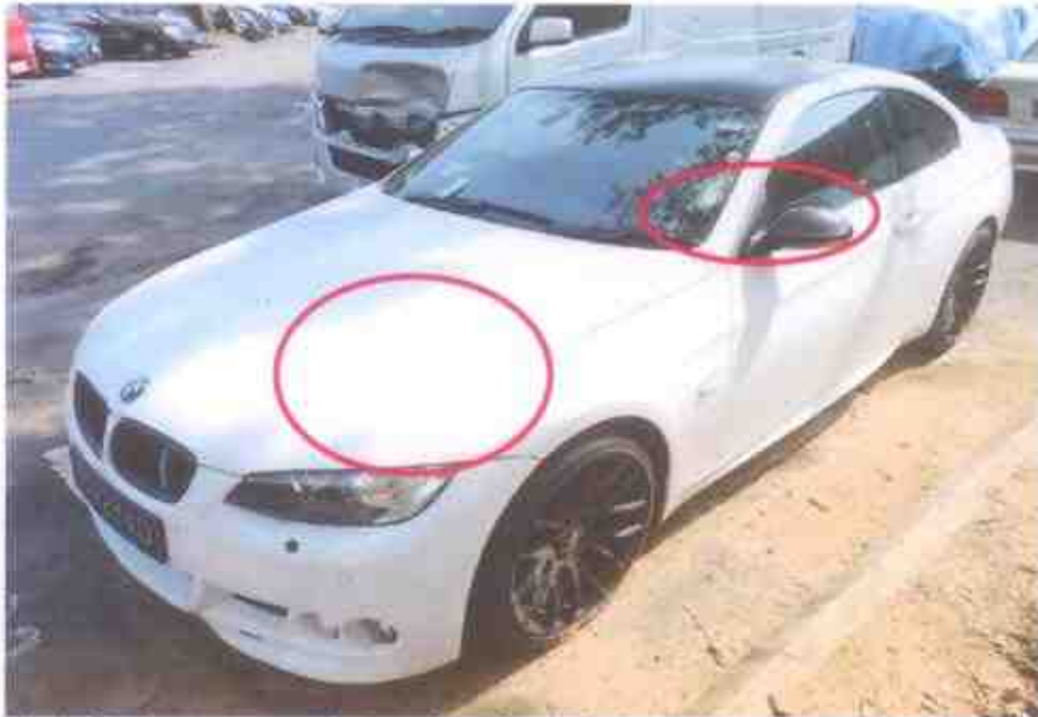
Photo 3 shows a general view of the front left body of the Motor Car at the time of our inspection. The Motor Car was observed to have sustained a relatively minor impact damages that was confined to its frontal portion. Its front left bonnet was corrugated & its shattered windshield was observed to be affected likely due to the accident.
