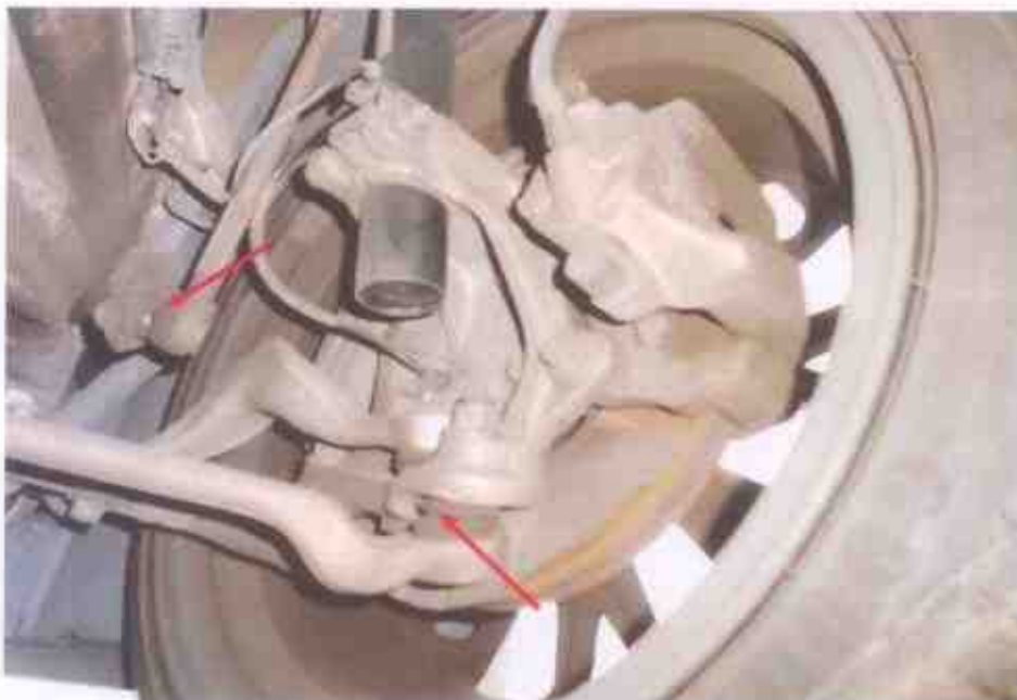
Photo 19 shows the various undercarriage components at the front right wheel of the Motor Car, in particular the steering tie rod (arrowed). The various steering components were all found to be intact, suggesting that the steering system of the Motor Car was likely to be in serviceable condition.
