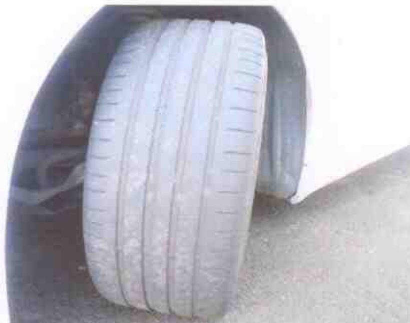
Photo 9 shows the condition of the front left tyre of the Motor Car, which was observed to be in serviceable condition with remaining tread depth of approximately 6mm. The tyre, which was wrapped around alloy wheel rim, was also observed to be sufficiently inflated for vehicular operation.
