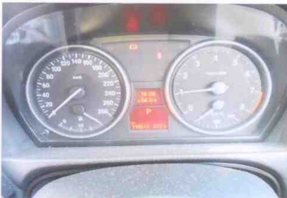
Photo 22 shows most warning lights disappearing from the instrument panel of the Motor Car after the engine was cranked.
