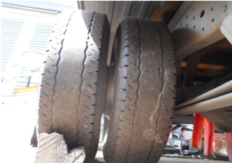
Photo 6 shows the rear right tyres of the insured vehicle at the time of my inspection. The pattern of the tread at the centre area of both rear right tyres were observed to be no longer visible. This was around the entire circumference of both the rear right tyres, and was largely due to the rubber wearing off. The pattern of the tread at the outer side of both these tyres were however still visible. Both these tyres were found to be sufficiently inflated for vehicular operation and without any tear, cut or burst mark(s) on the outer and the inner sidewalls as well as across the tread.
