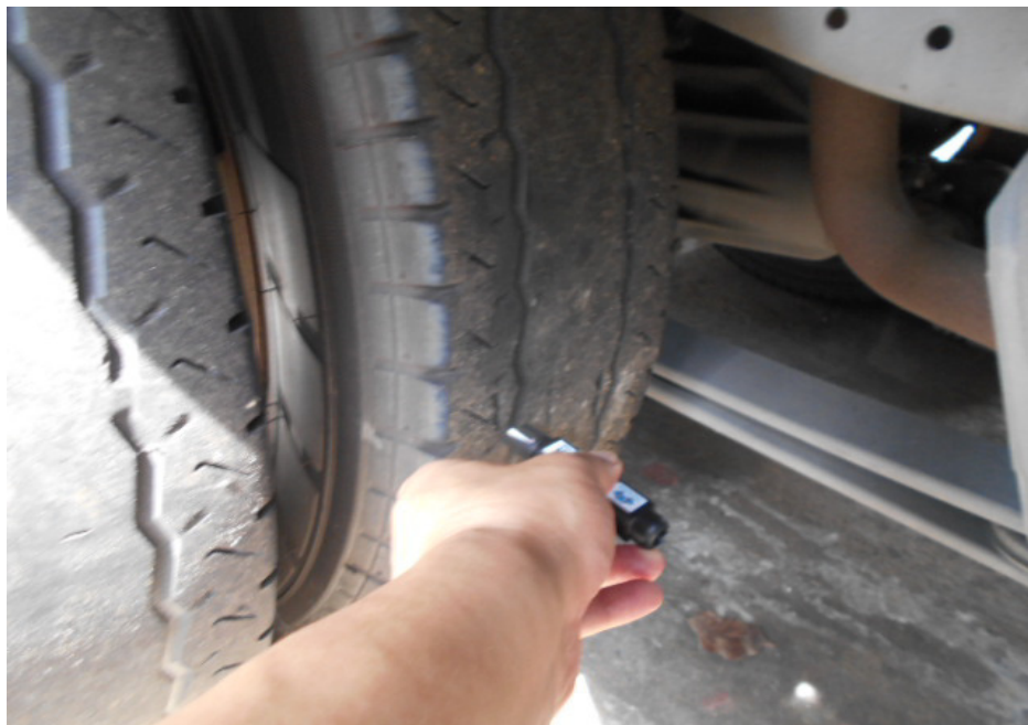
Photo 7 shows measurement being carried out to the remaining tread depth of the insured vehicle's rear right tyres.
