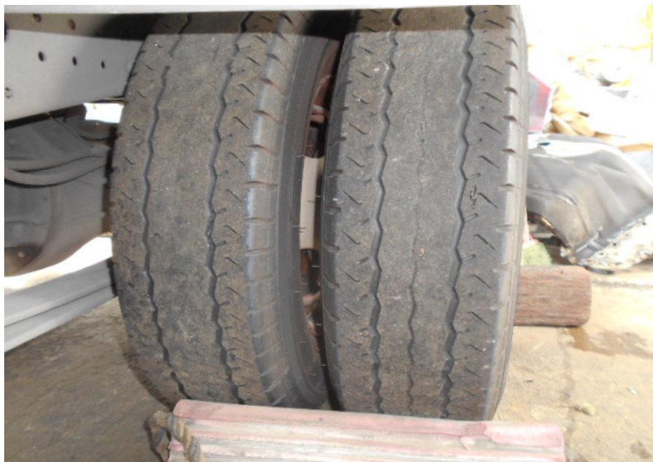
Photo 10 shows the rear left tyres of the insured vehicle at the time of my inspection. The pattern of the tread at the centre area of both rear left tyres were observed to be no longer visible at some areas due to the rubber wearing off. The pattern of the tread at the outer side of both these tyres were however still visible. Both these tyres were found to be sufficiently inflated for vehicular operation and without any tear, cut or burst mark(s) on the outer and the inner sidewalls as well as across the tread. The overall condition of the rear left tyres of the insured vehicle was slightly less worn as compared to the rear right tyres.
