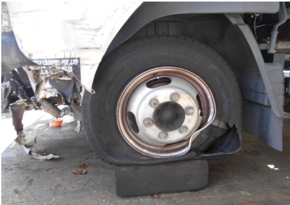
Photo 2 shows a general view of the front left tyre and front left wheel rim of the insured vehicle. The front left wheel rim was observed to be dented. A hole was also observed on the outer sidewall of the front left tyre. These were damages arising from the accident impact. As a result, the front left tyre was punctured.
