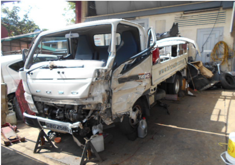
Photo 1 shows a general view of the front left body of the insured vehicle at the time of my inspection. The front bumper, front panel, front grille, front left headlamp and front left door were amongst the exterior body parts that had sustained impact damages as a result of the accident.
