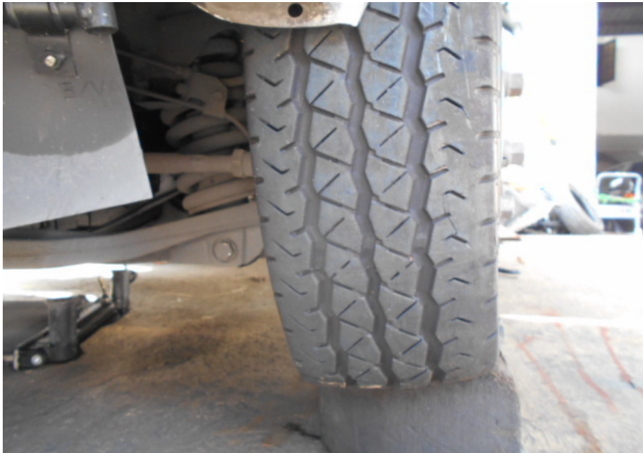
Photo 3 shows the condition of the front left tyre of the insured vehicle, which was observed to be in serviceable condition with remaining tread depth of approximately 5mm. It was however punctured as a result of the accident impact (see photograph 2 above).
