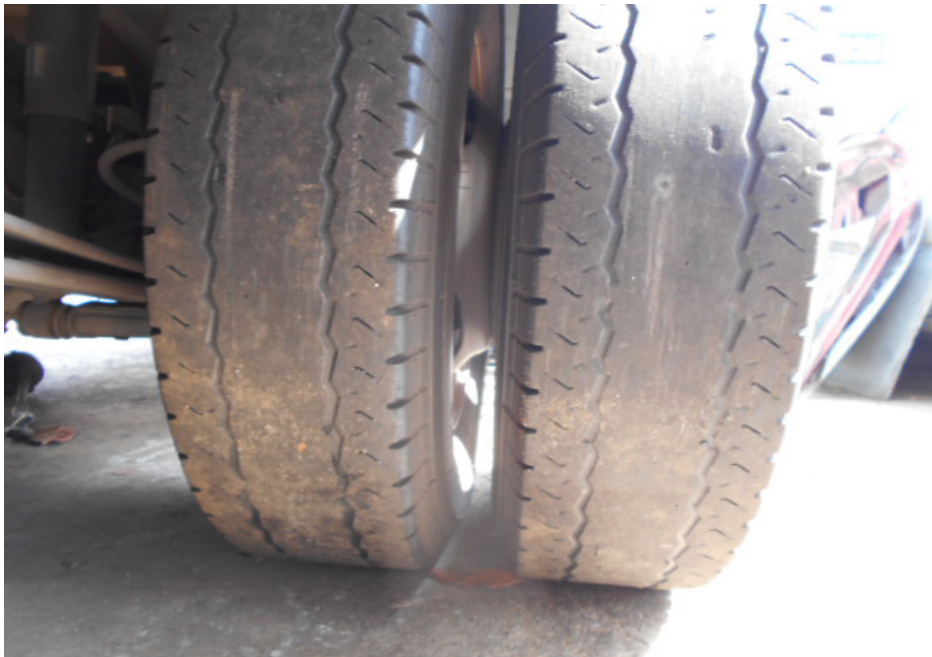
Photo 5 shows the rear right tyres of the insured vehicle at the time of my inspection. The pattern of the tread at the centre area of both rear right tyres were observed to be no longer visible. This was around the entire circumference of both the rear right tyres, and was largely due to the rubber wearing off. The pattern of the tread at the outer side of both these tyres were however still visible. Both these tyres were found to be sufficiently inflated for vehicular operation and without any tear, cut or burst mark(s) on the outer and the inner sidewalls as well as across the tread.
