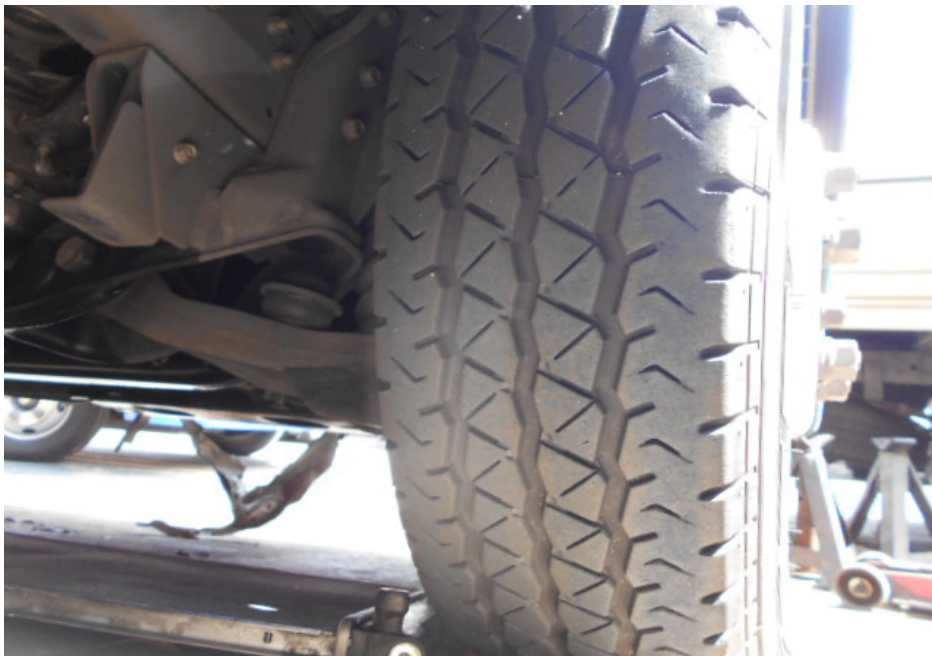
Photo 4 shows the condition of the front right tyre of the insured vehicle, which was observed to be in serviceable condition with remaining tread depth of approximately 5mm. The front right tyre was also observed to be sufficiently inflated for vehicular operation with no tear, cut or burst mark(s) on its outer and inner sidewalls, as well as across its tread.
