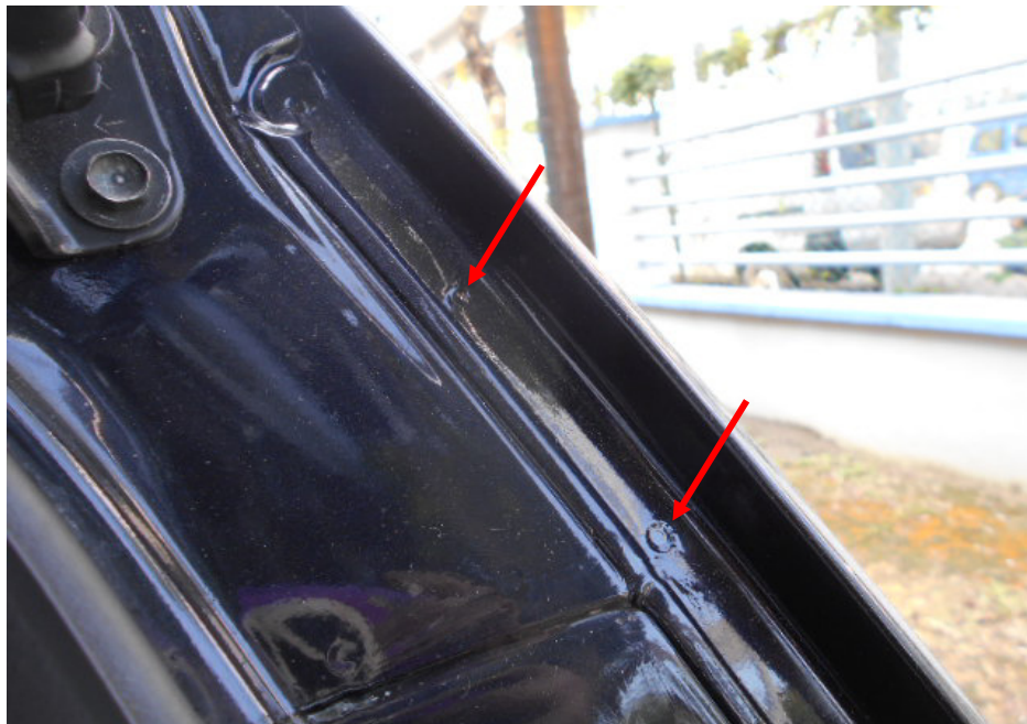
Photo 15 shows the original spot weld marks (arrowed) on the rear right fender of the Motor Car. The body panels of the Motor Car were found to be with original welding marks except for the rear left fender of the Motor Car, where signs of removal and re-fitting were found (refer to photograph 16 below).
