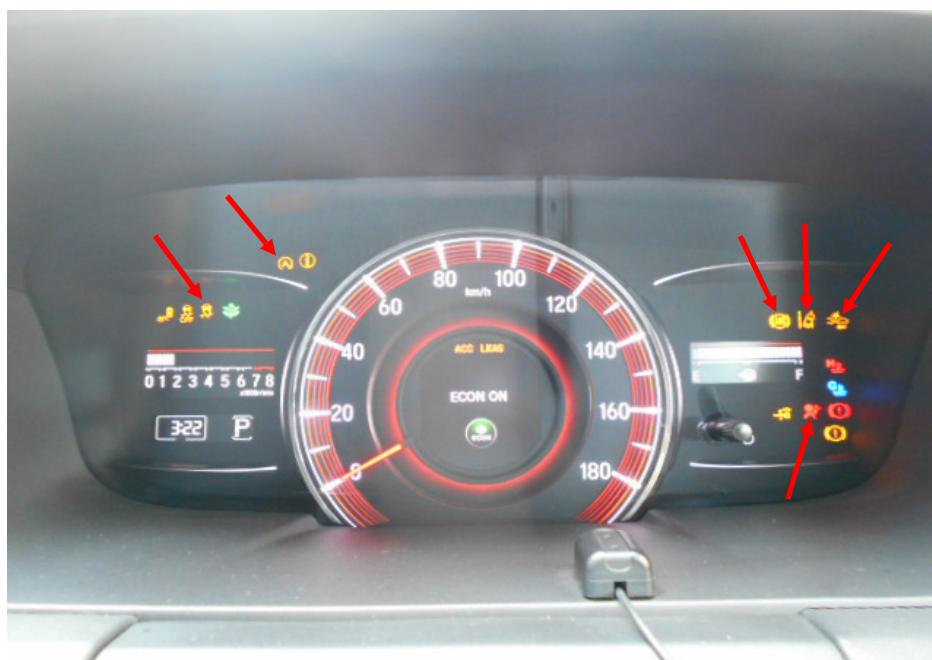
Photo 6 shows the warning lights for the various electronic safety features (arrowed) appearing on the instrument panel of the Motor Car during its self-test when the engine is cranked, in particular the Anti-Brake Lock System (ABS), Supplemental Restraint System (SRS), Electronic Power Steering (EPS), Collision Mitigation Braking System (CMBS), Lane Departure Warning (LDW) and Vehicle Stability Assist (VSA).
