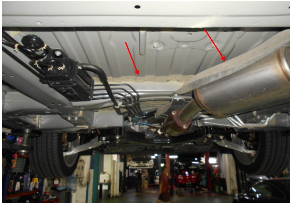
Photo 14 shows the structural body at the centre of the Motor Car. The joints (arrowed) along the chassis body was also untouched, indicating no work was done on the chassis body of the Motor Car and that the chassis body was originally fitted.
