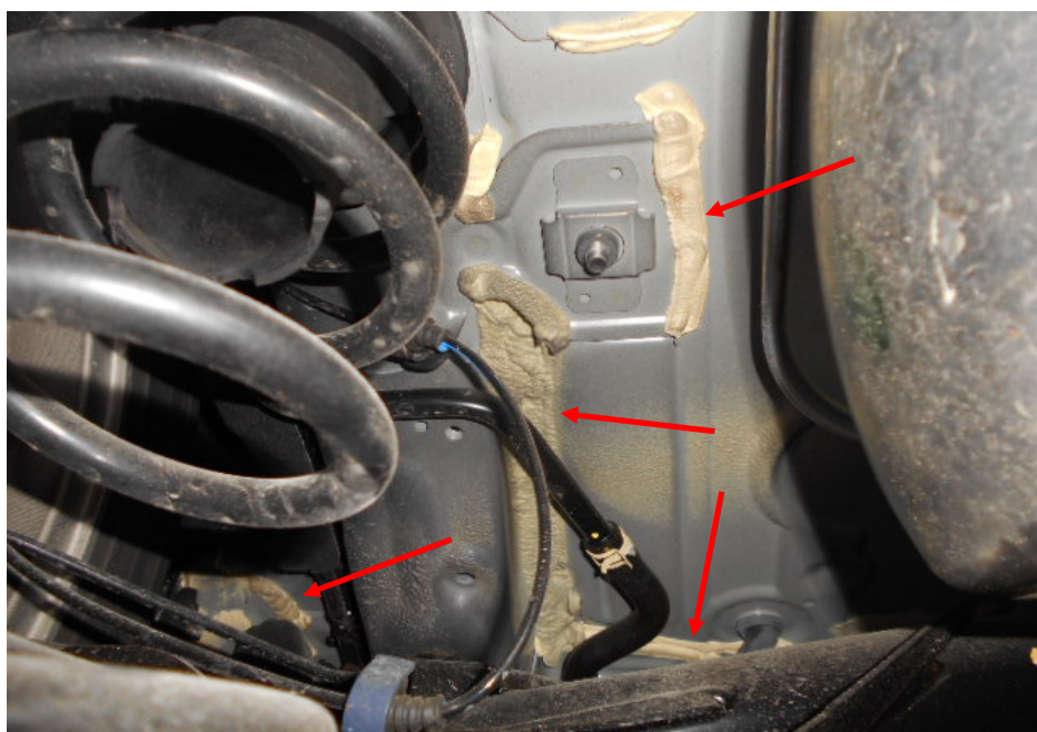
Photo 13 shows the structural body at the left rear of the Motor Car. Visually, I did not find any weld marks other than original spot weld marks on the chassis of the Motor Car. The joints (arrowed) along the chassis body was also untouched, indicating no work was done on the chassis body of the Motor Car and that the chassis body was originally fitted.
