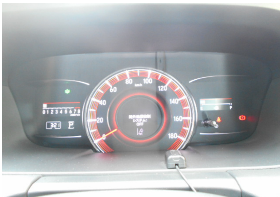
Photo 7 shows the respective warning lights no longer illuminated, indicating that there is no fault detected to the ABS, SRS, EPS, CMBS, LDW and VSA systems of the Motor Car during the self-test. These electronic systems were hence in working condition at the time of my inspection.
