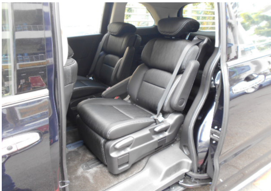
Photo 5 shows the rear seats of the Motor Car, which were secured via seat rails to the floor board. All the seats of the Motor Car were fitted with a retractable seat belt reel and pre-tensioner. The seat belts were also able to be fastened to the pretension that were fitted on the side of each individual seat.
