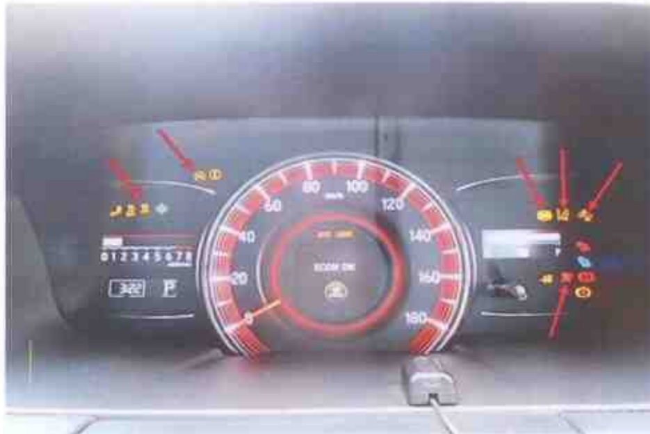
Photo 6 shows the warning lights for the various electronic safety features (arrowed) appearing on the instrument panel of the Motor Car during its self-test when the engine is cranked, in particular the Anti-Brake Lock System (ABS), Supplemental Restraint System (SRS), Electronic Power Steering (EPS), Collision Mitigation Braking System (CMBS), Lane Departure Warning (LDW) and Vehicle Stability Assist (VSA).
