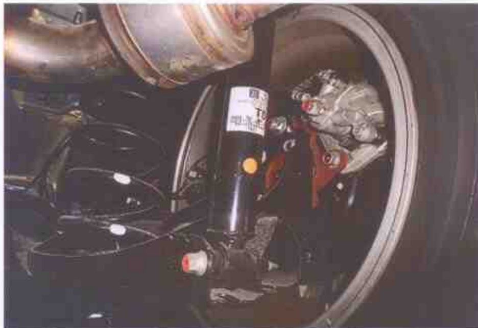
Photo 9 shows a general view of the control arms and linkages at the rear right wheel of the Motor Car. I did not observe any fluid leak and/or fluid stain on the underside of the Motor Car. All of the Motor Car's undercarriage components were observed to be intact and secured in an appropriate manner.
