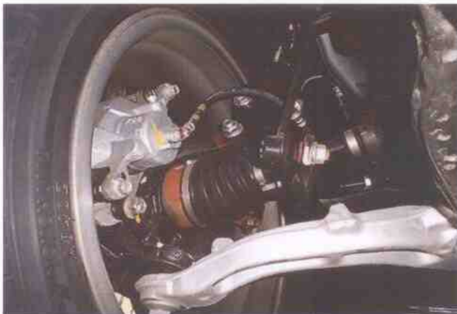
Photo 11 shows the various undercarriage components at the front right wheel of the Motor Car. The mechanical components, control arms and linkages were all found to be intact and secured in an appropriate manner.
