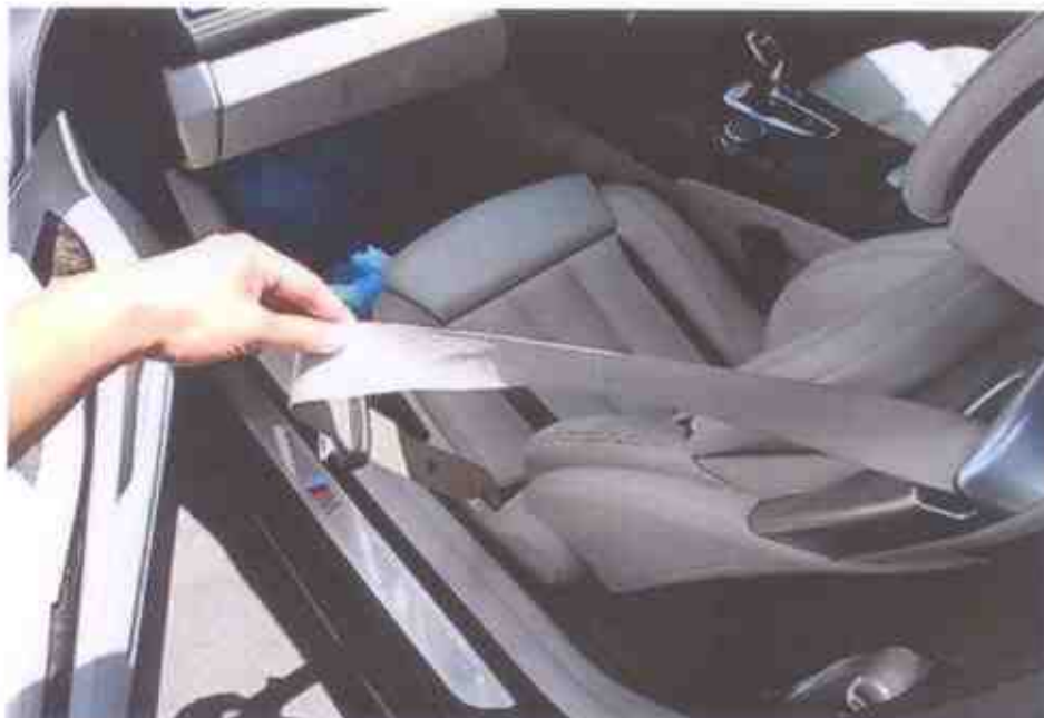
Photo 5 shows the front left seat of the Motor Car, which were secured via seat rails to the floor board. All the seats of the Motor Car were fitted with a retractable seat belt reel and pre-tensioner. The seat belts were also able to be fastened to the pretension that were fitted on the side of each individual seat.
