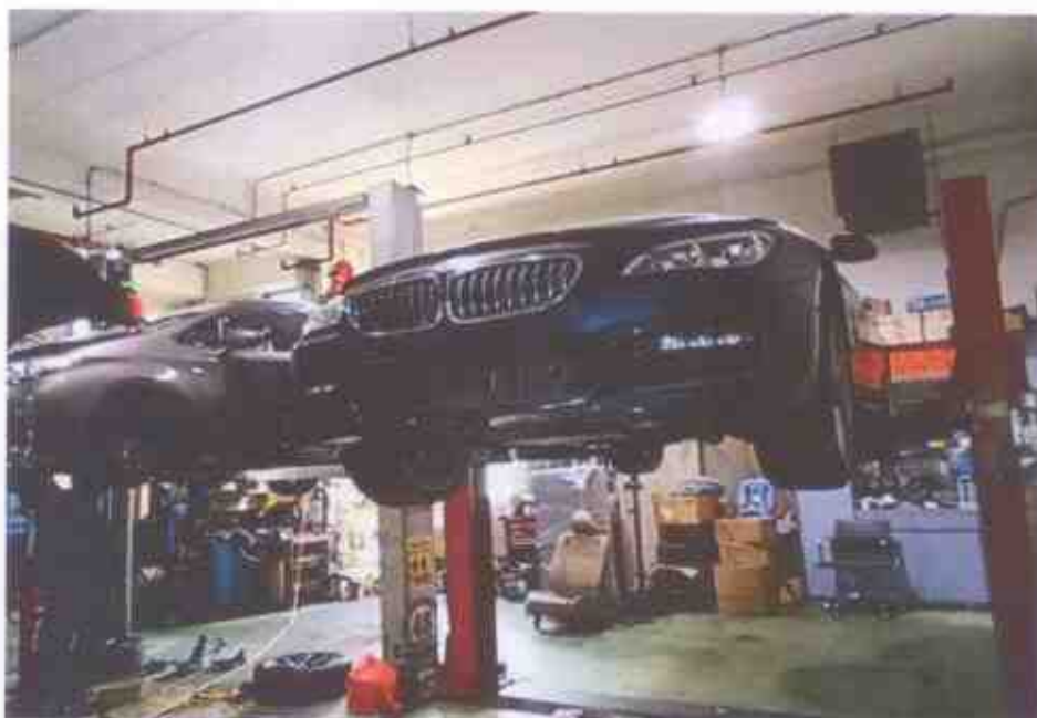
Photo 9 shows the Motor Car hoisted up for checks on its undercarriage. There was no sign(s) or indication(s) of fluid leakage and/or fluid stain(s). The undercarriage components of the Motor Car were also all observed to be intact and secured in an appropriate manner.
