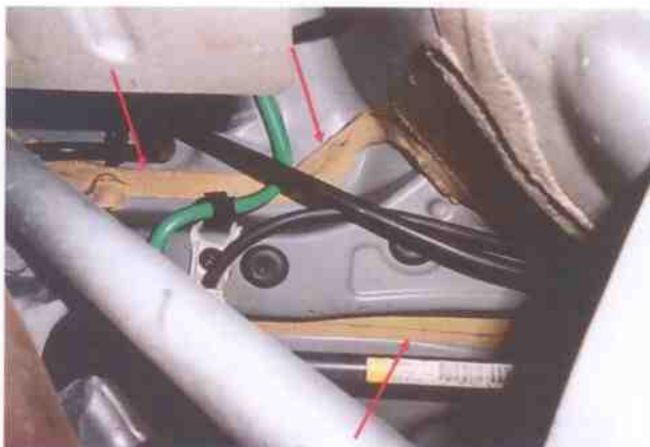
Photo 13 shows the structural body at the left rear of the Motor Car. Visually, I did not find any weld marks other than original spot weld marks on the chassis body of the Motor Car. The joints (arrowed) along the chassis body was also untouched, indicating no work was done on the chassis body of the Motor Car and that the chassis body was originally fitted.
