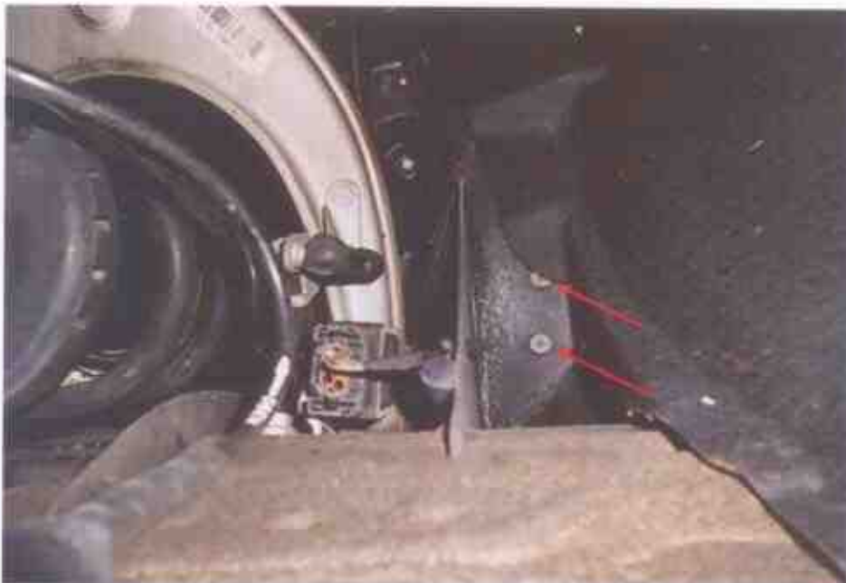
Photo 15 shows the structural body at the front left of the Motor Car. Visually, I did not find any weld marks other than original spot weld marks (arrowed) on the chassis of the Motor Car, indicating no work was done on the chassis body of the Motor Car and that the chassis body was originally fitted.
