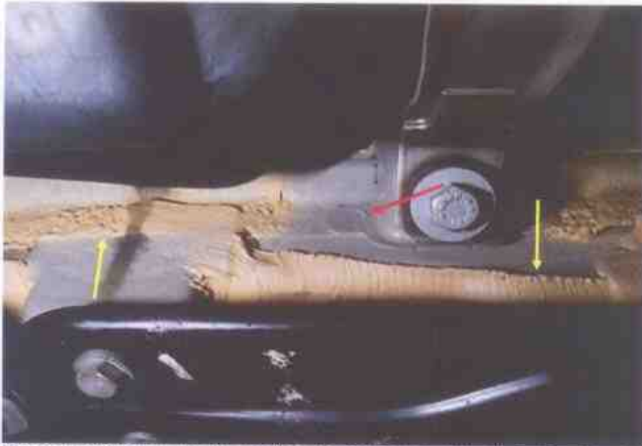
Photo 14 shows the structural body at the right centre of the Motor Car. Visually, I did not find any weld marks other than original spot weld marks (red arrow) on the chassis of the Motor Car. The joints (yellow arrow) along the chassis body was also untouched, indicating no work was done on the chassis body of the Motor Car and that the chassis body was originally fitted.
