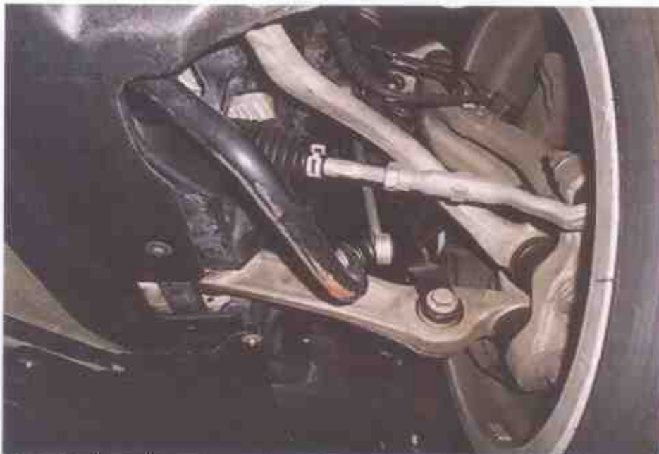
Photo 11 shows the various undercarriage components at the front left wheel of the Motor Car. The mechanical components, control arms and linkages were all found to be intact and secured in an appropriate manner.
