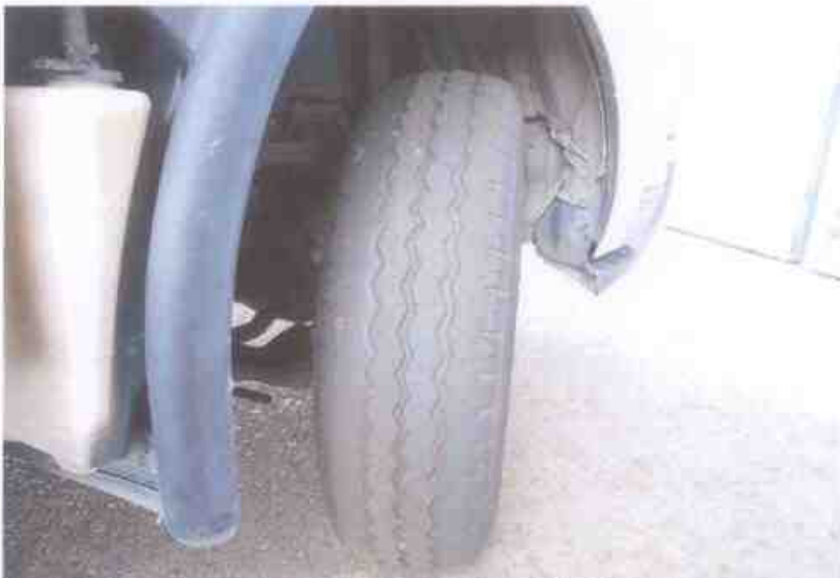
Photo 9 shows the condition of the front right tyre of the Motor Lorry, which was observed to be in serviceable condition with remaining tread depth of approximately 4mm. The tyre, which was wrapped around standard alloy wheel rim, was also observed to be sufficiently inflated for vehicular operation.
