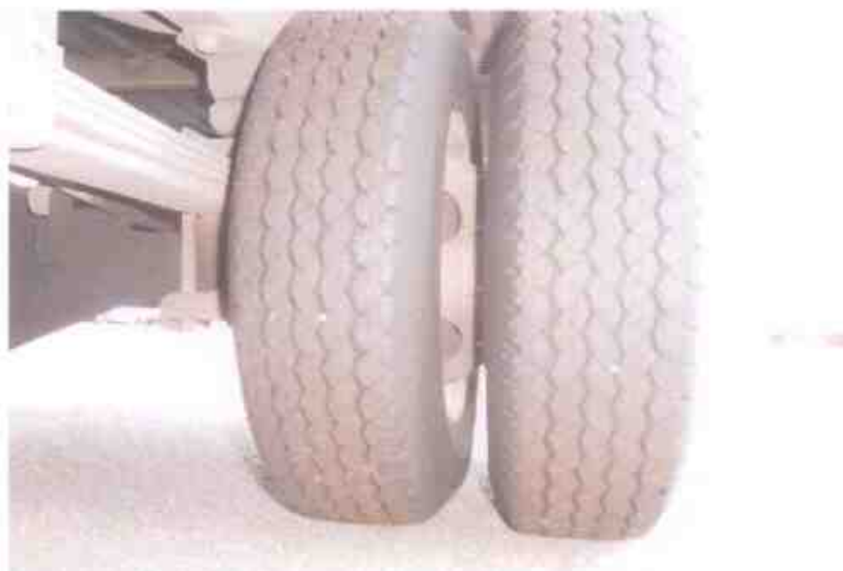
Photo 10 shows the condition of the rear left tyres of the Motor Lorry, which was observed to be in serviceable condition with remaining tread depth of approximately 5mm. The tyres, which were wrapped around standard alloy wheel rim, were also observed to be sufficiently inflated for vehicular operation,
