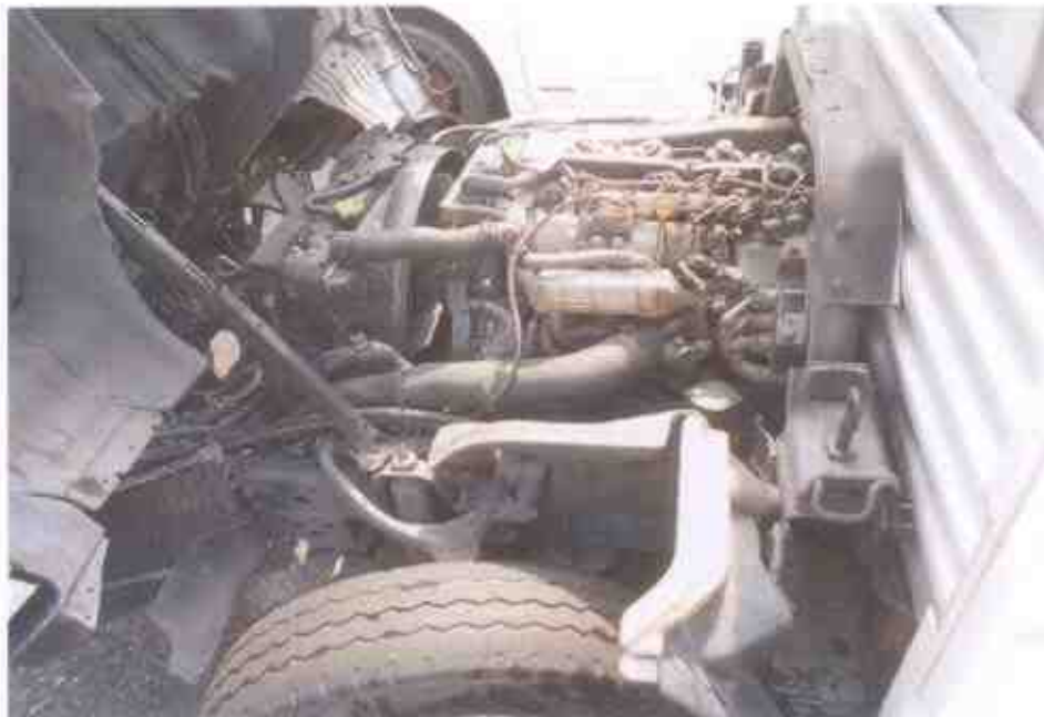
Photo 12 shows a general view of the Motor Lorry's engine compartment, which was accessed by lifting the front cabin of the Motor Lorry. The various parts and components inside the engine compartment were unaffected by the accident. There was also no sign(s) or indication(s) of fresh fluid leakage and/or fluid stain within the engine.
