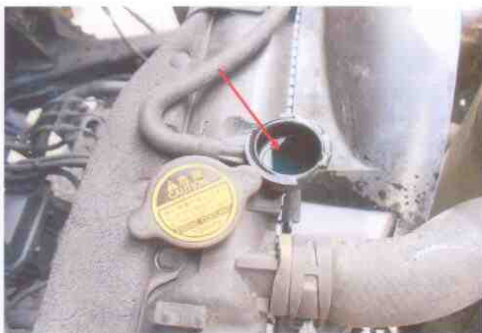
Photo 14 shows the engine coolant reservoir of the Motor Lorry at the time of our inspection. The engine coolant was observed to be of sufficient level and without any visible contamination (arrowed).
