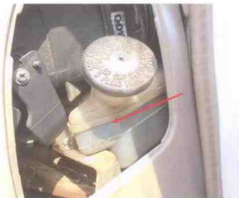
Photo 13 shows the brake fluid reservoir of the Motor Lorry at the time of our inspection. The brake fluid was observed to be of sufficient level and without any visible contamination (arrowed).
