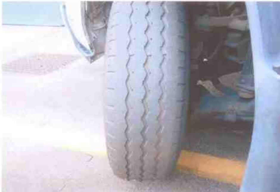
Photo 8 shows the condition of the front left tyre of the Motor Lorry, which was observed to be in serviceable condition with remaining tread depth of approximately 5mm. The tyre, which was wrapped around standard alloy wheel rim, was also observed to be sufficiently inflated for vehicular operation.
