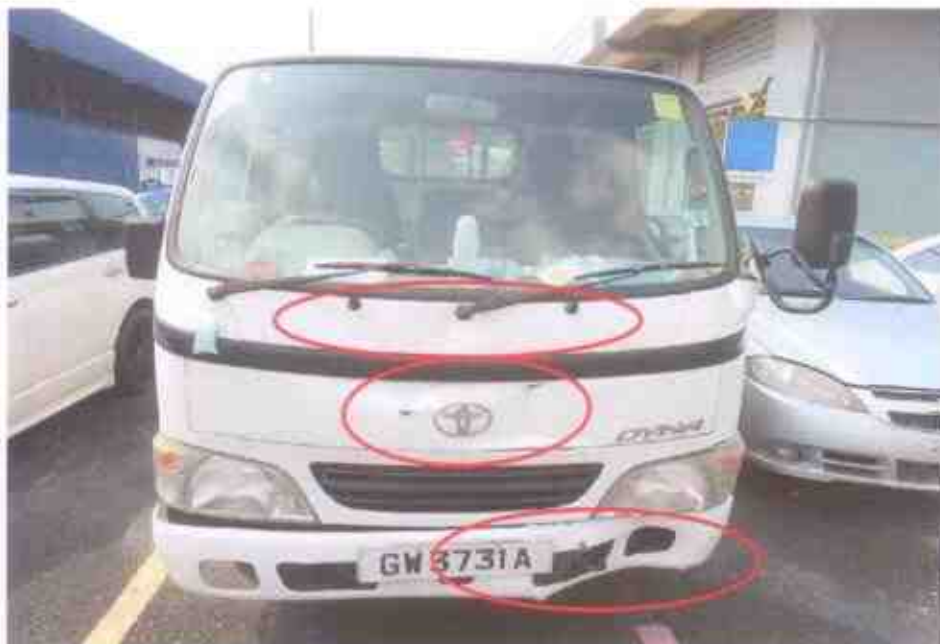
Photo 2 shows a general view of the front portion of the Motor Lorry at the time of our inspection. The Motor Lorry was observed to have sustained minor damage at its front lower bumper and its front panel were amongst the body parts that were damaged as a result of the accident.
