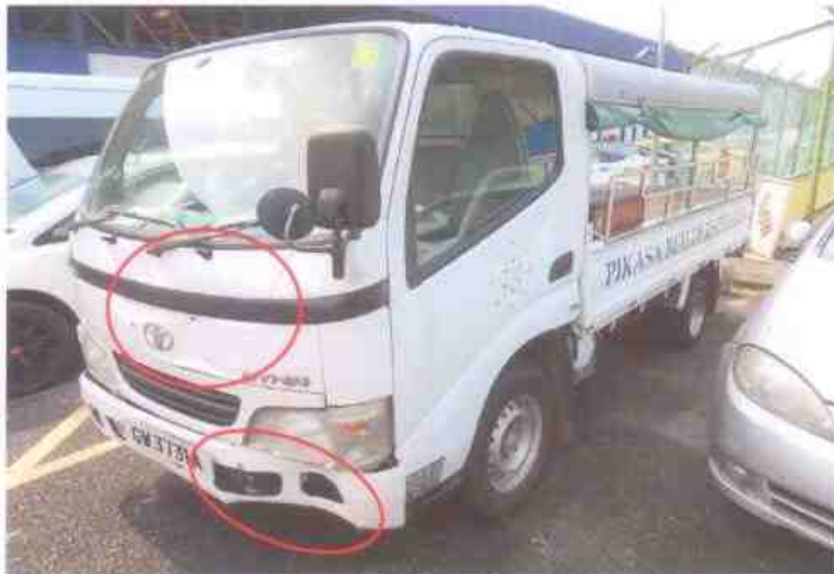
Photo 3 shows a general view of the front left portion of the Motor Lorry at the time of our inspection. The Motor Lorry was observed to have sustained minor damage at its front lower bumper and its front panel were amongst the body parts that were damaged as a result of the accident.
