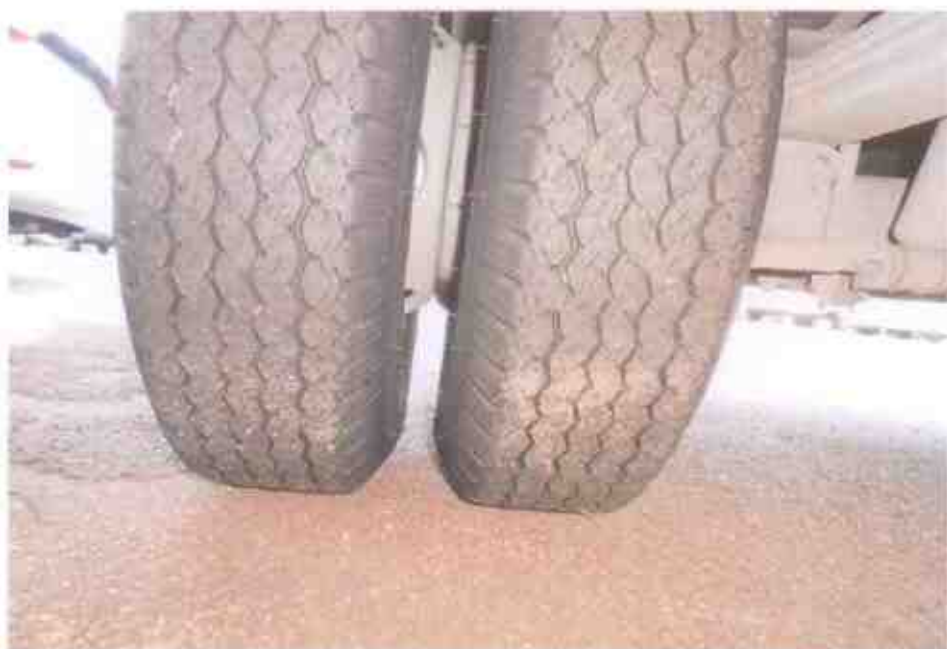
Photo 11 shows the condition of the rear right tyres of the Motor Lorry, which were observed to be in serviceable condition with remaining tread depth of approximately 5mm.
