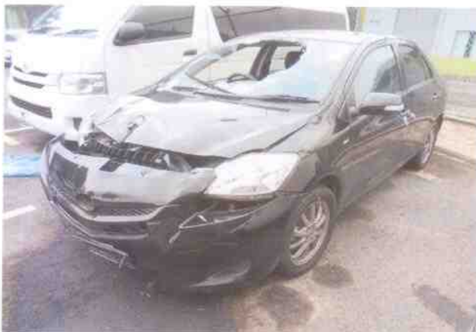
Photo 3 shows a general view of the front left portion of the Motor Car at the time of our inspection. The Motor Car was observed to have sustained extensive impact damage at its front left portion.
