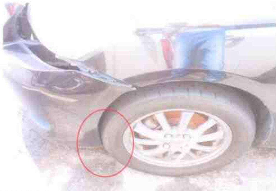
Photo 18 shows the stuck lower bumper & the front tyre as a result of the accident's impact.
