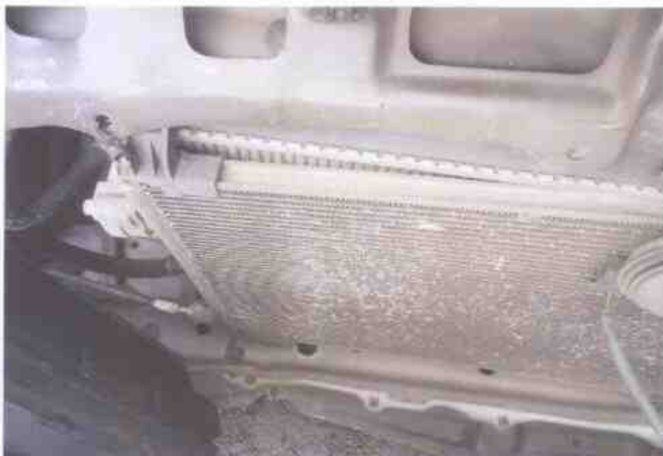
Photo 16 shows the close up view of the damaged radiator as a result of the accident.
