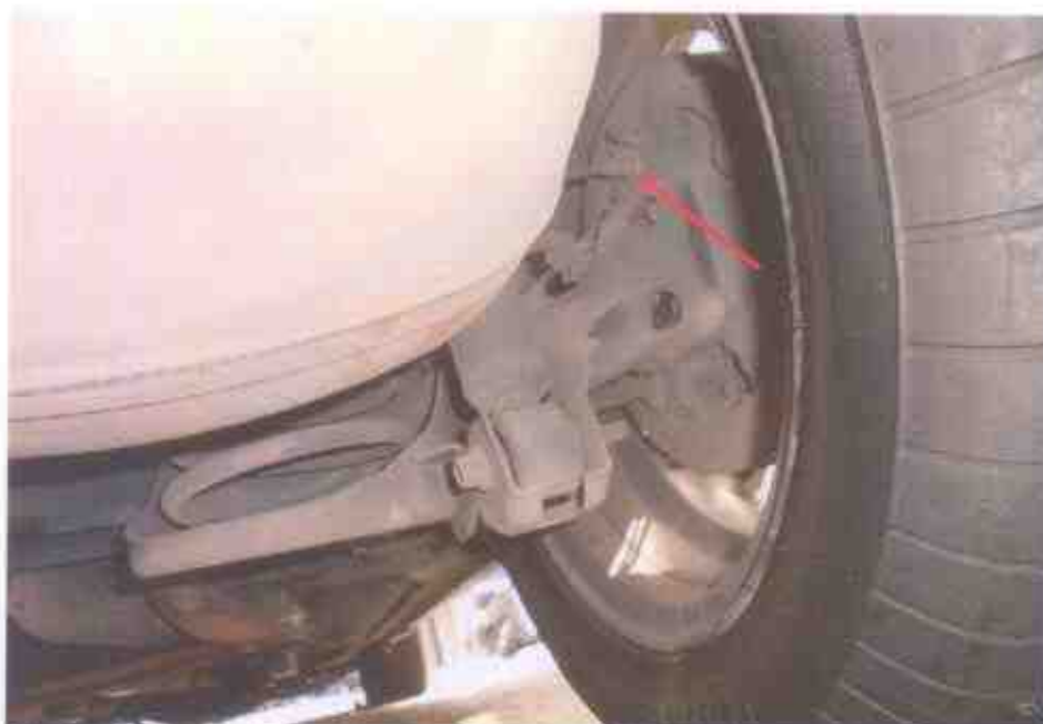
Photo 21 shows the braking components at the rear right wheel of the Motor Taxi. We did not observe any leakage of brake fluid at the time of our inspection of the Motor Taxi.
