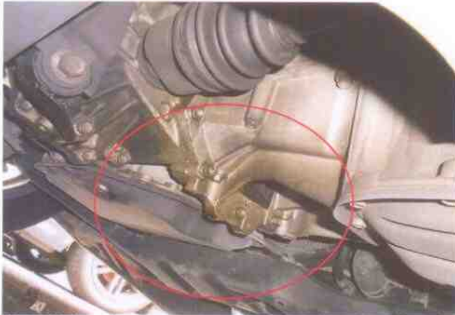
Photo 15 shows the close up view of the undercarriage of the Motor Car. Leakage of fluid was seen. However, we were unable to determine where are the source of the leakage due to the inaccessibility of the engine compartment.
