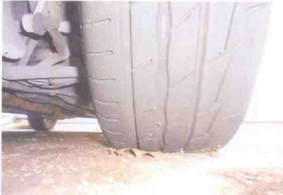
Photo 12 shows the condition of the front left tyre of the Motor Car, which was observed to be in serviceable condition with remaining tread depth of approximately 6mm. There was no tear, cut or burst mark(s) on the outer and the inner sidewalls as well as across the tread of this tyre, which was also sufficiently inflated for vehicular operation.
