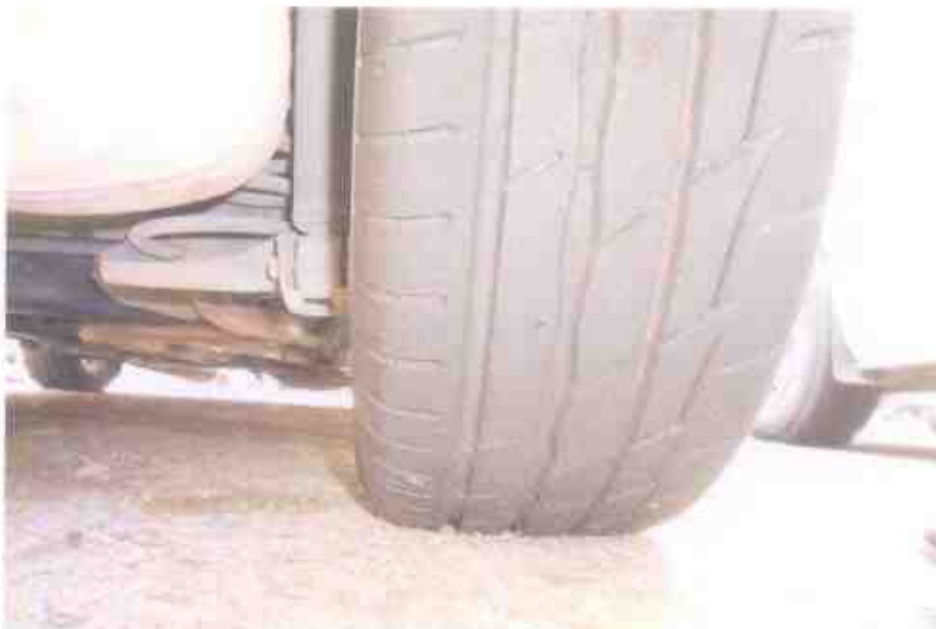
Photo 13 shows the condition of the rear right tyre of the Motor Car, which was observed to be in serviceable condition with remaining tread depth of approximately 5mm. There was also no tear, cut or burst mark(s) on the outer and the inner sidewalls as well as across the tread of this tyre.
