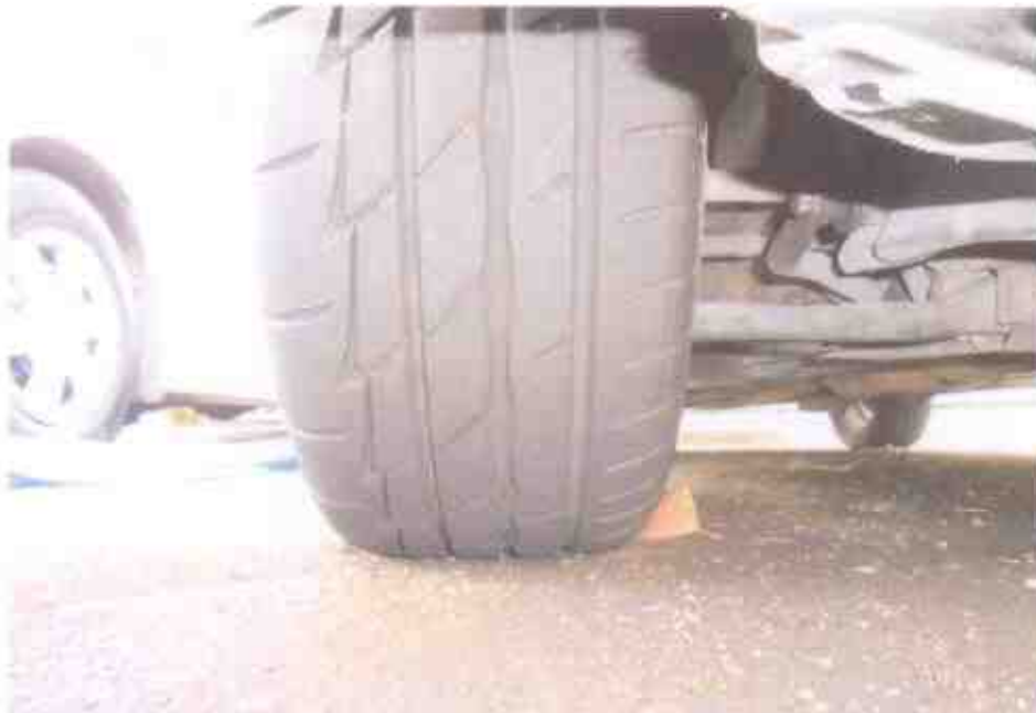
Photo 11 shows the condition of the front right tyre of the Motor Car, which was observed to be in serviceable condition with remaining tread depth of approximately 5mm. There was no tear, cut or burst mark(s) on the outer and the inner sidewalls as well as across the tread of this tyre.
