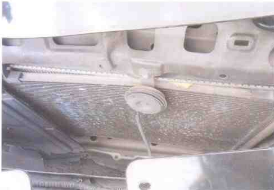
Photo 7 shows a closer view of the damaged radiator of the Motor Car from the front view. The impact force was significant, causing the various parts and components inside the engine compartment to be pushed inwards, towards the rear of the Motor Car.
