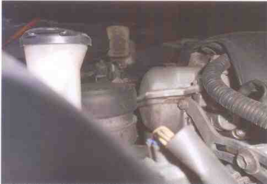
Photo 6 shows a closer view of the engine compartment of the Motor Car from the right hand side of the bonnet opening. The impact force was significant, causing the various parts and components inside the engine compartment to be pushed inwards, towards the rear of the Motor Car.
