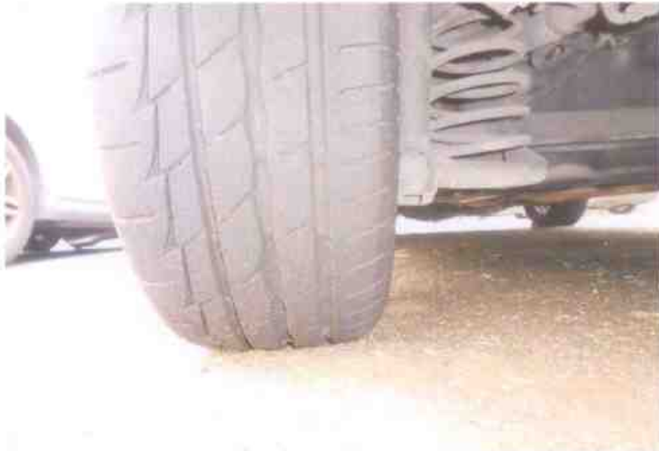
Photo 14 shows the condition of the rear left tyre of the Motor Car, which was observed to be in serviceable condition with remaining tread depth of approximately 5mm. There was also no tear, cut or burst mark(s) on the outer and the inner sidewalls as well as across the tread of this tyre.
