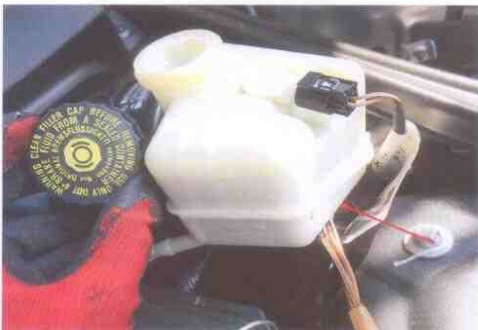
Photo 18 shows the close up view of the brake fluid that was seen with sufficient level not affected by the accident's impact.
