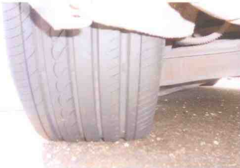
Photo 14 shows the condition of the rear left tyre of the Motor Car, which was observed to be in serviceable condition with remaining tread depth of approximately 6mm. It was also observed to be deflated due to the accident.
