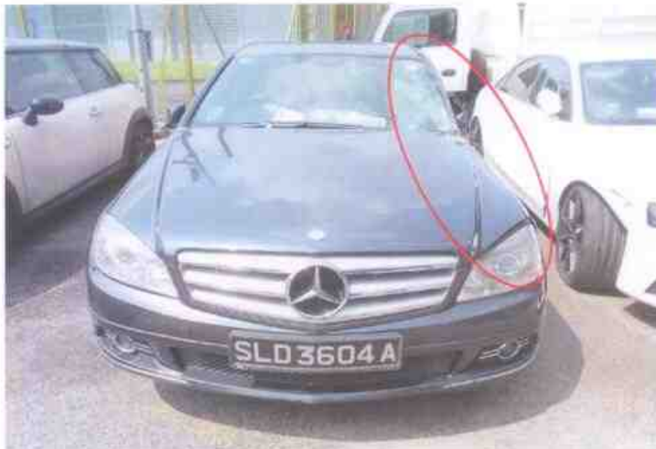
Photo 1 shows a general view of the frontal portion of the Motor Car at the time of our inspection. The Motor Car was observed to have sustained extensive impact damage at its frontal, left & rear portion. The impact force was significant, causing the various parts and components to be damaged as a result of the accident.
