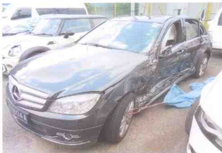
Photo 3 shows a general view of the front left portion of the Motor Car at the time of our inspection. The Motor Car was observed to have sustained extensive impact damage at its left portion.
