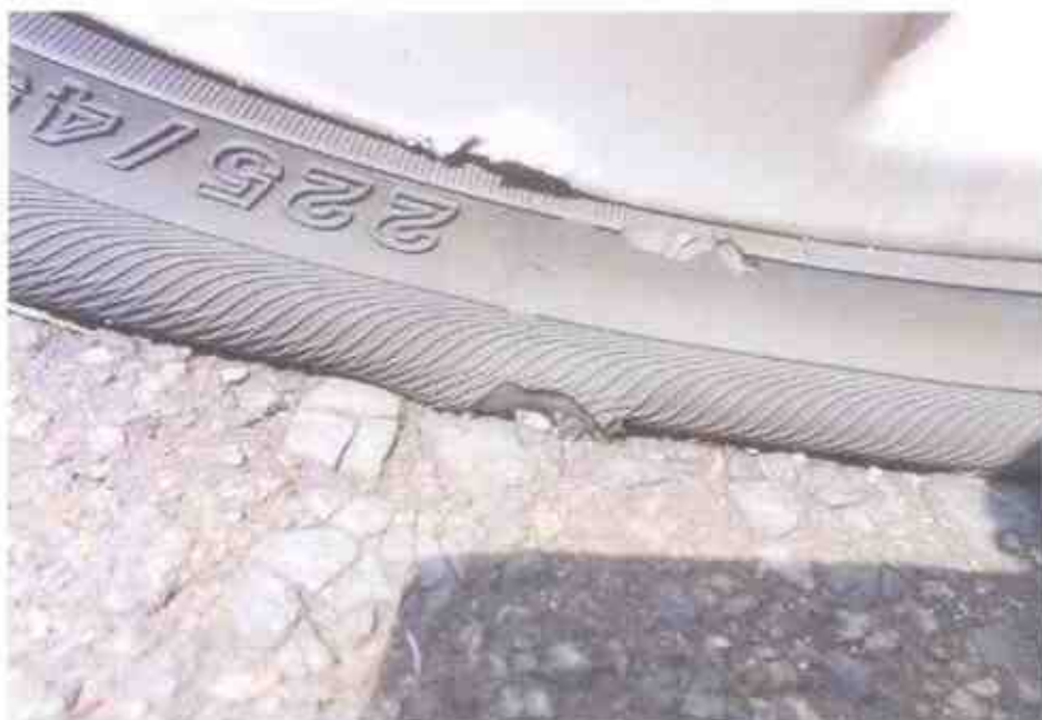
Photo 15 shows the torn mark on the rear left tyre of the Motor Car, which deflates the tyre caused by the accident.
