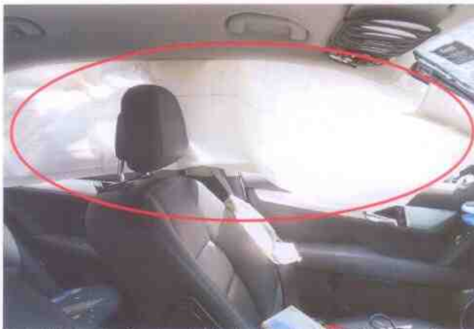
Photo 28 shows the Supplemental Restraint System (SRS) of the Motor Car was however likely to be in normal operating condition at the material time of the accident. The evidence of the deployed window's airbag indicates that the impact sensors and control module of the Motor Car's SRS were all in serviceable condition at the material time of accident.
