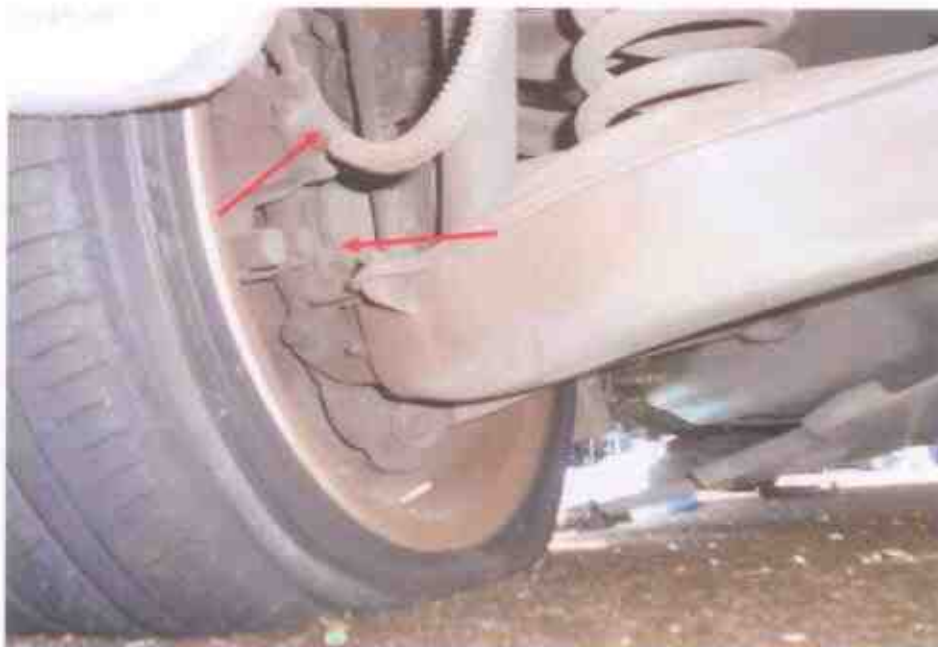
Photo 27 shows the braking components at the rear left wheel of the Motor Car. We did not observe any leakage of brake fluid at the time of our inspection of the Motor Car. Nevertheless, the tyre was found to be deflated likely due to the accident's impact.
