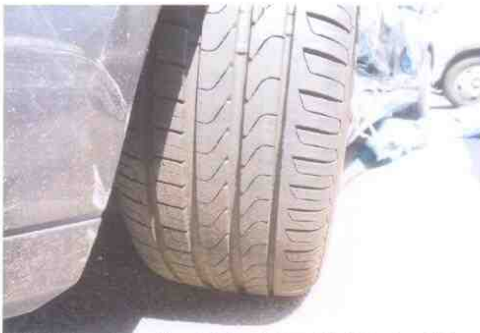
Photo 12 shows the condition of the front left tyre of the Motor Car, which was observed to be in serviceable condition with remaining tread depth of approximately 5mm. There was no tear, cut or burst mark(s) on the outer and the inner sidewalls as well as across the tread of this tyre, which was also sufficiently inflated for vehicular operation.
