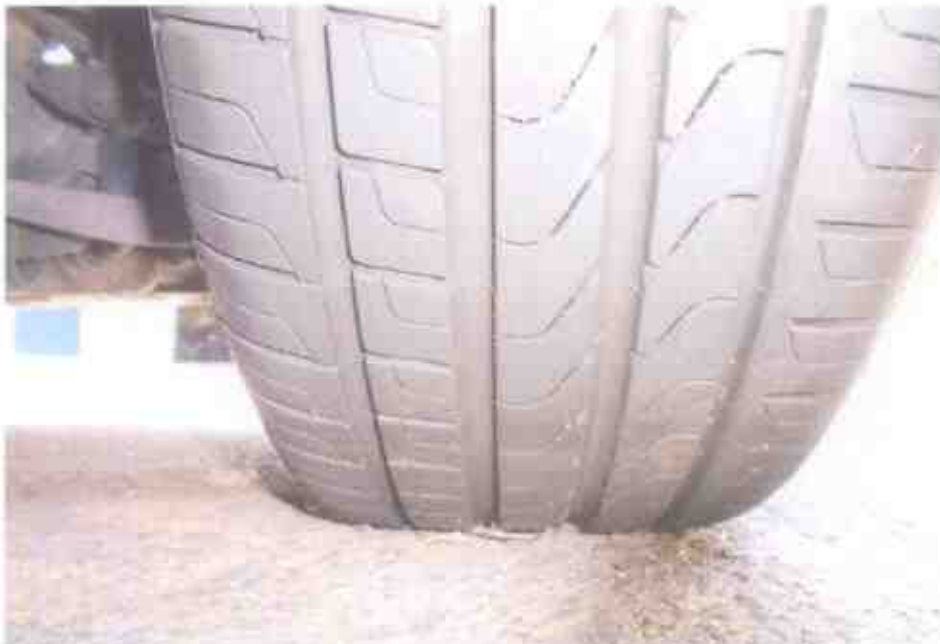
Photo 11 shows the condition of the front right tyre of the Motor Car, which was observed to be in serviceable condition with remaining tread depth of approximately 5mm. There was no tear, cut or burst mark(s) on the outer and the inner sidewalls as well as across the tread of this tyre.
