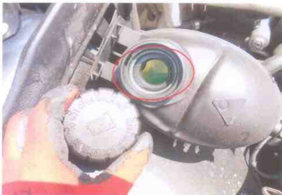
Photo 17 shows the close up view of the engine coolant that was seen with sufficient level not affected by the accident's impact
