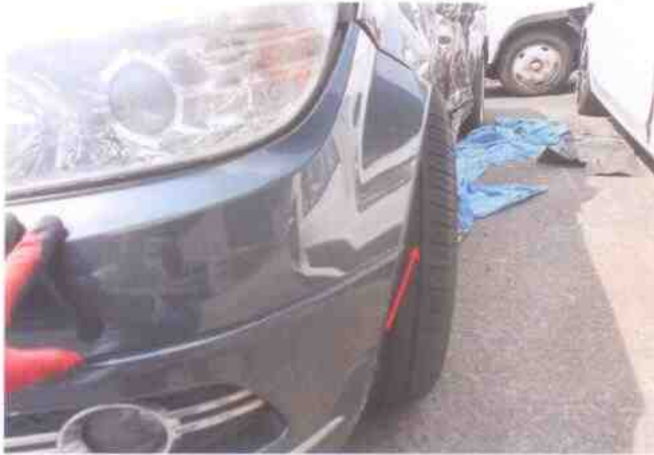
Photo 21 shows the misalignment at the front left wheel of the Motor Car.
