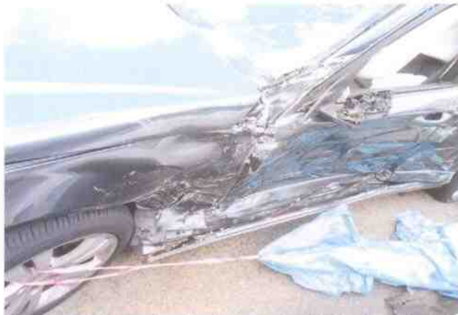
Photo 4 shows a closer view of the damage sustained on the left portion of the Motor Car. The impact force was significant, causing the left portion of the Motor Car to be pushed inwards, towards the right of the Motor Car.
