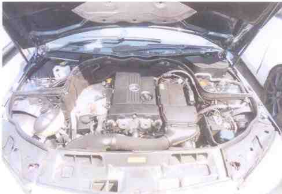
Photo 16 shows a general view of the Motor Car's engine compartment. The various parts and components inside the engine compartment were unaffected by the accident. There was also no sign(s) or indication(s) of fluid leakage and/or fluid stain within the engine compartment.
