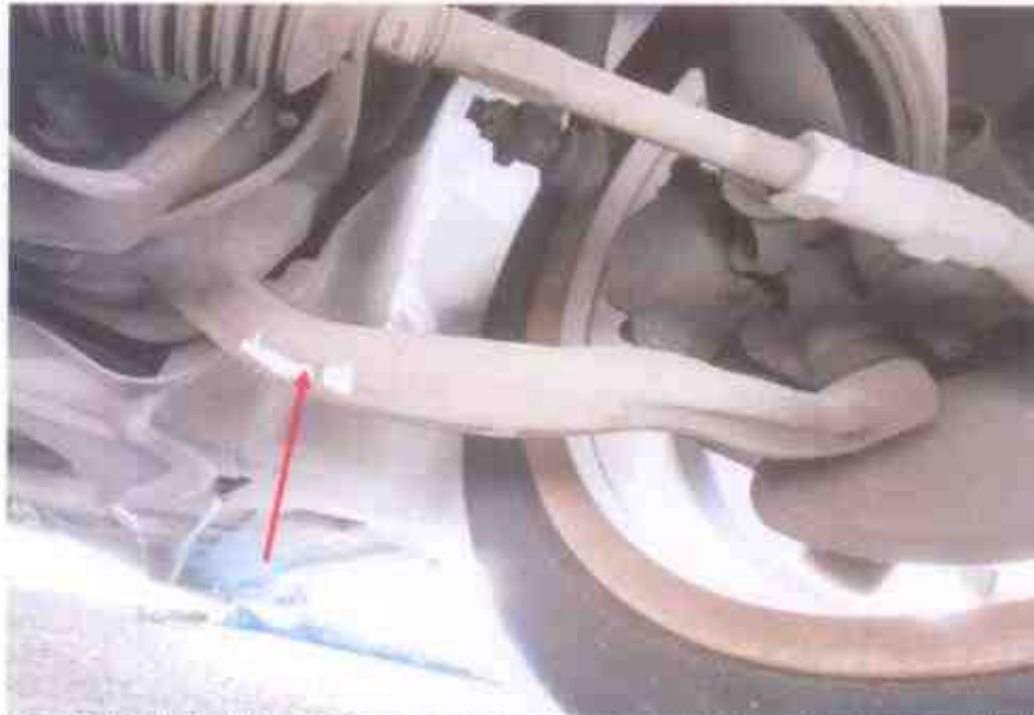
Photo 23 shows the steering rod that was observed to be with damages likely due to the accident's impact.
