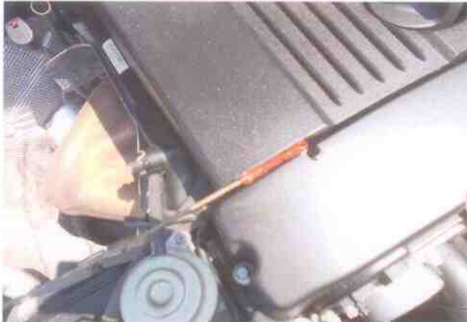
Photo 19 shows the engine oil dip stick of the Motor Taxi at the time of our inspection. The engine oil was observed to be of sufficient level and without any visible contamination.
