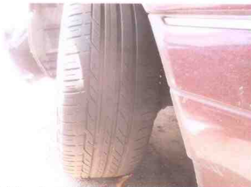
Photo 9 shows the condition of the front left tyre of the Motor Car, which was observed to be in serviceable condition with remaining tread depth of approximately 5mm. The tyre, which was wrapped around alloy wheel rim, was also observed to be sufficiently inflated for vehicular operation.
