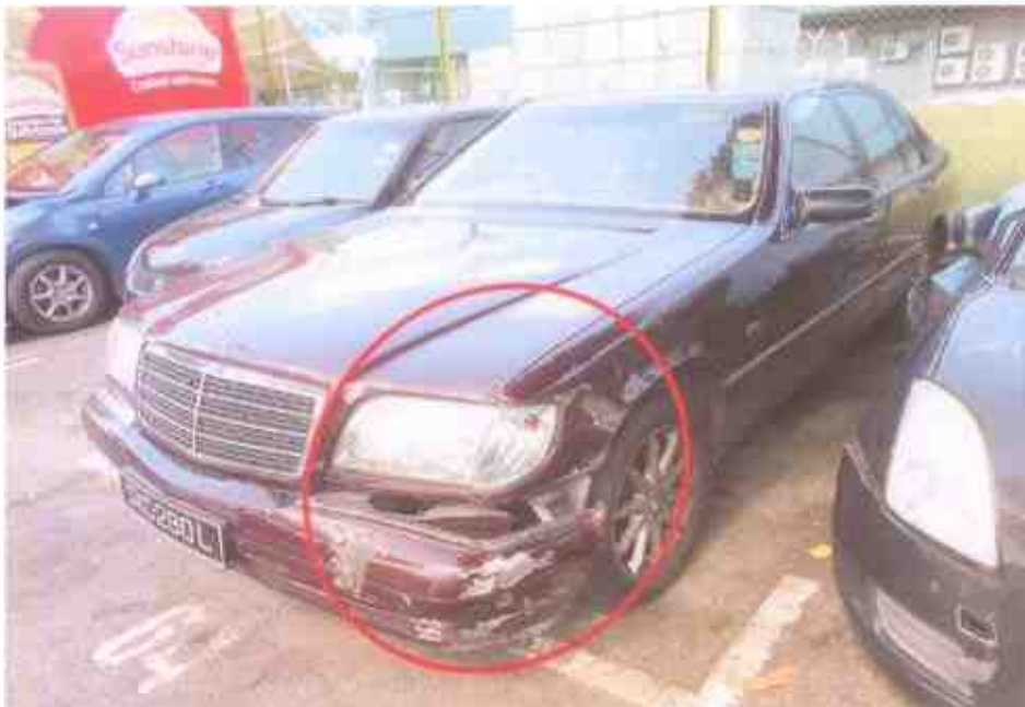
Photo 4 shows a general view of the front left body of the Motor Car at the time of our inspection. The Motor Car was observed to have sustained a relatively minor impact damages that was confined to its front left portion.
