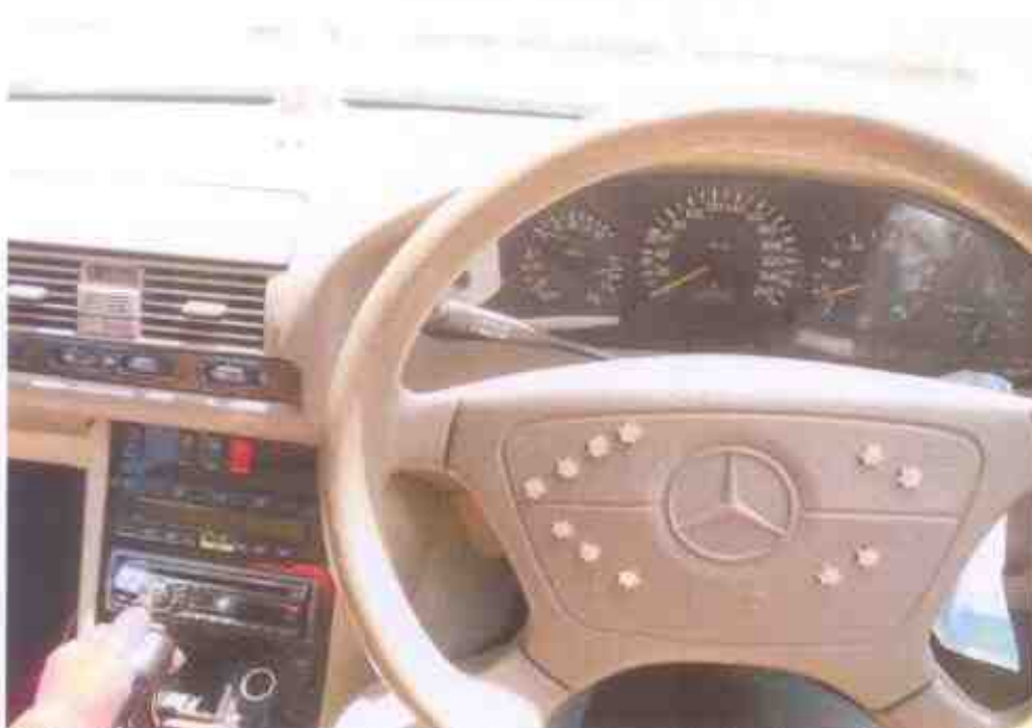
Photo 23 shows no warning lights illuminated on the instrument panel of the Motor Car after the engine was cranked. This would suggest that there was no abnormality to the various electronic operating systems of the Motor Car, like the ABS and SRS.
