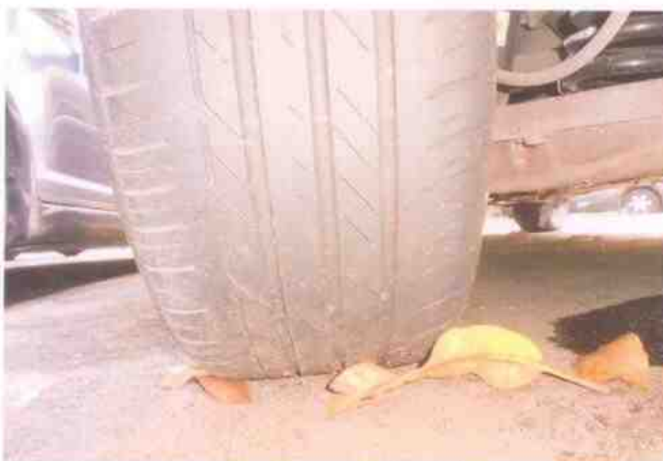
Photo 10 shows the condition of the rear left tyre of the Motor Car, which was observed to be in serviceable condition with remaining tread depth of approximately 4mm.
