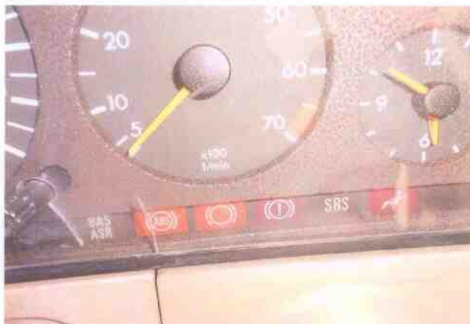
Photo 22 shows the warning lights for the various electronic operating systems of the Motor Car appearing on its instrument panel during the self-test when the engine is cranked, in particular the ABS light and SRS light.
