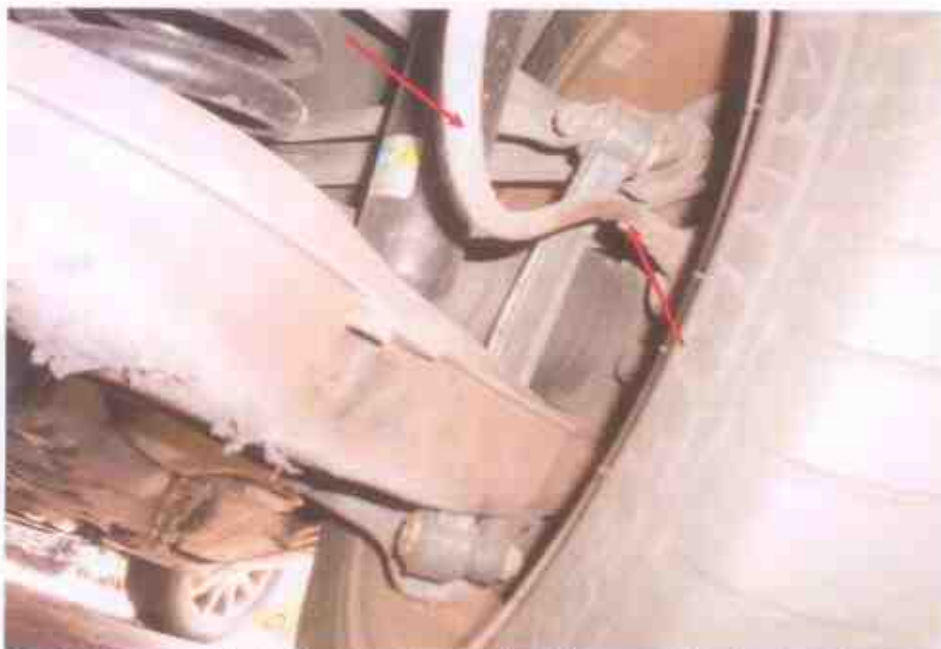
Photo 18 shows the brake hose (arrowed) at the rear right wheel of the Motor Car. We did not observe any leakage of brake fluid at the time of our inspection of the Motor Car. Our visual inspection of the various mechanical components of the Motor Car's braking system revealed all to be intact without visible damage.
