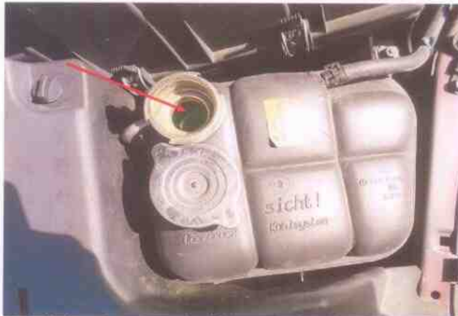
Photo 14 shows the engine coolant fluid reservoir of the Motor Car at the time of our inspection. The engine coolant fluid was observed to be of sufficient level and without any visible contamination.
