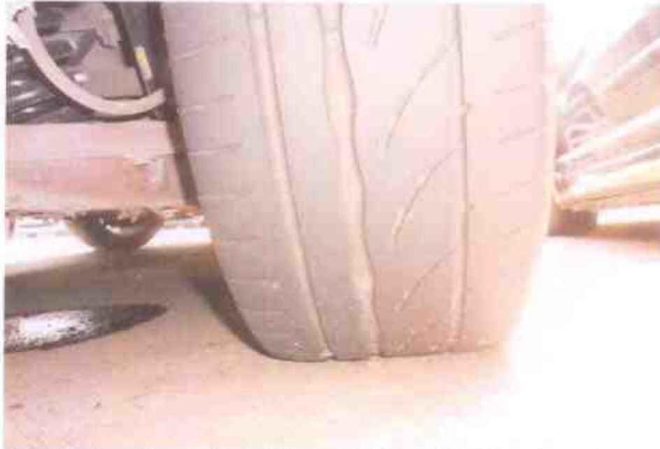
Photo 11 shows the condition of the rear right tyre of the Motor Car, which was observed to be in serviceable condition with remaining tread depth of approximately 4mm.
