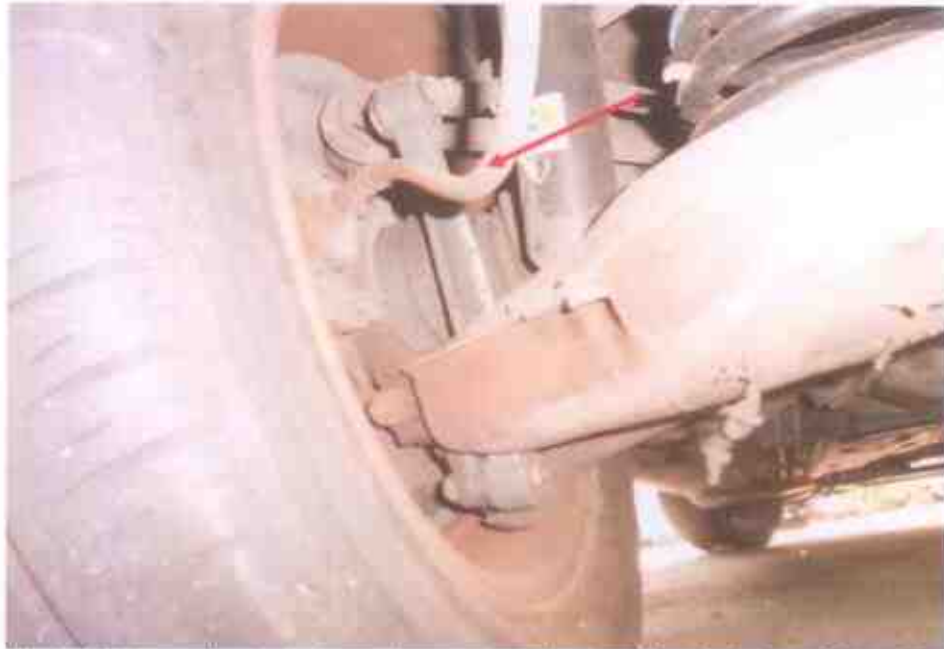
Photo 17 shows the brake hose (arrowed) at the rear left wheel of the Motor Car. We did not observe any leakage of brake fluid at the time of our inspection of the Motor Car. Our visual inspection of the various mechanical components of the Motor Car's braking system revealed all to be intact without visible damage.
