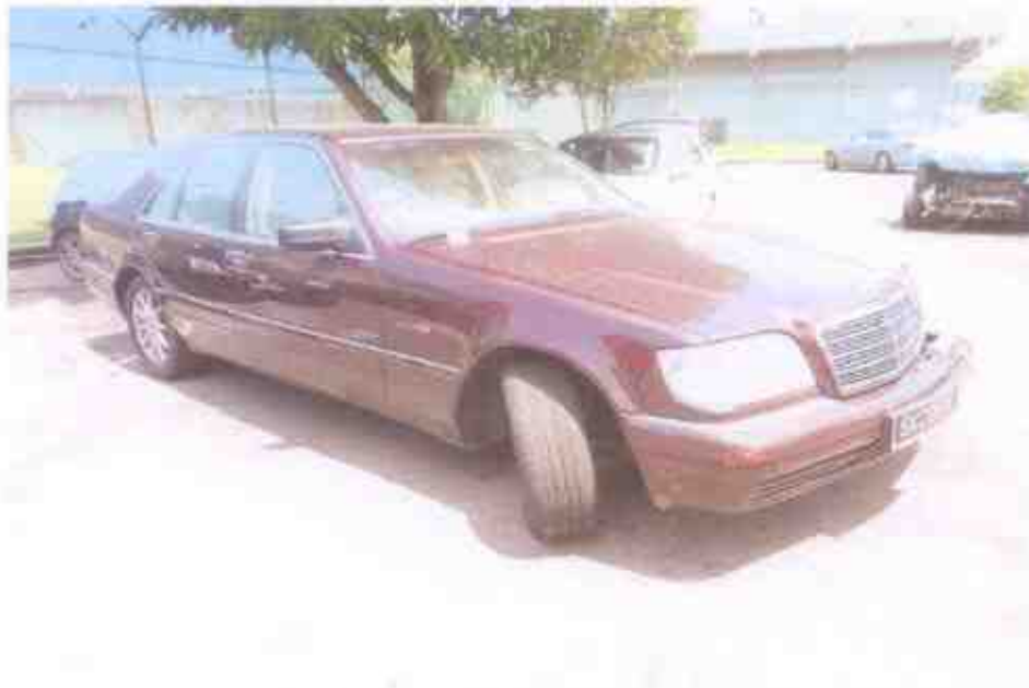
Photo 24 shows we conducted an operational test on the Motor Car. Drive mode, Reverse mode & Neutral mode were engaged at time of our test. Brake pedal was also engaged to a complete stop. There was no abnormality observed at time of testing.
