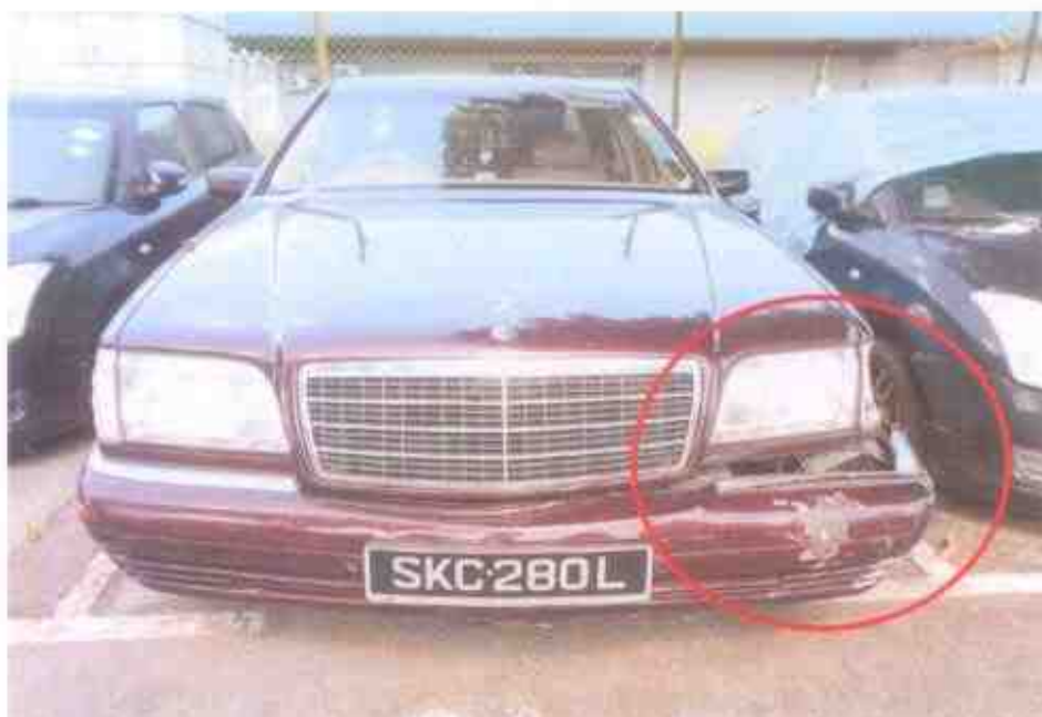
Photo 2 shows a general view of the front body of the Motor Car at the time of our inspection. The Motor Car was observed to have sustained a relatively minor impact damages that was confined to its front left portion. Its front left bumper was observed to be damaged; its left hand signal light cover was broken; its front left bonnet & left fender was dented & its windshield was cracked likely due to the accident's collision impact.
