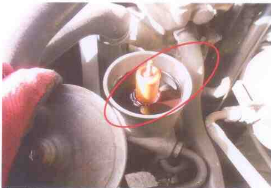
Photo 16 shows the power steering fluid of the Motor Car at the time of our inspection. It was observed to be of sufficient level and without any visible contamination.
