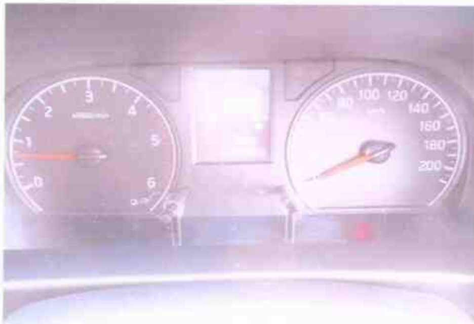
Photo 20 shows the warning lights disappearing after cranking of the engine.
