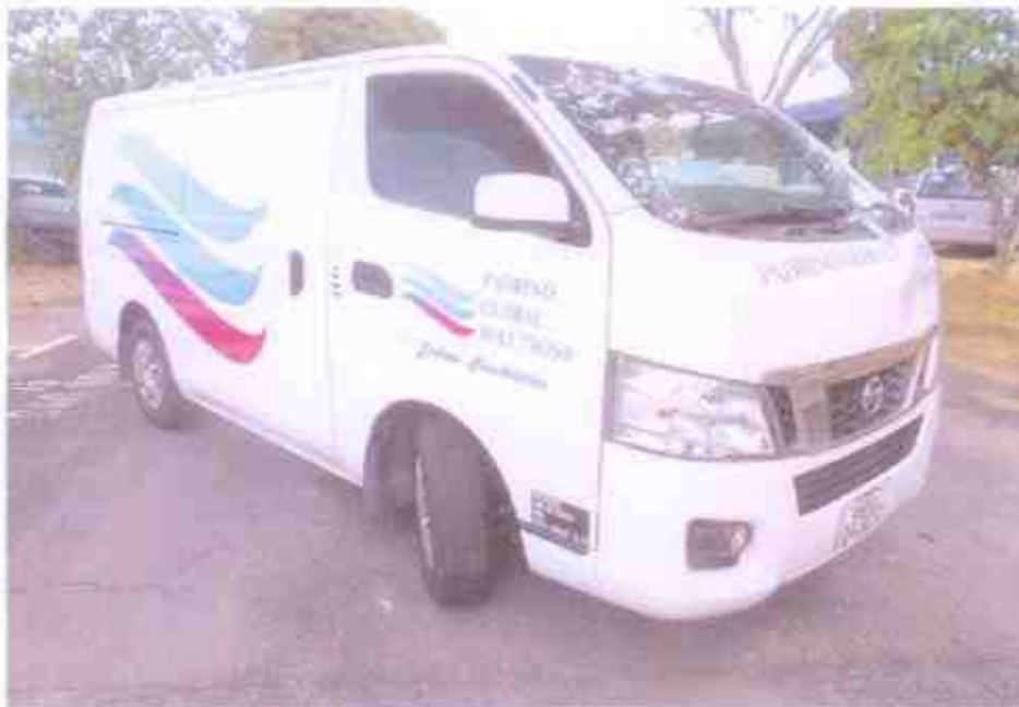
Photo 21 shows a short operational test of the Motor Van, to primarily determine whether there was any abnormality to its various operating systems like its engine system, its transmission system, steering system and braking system was subsequently carried out. The test was conducted by driving the Motor Van forward, stopping, before reversing and coming to a stop again.
