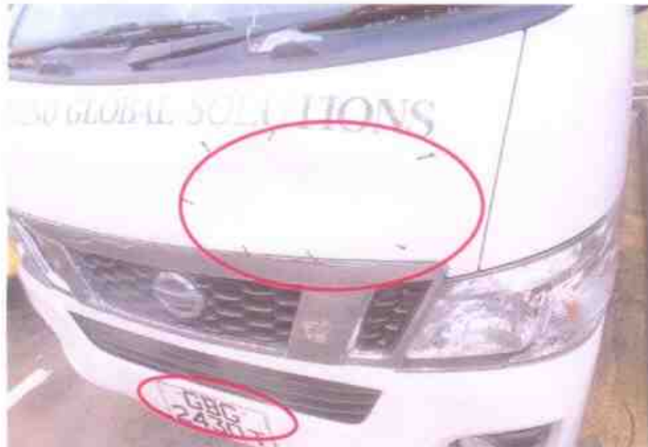
Photo 3 shows a general view of the front body of the Motor Van at the time of our inspection. The Motor Van was observed to sustained minor damage at the front left panel & lower bumper.
