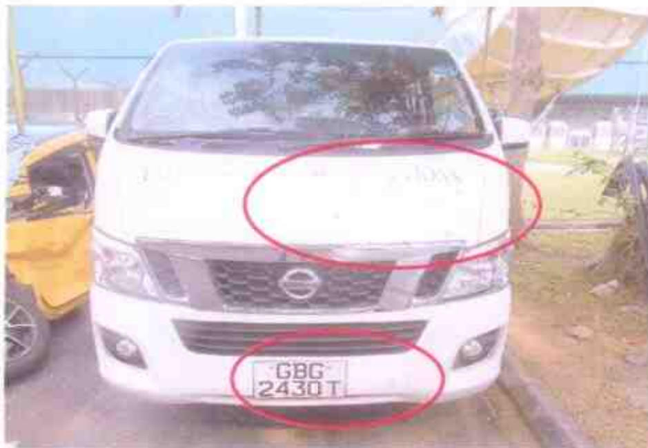
Photo 2 shows a general view of the front body of the Motor Van at the time of our inspection. The Motor Van was observed to sustained minor damage at the front left panel & lower bumper.
