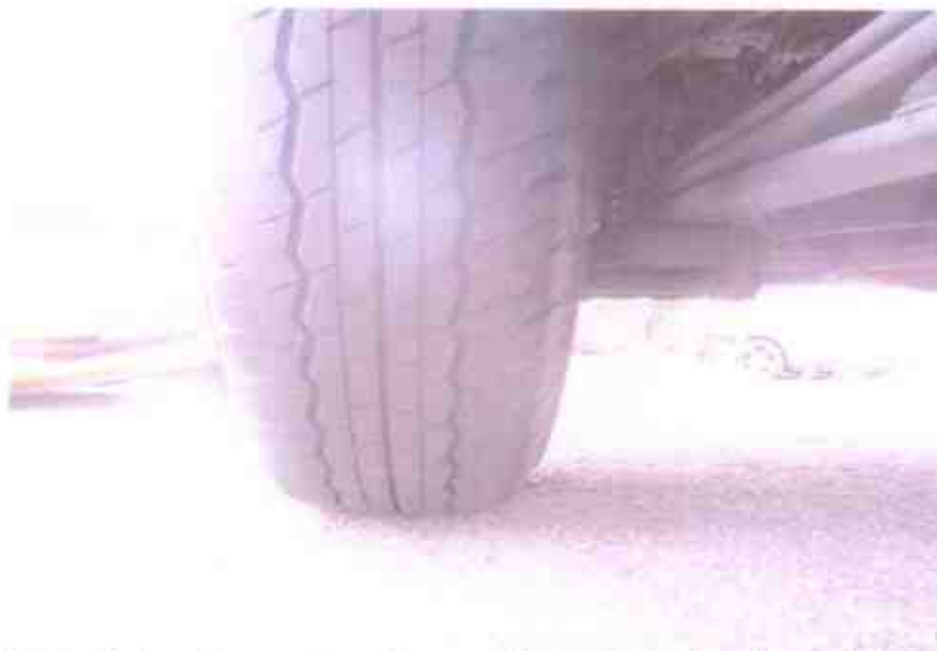
Photo 11 shows the condition of the rear right tyre of the Motor Van, which was observed to be in serviceable condition with remaining tread depth of approximately 5mm. There was also no tear, cut or burst mark(s) on the outer and the inner sidewalls as well as across the tread of the tyre, which was also sufficiently inflated for vehicular operation.
