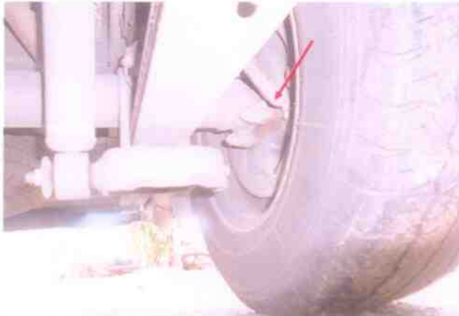
Photo 15 shows the various undercarriage components at the rear left wheel of the Motor Van, in particular the brake hose (arrowed). We did not observe any leakage of brake fluid at the time of our inspection of the Motor Van.
