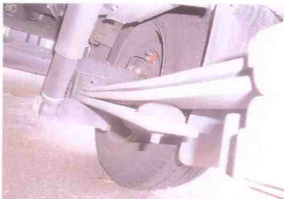
Photo 18 shows the various undercarriage components at the rear right wheel of the Motor Van. The various steering components were all found to be intact, suggesting that the steering system of the Motor Van was likely to be in serviceable condition at the material time of accident. There was also no sign of fluid stain(s) observed on the various undercarriage components at the 4 wheels of the Motor Van.
