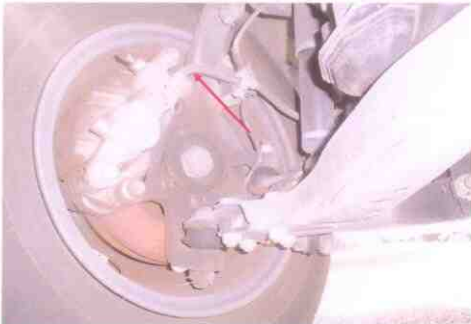
Photo 16 shows the brake hose (arrowed) at the front left wheel of the Motor Van. We did not observe any leakage of brake fluid. Our visual inspection of the various mechanical components of the Motor Van's braking system revealed all to be intact and without visible damage, indicating that the braking system was likely to be in serviceable condition at the material time of accident.
