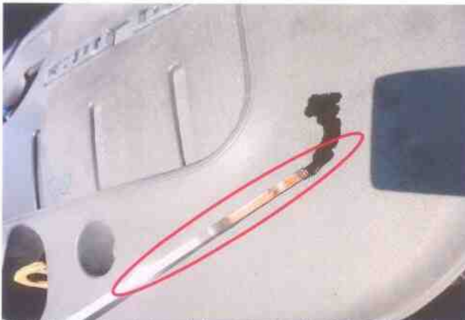
Photo 17 shows the auto transmission oil dip stick of the Motor Taxi at the time of our inspection. The ATF oil was observed to be of sufficient level and without any visible contamination.
