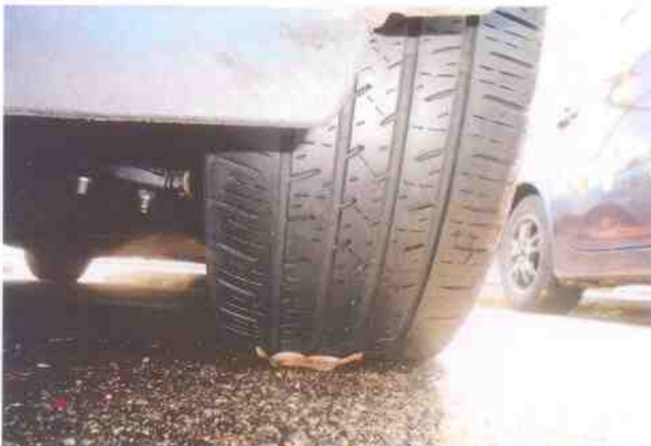
Photo 10 shows the condition of the front left tyre of the Motor Taxi, which was observed to be in serviceable condition with remaining tread depth of approximately 5mm. The tyre, which was wrapped around alloy wheel rim, was also observed to be sufficiently inflated for vehicular operation.
