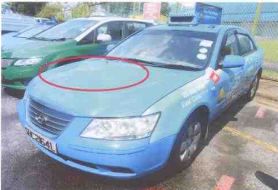
Photo 4 shows a general view of the front right body of the Motor Taxi at the time of our inspection. The Motor Taxi was observed to have sustained a relatively minor impact damages that was confined to its frontal portion.
