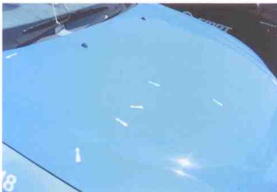
Photo 7 shows a semi close up view of the front portion of the Motor Taxi at the time of our inspection. The Motor Taxi had sustained relatively minor dent at the front bonnet portion likely due to the accident.
