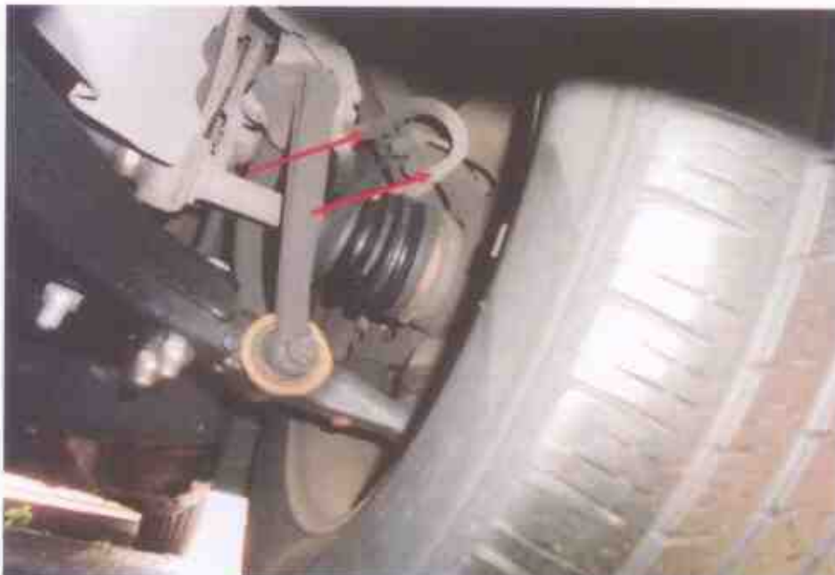
Photo 22 shows the various undercarriage components at the front left wheel of the Motor Taxi. We did not observe any leakage of brake fluid (arrowed) at the time of our inspection of the Motor Taxi. Our visual inspection of the various mechanical components of the Motor Taxi's braking system revealed all to be intact and without visible damage, indicating that the braking system was likely to be in serviceable condition at the material time of accident.
