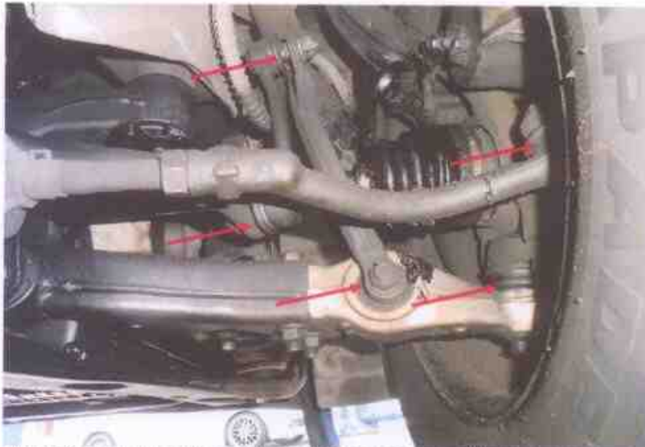
Photo 21 shows the various undercarriage components at the front right wheel of the Motor Taxi, in particular the steering tie rod (arrowed). The various steering components were all found to be intact, suggesting that the steering system of the Motor Taxi was likely to be in serviceable condition.
