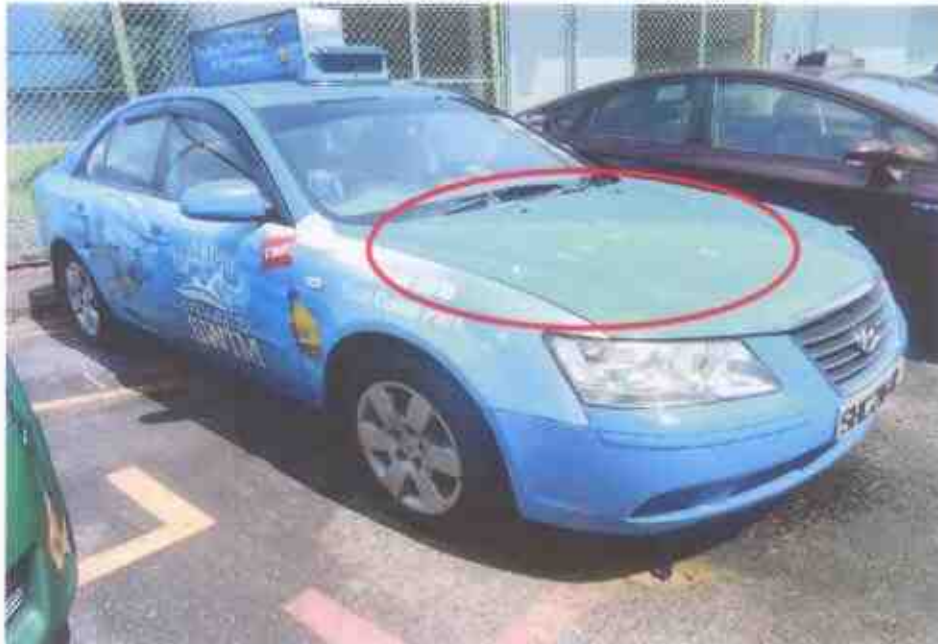
Photo 3 shows a general view of the front left body of the Motor Taxi at the time of our inspection. The Motor Taxi was observed to have sustained a relatively minor impact damages that was confined to its frontal portion.
