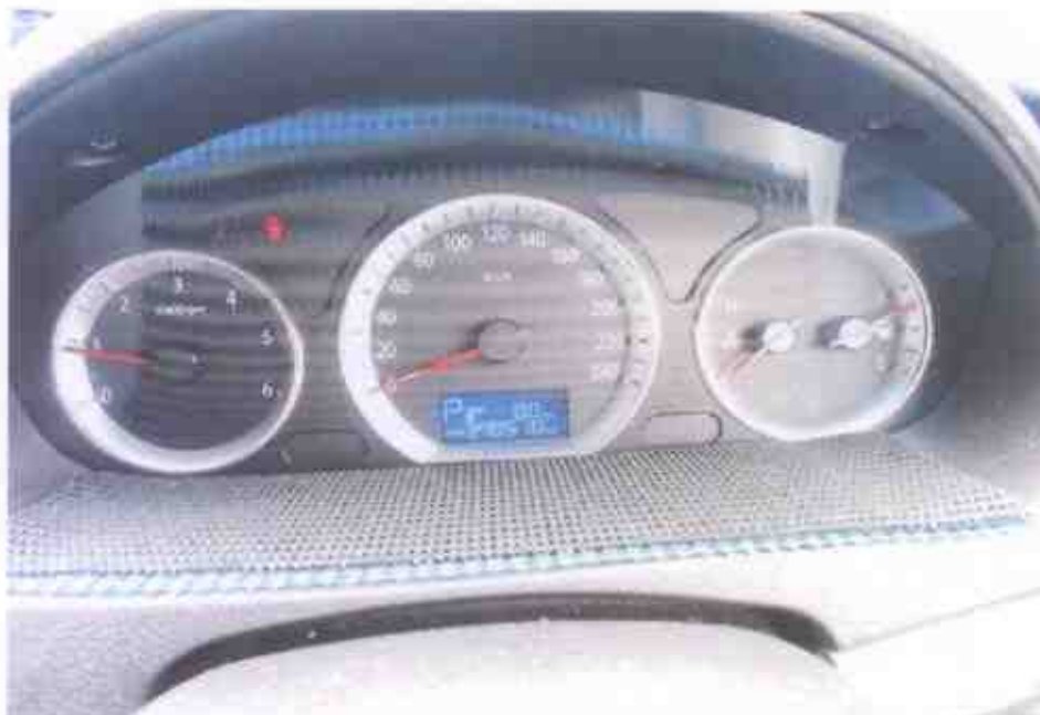
Photo 24 shows no warning lights illuminated on the instrument panel of the Motor Taxi after the engine was cranked. This would suggest that there was no abnormality to the various electronic operating systems of the Motor Taxi, like the ABS light engine check light, battery light and diesel glow plug.
