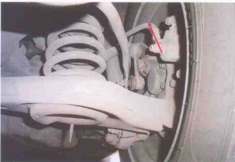
Photo 20 shows the brake hose (arrowed) at the rear right wheel of the Motor Taxi. We did not observe any leakage of brake fluid at the time of our inspection of the Motor Taxi. Our visual inspection of the various mechanical components of the Motor Taxi's braking system revealed all to be intact without visible damage.
