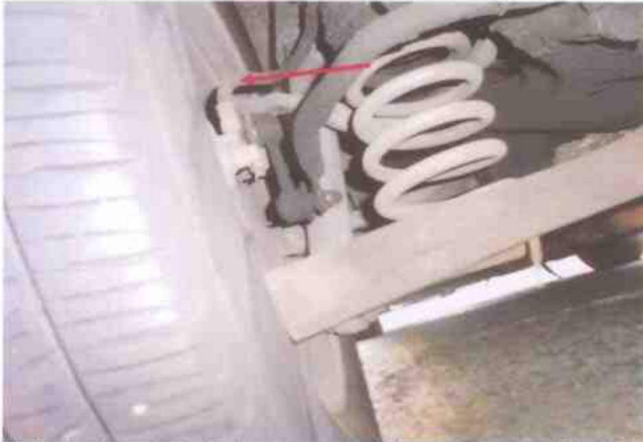
Photo 19 shows the brake hose (arrowed) at the rear left wheel of the Motor Taxi. We did not observe any leakage of brake fluid at the time of our inspection of the Motor Taxi. Our visual inspection of the various mechanical components of the Motor Taxi's braking system revealed all to be intact without visible damage.
