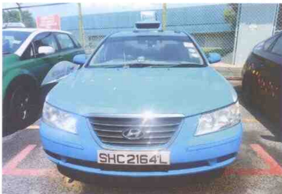
Photo 2 shows a general view of the front body of the Motor Taxi at the time of our inspection. The Motor Taxi was observed to have sustained a relatively minor impact damages that was confined to its frontal portion. its front bonnet was observed to be slightly dented likely due to the accident's collision impact.
