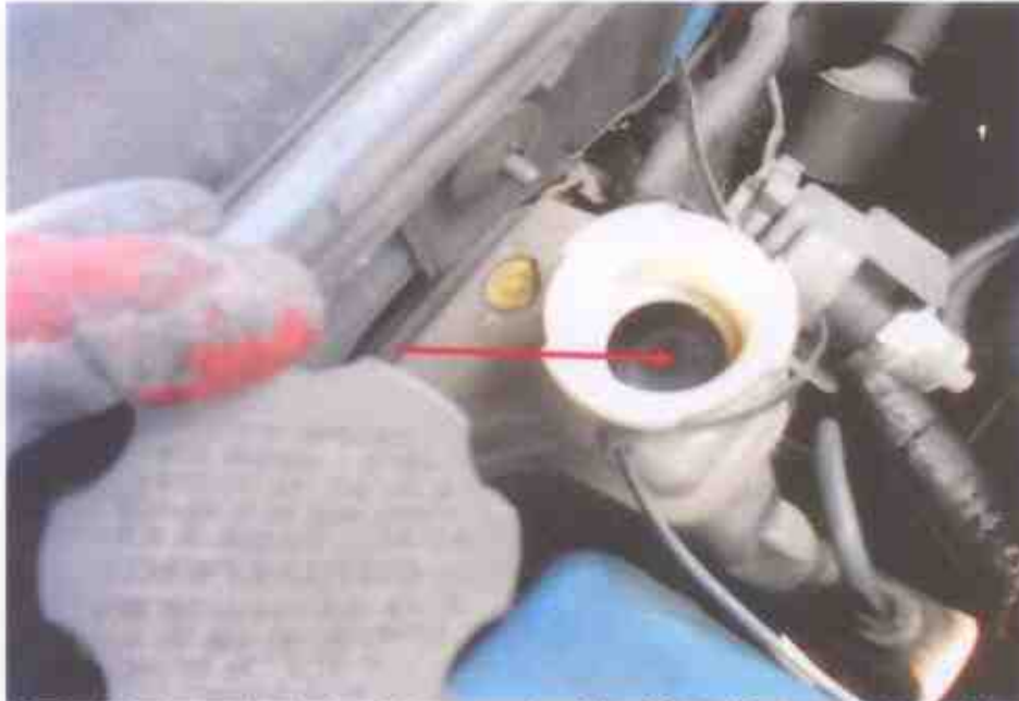
Photo 14 shows the brake fluid reservoir of the Motor Taxi at the time of our inspection. The brake fluid was observed to be of sufficient level (arrowed) and without any visible contamination.
