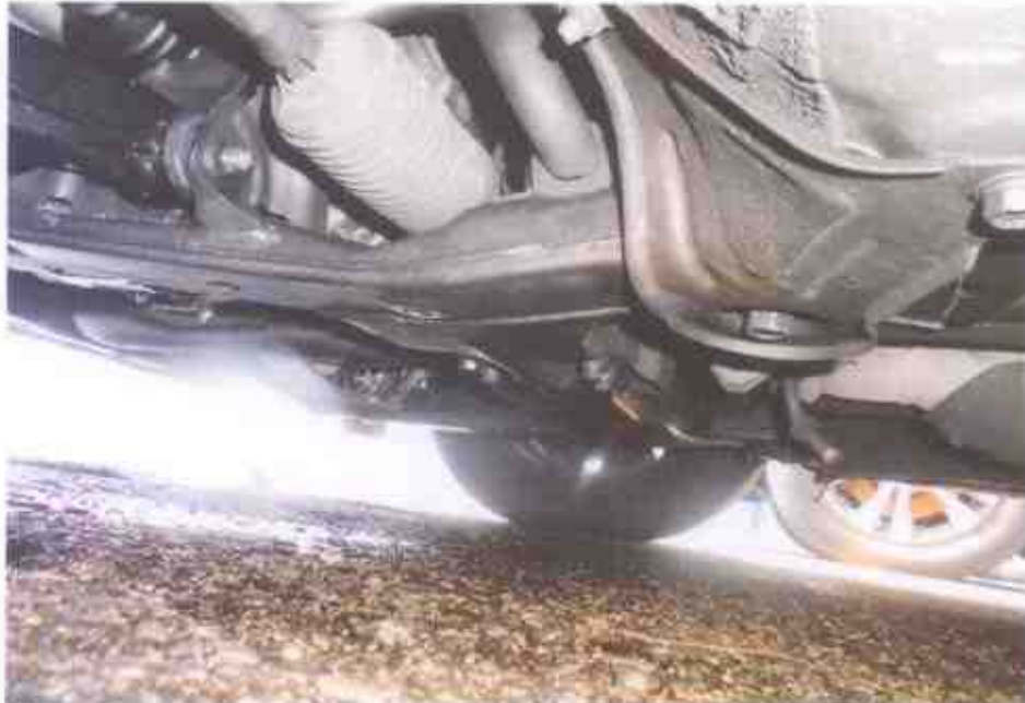
Photo 18 shows the engine underside of the Motor Taxi engine at the time of our inspection. The engine was observed to be with a pre-existed oil stain prior the accident. This was based on the dust that associated with the fluid stain.
