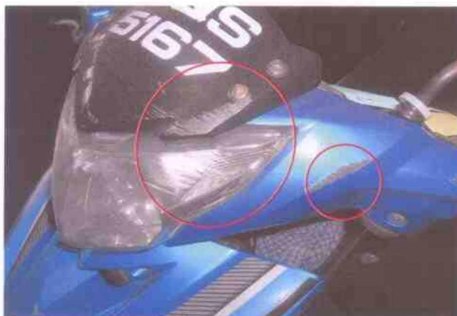
Photo 8 shows a closer view of the left side of the Motorcycle at the time of our inspection. The Motorcycle was observed to have sustained with relatively minor damages due to the accident collision. (Circled)
