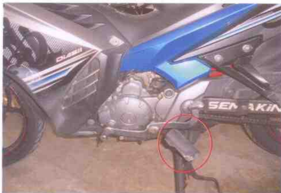
Photo 6 shows a closer view of the left foot rest of the Motorcycle at the time of our inspection. The Motorcycle was observed to have sustained with relatively minor damages due to the accident collision. (Circled)
