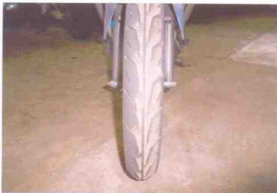
Photo 10 shows the front tyre of the Motorcycle. The front tyre was observed to be in serviceable condition with remaining tread depth of approximately 2mm. The tyre was also observed to be sufficiently inflated for vehicular operation.
