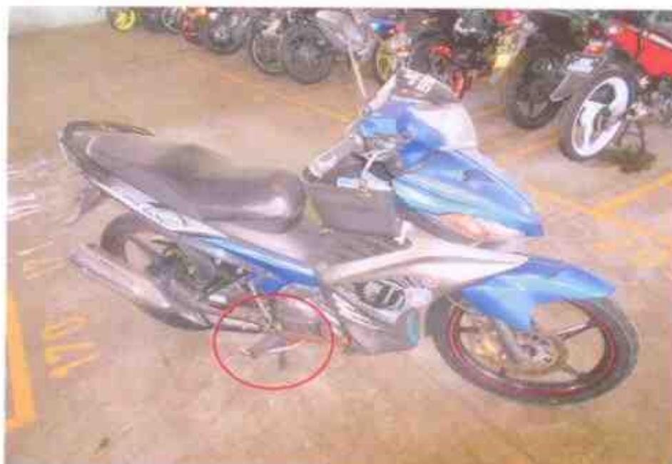
Photo 3 shows a general view of the right body of the Motorcycle at the time of our inspection. The Motorcycle was observed to sustained with damaged rear brake pedal.
