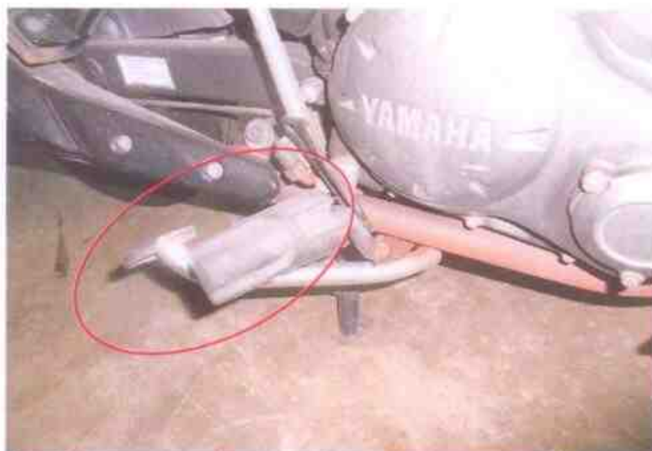
Photo 7 shows a closer view of the right rear brake pedal of the Motorcycle at the time of our inspection. The Motorcycle was observed to have sustained with relatively minor damages due to the accident collision. (Circled)
