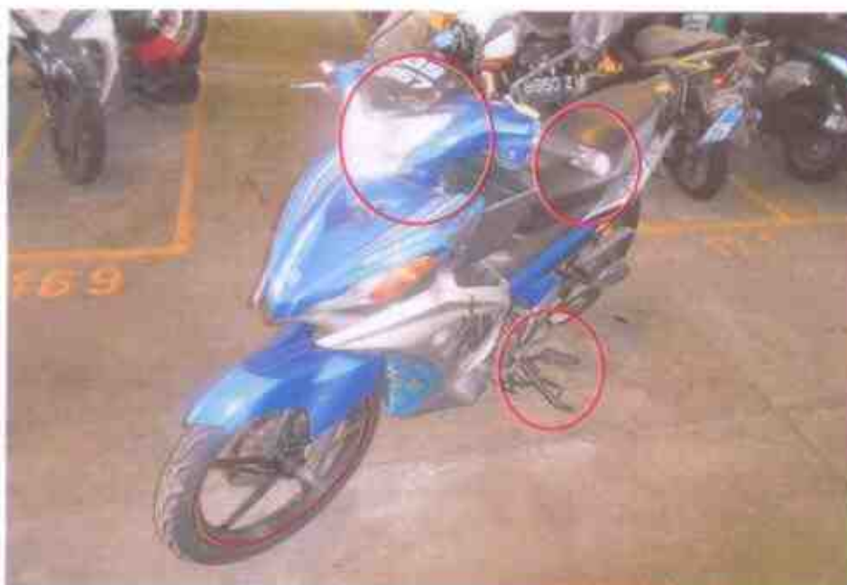
Photo 2 shows a general view of the front body of the Motorcycle at the time of our inspection. The Motorcycle was observed to have sustained relatively minor damages at time of inspection. The damages were observed to be confined to its left side of the Motorcycle.
