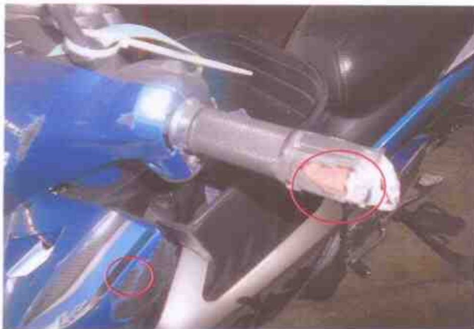
Photo 5 shows a semi close-up view of the left body of the Motorcycle at the time of our inspection. The Motorcycle was observed to have sustained relatively minor damages on the left side handle at time of our inspection.
