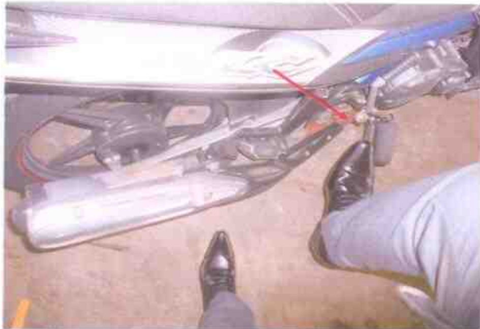
Photo 19 shows testing of the braking of the rear brake in progress. The rear brake was observed to be jammed due to the accident's impact collision.
