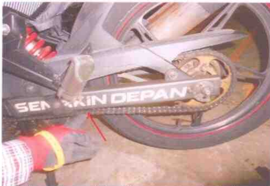
Photo 14 shows the general view of the gear train (arrowed) of the Motorcycle, which was observed to be intact with no misalignment. It was also adequately lubricated for operating purposes. Free play tension was also observed & found adequately acceptable.
