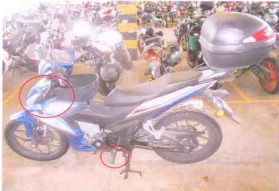
Photo 5 shows a general view of the left body of the Motorcycle at the time of our inspection. The Motorcycle was observed to have sustained relatively minor damages on the left side fairing at time of our inspection.
