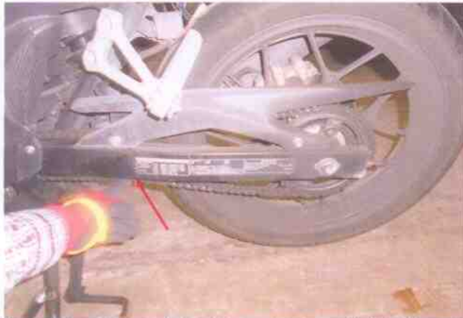
Photo 15 shows the general view of the gear train (arrowed) of the Motorcycle, which was observed to be intact with no misalignment. It was also adequately lubricated for operating purposes. Free play tension was also observed & found adequately acceptable.
