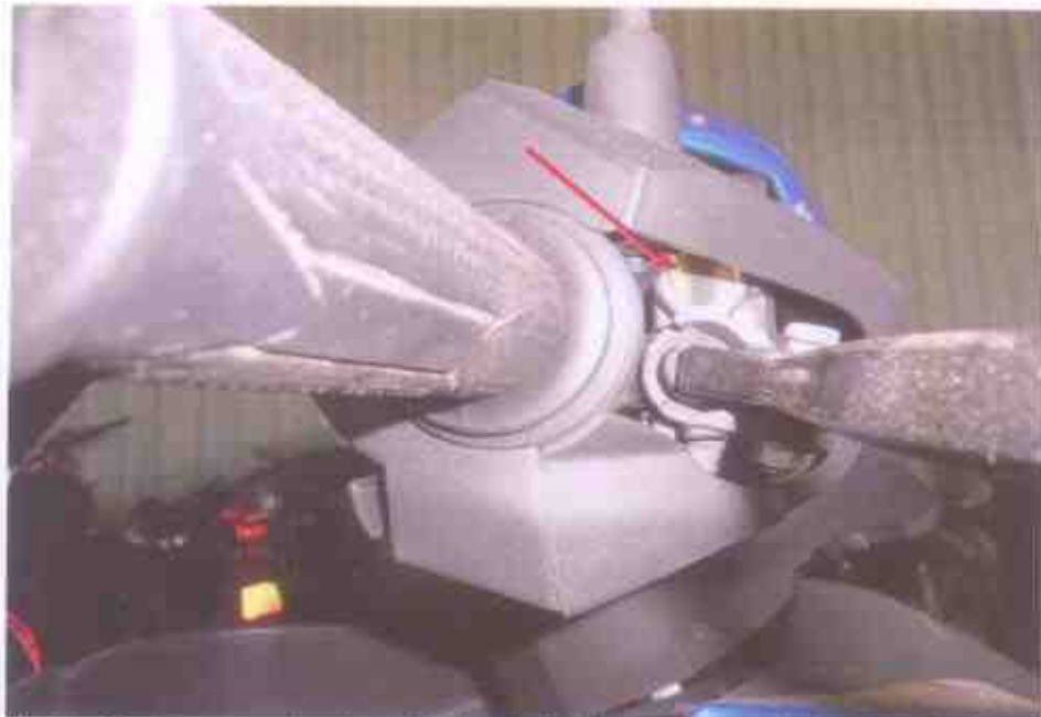
Photo 16 shows our checks on the brake fluid (front) reservoir had also indicated that the brake fluid was of sufficient level for operational purposes, and without contamination.
