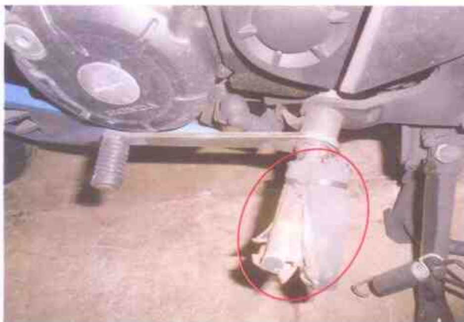
Photo 9 shows a closer view of the left foot rest of the Motorcycle at the time of our inspection. The Motorcycle was observed to have sustained with relatively minor damages due to the accident collision. (Circled)
