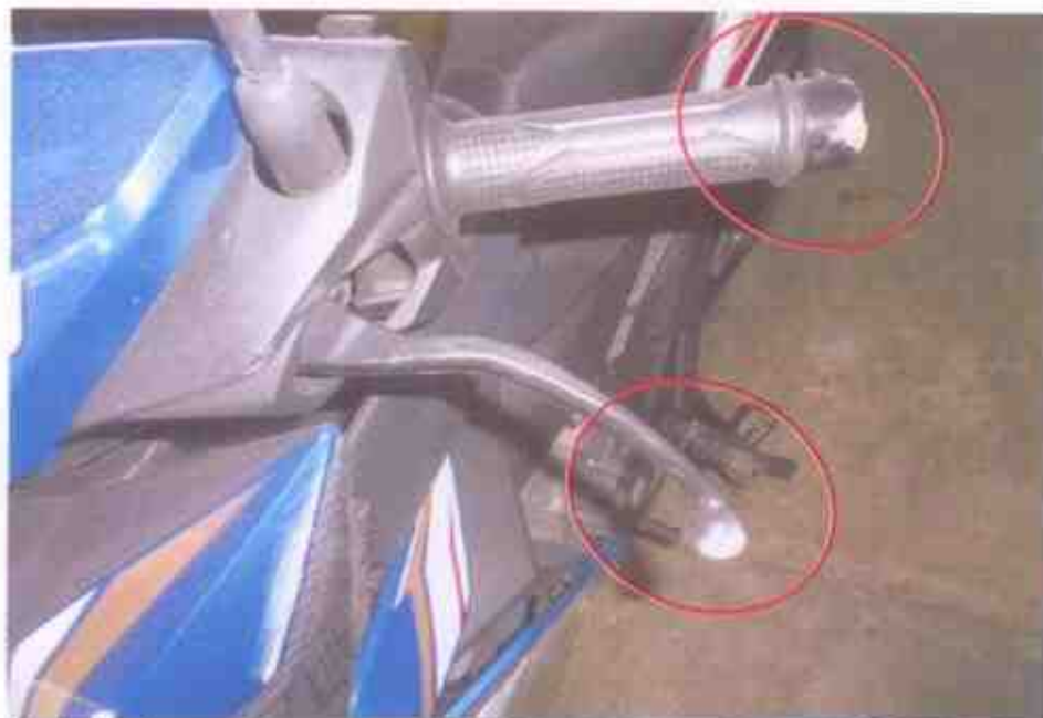
Photo 8 shows a closer view of the left handle of the Motorcycle at the time of our inspection. The Motorcycle was observed to have sustained with relatively minor damages due to the accident collision. (Circled)
