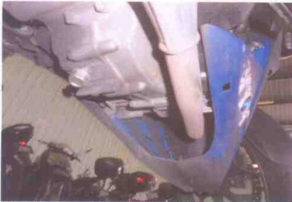
Photo 12 shows no sign(s) or indication(s) of fluid leak observed around the underside of the engine area of the Motorcycle.
