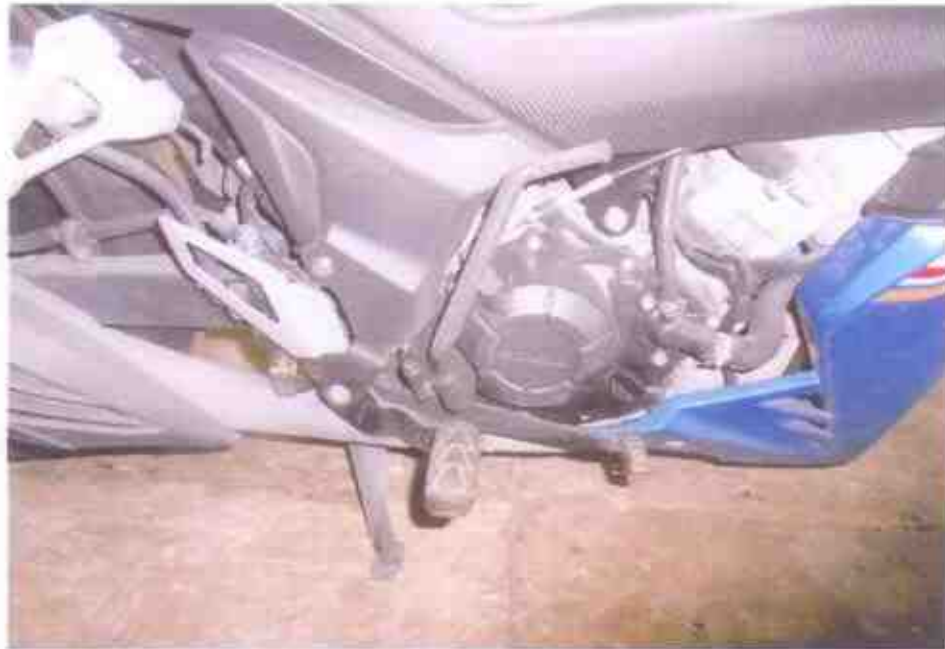
Photo 13 shows no sign(s) or indication(s) of fluid leakage stain observed around the engine area of the Motorcycle.
