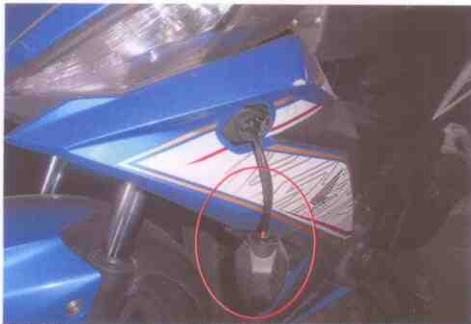
Photo 6 shows a closer view of the front left signal lamp of the Motorcycle at the time of our inspection. The Motorcycle was observed to have sustained with relatively minor damages due to the accident collision. (Circled)
