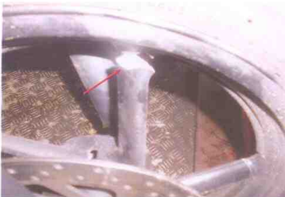
Photo 15 shows the front wheel rim that was observed to be damaged by the accident.
