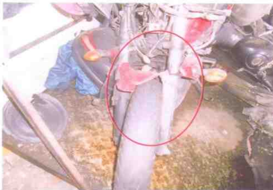
Photo 18 shows the front fork (circled) was observed to be damaged as a result of the accident. Hence, we are unable to conduct any tests on the steering system of the Motorcycle.
