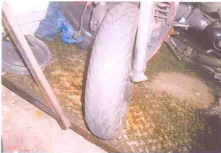
Photo 8 shows the front tyre of the Motorcycle at the time of our inspection. The pattern of the tread was clearly visible with remaining tread depth of approximately 5mm. There was no tear, burst mark(s) and/or punctured hole(s) on the sidewalls as well as across the tread of the front tyre. However, the wheel rim was observed to be broken as a result of the accident.
