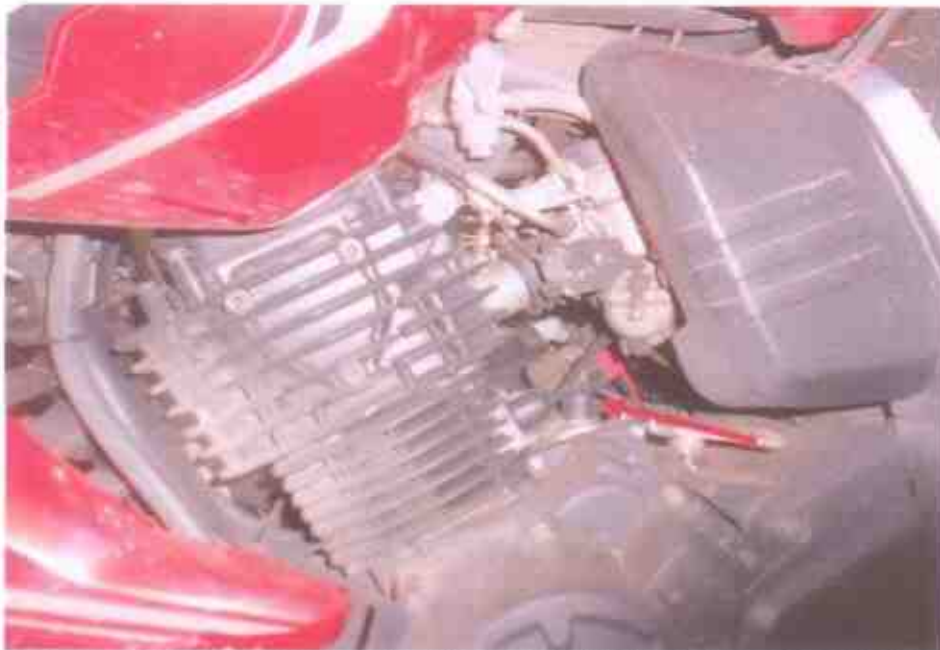
Photo 9 shows no sign(s) or indication(s) of fluid leakage observed around the engine's underside area of the Motorcycle.
