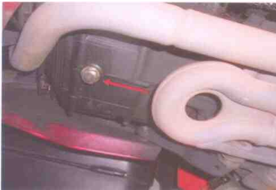
Photo 10 shows no sign(s) or indication(s) of fluid leakage observed around the engine's undercarriage area of the Motorcycle.
