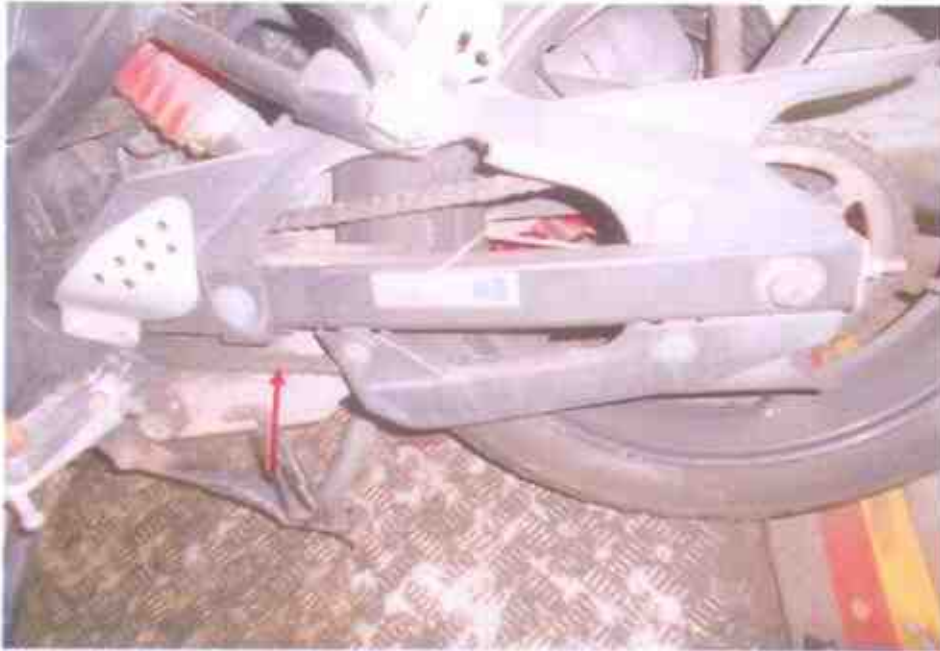
Photo 11 shows the general view of the gear train (arrowed) of the Motorcycle, which was observed to be intact with no misalignment. It was also adequately lubricated for operating purposes.
