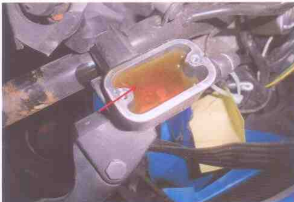
Photo 14 shows the front brake fluid reservoir (arrowed) was observed to be unaffected by the accident. It was observed to be of sufficient level & not contaminated at the time of our inspection.
