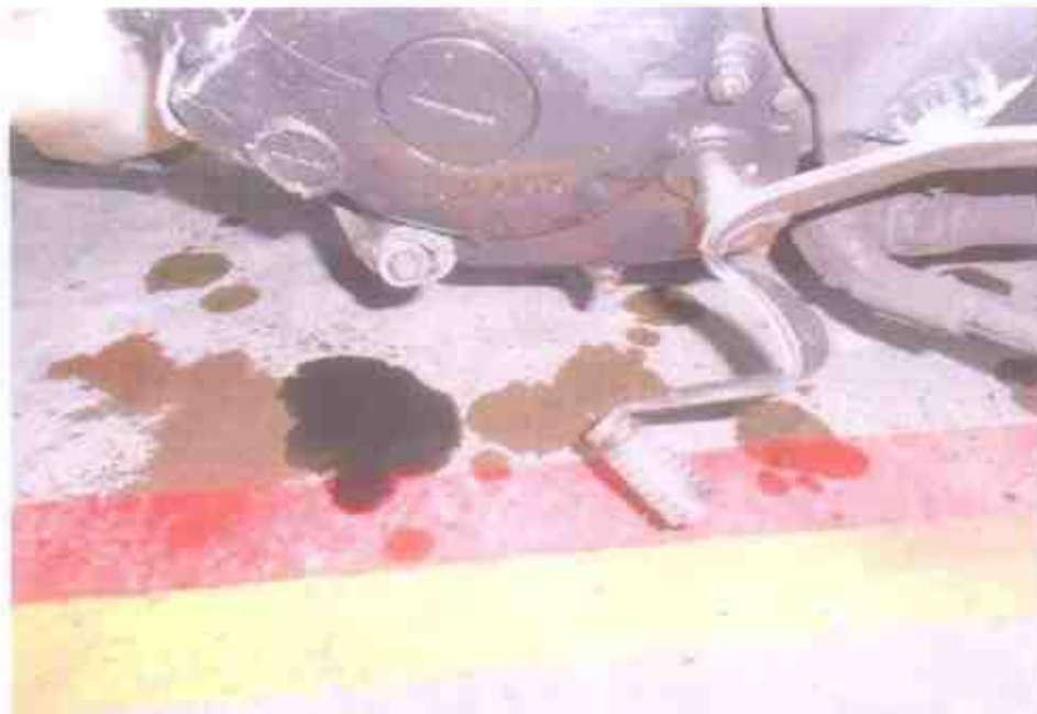
Photo 10 shows sign(s) or indication(s) of fluid leakage observed around the engine's area & fluid stain on the floor right under the engine pan of the Motorcycle.
