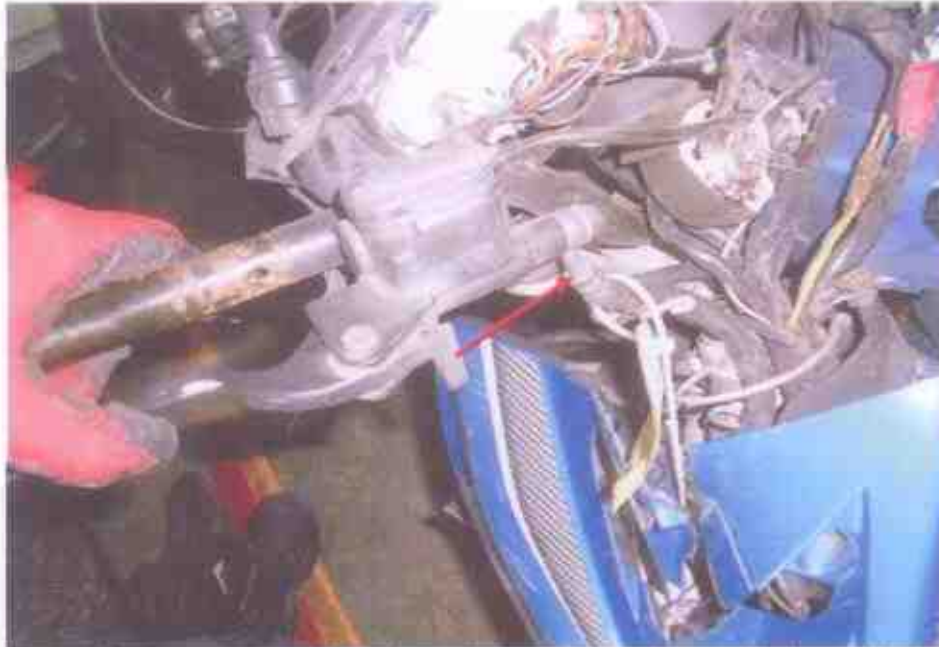
Photo 13 shows the hand brake lever (arrowed) was observed to be unaffected by the accident. However, we are unable to conduct any tests on the braking system of the Motorcycle due to some other braking system were damaged as a result of the accident.
