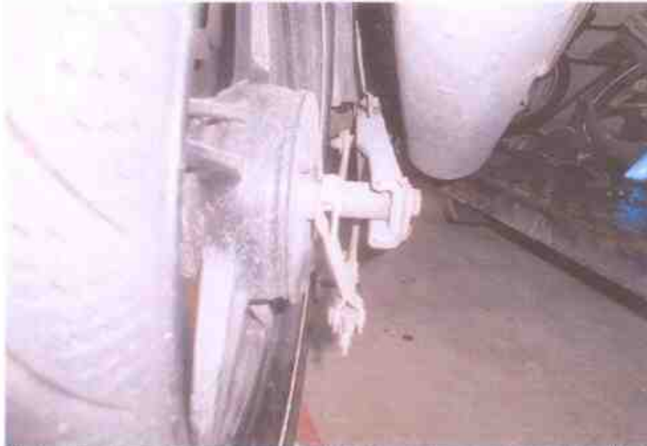
Photo 17 shows the rear brake pedal (arrowed) was observed to be in serviceable unaffected by the accident.
