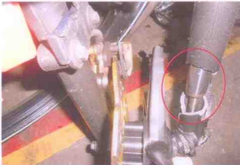
Photo 18 shows the front fork (circled) was observed to be broken & the brake disc was damaged as a result of the accident. Hence, we are unable to conduct any tests on the steering system of the Motorcycle. However, the brake pad was noted to be with sufficient frictional material at time of our inspection.
