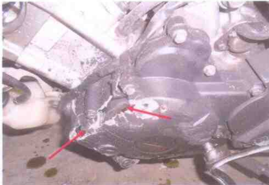
Photo 9 shows sign(s) or indication(s) of fluid leakage observed around the engine's underside area of the Motorcycle.
