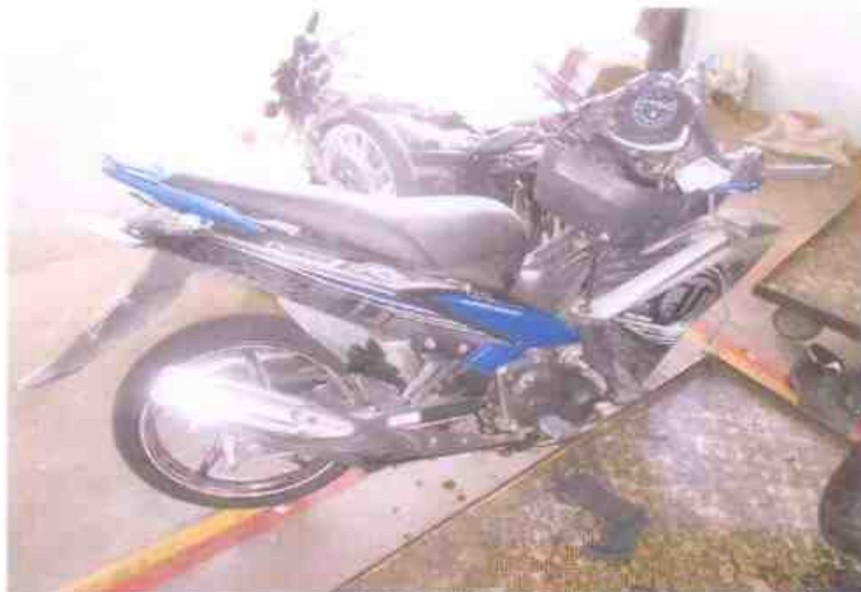
Photo 5 shows a general view of the right portion of the Motorcycle at the time of our inspection. The Motorcycle was observed to have sustained relatively extensive impact due to the accident collision.
