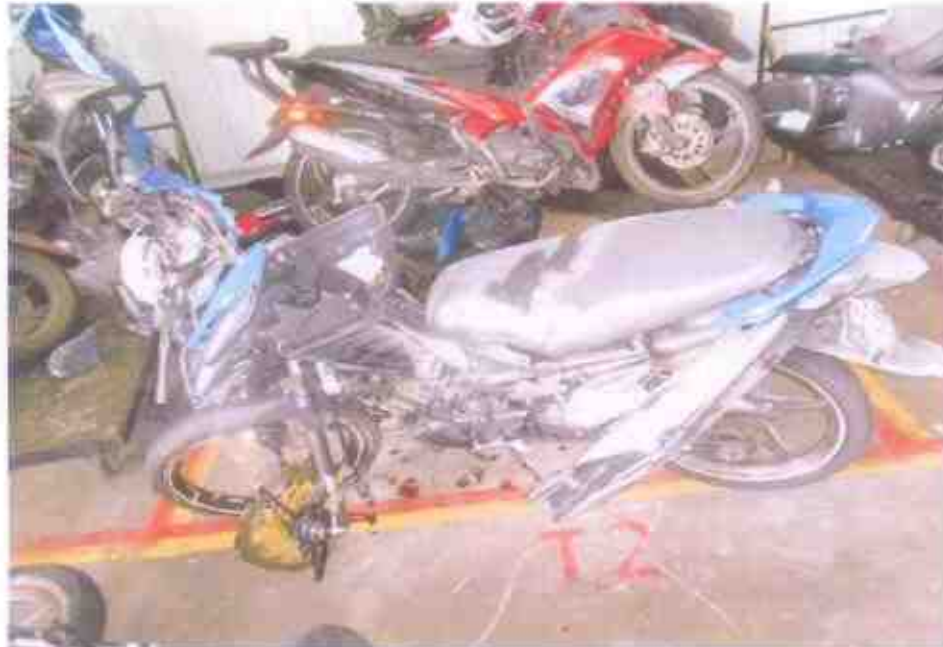
Photo 4 shows a general view of the left body of the Motorcycle at the time of our inspection. The Motorcycle was observed to have sustained damages at the frontal portion, rear portion, along both its left side and right side.
