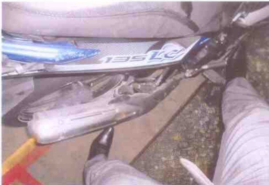
Photo 16 shows the rear brake pedal (arrowed) was observed to be in serviceable unaffected by the accident.
