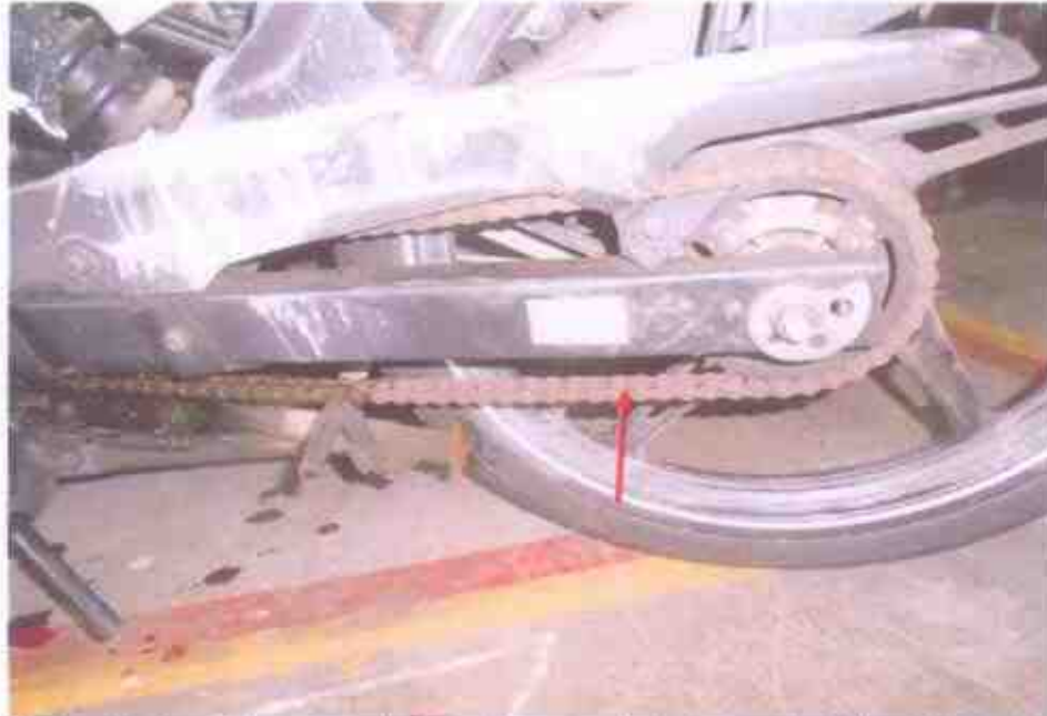
Photo 11 shows the general view of the gear train (arrowed) of the Motorcycle, which was observed to be intact with no misalignment. It was also adequately lubricated for operating purposes.
