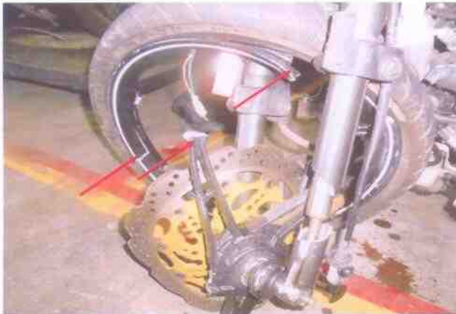
Photo 15 shows the front brake was observed to be dislodged from the original installation affected by the accident.
