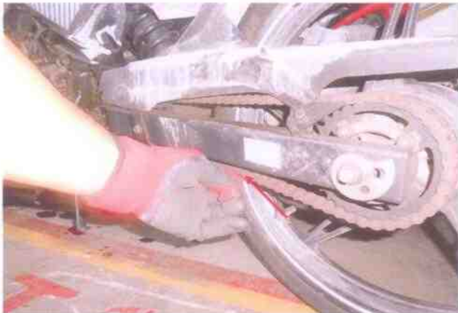
Photo 12 shows the general view of the gear train (arrowed) of the Motorcycle, which was observed to be intact with no misalignment. It was also adequately lubricated for operating purposes.
