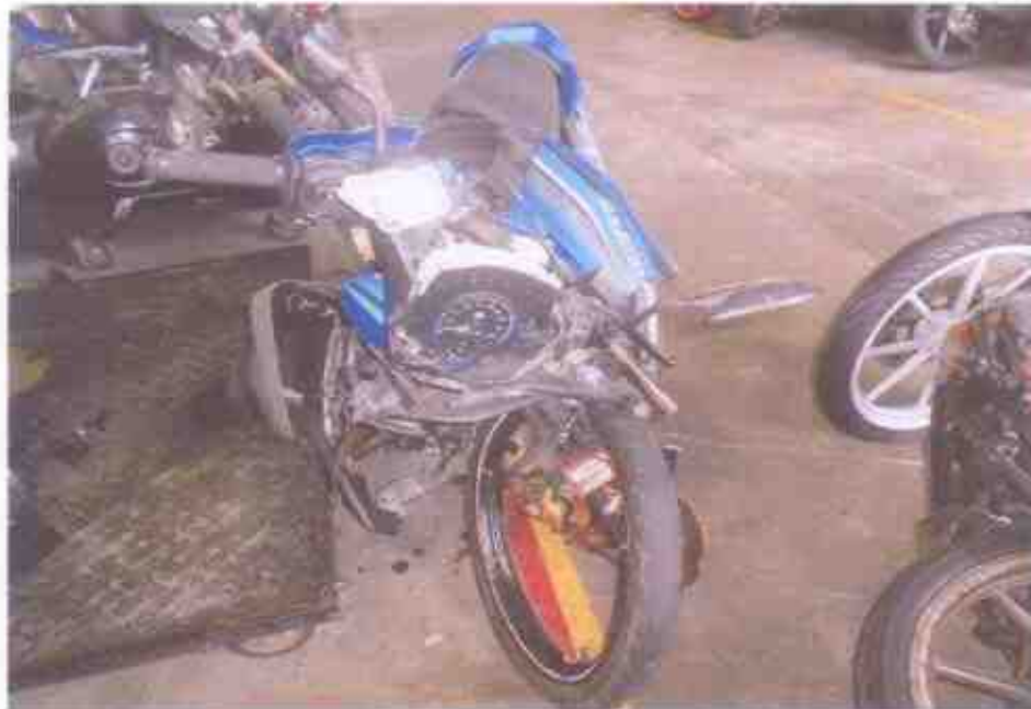
Photo 6 shows a close-up view of the frontal portion of the Motorcycle at the time of our inspection. The Motorcycle was observed to have sustained relatively extensive impact including damages to the steering system to the accident collision.
