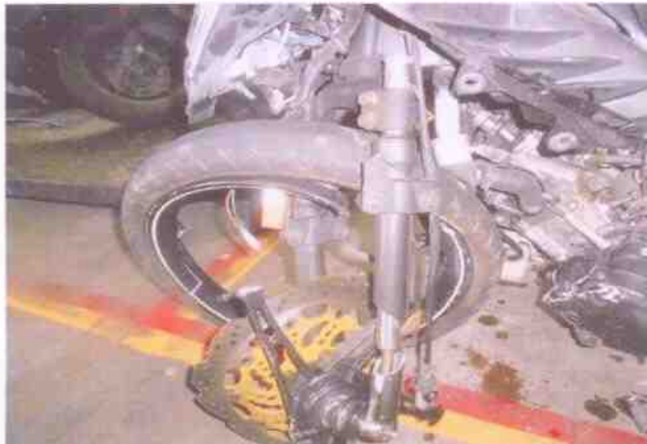
Photo 8 shows the front tyre of the Motorcycle at the time of our inspection. The pattern of the tread was clearly visible. There was no tear, burst mark(s) and/or punctured hole(s) on the sidewalls as well as across the tread of the front tyre. However, the wheel rim was observed to be broken as a result of the accident.
