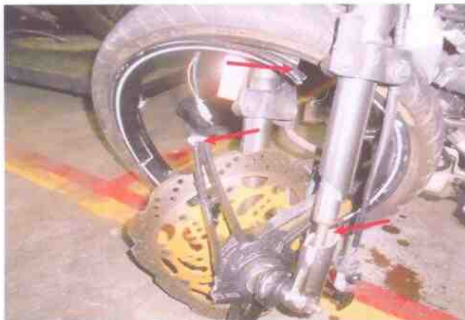
Photo 3 shows a general view of the front wheel of the Motorcycle at the time of our inspection. The Motorcycle was observed to have sustained with relatively extensive impact due to the accident collision. Amongst the body parts damaged was its front fork & broken rim (arrowed), which was observed to be broken.
