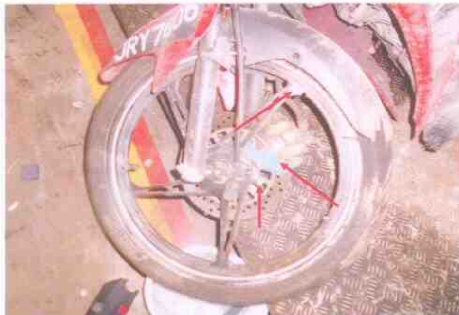
Photo 15 shows the front wheel rim & braking components was observed to be damaged by the accident.
