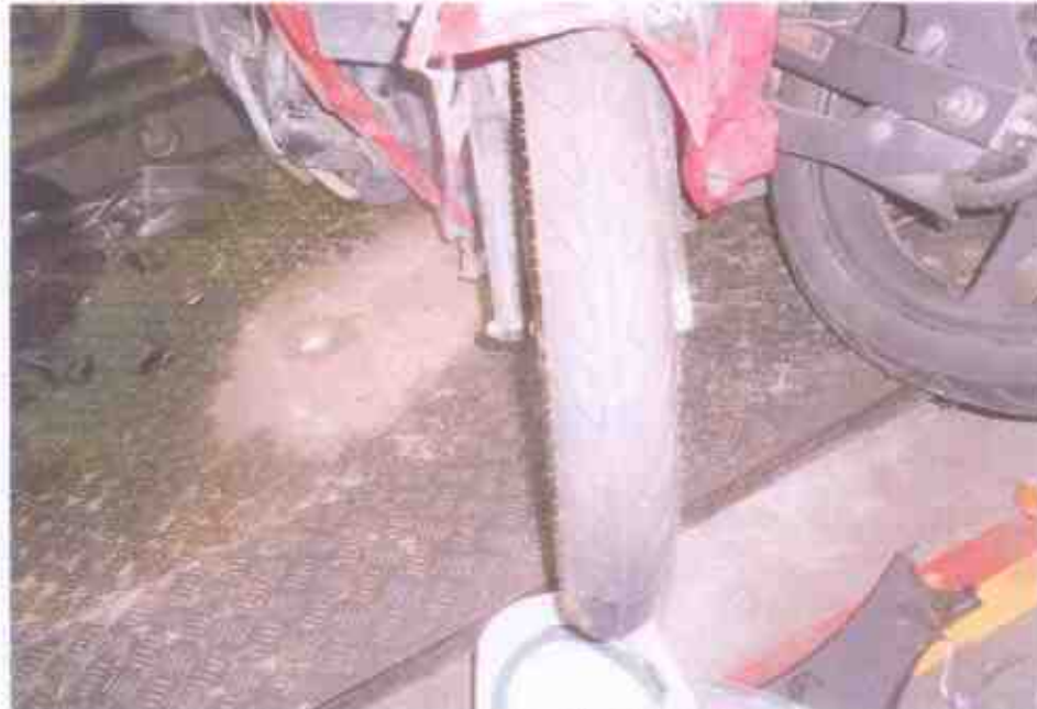
Photo 8 shows the front tyre of the Motorcycle at the time of our inspection. The pattern of the tread was clearly visible with remaining tread depth of approximately 5mm. There was no tear, burst mark(s) and/or punctured hole(s) on the sidewalls as well as across the tread of the front tyre. However, the wheel rim was observed to be broken as a result of the accident.
