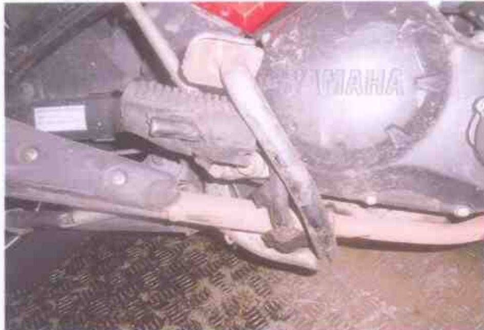
Photo 16 shows the rear brake pedal (arrowed) was observed to be in damaged due to the accident's impact collision.
