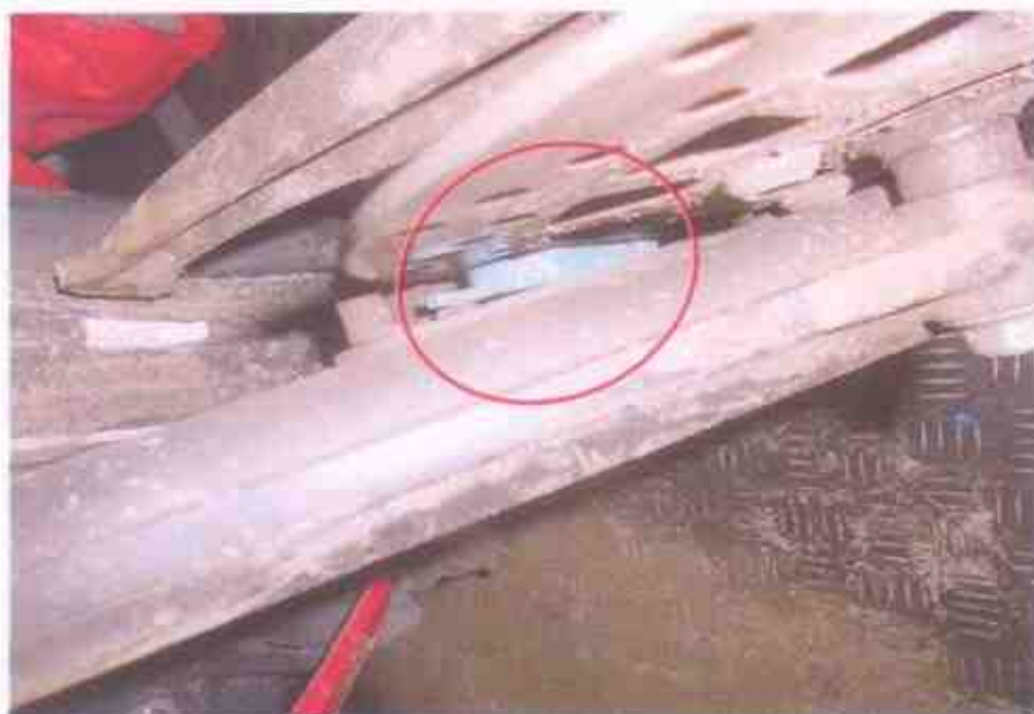
Photo 19 shows the brake pad was noted to be with sufficient frictional material at time of our inspection.
