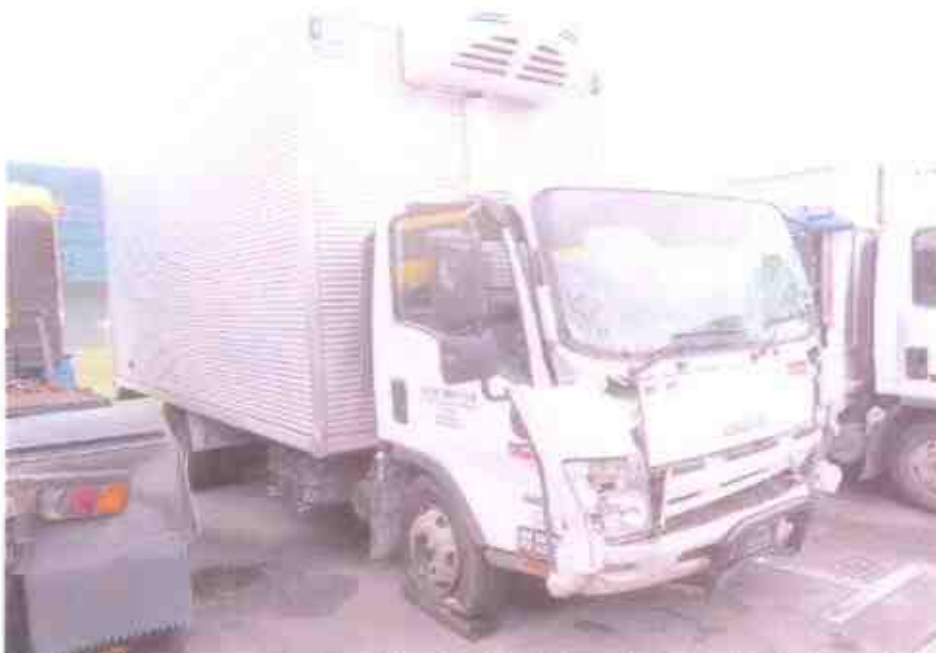
Photo 2 shows a general view of the frontal right portion of the Motor Lorry at the time of our inspection. The Motor Lorry was observed to have sustained extensive impact damage at its frontal portion. The impact force was relatively significant, causing its front portion to be pushed towards the rear.
