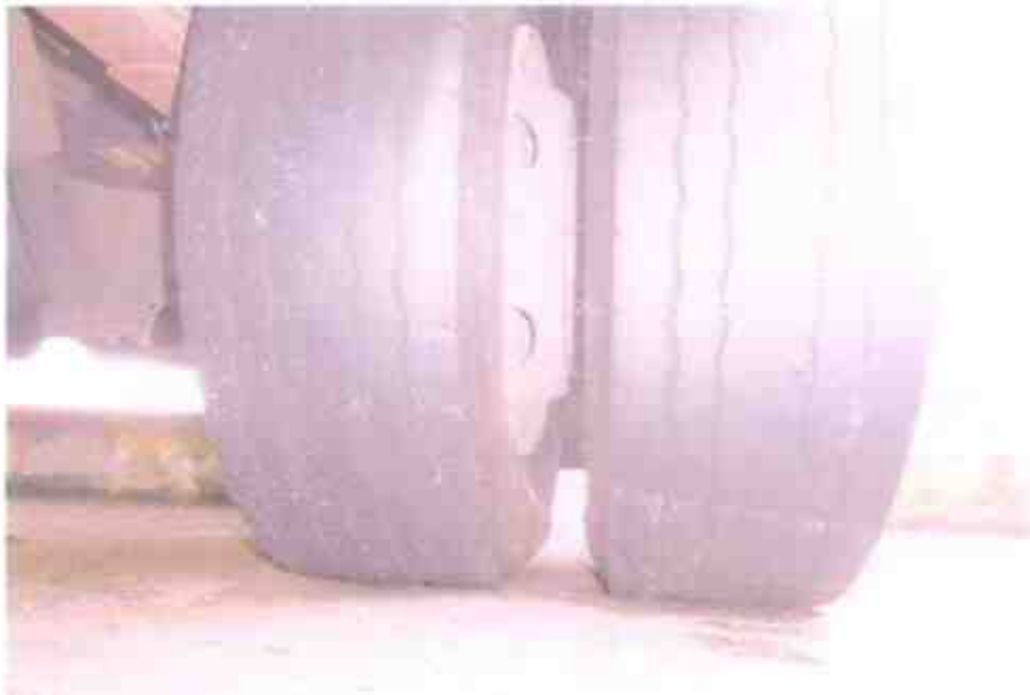
Photo 12 shows the condition of the rear left tyres of the Motor Lorry with remaining tread depth of approximately 1.6mm. However, the inner tyre was found to be deflated with dented wheel rim.
