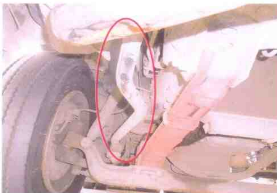
Photo 18 shows the steering rod of the Motor Lorry. It was observed to be in serviceable condition unaffected by the accident's impact collision.
