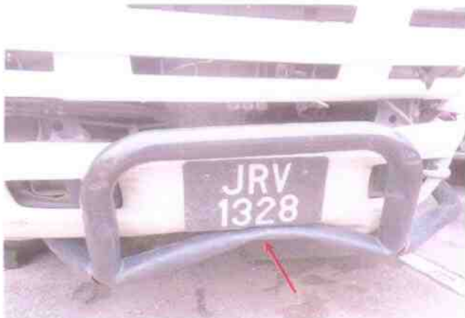
Photo 7 shows a closer view of the frontal lower portion (crash bar) of the Motor Lorry at the time of our inspection. A number of mechanical parts and components at the frontal portion were also severely damaged as a result of the accident.
