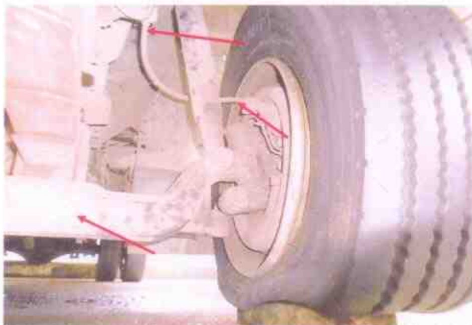
Photo 19 shows the unaffected mechanical components on the front left wheel of the steering system. The steering shaft and steering rack of the Motor Lorry were observed to be intact and securely attached to the front left wheel. No fluid leakage on the brake fluid hoses.
