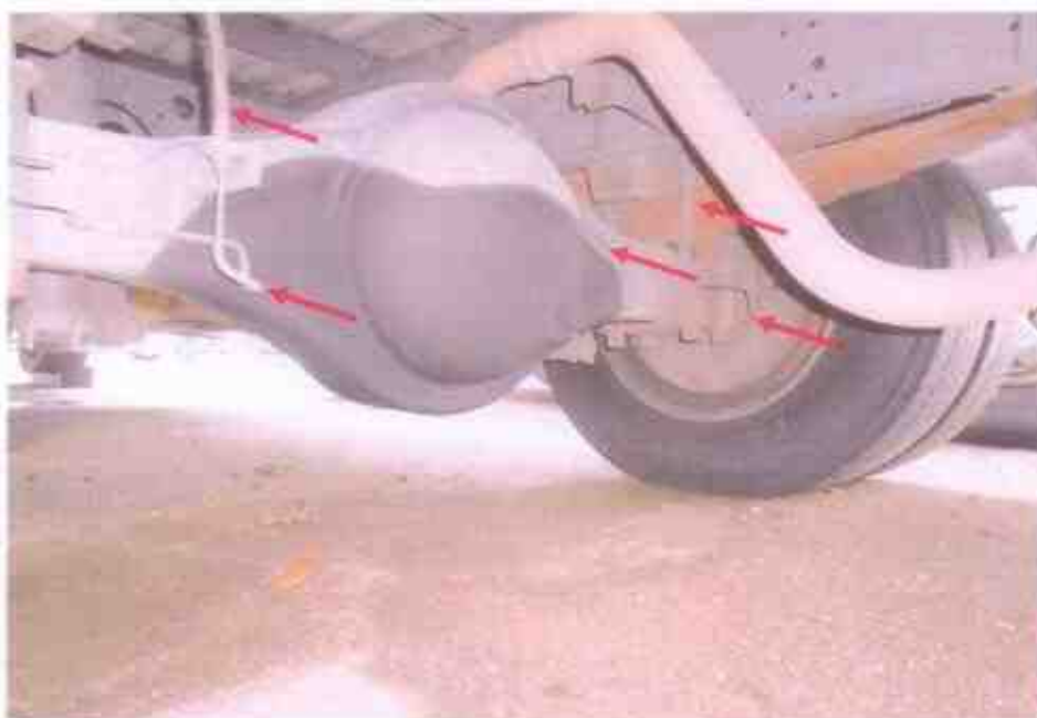
Photo 23 shows the brake pipes and hoses, which were visibly unaffected by the accident. We were however not able to carry out any operational tests to the braking system of the Motor Lorry due to the extent of damage to its front cabin, which had affected several mechanical components of the braking system like the brake booster and brake pedal amongst others.
