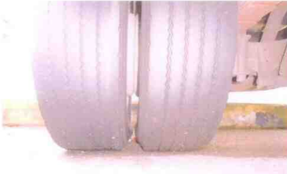
Photo 11 shows the condition of the rear right tyres of the Motor Lorry with remaining tread depth of approximately 4mm. However, the outer tyre was found to be deflated with cut mark on the outer sidewall & dented wheel rim.
