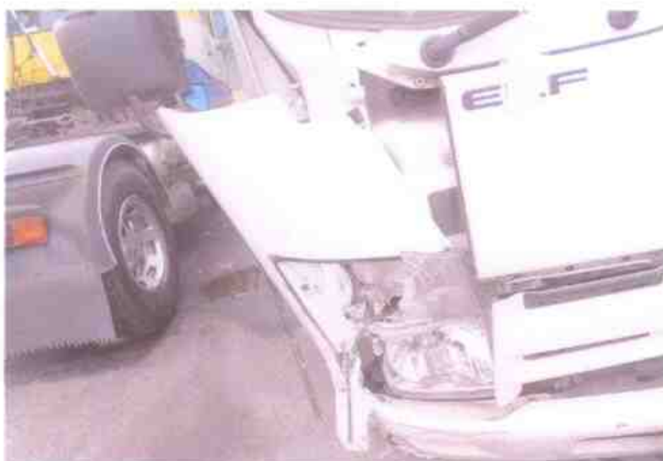
Photo 6 shows a closer view of the right headlamp of the Motor Lorry at the time of our inspection. It had also sustained damages on other components as a result of the accident.
