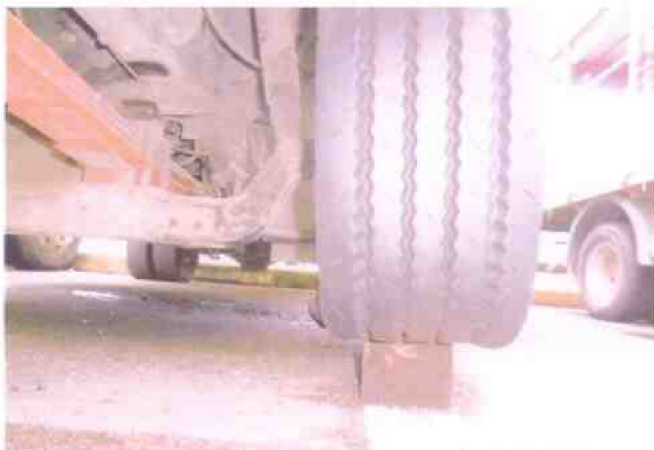
Photo 13 shows the condition of the front left tyre of the Motor Lorry with remaining tread depth of approximately 8mm. However, it was found to be deflated with cut mark on the sidewall & dented wheel rim.
