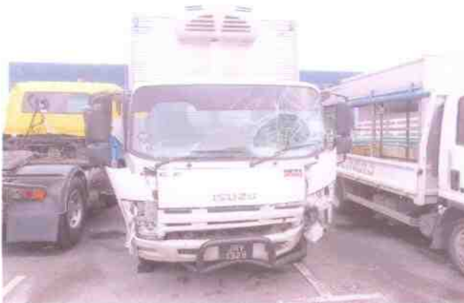
Photo 1 shows a general view of the frontal portion of the Motor Lorry at the time of our inspection. The Motor Lorry was observed to have sustained extensive impact damage at its frontal portion. The impact force was relatively significant, causing its front portion to be pushed towards the rear.
