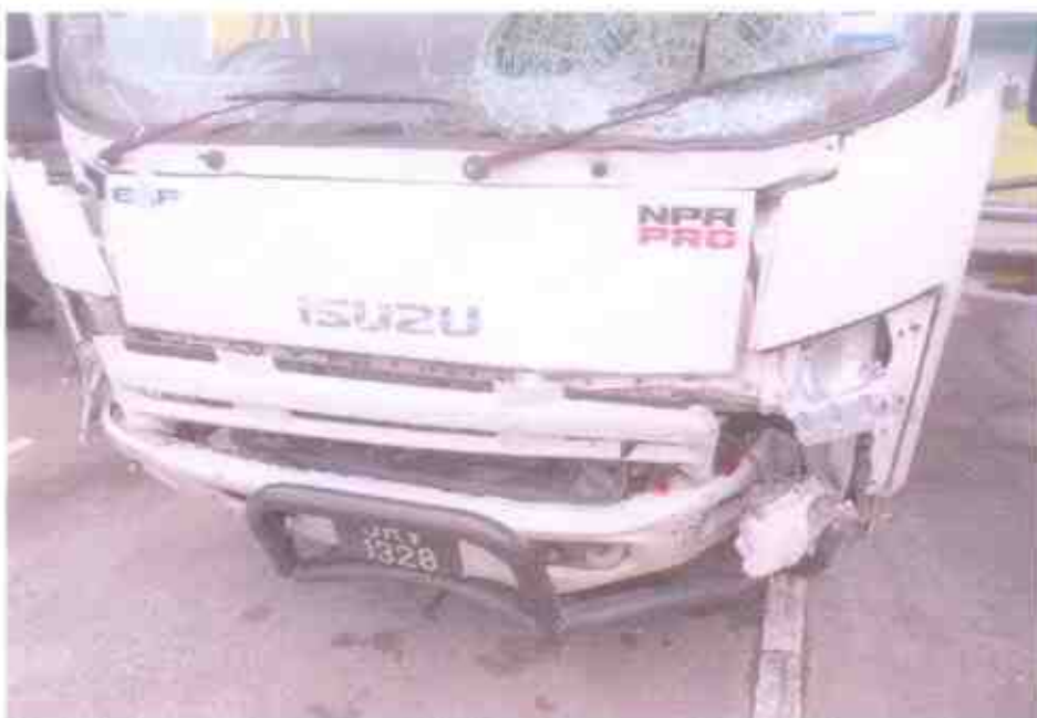
Photo 4 shows a closer view of the frontal portion of the Motor Lorry at the time of our inspection. A number of mechanical parts and components at the frontal portion were also severely damaged as a result of the accident.
