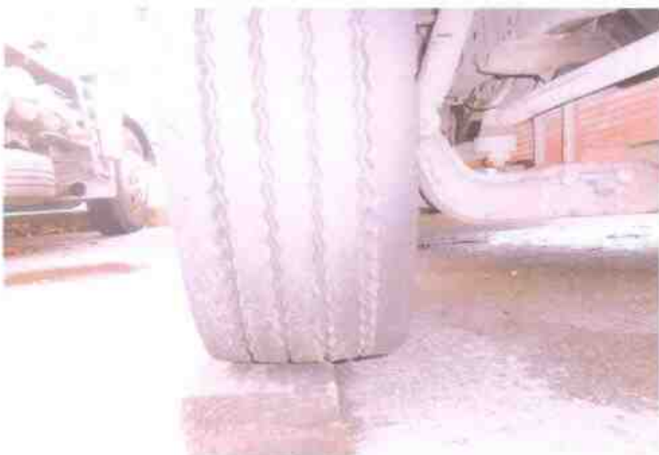
Photo 14 shows the condition of the front right tyre of the Motor Lorry with remaining tread depth of approximately 7mm. However, it was found to be deflated with dented wheel rim.
