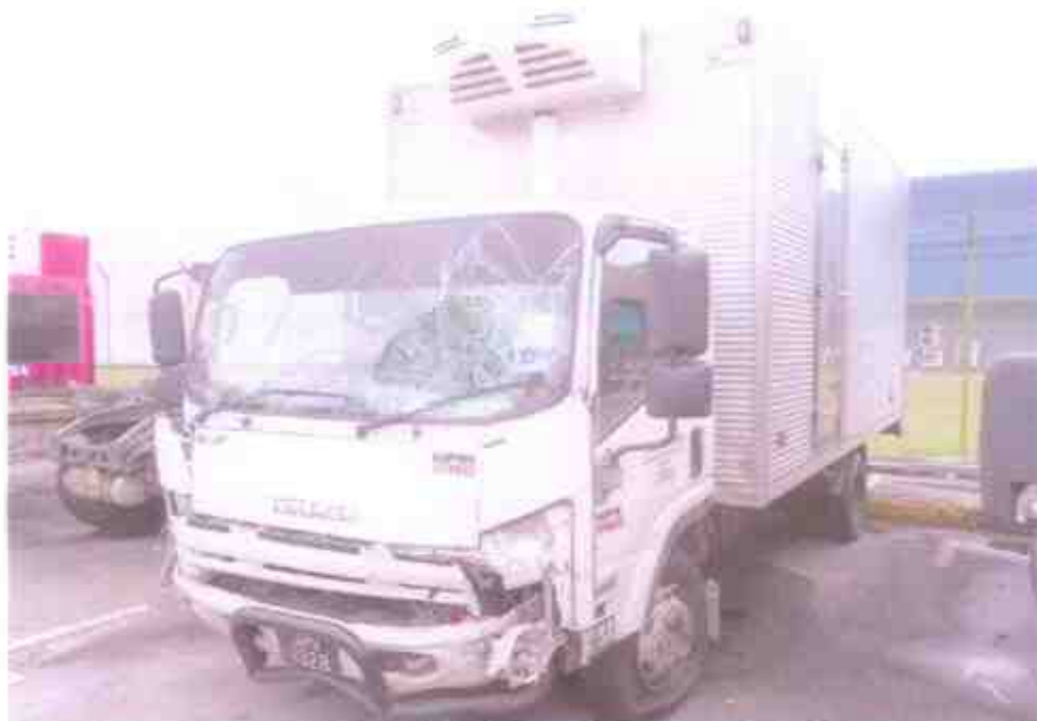
Photo 3 shows a general view of the frontal left portion of the Motor Lorry at the time of our inspection. The Motor Lorry was observed to have sustained extensive impact damage at its frontal portion. The impact force was relatively significant, causing its front portion to be pushed towards the rear.
