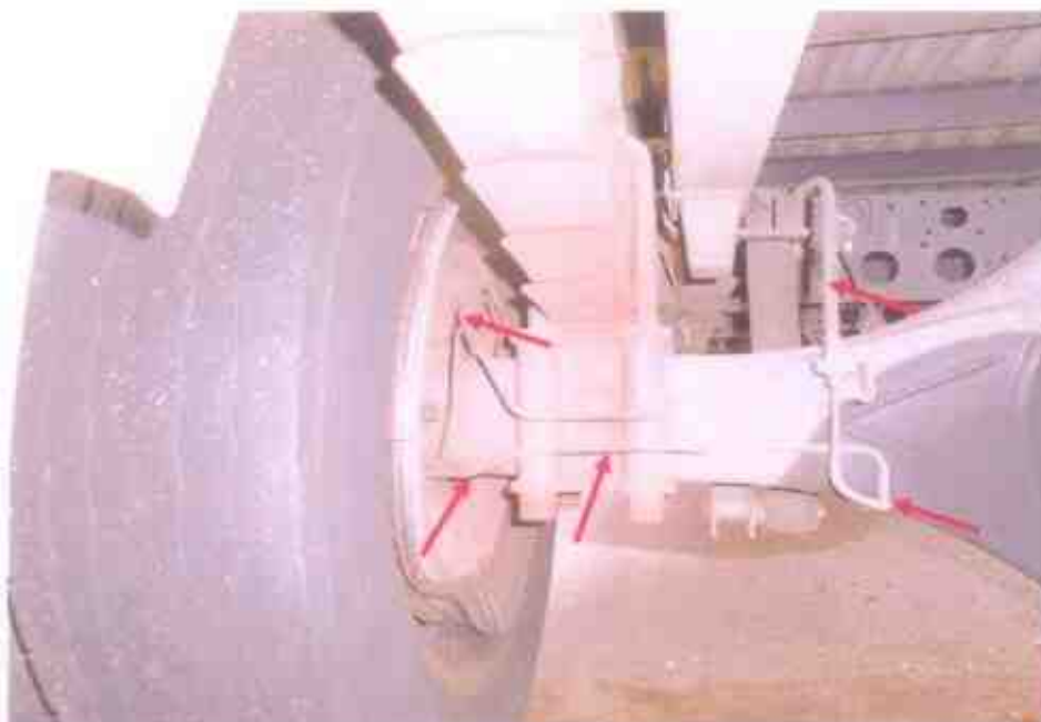
Photo 22 shows the brake pipes and hoses, which were visibly unaffected by the accident. We were however not able to carry out any operational tests to the braking system of the Motor Lorry due to the extent of damage to its front cabin, which had affected several mechanical components of the braking system like the brake booster and brake pedal amongst others.
