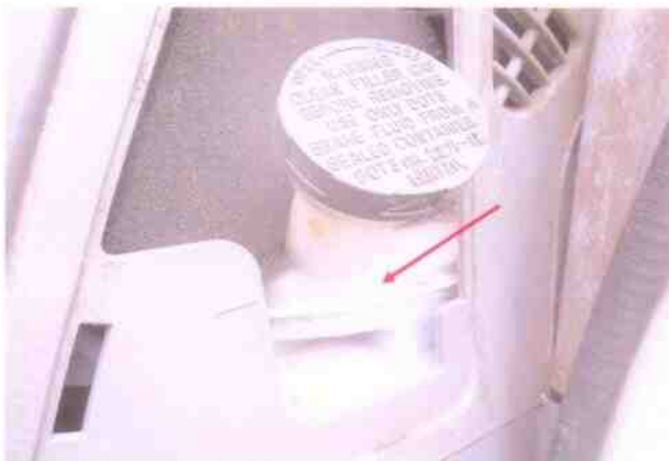
Photo 21 shows the brake fluid reservoir of the Motor Lorry. I had found the brake fluid to be of sufficient level for operational purposes. Visually there was also no contamination found to the brake fluid.
