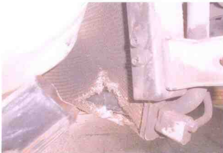
Photo 16 shows the radiator was observed to be damaged due to the accident's impact.
