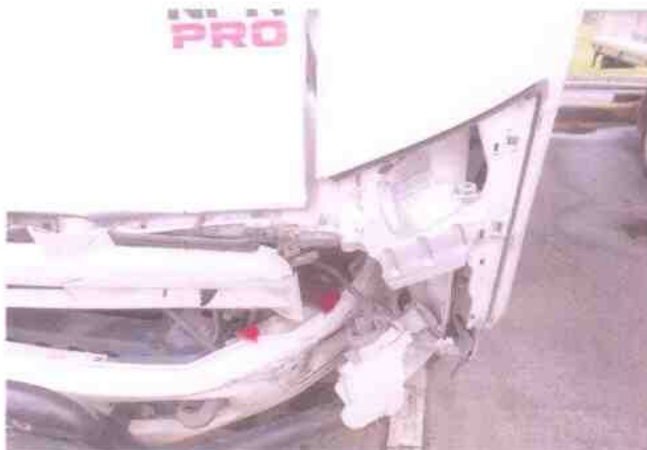
Photo 5 shows a closer view of the left headlamp of the Motor Lorry at the time of our inspection. It had also sustained damages on other components as a result of the accident.
