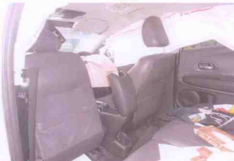
Photo 38 shows the Supplemental Restraint System (SRS) of the Motor Car was however likely to be in normal operating condition at the material time of the accident. The evidence of the deployed right window's airbag indicates that the impact sensors and control module of the Motor Car's SRS were all in serviceable condition at the material time of accident.
