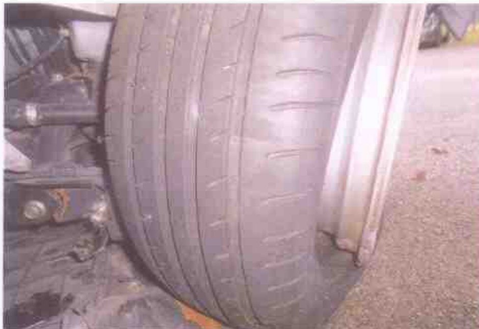
Photo 15 shows the condition of the front left tyre of the Motor Car, which was observed to be deflated not in serviceable condition. The alloy wheel rim was also observed to have come off slightly from the tyre fitting due to the accident's impact.
