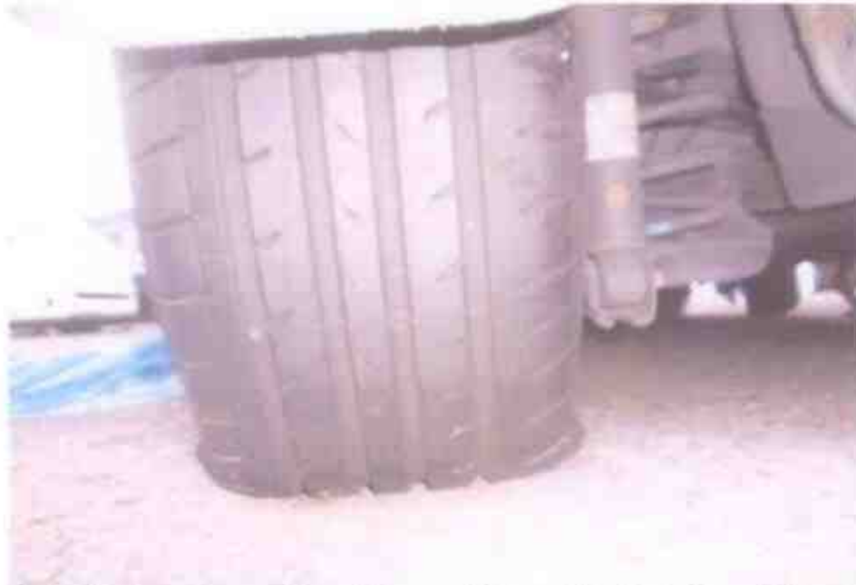
Photo 16 shows the condition of the rear left tyre of the Motor Car, which was observed to be deflated not in serviceable condition likely due to the accident's impact collision. However, its tread depth was clearly visible, measured approximately around 6mm.
