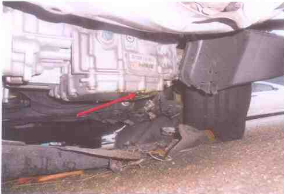
Photo 21 shows the close up view of the undercarriage of the Motor Car. Signs of fluid leakage were observed due to the accident's impact.
