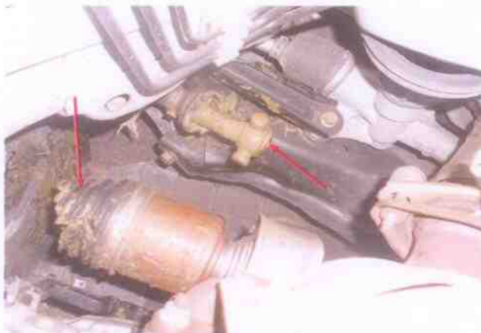
Photo 29 shows a close up view on the front right drive shaft of the Motor Car that were damaged due to the accident's impact collision.
