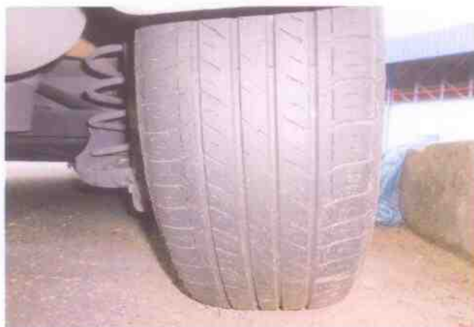
Photo 19 shows the condition of the rear right tyre of the Motor Car, which was observed to be deflated not in serviceable condition likely due to the accident's impact collision. However, its tread depth was clearly visible, measured approximately around 6mm.
