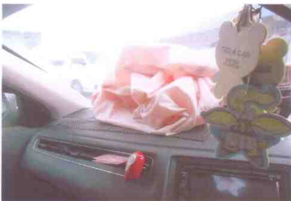
Photo 9 shows a closer view of the left front passenger seat of the Motor Car. The impact force was significant, causing the airbag to be activated.
