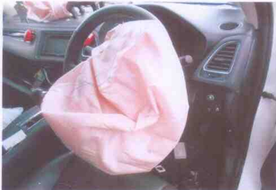
Photo 35 shows the Supplemental Restraint System (SRS) of the Motor Car was however likely to be in normal operating condition at the material time of the accident. The evidence of the deployed front driver's airbag indicates that the impact sensors and control module of the Motor Car's SRS were all in serviceable condition at the material time of accident.
