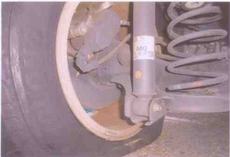
Photo 33 shows the rear left braking & undercarriage components that was unaffected by the accident's impact collision.
