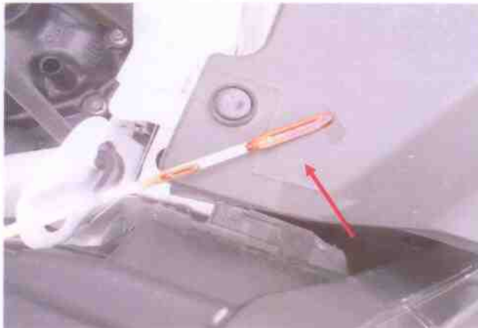
Photo 26 shows a close up view of the engine fluid. Despite there's leakage to the engine fluid, it still contain sufficient level.
