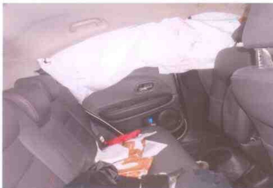
Photo 10 shows a closer view of the damages at the interior portion of the Motor Car due to the extensive impact collision at time of the accident. The window's airbag was also observed to be activated.
