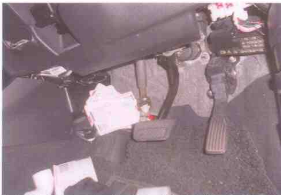
Photo 6 shows a closer view of the damage at the frontal internal portion of the Motor Car which includes the steering system & ignition system. The impact force was significant, causing the various parts and components inside the interior cabin to be pushed inwards, towards the rear of the Motor Car.
