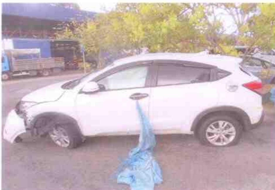
Photo 7 shows a general view of the damage at the left portion of the Motor Car. The impact force was significant, causing the body structure to be affected by the accident's impact collision.
