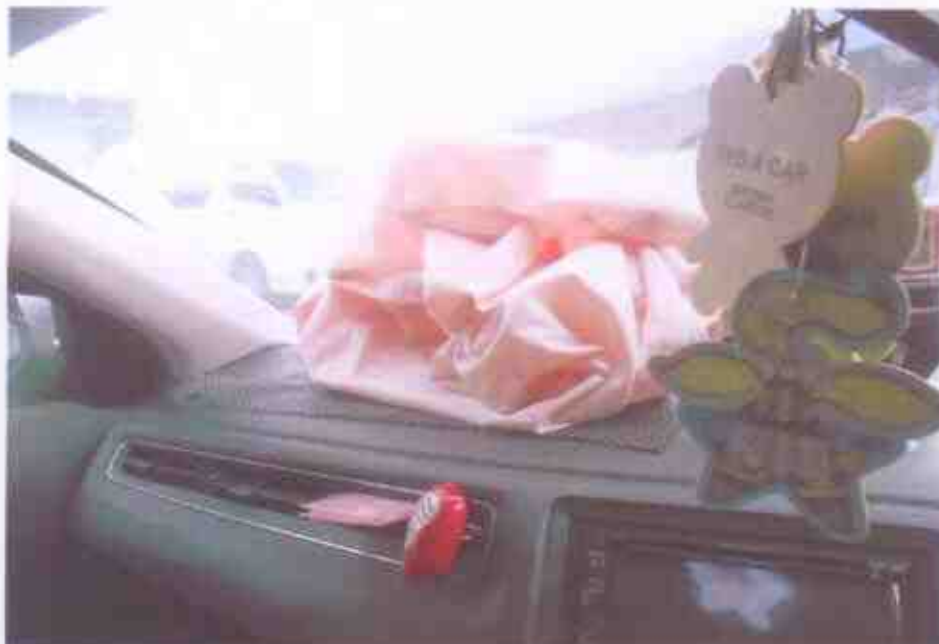
Photo 36 shows the Supplemental Restraint System (SRS) of the Motor Car was however likely to be in normal operating condition at the material time of the accident. The evidence of the deployed front passenger's airbag indicates that the impact sensors and control module of the Motor Car's SRS were all in serviceable condition at the material time of accident.
