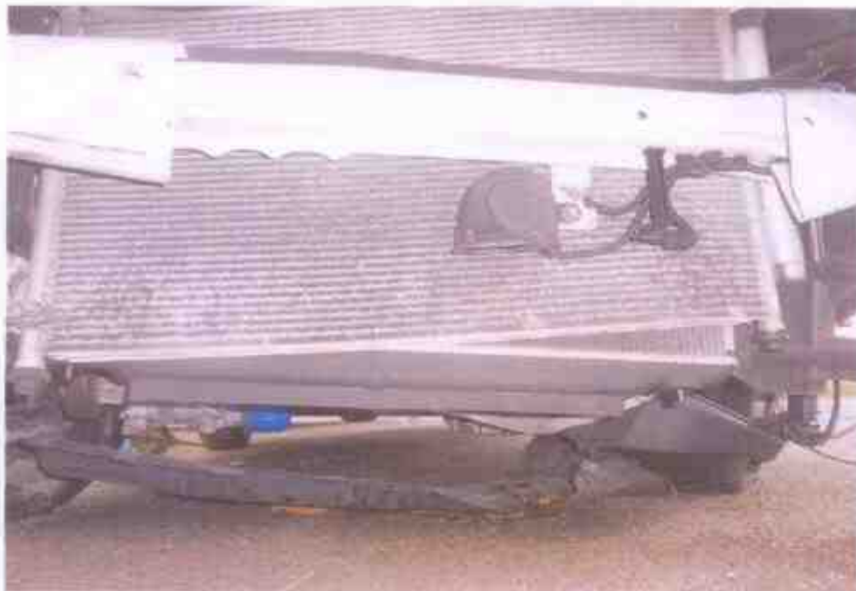
Photo 22 shows the close up view of the radiator's tank that was observed to be damaged likely due to the accident impact.
