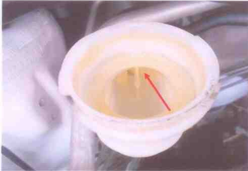
Photo 25 shows a close up view of an empty brake fluid reservoir due to the accident impact. It relatively affects the braking system.
