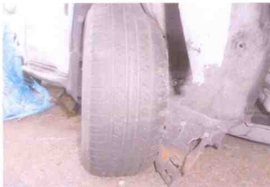
Photo 13 shows the condition of the front right portion of the Motor Car, which was observed to be in severe damage. The tyre was found to be deflated & the alloy wheel rim was damaged due to the accident's impact.
