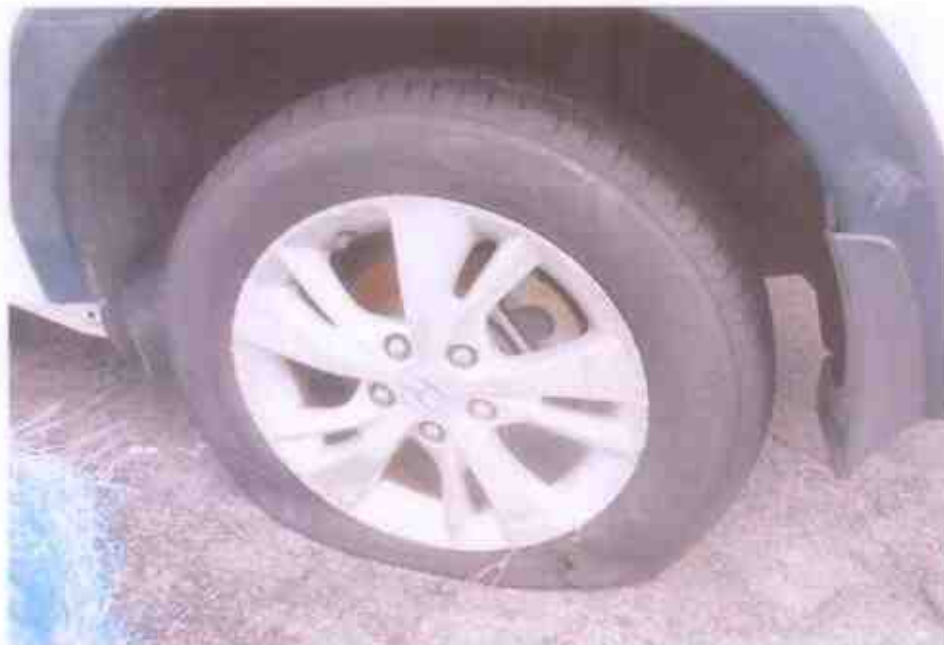
Photo 17 shows the condition of the rear left tyre of the Motor Car, which was observed to be deflated not in serviceable condition likely due to the accident's impact collision. However, its tread depth was clearly visible, measured approximately around 6mm.
