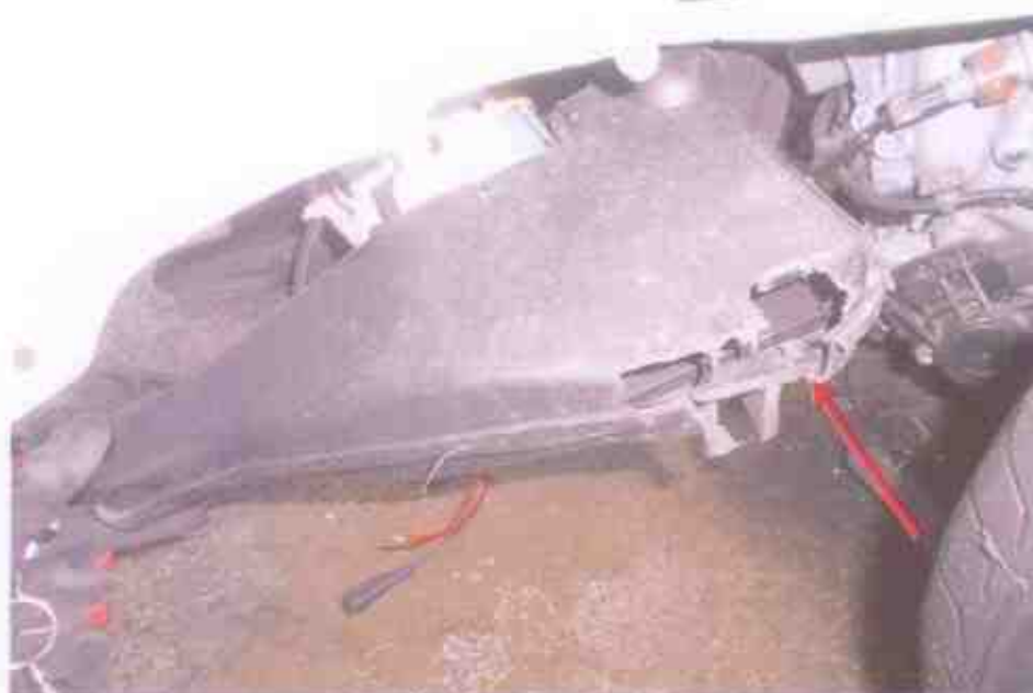
Photo 23 shows the close up view of the damage air intake due to the accident impact.
