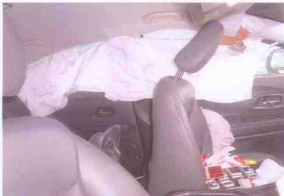
Photo 37 shows the Supplemental Restraint System (SRS) of the Motor Car was however likely to be in normal operating condition at the material time of the accident. The evidence of the deployed left window's airbag indicates that the impact sensors and control module of the Motor Car's SRS were all in serviceable condition at the material time of accident.
