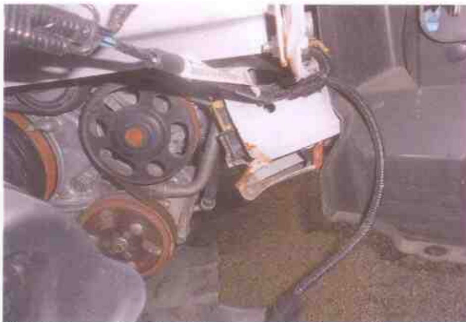
Photo 5 shows a closer view of the damage at the frontal right portion of the Motor Car. The impact force was significant, causing the re-inforcement bar to be pushed inwards.
