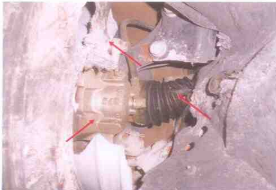
Photo 30 shows the damaged on the front left drive shaft of the Motor Car. We were not able to conduct any tests on the steering system of the Motor Car due to the damage to this components, as well as leakage of fluids.
