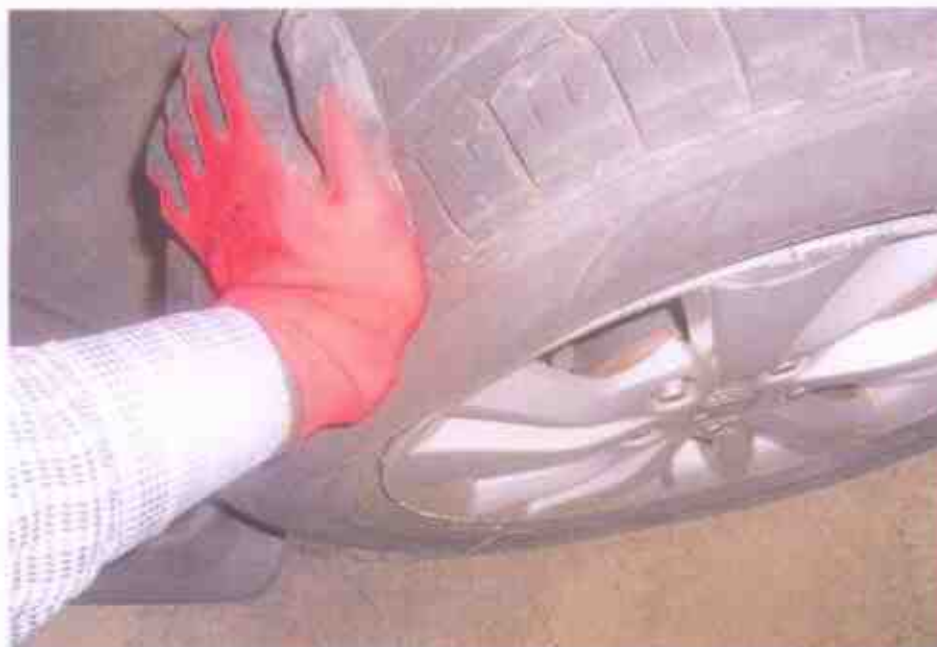
Photo 20 shows the condition of the rear right tyre of the Motor Car, which was observed to be deflated not in serviceable condition likely due to the accident's impact collision. However, its tread depth was clearly visible, measured approximately around 6mm.
