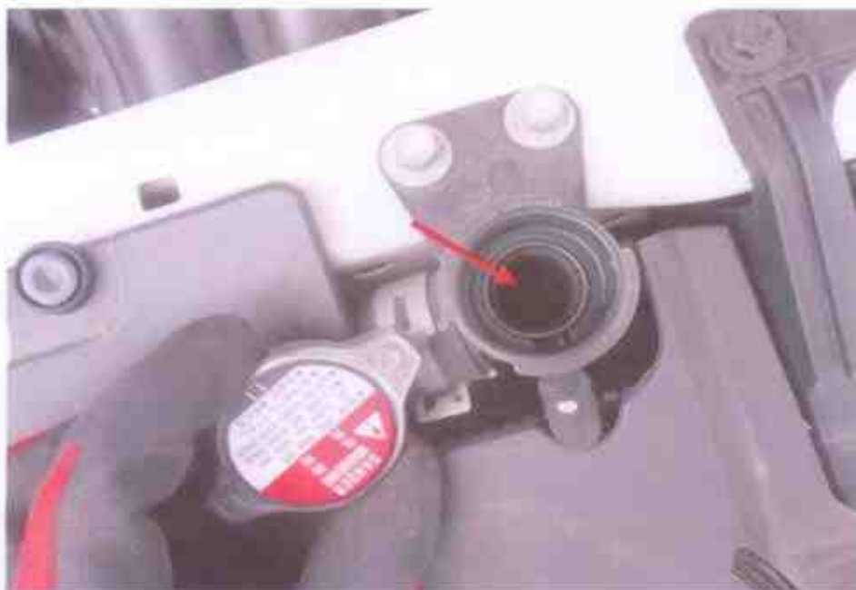
Photo 24 shows the close up view of the empty coolant fluid reservoir due to the damages sustained due to the accident's impact.
