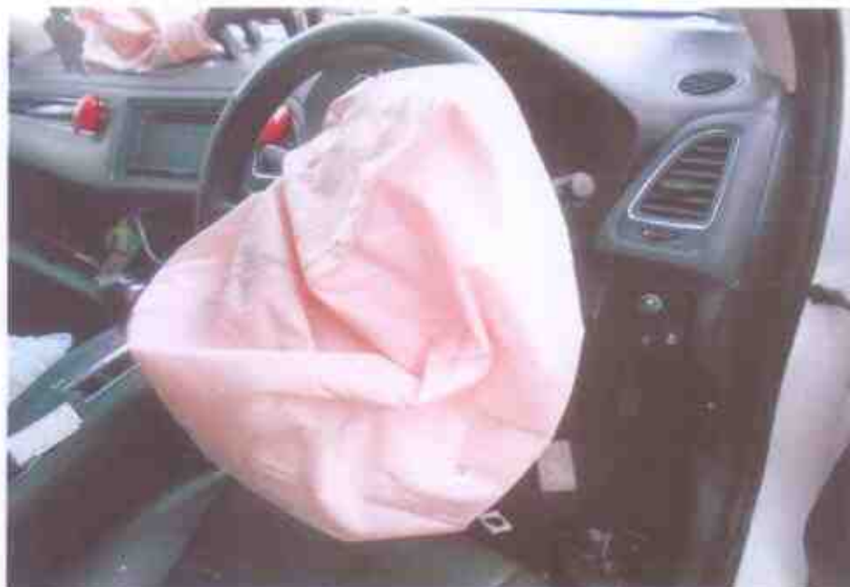
Photo 8 shows a closer view of the damage at the driver's seat of the Motor Car. The impact force was significant, causing the various parts and components inside the interior compartment to be pushed inwards, including its ignition system. The driver's airbag was also activated.
