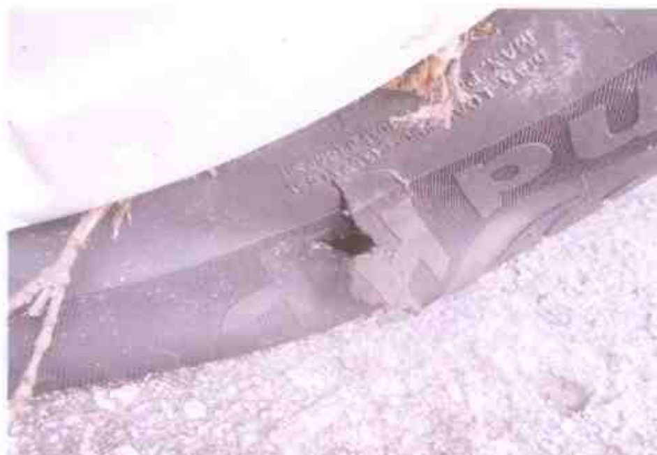
Photo 18 shows the condition of the rear left tyre of the Motor Car, which was observed to be deflated not in serviceable condition likely due to the accident's impact collision. However, its tread depth was clearly visible, measured approximately around 6mm.
