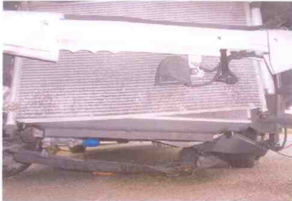
Photo 4 shows a closer view of the damage at the frontal portion of the Motor Car's engine. The impact force was significant, causing the various parts and components inside the engine compartment to be pushed inwards.
