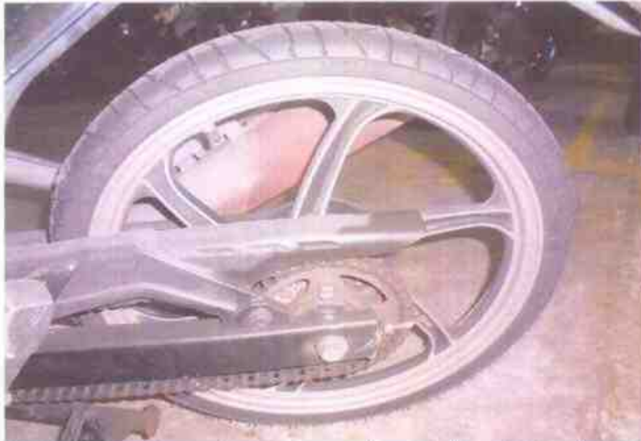
Photo 12 shows the rear tyre was wrapped around alloy wheel rim that was found to be without any significant damage.
