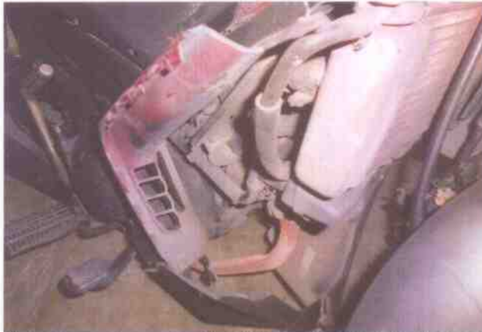
Photo 7 shows a close-up view of the right fairing of the Motorcycle at the time of our inspection. The Motorcycle was observed to be sustained relatively extensive impact due to the accident collision.
