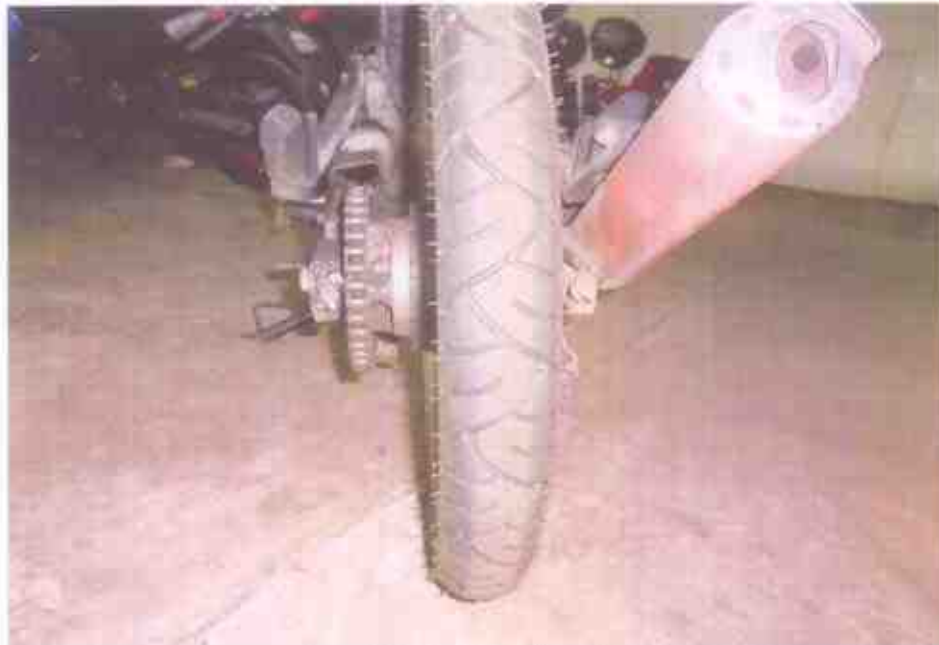
Photo 10 shows the rear tyre of the Motorcycle at the time of our inspection. The rear tyre was observed to be in serviceable condition with remaining tread depth of approximately 4mm. Although the rim was observed to be slightly it was also sufficiently inflated for vehicular operation.
