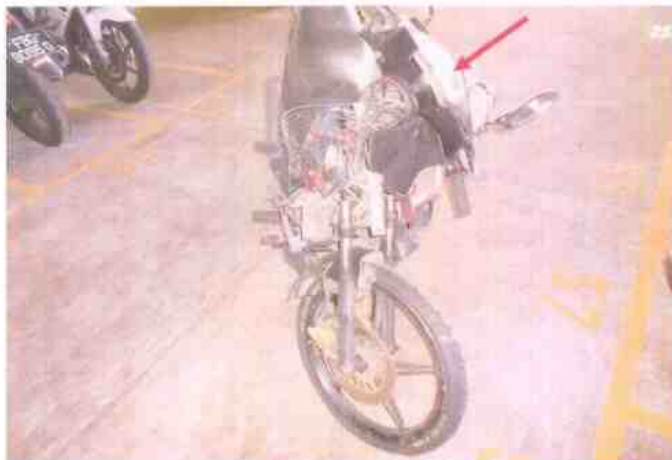
Photo 2 shows a general view of the front body of the Motorcycle at the time of our inspection. The Motorcycle was observed to be sustained with relatively extensive impact due to the accident collision. Amongst the body parts damaged was its handle bar (arrowed), which was observed to be dislodged.
