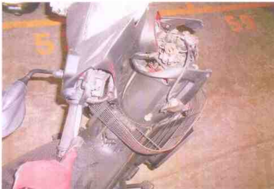
Photo 13 shows the front handle bar was observed to be dislodged as a result of the accident. Hence, we are not able to conduct any tests on the steering system of the Motorcycle.
