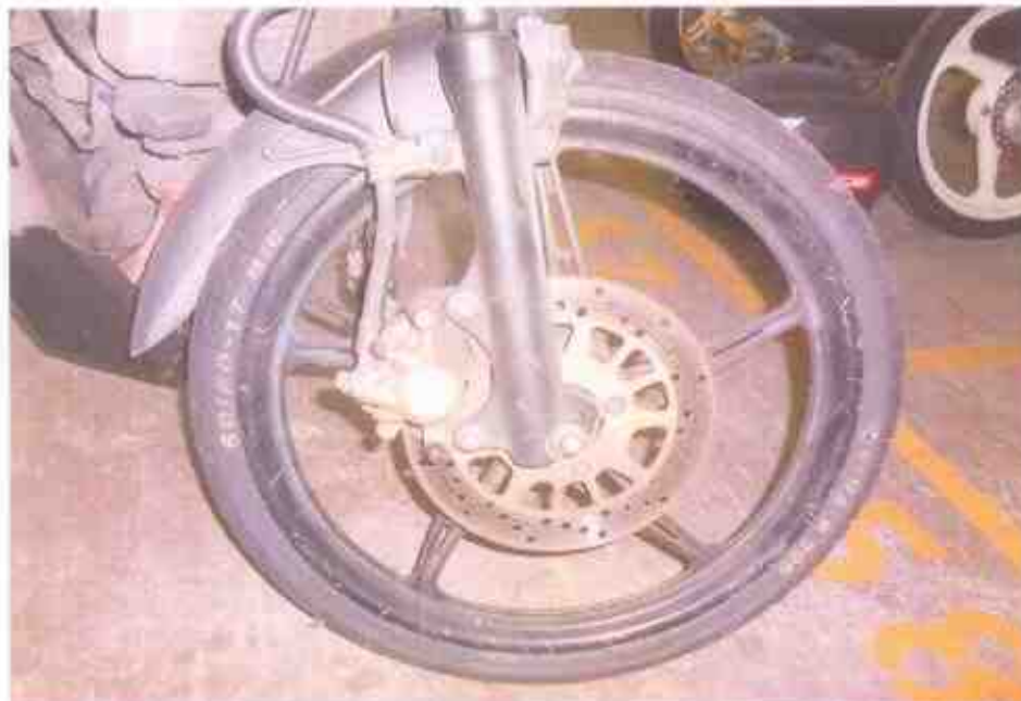
Photo 11 shows the front tyre was wrapped around alloy wheel rim that was found to be without any significant damage.
