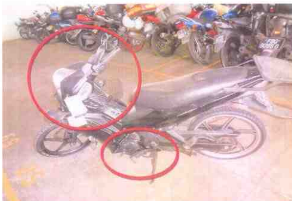
Photo 4 shows a general view of the frontal left portion of the Motorcycle at the time of our inspection. The Motorcycle was observed to be sustained relatively extensive impact due to the accident collision.
