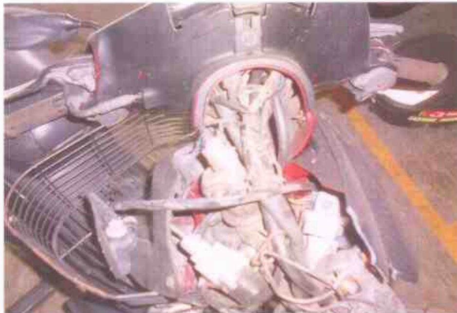
Photo 6 shows a close-up view of the damaged steering system & ignition system of the Motorcycle at the time of our inspection. The Motorcycle was observed to be sustained relatively extensive impact due to the accident collision.
