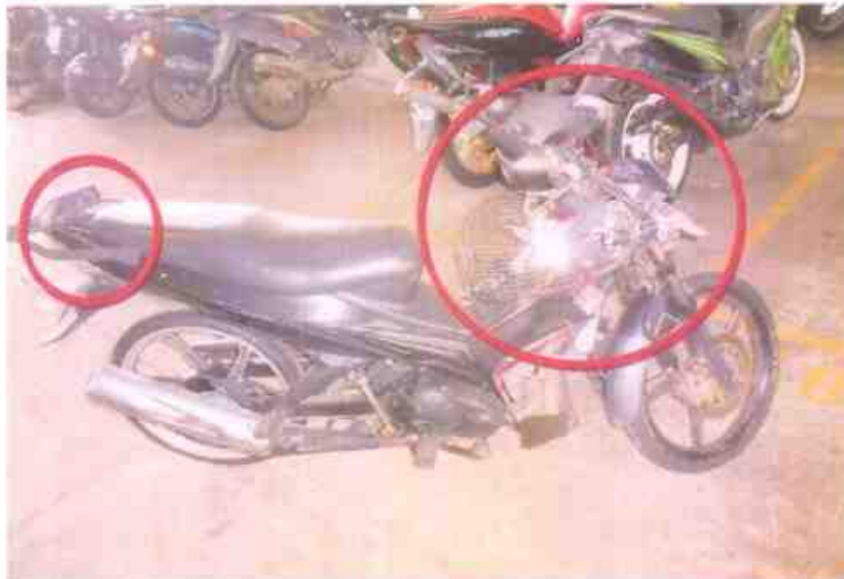
Photo 5 shows a general view of the frontal right portion of the Motorcycle at the time of our inspection. The Motorcycle was observed to be sustained relatively extensive impact due to the accident collision.
