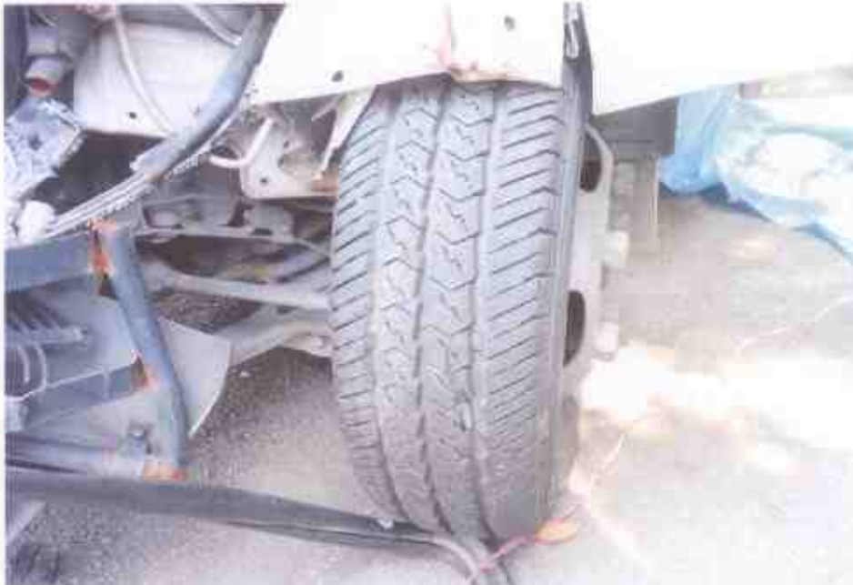
Photo 13 shows the condition of the front left tyre of the Motor Lorry, which was observed to be in serviceable condition with remaining tread depth of approximately 7mm. There was also no tear, cut or burst mark(s) on the outer and the inner sidewalls as well as across the tread of this tyre.
