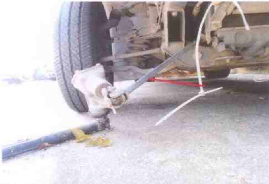
Photo 17 shows the damaged steering wheel rod (red arrow) of the Motor Lorry. Hence, we were not able to conduct any tests on the steering system of the Motor Lorry.
