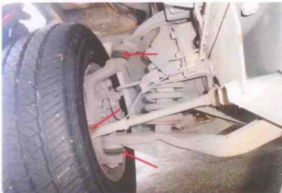
Photo 20 shows the unaffected mechanical components on the front right wheel of the steering system. The steering shaft and steering rack of the Motor Lorry were observed to be intact and securely attached to the front left wheel. No fluid leakage on the brake fluid hoses.
