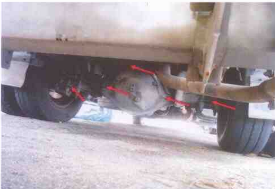
Photo 22 shows the brake pipes and hoses, which were visibly unaffected by the accident. We were however not able to carry out any operational tests to the braking system of the Motor Lorry due to the extent of damage to its front cabin, which had affected several mechanical components of the Motor Lorry.
