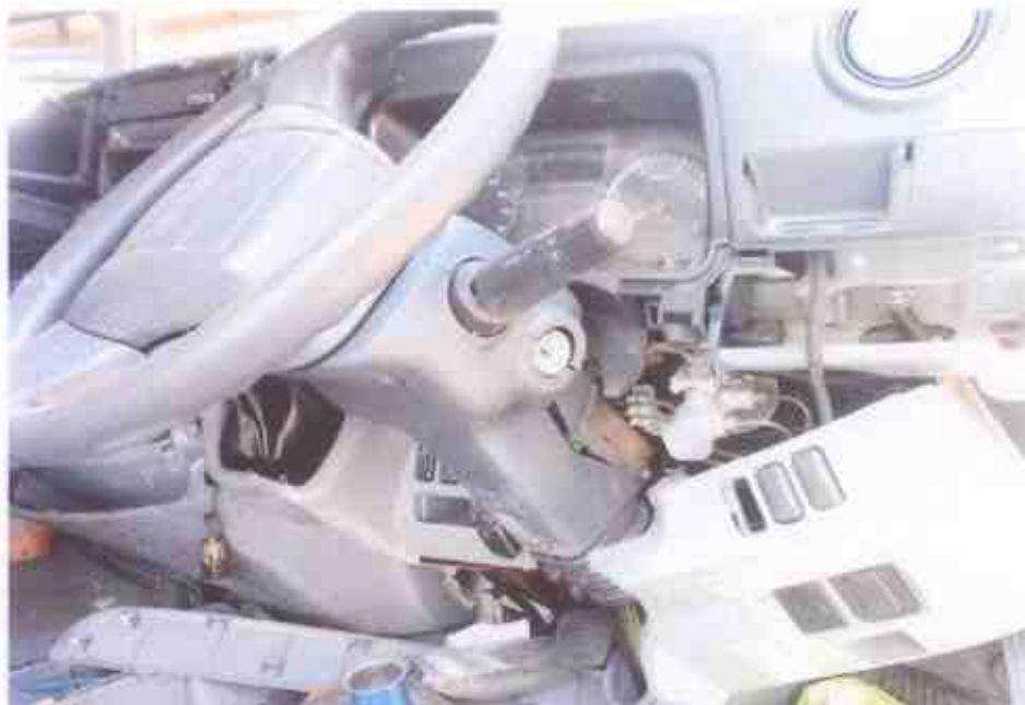
Photo 18 shows the damaged steering wheel rod due to the accident's impact.
