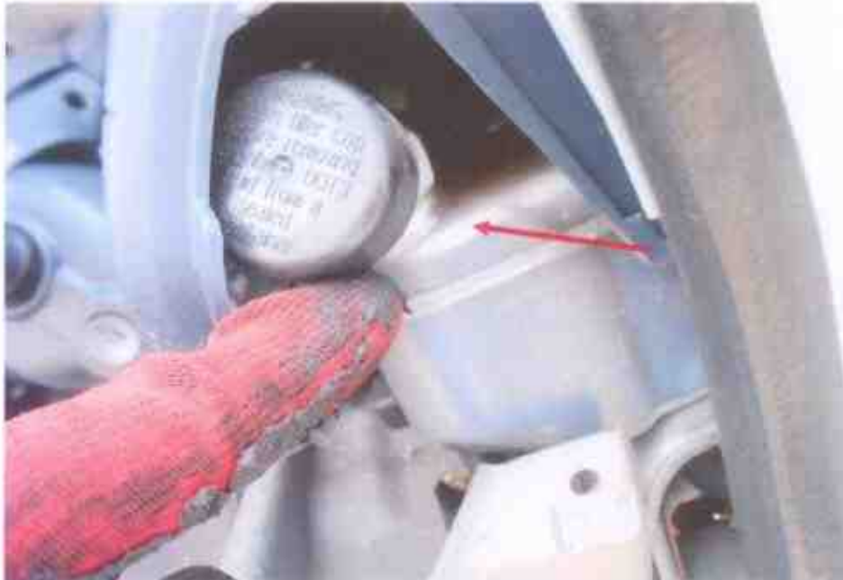
Photo 21 shows the brake fluid reservoir of the Motor Lorry. We had found the brake fluid to be of sufficient level for operational purposes. Visually there was also no contamination found to the brake fluid.
