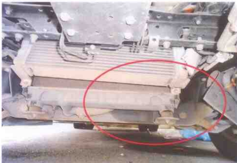
Photo 15 shows that there was also a fresh fluid stains covering the engine underside, indicating fluid leakage that had occurred due to the accident's impact.
