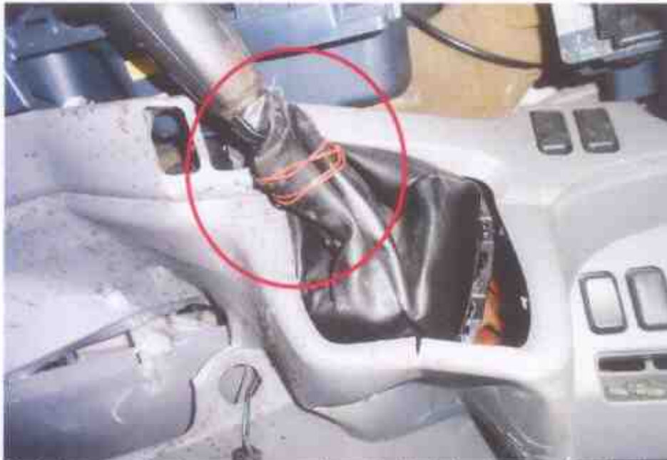
Photo 16 shows the transmission system which includes the gear knob (circled) of the Motor Lorry was observed to be bent due to the accident's collision.
