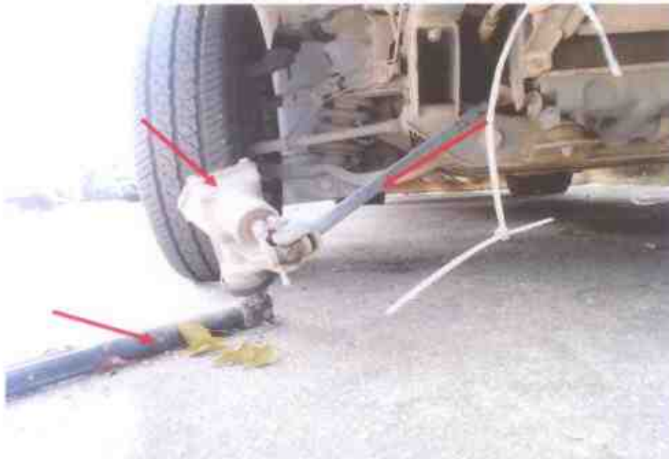
Photo 5 shows a closer view of the dislodged steering wheel rod of the Motor Lorry at the time of my inspection. It was likely due the result of the accident.
