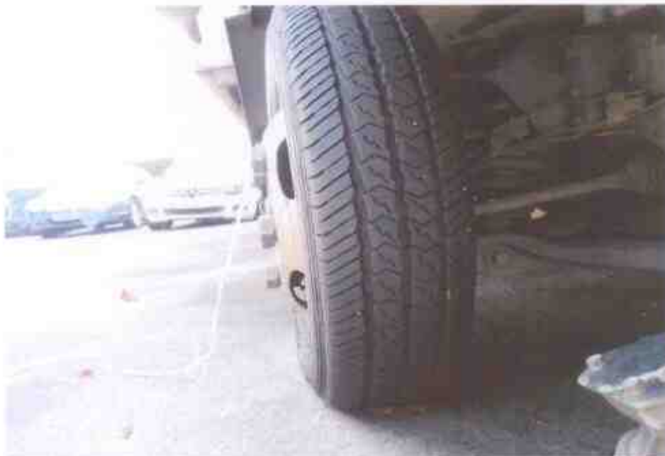
Photo 14 shows the condition of the front right tyre of the Motor Lorry. The front right tyre was observed to be in serviceable condition with remaining tread depth of approximately 7mm. There was also no tear, cut or burst mark(s) on the outer and the inner sidewalls as well as across the tread of this tyre. The tyre, which was wrapped around alloy wheel rim, was also observed to be sufficiently inflated for vehicular operation.
