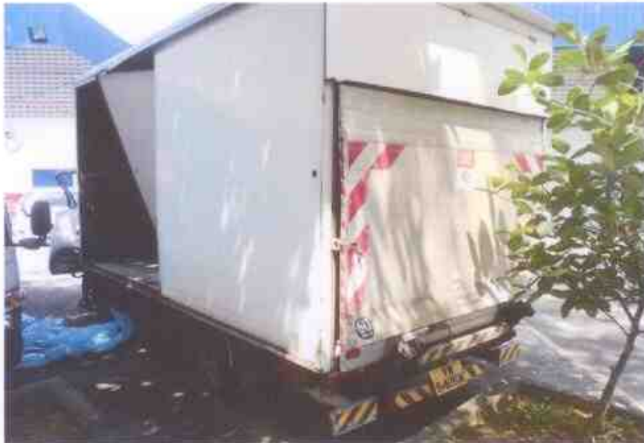
Photo 9 shows a general view of the rear left portion of the Motor Lorry at the time of my inspection. The rear portion was observed to be relatively unaffected by the accident.
