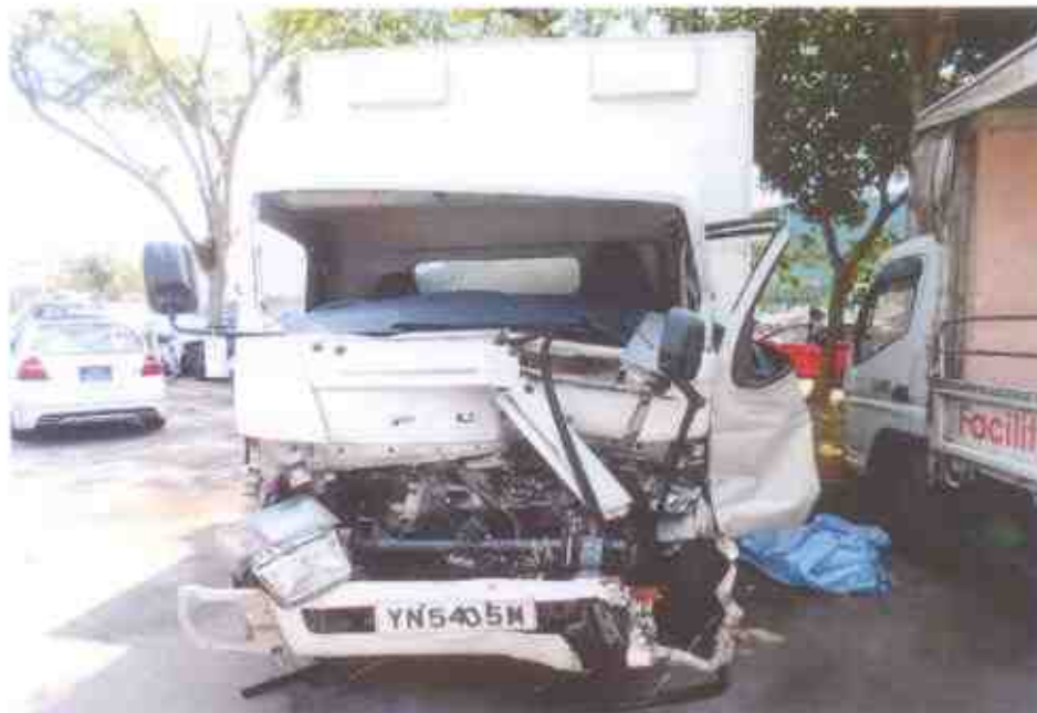
Photo 1 shows a general view of the frontal portion of the Motor Lorry at the time of my inspection. The Motor Lorry was observed to have sustained extensive impact damage at its frontal portion. The impact force was relatively significant, causing its entire front cabin to be buckled and crumpled.
