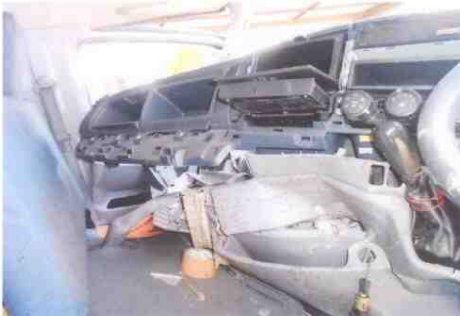
Photo 7 shows the interior of the front cabin. The dashboard, steering wheel, seats, floor panel and roof panel inside the front cabin were all observed to be pushed/buckled inwards, towards the rear of the Motor Lorry. This is consistent to the nature of this accident where the direction of impact onto the Motor Lorry was from a front to rear direction.
