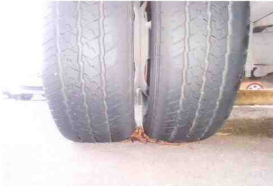
Photo 11 shows the condition of the rear right tyres of the Motor Lorry, which was observed to be in serviceable condition with remaining tread depth of approximately 8mm.
