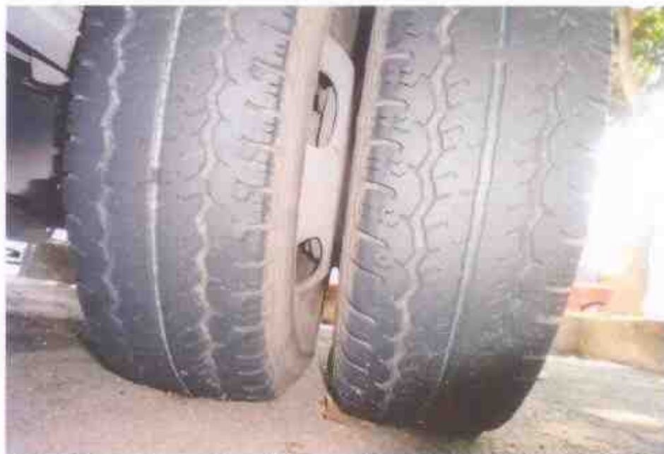
Photo 12 shows the condition of the rear left tyres of the Motor Lorry, which was observed to be in serviceable condition with remaining tread depth of approximately 8mm. There was no tear, cut or burst mark(s) on the outer and the inner sidewalls as well as across the tread of these 2 tyres, which were also observed to be sufficiently inflated for vehicular operation.
