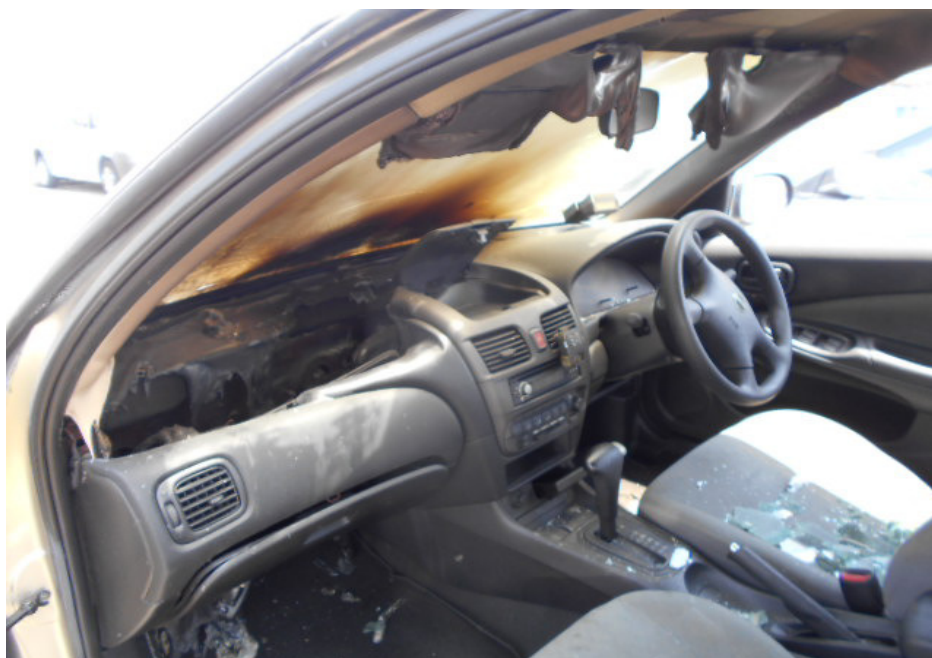
Photo 4 shows the interior compartment of the Insured Vehicle, which was observed to be partially burnt and/or melted at the front area. The front dashboard and roof upholstery were amongst the parts that were found to have been burnt and/or melted as a result of the fire.
