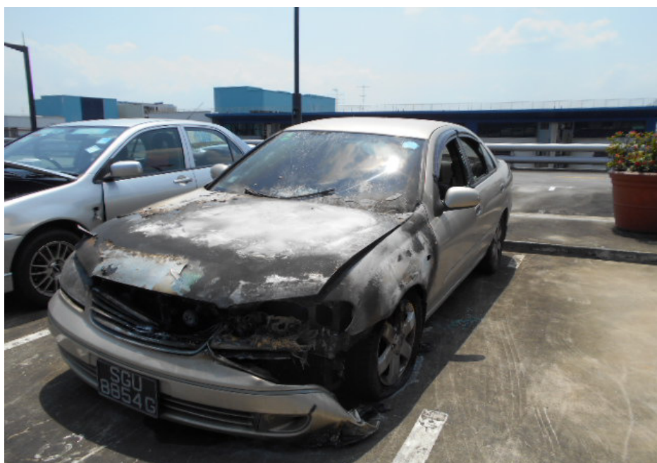
Photo 2 shows a general view of the front left portion of the Insured Vehicle at the time of my inspection. The fire damage to the Insured Vehicle was confined to its front portion. Its front bumper, front bonnet, front left headlamp, front windscreen and front left fender were amongst the body parts that were found to have been affected as a result of the fire.
