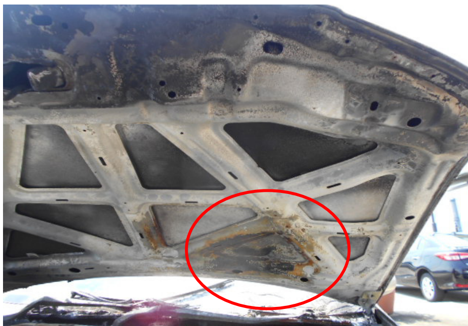
Photo 8 shows the whitish burn marks on the underside of the front bonnet, directly under the area where similar whitish burn marks were found. These whitish burn marks are a result of exposure to prolong heat intensity. Rust (circled) would normally start to develop around these areas soon after a fire as prolonged exposure to high heat intensity causes steel/metal material body parts to be exposed to natural environmental condition.
