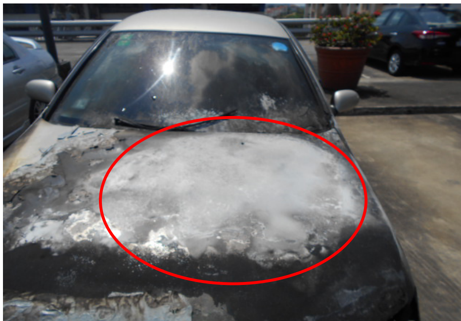
Photo 7 shows the whitish burn marks (circled) that were found on the rear left area of the Insured Vehicle's front bonnet. Such whitish burn marks are a result of exposure to prolong heat intensity. Following the characteristic of heat rising upwards, the fire to the Insured Vehicle can then be determined to have originated around the rear left area of the engine compartment.
