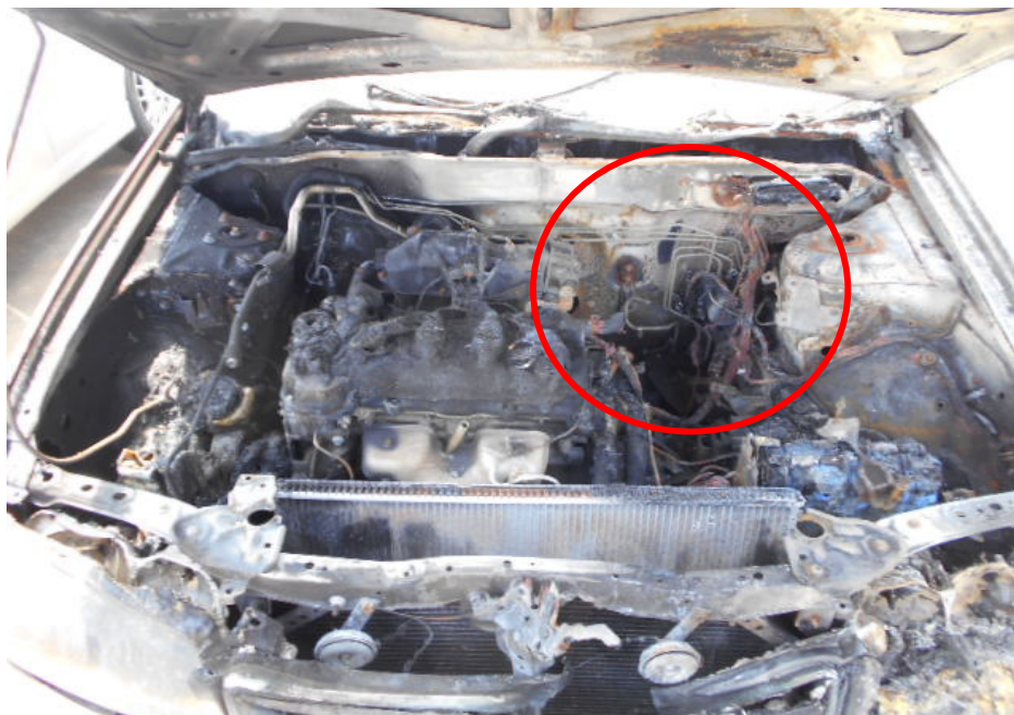
Photo 9 shows a general view of where the fire to the Insured Vehicle had originated, which was around the rear left area of the engine compartment (circled). This was established basing on the burn pattern (whitish burn marks and rust) that was found on the Insured Vehicle's front bonnet.
