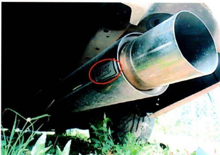
Photo 17 shows a close up left side view of the non-standard rear exhaust muffler that was found to be fitted on the Insured Vehicle at the time of our inspection. The brand of the rear exhaust muffler was 'DRIFT RACING' (circled).
