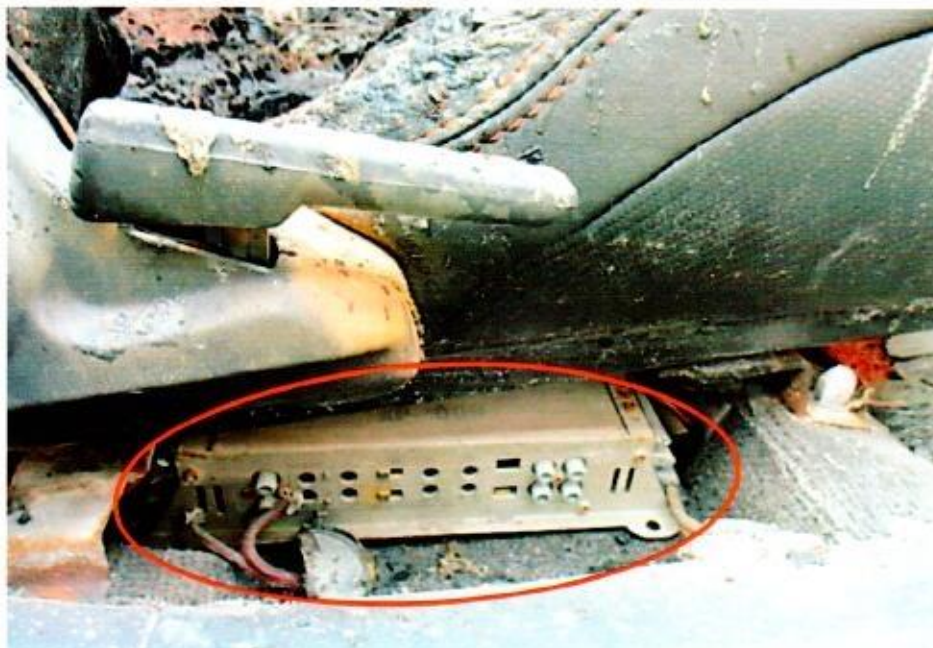
Photo 10 shows the 2nd aftermarket amplifier fitted underneath the driver seat of the Insured Vehicle upon our inspection (circled).
