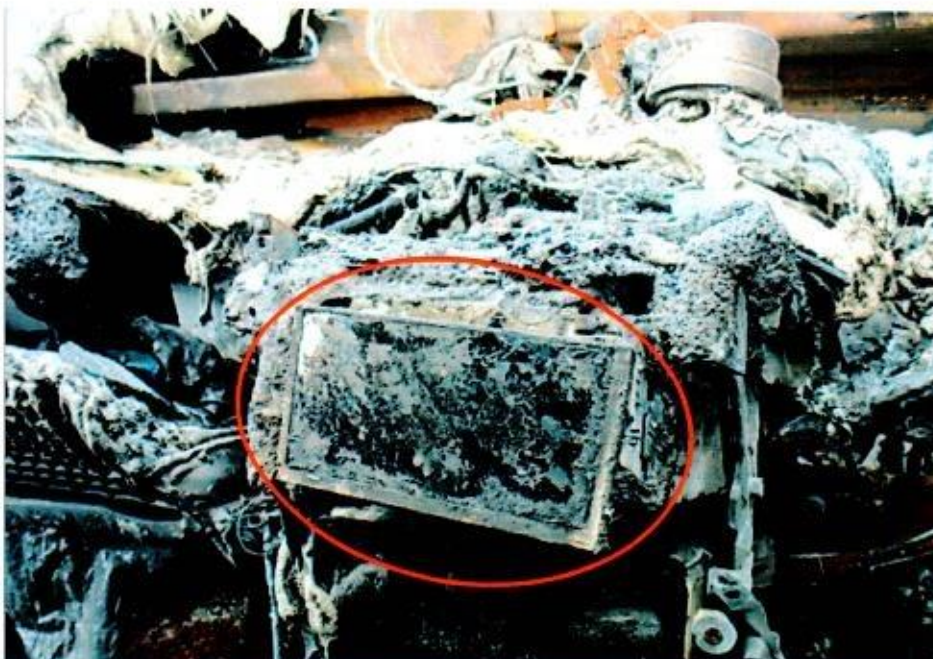
Photo 13 shows the in-car DVD player that was fitted at the centre portion of the front dashboard of the Insured Vehicle which had sustained extensive fire damage (circled).
