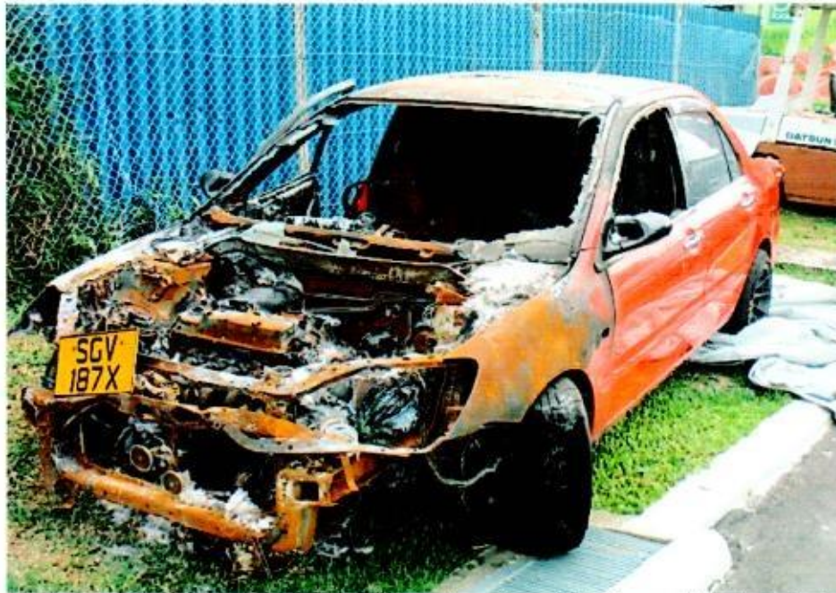
Photo 3 shows the general view of the left portion of the Insured Vehicle at the time of our inspection. The exterior body of the Insured Vehicle had sustained visible fire damage. This included its windscreen, front bonnet, headlights, front bumper, front bumper reinforcement panel, left side panel, left front rim and left front tyre.
