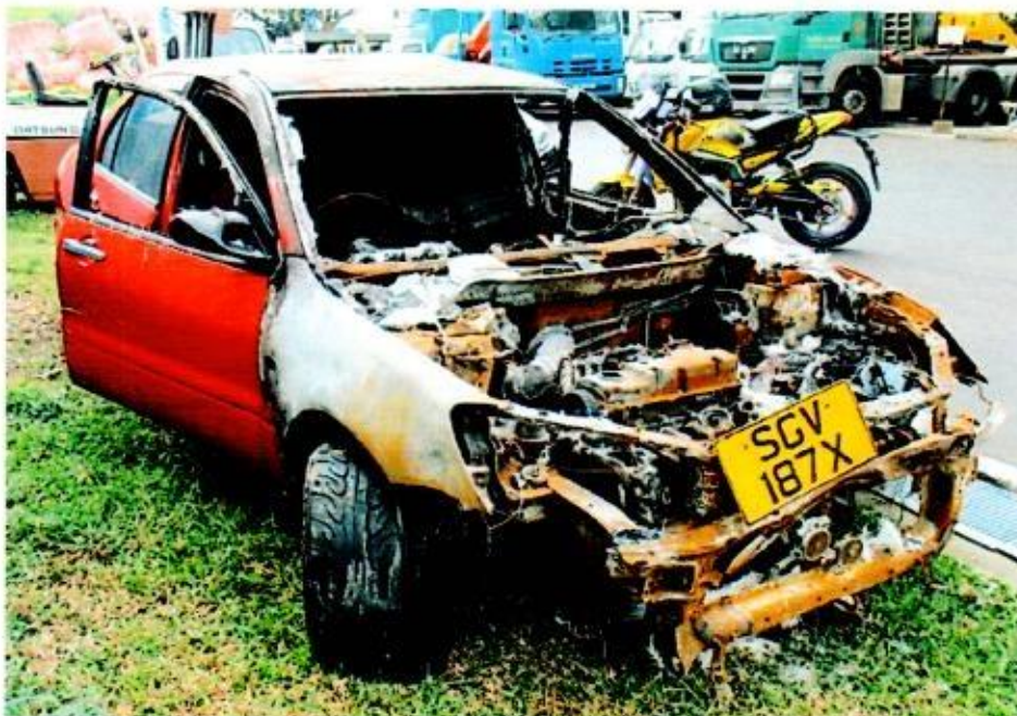
Photo 2 shows the general view of the right portion of the Insured Vehicle at the time of our inspection. The exterior body of the Insured Vehicle had sustained visible fire damage. This included its windscreen, front bonnet, headlights, front bumper, front bumper reinforcement panel, right side panel, right front rim and right front tyre.
