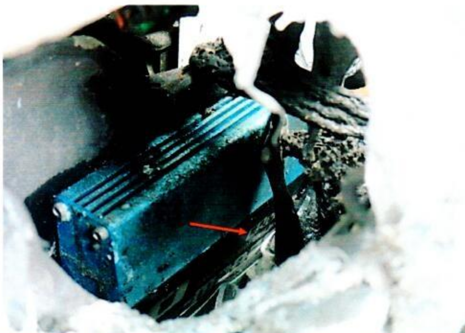
Photo 8 shows the fuel management system module that was fixed underneath the left portion of the front dashboard of the Insured Vehicle which had sustained serious fire damage. The brand of the module was 'GREDDY' (arrowed).
