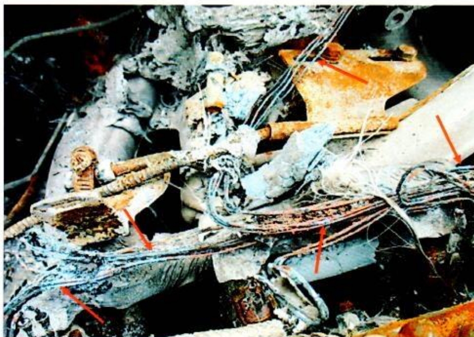
Photo 21 shows a close up view of the greenish residue on the wirings at the rear portion of the engine compartment. The presence of such greenish residue suggests occurrence of an electrical short circuit.
