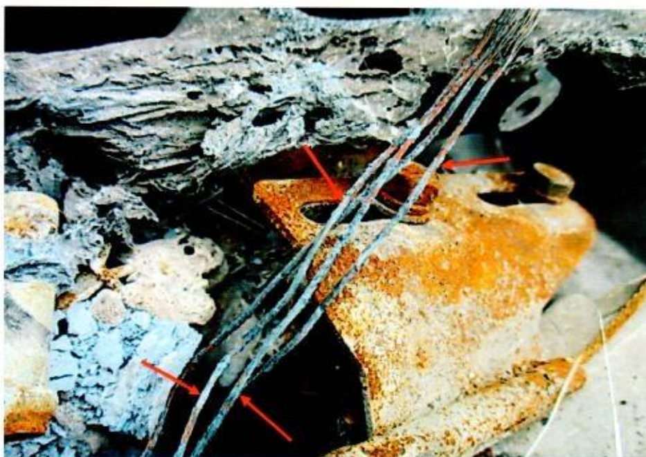
Photo 22 shows a close up view of the greenish residue on several burnt wirings at the rear portion of the engine compartment (arrowed). The presence of such greenish residue suggests occurrence of an electrical short circuit.
