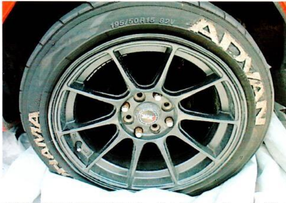
Photo 18 shows the non-standard rim found to be fitted on the Insured Vehicle at the time of our inspection. The 15- inch alloy rims fitted on the Insured Vehicle were not the standard type for the Insured Vehicle.
