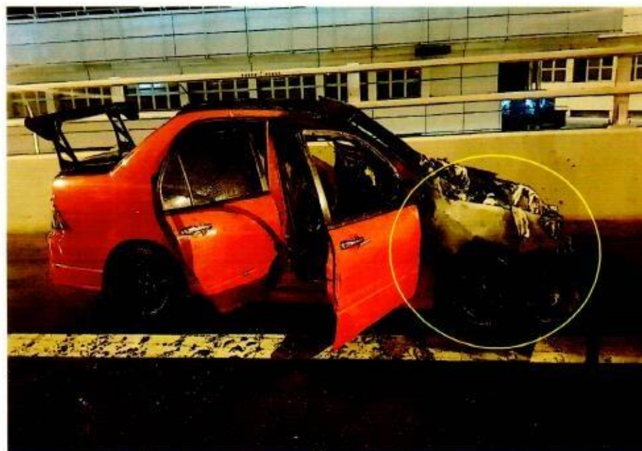
Photo 28 shows the right side view of the Insured Vehicle after the fire was extinguished. In general, the extensive damages sustained to the front portion had corresponded to the events that were related to us by Mr Nur, which is the fire started from the front bonnet (circled).
