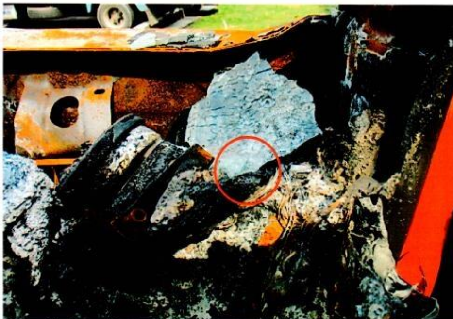
Photo 11 shows the 1st aftermarket twitter fitted onto the right corner of the dashboard of the Insured Vehicle upon our inspection which had sustained extensive fire damage (circled).
