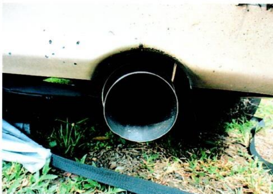
Photo 16 shows a front view of the non-standard rear exhaust muffler that was found to be fitted on the Insured Vehicle at the time of our inspection.
