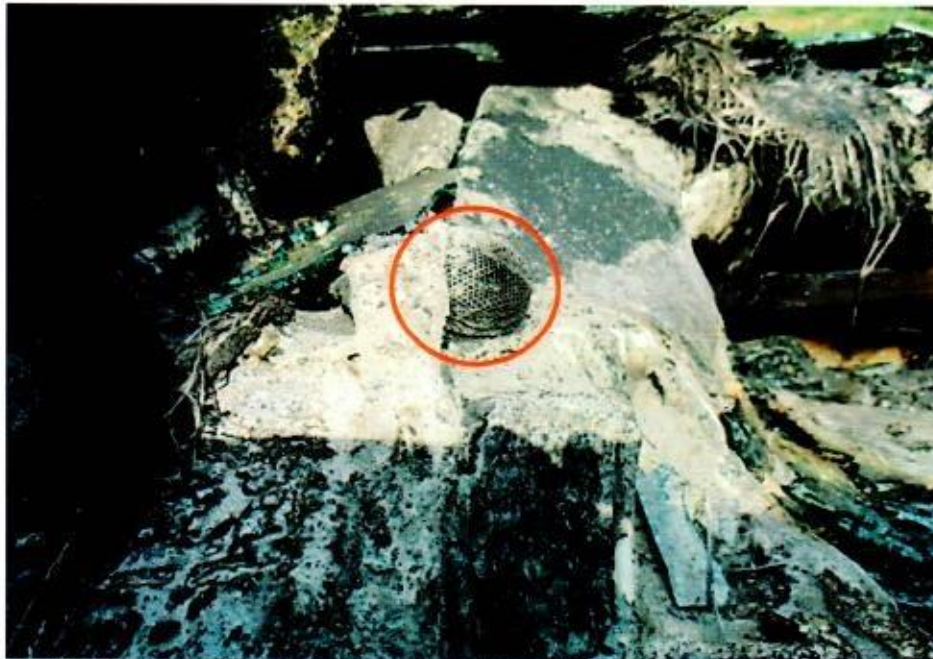
Photo 12 shows the 2nd aftermarket twitter fitted onto the left corner of the dashboard of the Insured Vehicle upon our inspection (circled) which had sustained serious fire damage.
