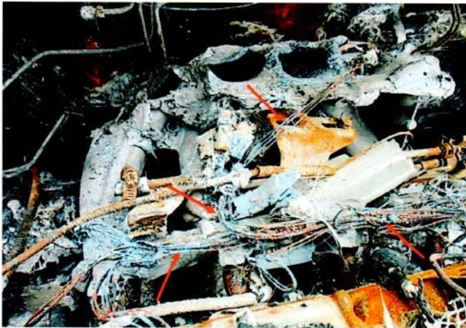
Photo 20 shows a closer view the greenish residue on several stretches of burnt wirings at the rear portion of the engine compartment (red arrows). The presence of greenish residue indicates internal heating of copper wires, a sign of an electrical short circuit occurring. The greenish residue is normally left behind from oxidation as a result of chemical reaction involving the copper wires.
