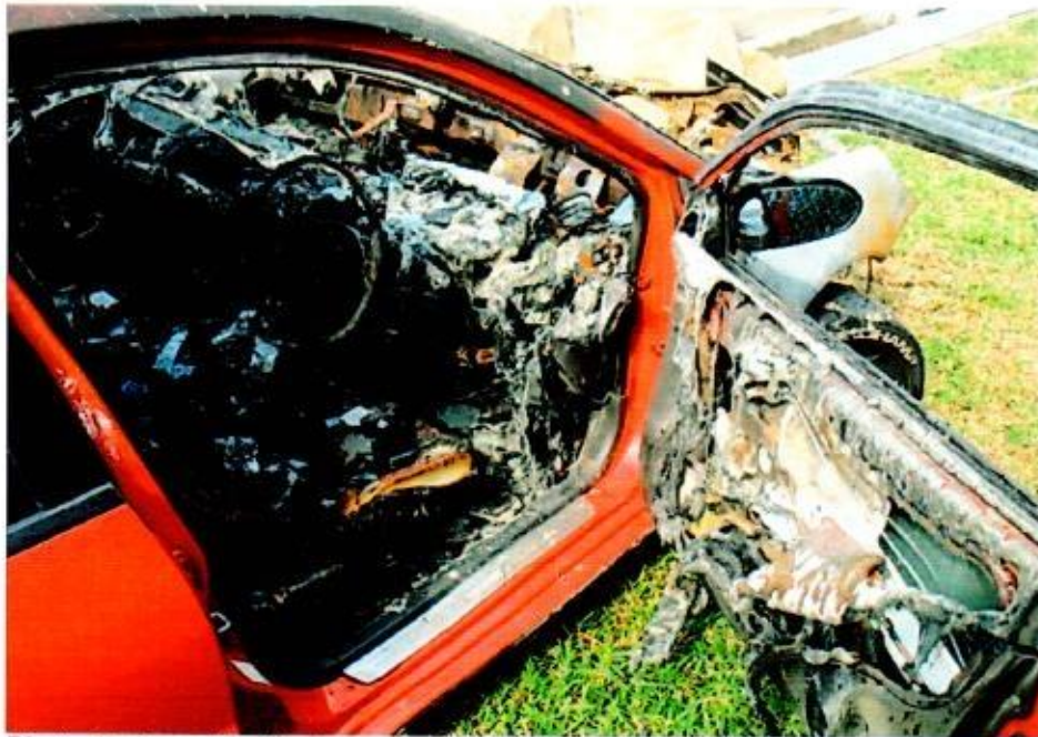
Photo 5 shows the interior compartment of the Insured Vehicle at the time of our inspection. The interior compartment of the Insured Vehicle was observed to be severely affected by the fire.
