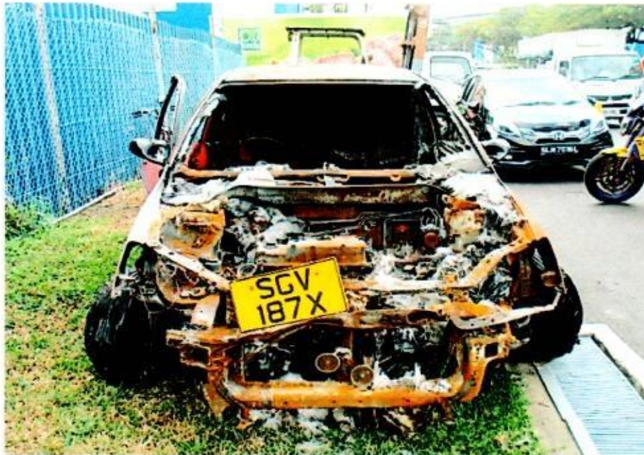
Photo 1 shows the general view of the front portion of the Insured Vehicle at the time of our inspection. The exterior body of the Insured Vehicle had sustained visible fire damage. This included its windscreen, front bonnet, headlights, front bumper, front bumper reinforcement panel, side panels, front rims and front tyres.
