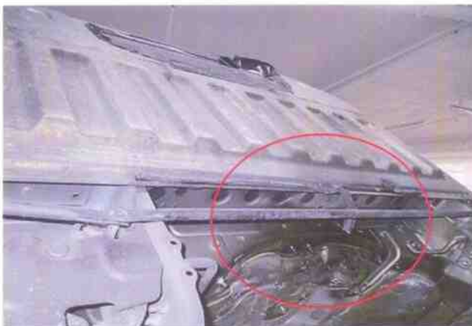
Photo 4 shows the exterior rear portion of the cab of the Insured Vehicle at the time of our inspection. The fire damage to the Insured Vehicle was confined to its centre portion (circled).
