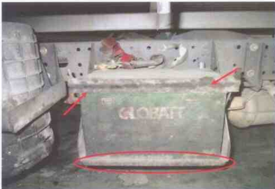
Photo 8 shows the high heat intensity burn marks (whitish burn marks) found on the metal brackets holding the battery of the Insured Vehicle (circled). Rust had also developed on these metal brackets (arrowed). The nature of fire damage is an indication as to where the fire started.
