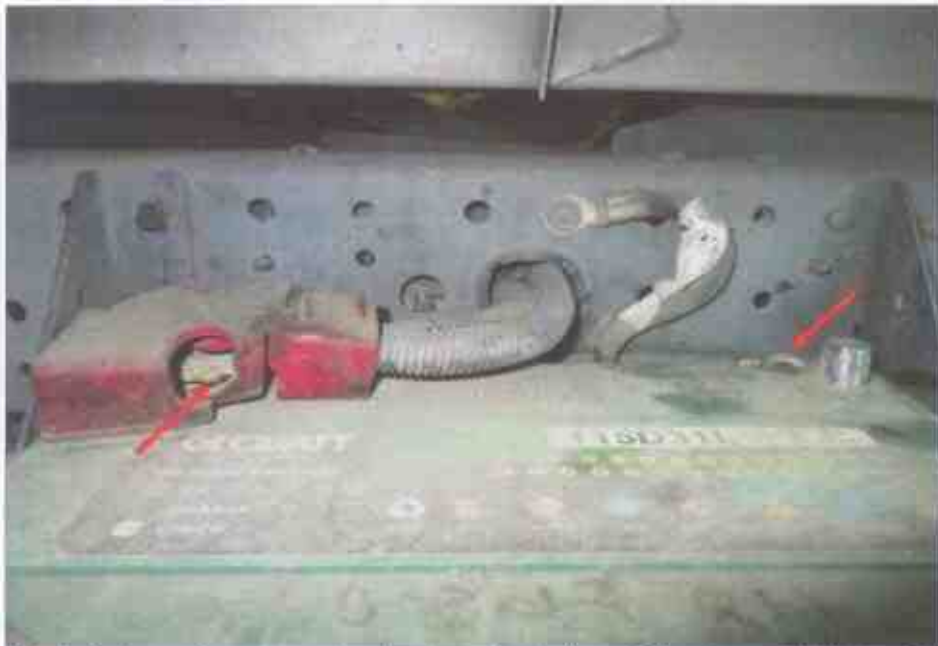
Photo 9 shows the wirings leading from the battery of the Insured Vehicle. The wirings were original factory fitted wirings. We observed traces of greenish residue on these wirings (arrowed). The presence of such greenish residue indicates internal heating of copper wires, a sign of an electrical short circuit occurring. The greenish residue is normally left behind from oxidation as a result of chemical reaction involving the copper wires. This physical evidence would then appear to suggest that the cause of fire to the Insured Vehicle could have possibly been due to electrical in nature.
