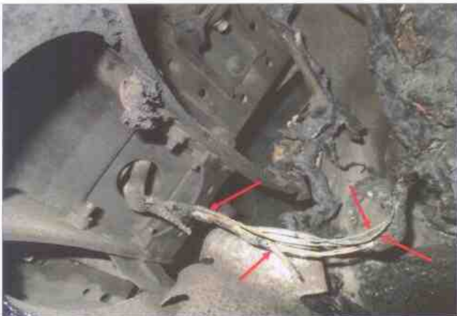
Photo 13 shows a close up view of the greenish residue found on some of the burnt wirings of the Insured Vehicle's air cleaner assembly (arrowed). This seems to suggest the occurrence of an electrical short circuit.
