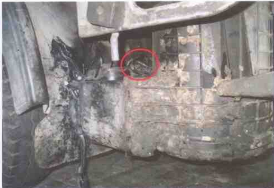
Photo 11 shows the burnt wirings of the Insured Vehicle's air cleaner assembly. We observed traces of greenish residue on some of these wirings (circled).
