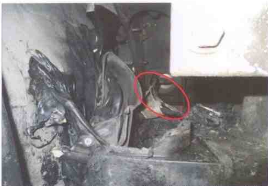
Photo 12 shows a closer view of the greenish residue found on the burnt wirings of the Insured Vehicle's air cleaner assembly (circled). This seems to suggest the occurrence of an electrical short circuit.
