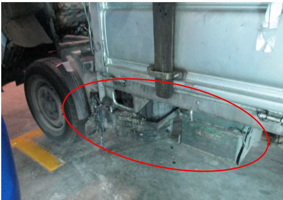
Photo 6 shows the left centre portion of the Insured Vehicle, where the air cleaner assembly and battery are located. The nature of fire damage was confined to these particular areas (circled).
