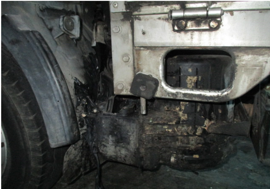
Photo 7 shows a closer view of the air cleaner assembly. The various components of the air cleaner assembly were observed to have been partly melted from the high heat intensity.
