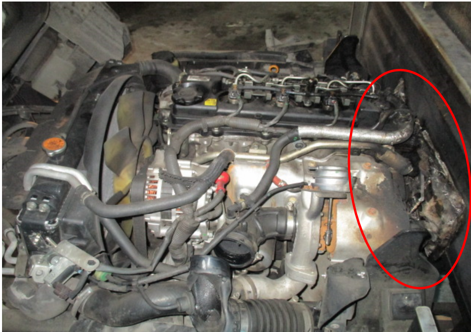
Photo 5 shows the engine compartment of the Insured Vehicle which is situated beneath the cab at the time of our inspection. The rear portion of the engine compartment of the Insured Vehicle was significantly unaffected by the fire (circled).
