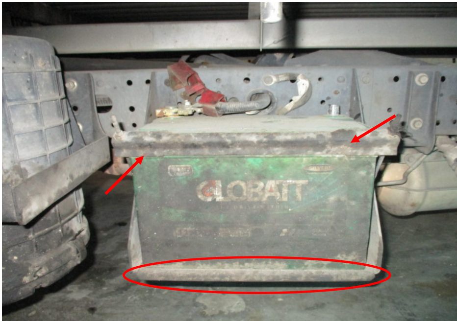
Photo 8 shows the high heat intensity burn marks (whitish burn marks) found on the metal brackets holding the battery of the Insured Vehicle (circled). Rust had also developed on these metal brackets (arrowed). The nature of fire damage is an indication as to where the fire started.
