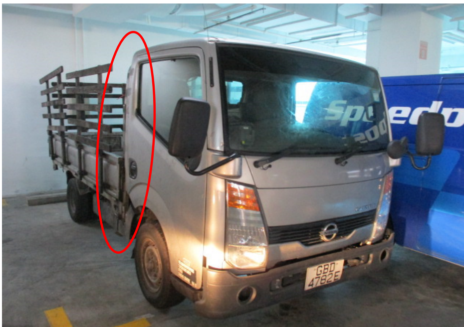
Photo 2 shows the right side view of the Insured Vehicle at the time of our inspection. The exterior body of the Insured Vehicle was relatively unaffected by the fire except for the centre portion. The fire damage to the Insured Vehicle was confined to its centre portion (circled).
