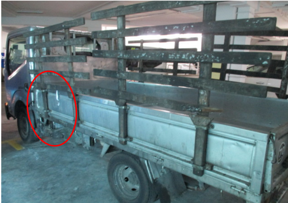
Photo 3 shows the left rear view of the Insured Vehicle at the time of our inspection. The exterior body of the Insured Vehicle was relatively unaffected by the fire except for the centre portion. The fire damage to the Insured Vehicle was confined to its centre portion. The fire damage was observed to be most severe at its left centre portion (circled).
