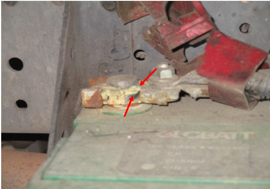
Photo 10 shows a closer view of the greenish residue found on the wirings leading from the battery of the Insured Vehicle (arrowed). This seems to suggest the occurrence of an electrical short circuit.
