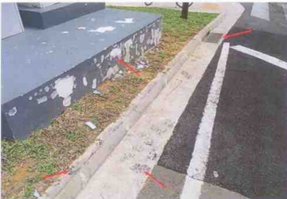
Photo 13 shows the burn marks and/or burnt residual remains on the ground, kerb, electrical fixtures and drain grating nearest to where the Insured Vehicle was positioned when the fire occurred (arrowed).
