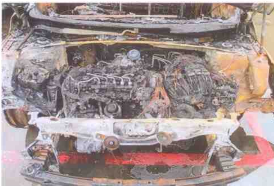
Photo 5 shows the engine compartment of the Insured Vehicle at the time of our inspection. The entire engine compartment of the Insured Vehicle was observed to be severely burnt. Most of the parts inside the engine compartment were found to be burnt and/or melted as a result of the fire.
