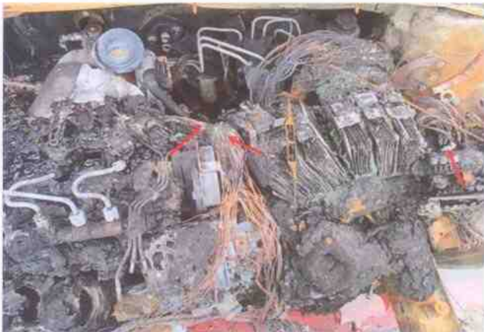
Photo 8 shows a closer view of the greenish residue found on some of the burnt stretches of original factory fitted wirings (arrowed). The presence of such greenish residue suggests occurrence of an electrical short circuit.
