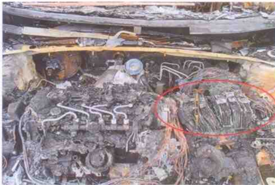
Photo 7 shows the original factory fitted wirings around the rear left portion of the engine compartment, which is in the immediate vicinity where the fire to the Insured Vehicle had likely started. We had found greenish residue on several burnt stretches of these wirings (circled). The presence of such greenish residue indicates internal heating of copper wires, a sign of an electrical short circuit occurring. The greenish residue is normally left behind from oxidation as a result of chemical reaction involving the copper wires.
