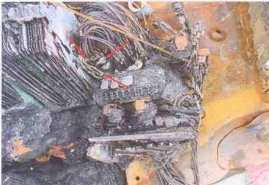
Photo 10 shows a close up view of the greenish residue found on some of the burnt stretches of original factory fitted wirings (arrowed). The presence of such greenish residue suggests occurrence of an electrical short circuit.
