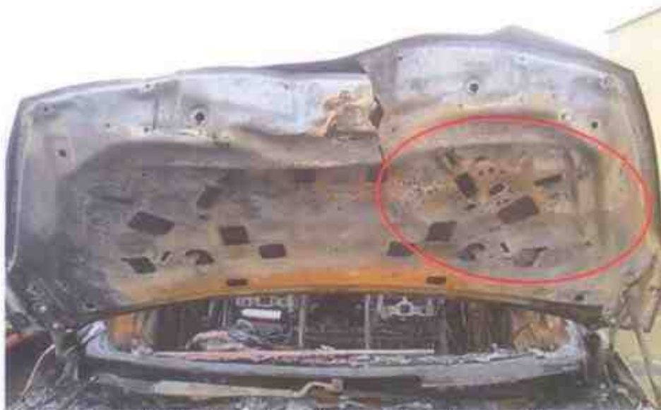
Photo 6 shows the rust that had developed on the underside of the front bonnet, around the bottom left portion (circled). The development of rust is an indication that this area was subjected to prolonged exposure to high heat intensity, which had caused the steel/metal material of the front bonnet to be exposed to natural environmental condition. Hence the fire to the Insured Vehicle can be determined to have originated towards the rear left portion of the engine compartment.
