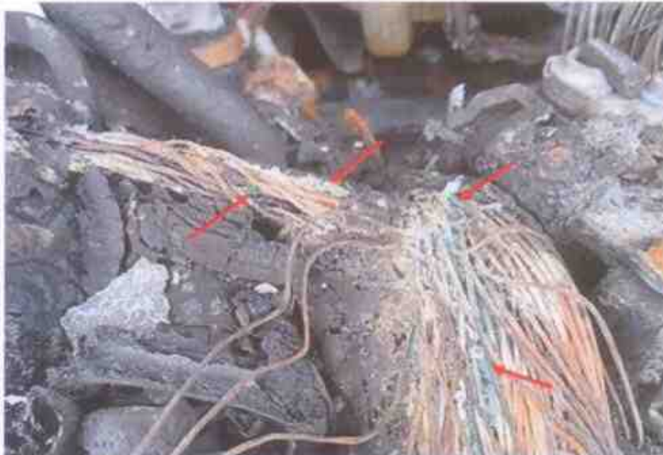
Photo 9 shows a close up view of the greenish residue found on some of the burnt stretches of original factory fitted wirings (arrowed). The presence of such greenish residue suggests occurrence of an electrical short circuit.
