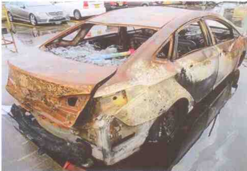
Photo 3 shows the general view of the rear right body of the Insured Vehicle at the time of our inspection. The Insured Vehicle was observed to have sustained extensive fire damage all around. Rust had accumulated all over the Insured Vehicle as a result of exposure to environmental condition for a period of time.
