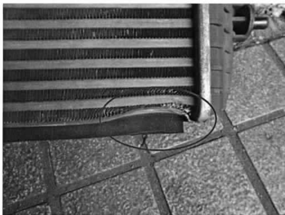
7. Intercooler. Photo 115 to 117 in Merimen. Bent (circled) below photo.
