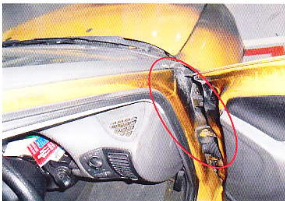
Photo 2 shows the semi close-up view of the front right door of the Insured Vehicle at the time of our inspection. The fire damage to the Insured Vehicle was observed to be affecting the driver side door internally.
