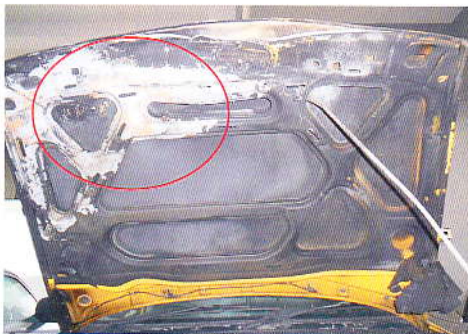
Photo 7 shows the discolouration of the insulating material on the underside of the front bonnet, around the front right side area (circled). The discolouration of the insulating material is an indication that the front right side area of the engine compartment had sustained exposure to prolonged high heat intensity. Hence the fire to the Insured Vehicle can be determined to have originated towards the front right side of the engine compartment.
