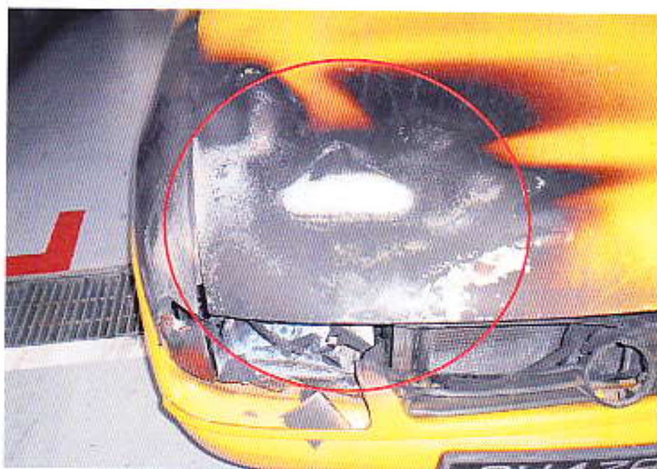
Photo 5 shows the burn pattern and whitish burn marks (circled) that were found on the rear left side of the front bonnet of the Insured Vehicle. Such whitish burn marks are a result of exposure to prolonged heat intensity, which may indicate where the fire had started. Rust would also begin to develop on these areas soon after the fire.
