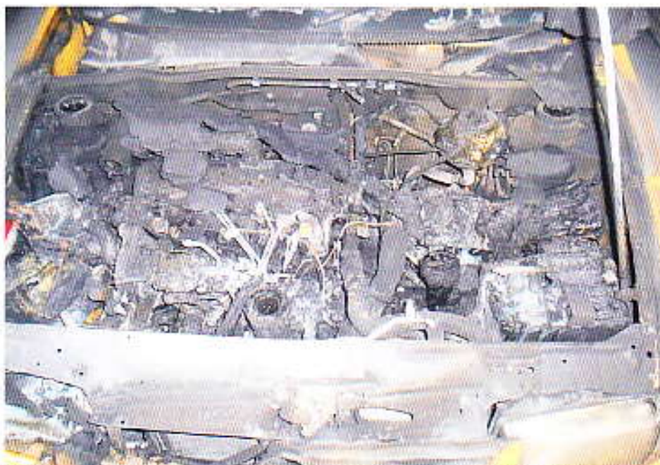
Photo 3 shows the engine compartment of the Insured Vehicle at the time of our inspection. The entire engine compartment of the Insured Vehicle was observed to be burnt and/or melted as a result of the fire.
