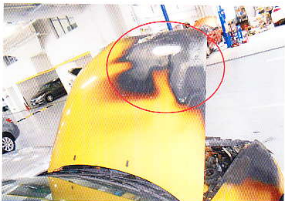
Photo 6 shows a close-up view of the burn pattern and whitish burn marks (circled) that were found on the front right side of the front bonnet of the Insured Vehicle. Such whitish burn marks are a result of exposure to prolonged heat intensity, which may indicate where the fire had started. Rust would also begin to develop on these areas soon after the fire.
