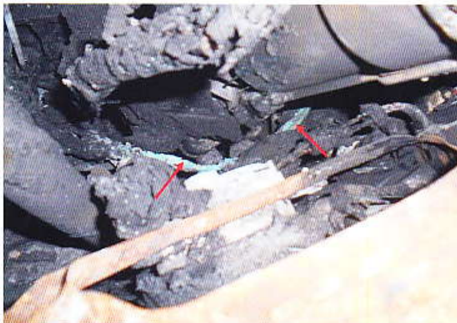
Photo 11 shows a closer view of the burnt wirings (red arrows) at the rear left side of the engine compartment. Such condition normally indicates internal heating of copper wires which is a sign of an electrical short circuit occurring.
