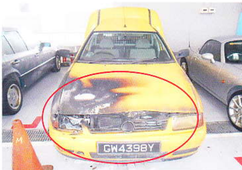
Photo 1 shows the general view of the front portion of the Insured Vehicle at the time of our inspection. The fire damage to the Insured Vehicle was confined to its front bonnet, headlamp, front bumper & grill & left & right side fenders were amongst the body parts that were found to have been affected as a result of the fire.
