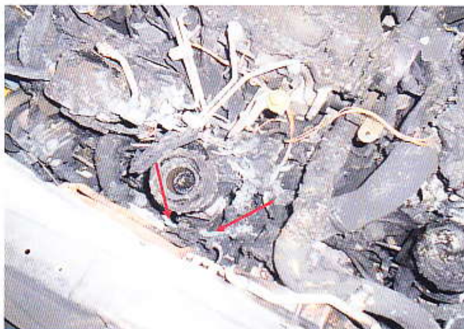
Photo 12 shows a close up view of the burnt wirings (red arrows) at the rear left side of the engine compartment. Such condition normally indicates internal heating of copper wires which is a sign of an electrical short circuit occurring
