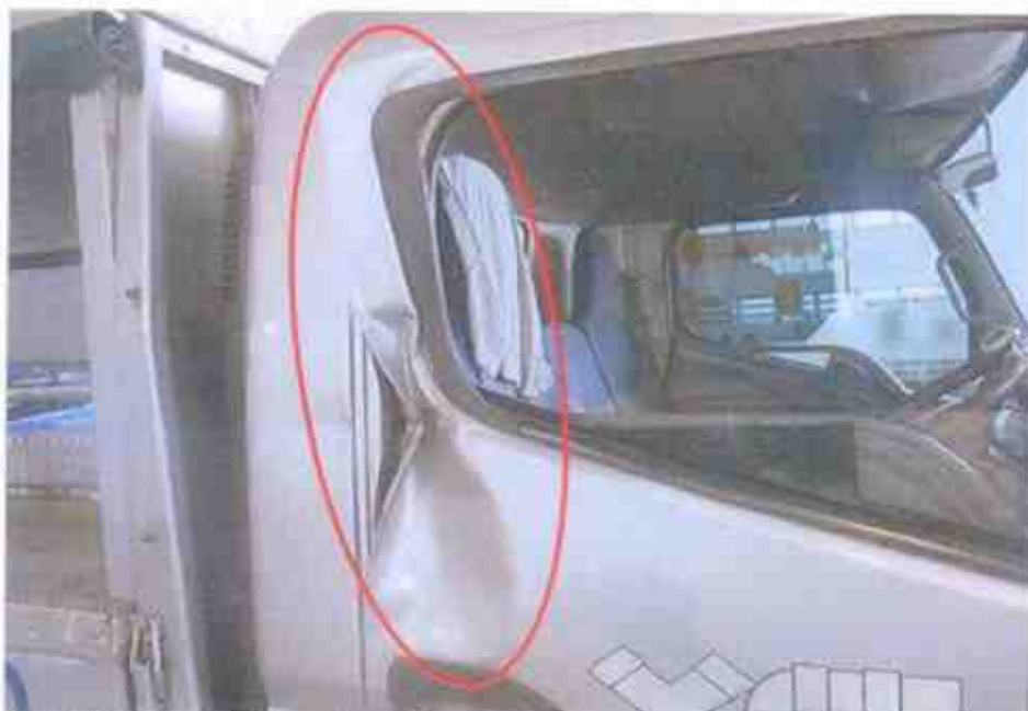
Photo 3 shows a closer view of the dislodgement and buckling of the driver door and a slight dent on the right front portion (circled).
