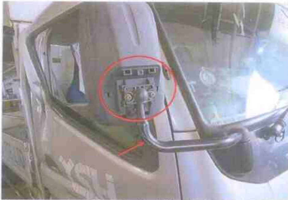
Photo 4 shows a close up view of the Mitsubishi's right side mirror. The right side mirror cover was missing (circled) and graze marks were found on the front portion of the right side mirror (arrowed).
