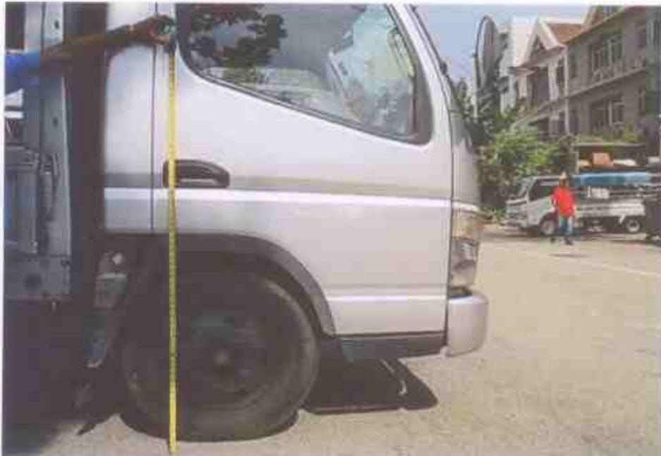
Photo 16 shows the height measurement being conducted on the right front portion of the Mitsubishi.
