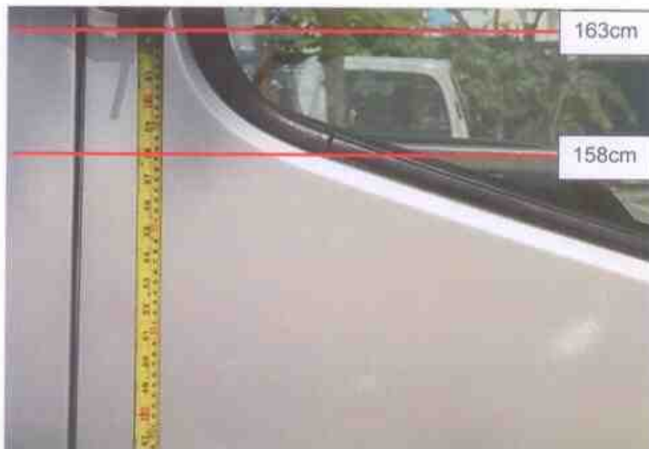
Photo 17 shows a closer view of the height measurement being conducted on the right front portion of the Mitsubishi. The height range above ground level of the driver door at the area where the driver door was buckled was measured to be approximately between 158cm to 163cm.
