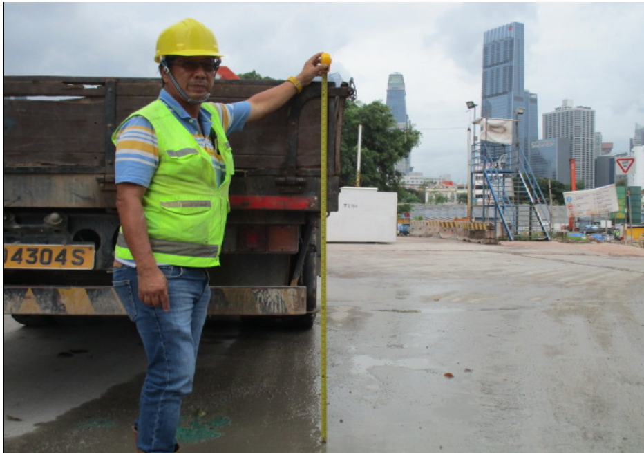
Photo 18 shows the height measurement being conducted on the rear right portion of the Hino.
