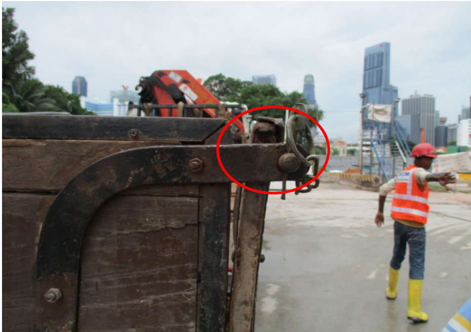
Photo 9 shows upon closer examination, we observed faint graze marks on the right tailgate lock (circled).
