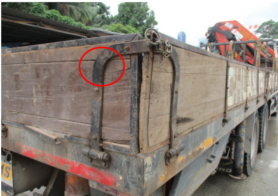
Photo 8 shows at the time of our inspection, we found the right side hinge of the Hino's tailgate to be buckled (circled).
