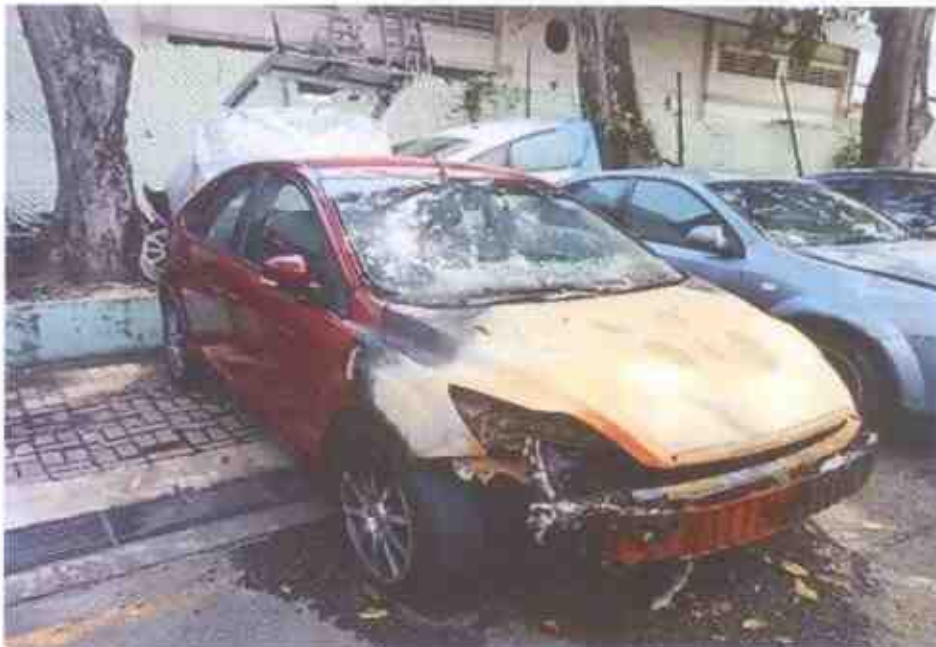
Photo 1 shows a general view of the front right body of the Insured Vehicle at the time of inspection. The Insured Vehicle was observed to have sustained severe fire damage at its frontal body. Its front bumper, front bonnet, front grille, front right headlamp and front right fender were amongst the body parts that were found to have been burnt as a result of the fire.
