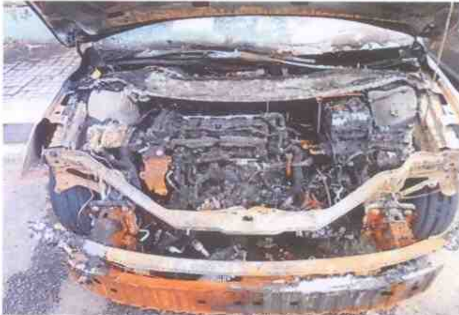
Photo 3 shows the engine compartment of the Insured Vehicle at the time of inspection. Almost all the parts inside the engine compartment were observed to be burnt and/or melted as a result of the fire. These parts had included its radiator, air condenser, cooling fan, intake manifold, fuse box, battery, air duct, hoses and pipes amongst others.
