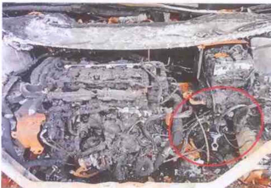
Photo 8 shows a general view of the Insured Vehicle's engine compartment. Faint greenish residue was observed along the wirings at the centre left area (circled) of the engine compartment. The presence of such greenish residue indicates internal heating of copper wires, which is a sign of an electrical short circuit occurring.
