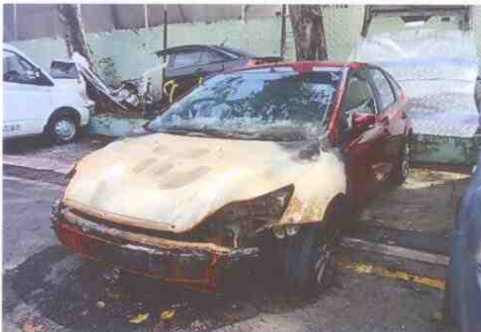
Photo 2 shows a general view of the front left body of the Insured Vehicle at the time of inspection. The Insured Vehicle was observed to have extensive sustained fire damage at its frontal body. Its front bumper, front left fender, front left headlamp, front bonnet and front windscreen were amongst the body parts that were found to have been burnt as a result of the fire.
