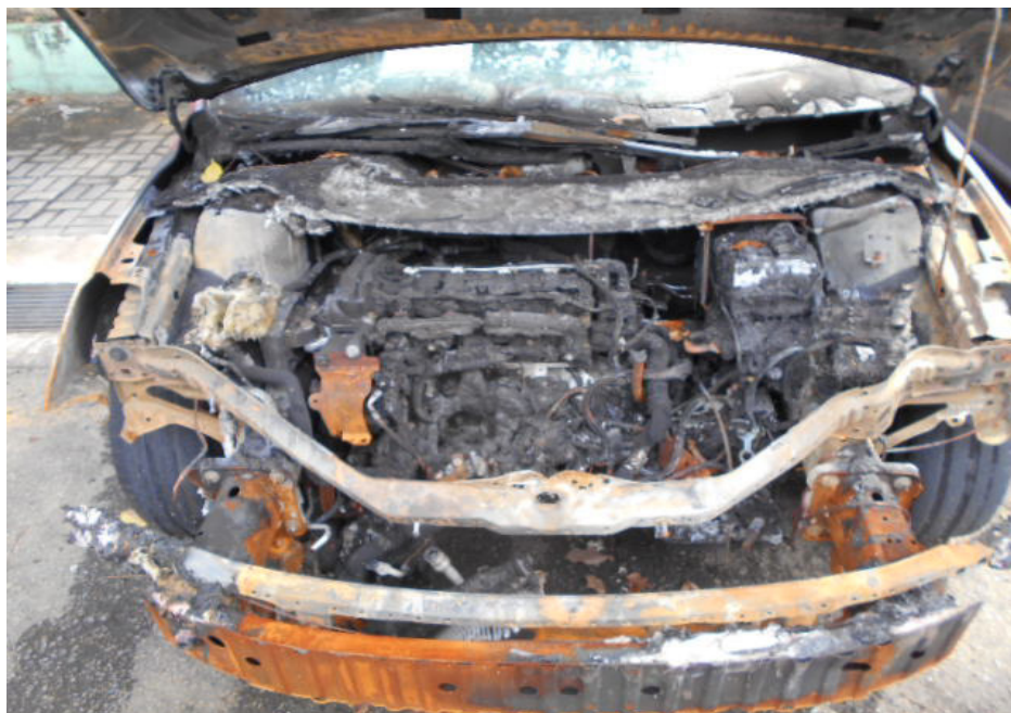
Photo 3 shows the engine compartment of the Insured Vehicle at the time of inspection. Almost all the parts inside the engine compartment were observed to be burnt and/or melted as a result of the fire. These parts had included its radiator, air condenser, cooling fan, intake manifold, fuse box, battery, air duct, hoses and pipes amongst others.
