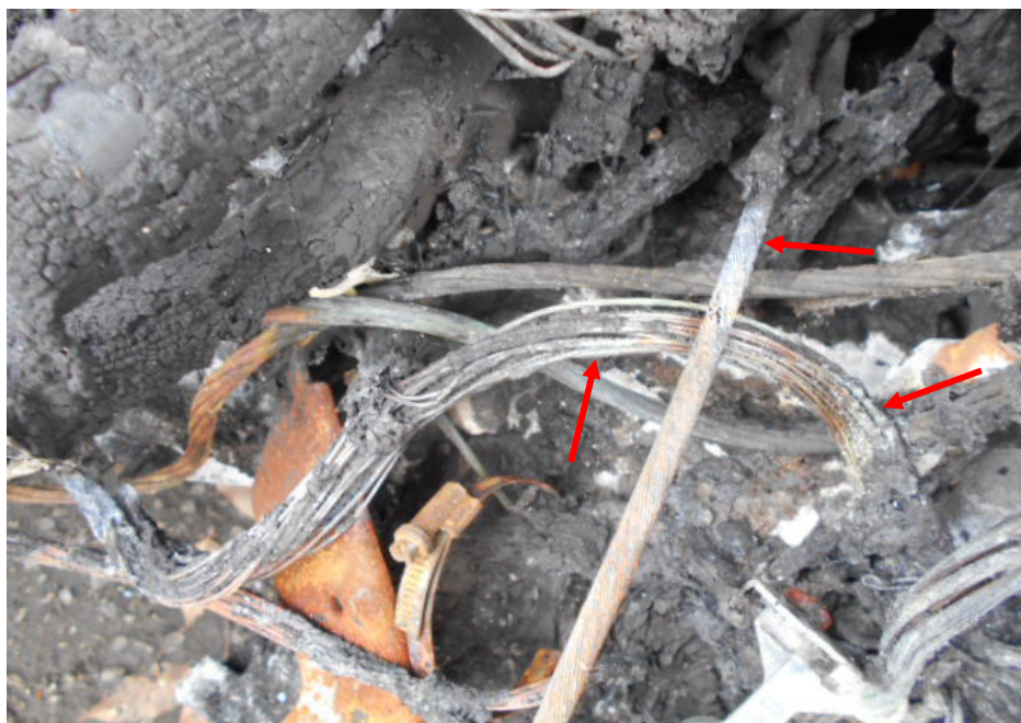
Photo 9 shows a closer view of the wirings (arrowed) at the centre left area of the Insured Vehicle's engine compartment, where faint greenish residue was found. These wirings were original factory fitted wirings.
