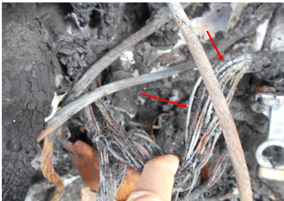
Photo 10 shows a closer view of the wirings (arrowed) at the centre left area of the Insured Vehicle's engine compartment, where faint greenish residue was found. These wirings were original factory fitted wirings. The presence of such greenish residue indicates internal heating of copper wires, which would suggest that the cause of fire to the Insured Vehicle was due to electrical in nature.
