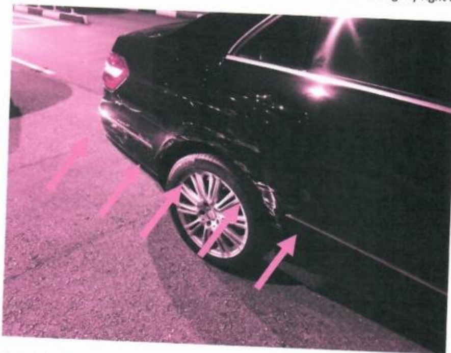
Photo showing damage to right rear extending from rear bumper to rear passenger door on the right side including the right rear tire
