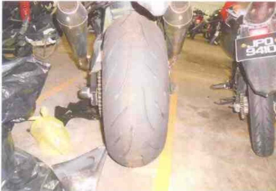
Photo 7 shows the rear tyre of the Motorcycle. The rear tyre was observed to be in serviceable condition with remaining tread depth of approximately 3mm. The tyre was also observed to be sufficiently inflated for vehicular operation.
