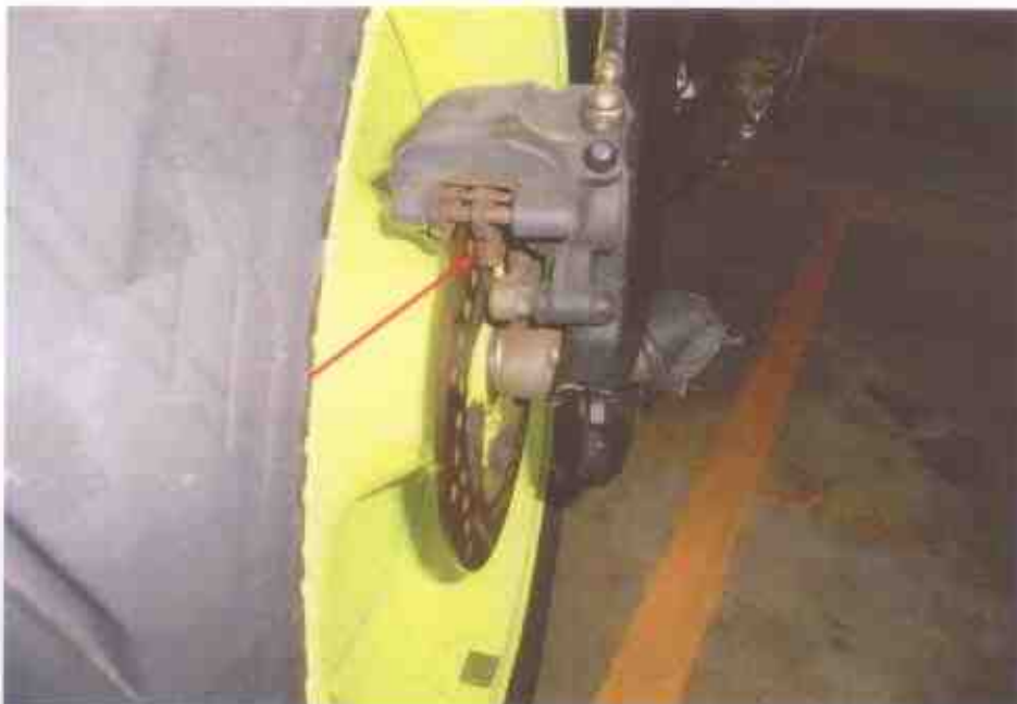
Photo 19 shows the brake pad for the rear brake observed to be in serviceable condition at time of our inspection. The frictional material found to be sufficient for operational purposes.
