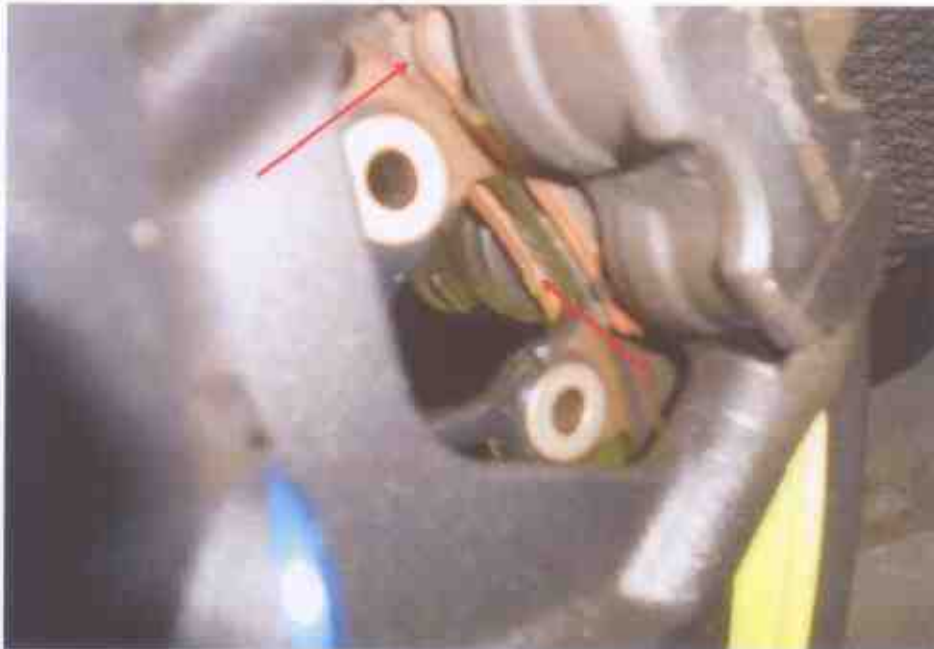
Photo 18 shows the brake pad for the front brake, observed to be in serviceable condition at time of our inspection. The frictional material found to be sufficient for operational purposes.
