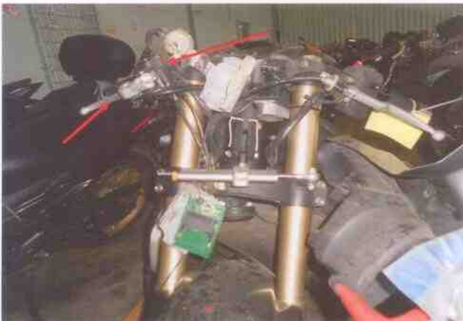
Photo 15 shows the steering system was observed to be damaged likely due to the accident's impact.
