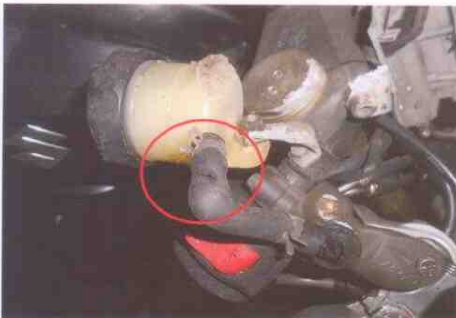
Photo 16 shows the fluid brake reservoir for the front brake that was observed to be broken due to the accident. Its brake hose was also found to be cut/damaged.
