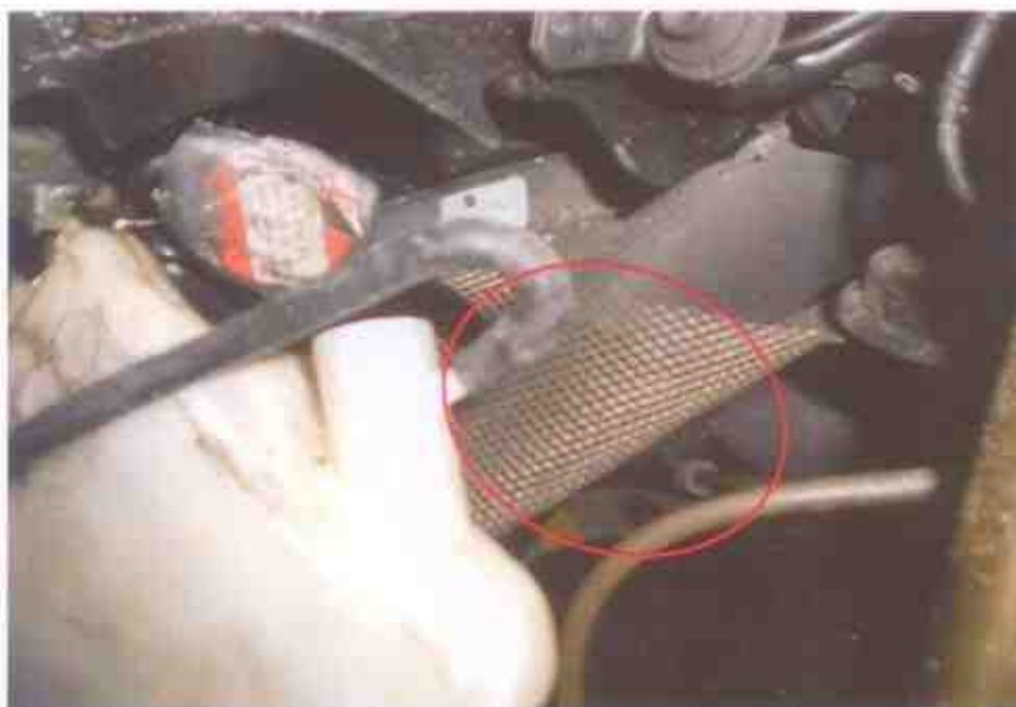
Photo 5 shows the damaged engine coolant reservoir & radiator as a result of the accident.(Circled)
