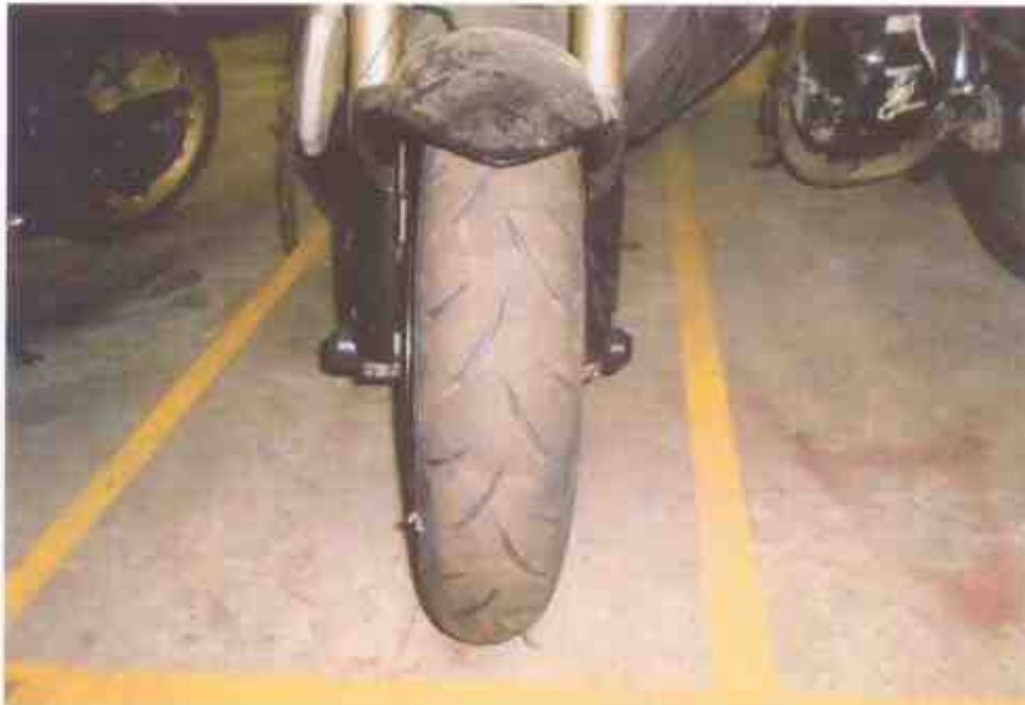
Photo 8 shows the front tyre of the Motorcycle. The pattern of the tread was clearly visible. There was no tear, burst mark(s) and/or punctured hole(s) on the sidewalls as well as across the tread of the front tyre. Except for it was observed to be deflated likely due to the accident's impact.
