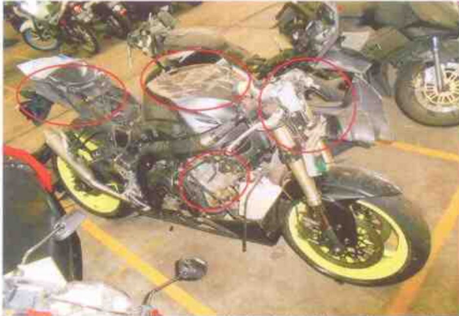
Photo 3 shows a general view of the right body of the Motorcycle at the time of our inspection. The Motorcycle was observed to have sustained extensive damages at the frontal, rear portion & along its right side. (Circled)
