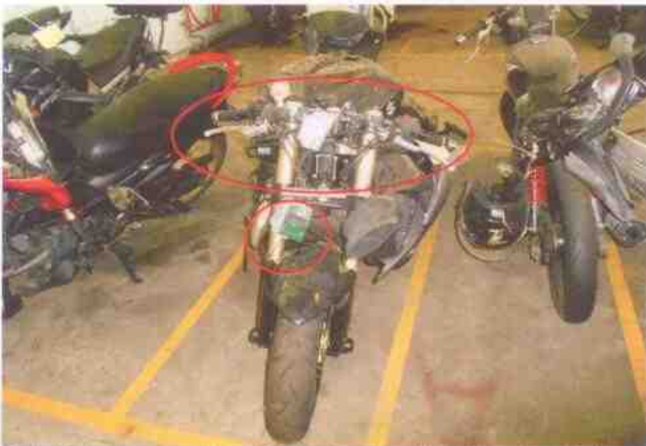
Photo 2 shows a general view of the front portion of the Motorcycle at the time of our inspection. The Motorcycle was observed to be sustained with damages due to the accident collision. (Circled)
