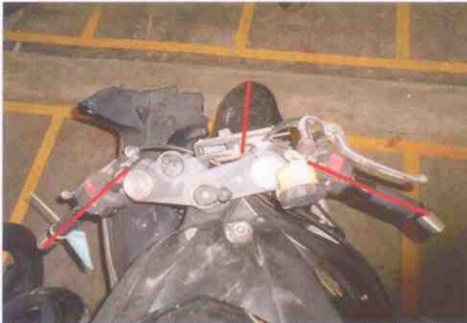
Photo 14 shows the handle bar was observed to be damaged by the accident's impact. It was observed to be misaligned likely due to the accident's impact.
