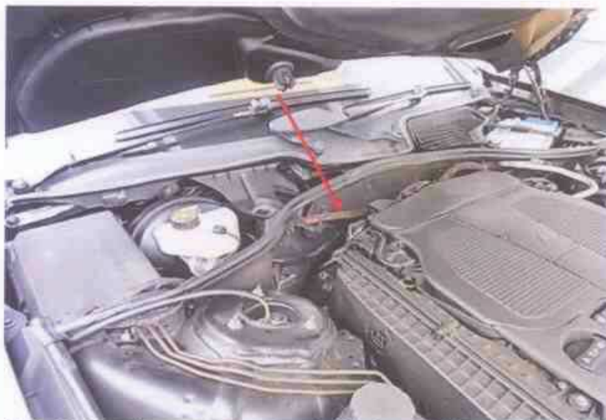
Photo 11 shows the engine compartment of the Insured Vehicle. The fire to the Insured Vehicle had originated within the engine compartment, at the centre rear area (arrowed) of the engine compartment. This was established given that there was only a single area on the Insured Vehicle where damage of burn nature was found.
