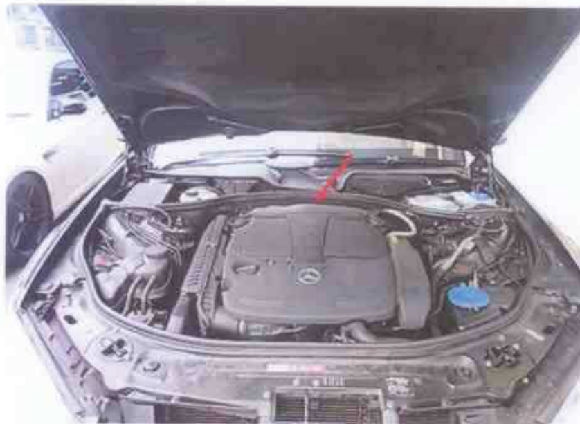
Photo 4 shows a general view of the engine compartment of the Insured Vehicle. Upon checking the engine compartment, I had found a stretch of wiring harness partially burnt/melted. This was towards the centre rear area (arrowed) of the engine compartment. The firewall insulator behind the stretch of partially burnt/melted wiring harness was also observed to be with minor burn marks.
