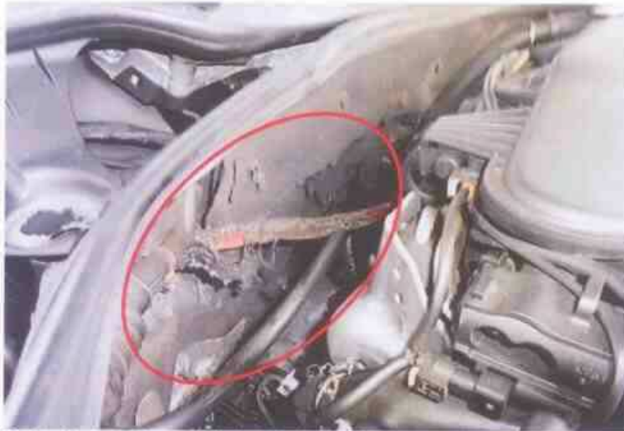
Photo 12 shows the partially burnt/melted wiring harness at the centre rear area of the engine compartment. The wiring harness was an original factory fitted wiring harness which connects the Engine Control Unit (ECU) to the fuse box of the Insured Vehicle. Heat generated during engine operation could have caused the rubber insulation of the wirings started to melt, exposing live wires that came into contact with each other, creating sparks that had ignited the fire.
