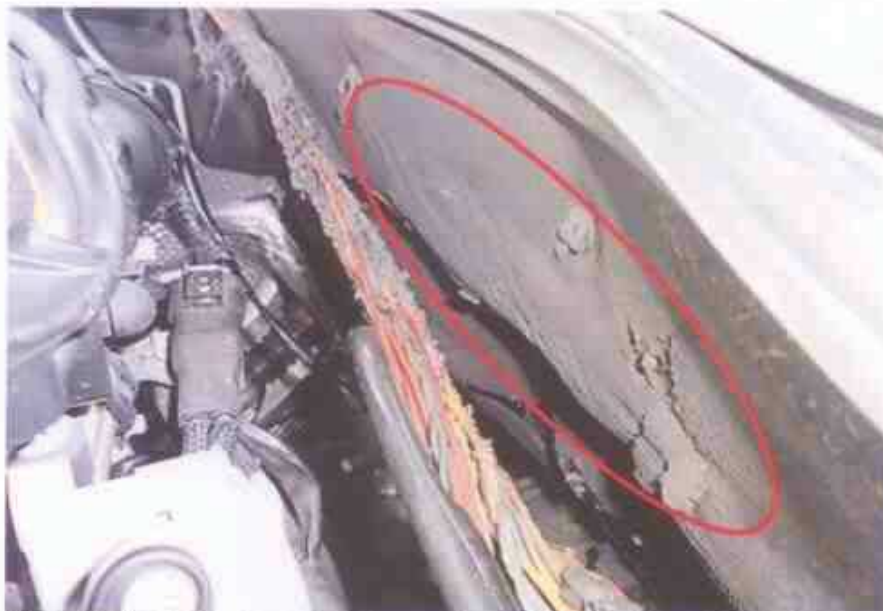
Photo 6 shows the damage of burn nature that was observed on the Insured Vehicle. This was towards the centre rear area of the engine compartment, where I had observed a stretch of partially burnt/melted wiring harness. The firewall insulator behind the stretch of partially burnt/melted wiring harness was also observed to be with minor burn marks (circled).
