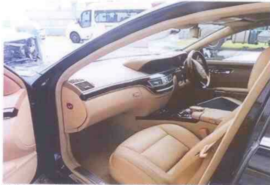
Photo 3 shows the interior compartment of the Insured Vehicle at the time of my inspection. There was no damage of burn nature observed within the interior compartment.
