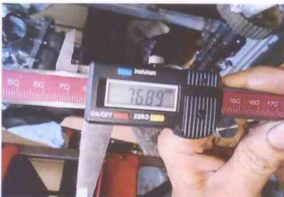
Photo 19 shows the stroke measurement of cylinder 4, which was recorded to be 76.89mm.
