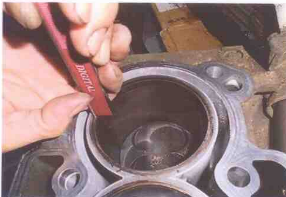
Photo 18 shows measurement being carried out to the stroke of cylinder 4 of the Honda engine. The bore and stroke measurements of the Honda engine were carried out using a digital Vernier Caliper that was calibrated before the start of measurements.
