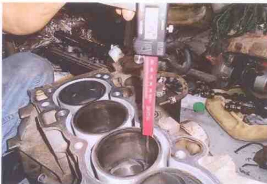
Photo 12 shows measurement of the stroke of cylinder 2 of the Honda engine that I had inspected. The bore and stroke measurements of the Honda engine were carried out using a digital Vernier Caliper that was calibrated before the start of the measurement.
