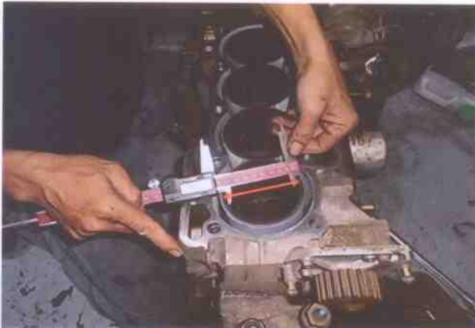
Photo 7 shows measurement being carried out to the bore of cylinder 1 of the Honda engine. The measurement was carried out using a digital Vernier Caliper.
