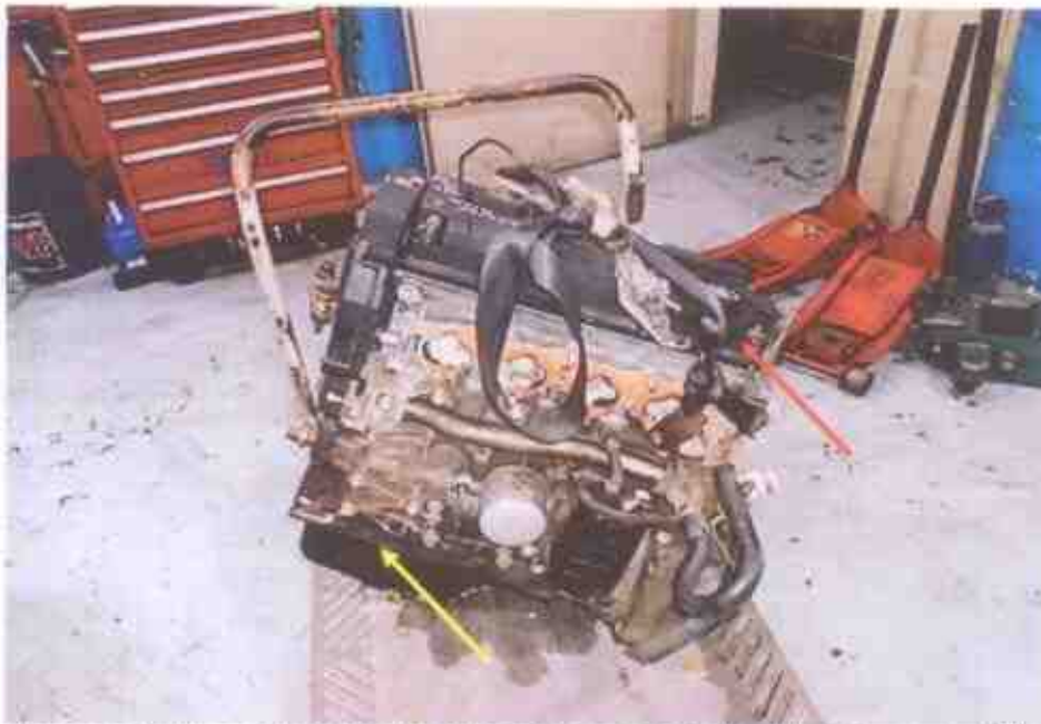
Photo 1 shows a general view of the Honda engine that I had inspected. The Honda engine was observed to be a used engine and was not fitted on any motor car. There was no crack and/or hole observed on the engine housing.
