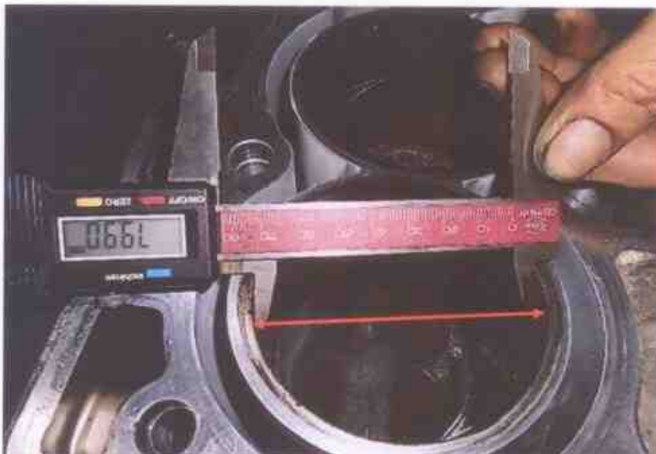
Photo 8 shows measurement being carried out to the bore of cylinder 1 of the Honda engine. The bore measurement of cylinder 1 was recorded to be 79.90mm.
