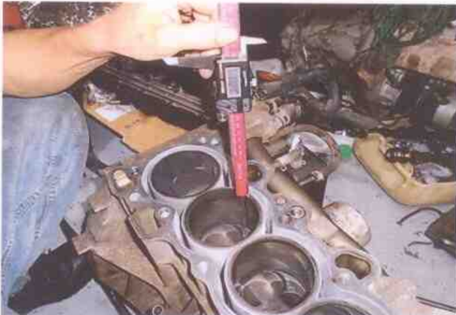
Photo 15 shows measurement of the stroke of cylinder 3 of the Honda engine that I had inspected. The bore and stroke measurements of the Honda engine were carried out using a digital Vernier Caliper that was calibrated before the start of measurements.
