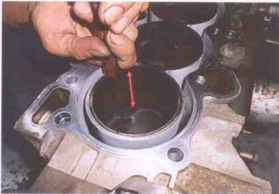
Photo 9 shows measurement being carried out to the stroke of cylinder 1 of the Honda engine. The bore and stroke measurements of the Honda engine were carried out using a digital Vernier Caliper that was calibrated before the start of the measurement.
