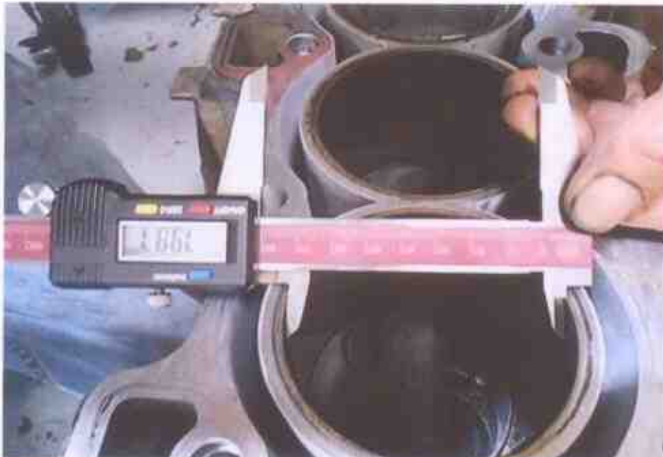
Photo 11 shows measurement being carried out to the bore of cylinder 2 of the Honda engine. The bore measurement of cylinder 2 was recorded to be 79.87mm.
