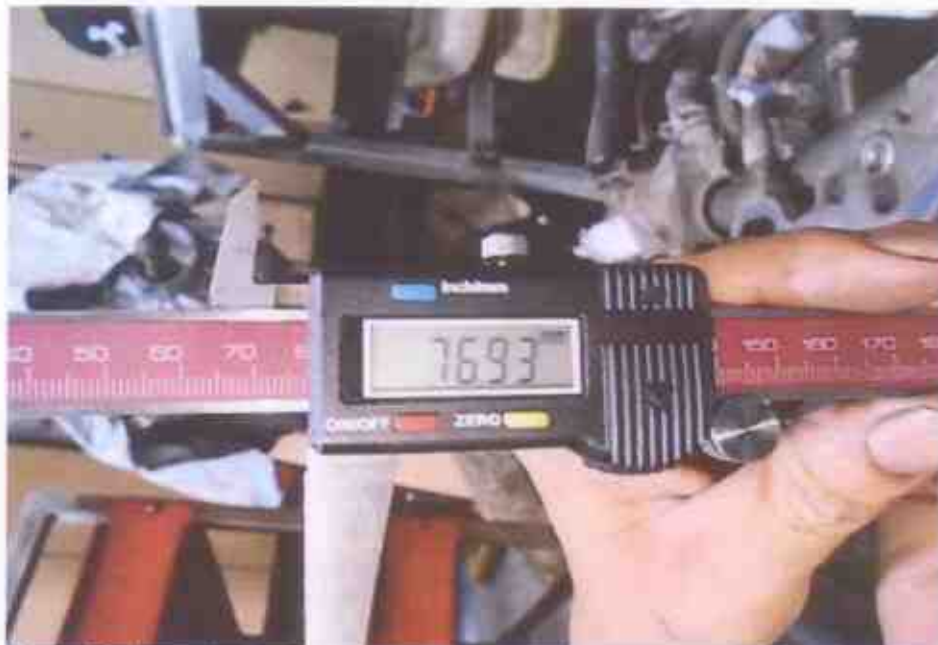
Photo 10 shows the stroke measurement of cylinder 1, which was recorded to be 76.93mm.
