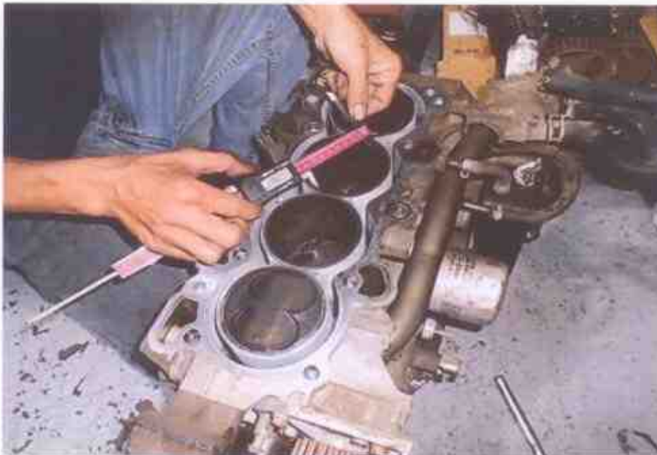
Photo 6 shows the bottom block of the Honda engine and the digital Vernier Caliper that was used to measure the bore and stroke of the Honda engine. The digital Vernier Caliper was calibrated before the start of the measurements.
