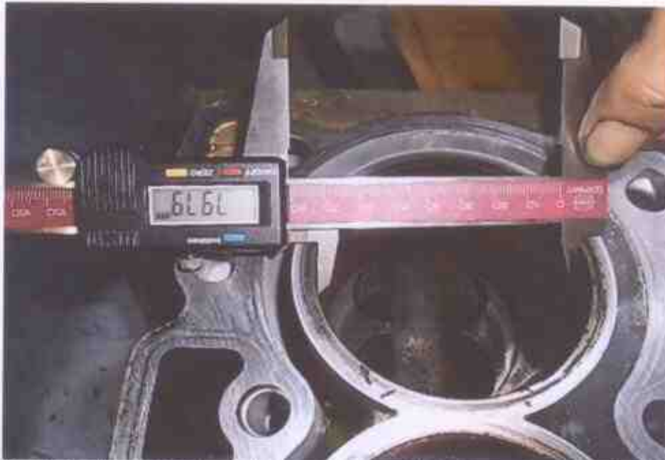
Photo 17 shows measurement being carried out to the bore of cylinder 4 of the Honda engine. The bore measurement of cylinder 4 was recorded to be 79.79mm.
