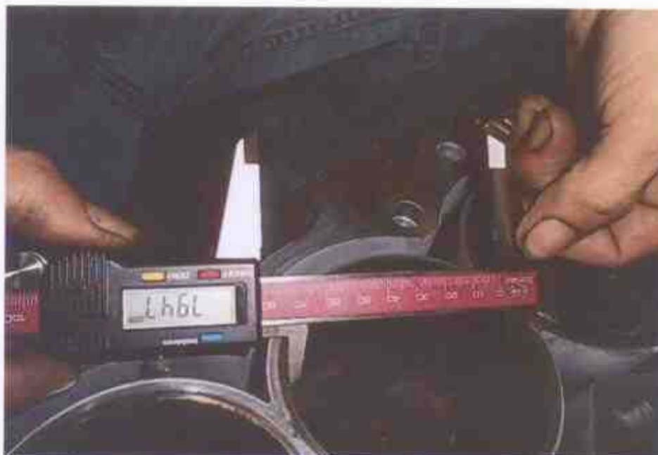
Photo 14 shows measurement being carried out to the bore of cylinder 3 of the Honda engine. The bore and stroke measurements of the Honda engine were carried out using a digital Vernier Caliper. The bore measurement of cylinder 3 was recorded to be 79.47mm.
