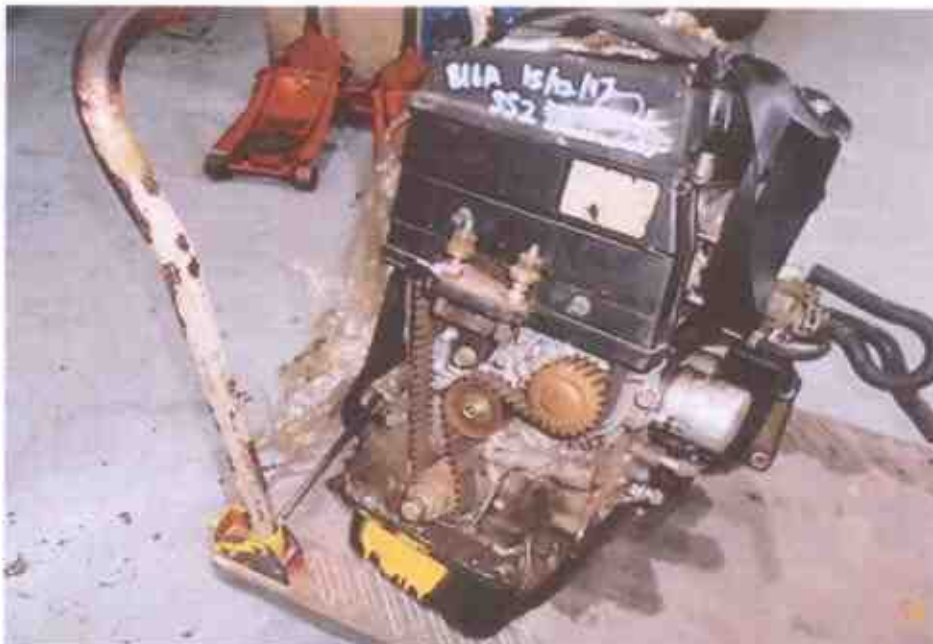
Photo 3 shows a general view of the Honda engine that I had inspected. The Honda engine was observed to be a used engine and was not fitted on any motor car. It was also observed to be a complete assembly with all mechanical parts still intact, within the engine housing.
