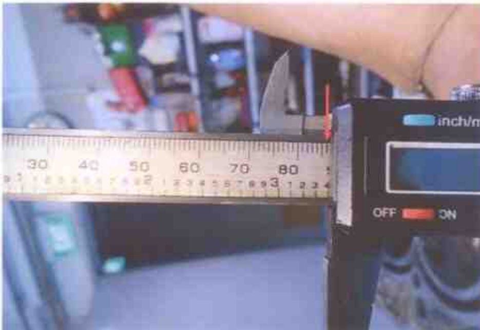
Photo 22 shows the stroke measurement of cylinder 4, which was recorded to be 86.00mm.
