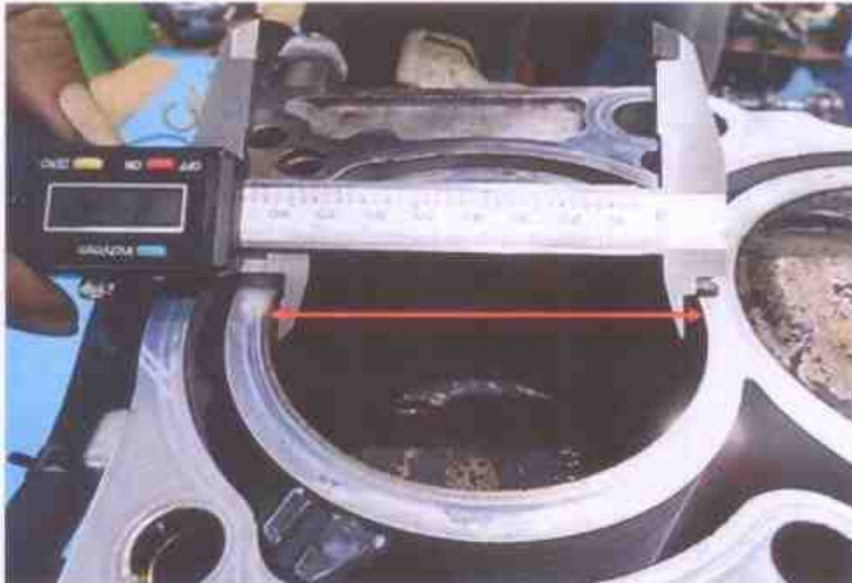
Photo 7 shows measurement being carried out to the bore of cylinder 1 of the Honda engine. The bore and stroke measurements of the Honda engine were carried out using a Vernier Caliper.
