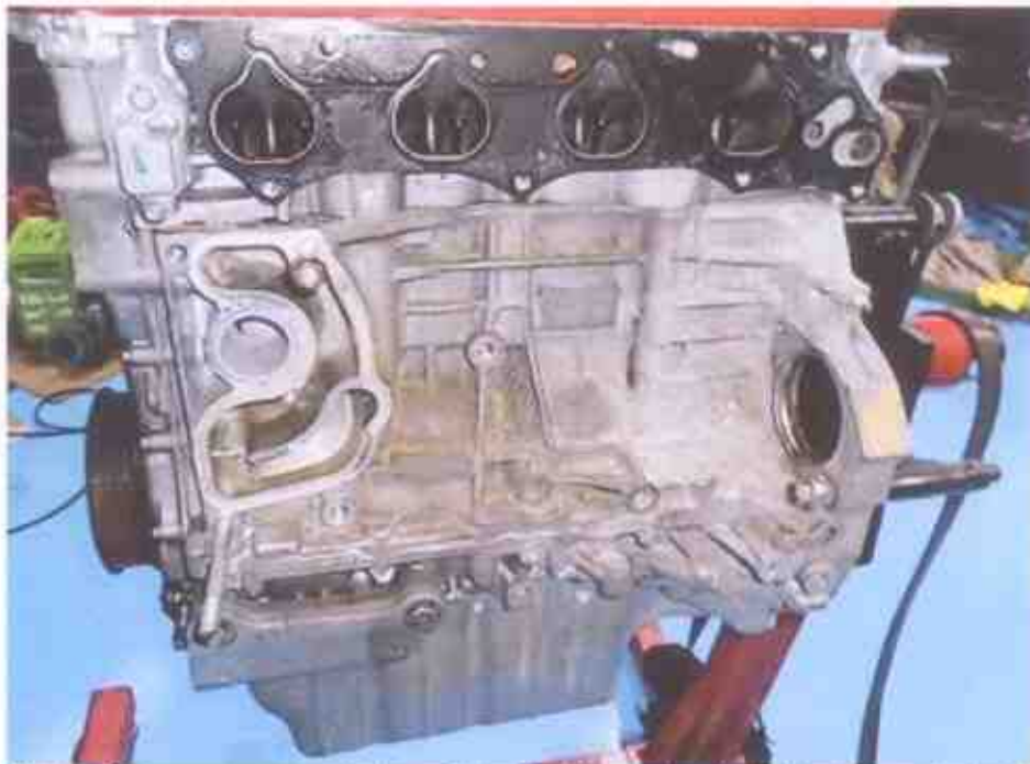
Photo 3 shows a general view of the Honda engine that I had inspected. My visual examination of the engine housing revealed the housing to be of serviceable/satisfactory condition. There was no crack and/or hole observed on the engine housing.
