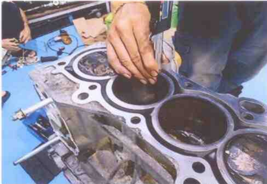
Photo 13 shows measurement of the stroke for cylinder 2 of the Honda engine that I had inspected.
