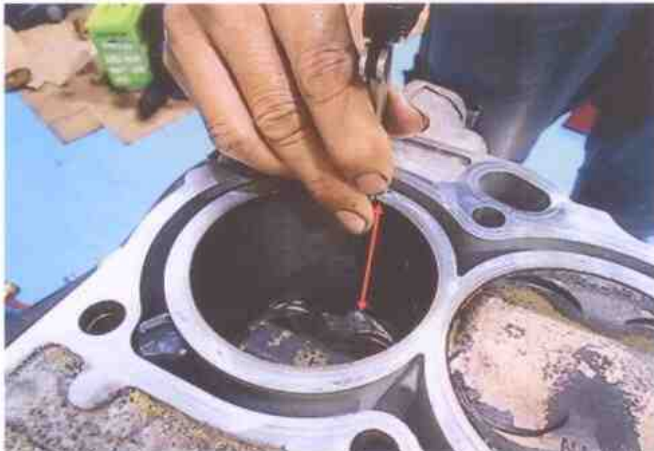
Photo 9 shows measurement being carried out to the stroke of cylinder 1 of the Honda engine. The bore and stroke measurements of the Honda engine were carried out using a Vernier Caliper.
