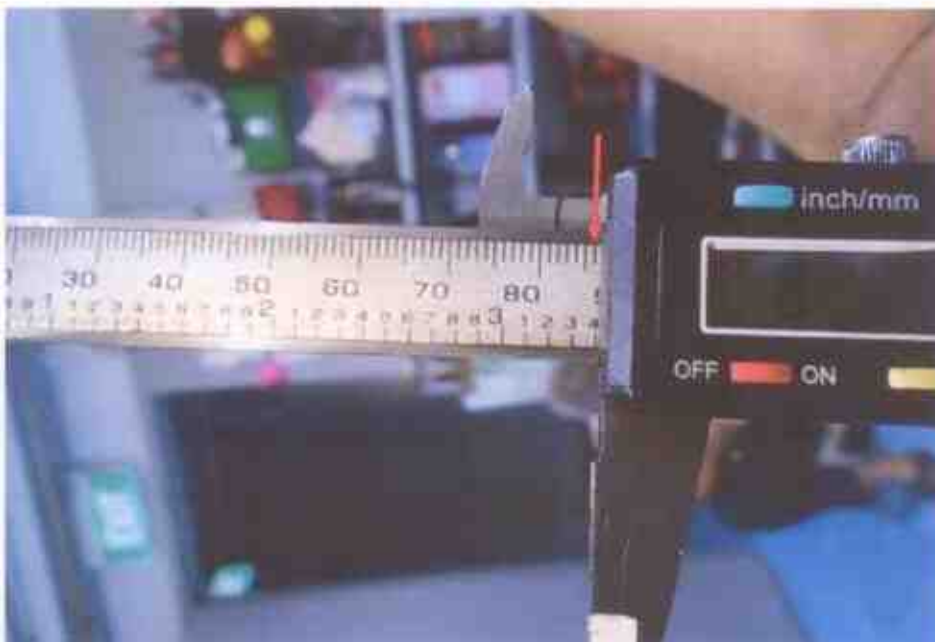
Photo 14 shows the stroke measurement of cylinder 2, which was recorded to be 86.00mm.
