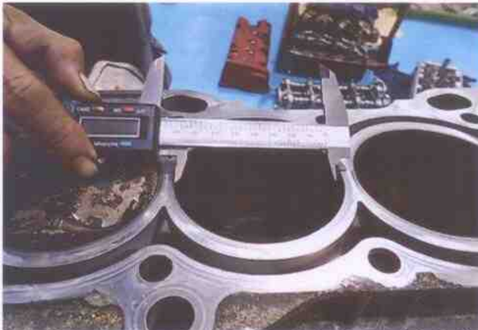
Photo 11 shows measurement being carried out to the bore of cylinder 2 of the Honda engine. The bore and stroke measurements of the Honda engine were carried out using a Vernier Caliper.
