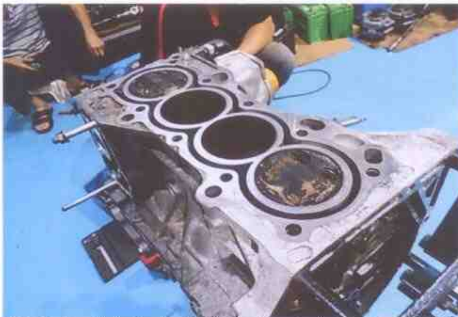
Photo 6 shows the bottom block of the Honda engine that I had inspected. The top block was separated from the bottom block for measurements of the cylinders, in particular the bore and stroke measurements of each cylinder, which typically can be used to determine the engine displacement or more commonly referred to as engine cc.
