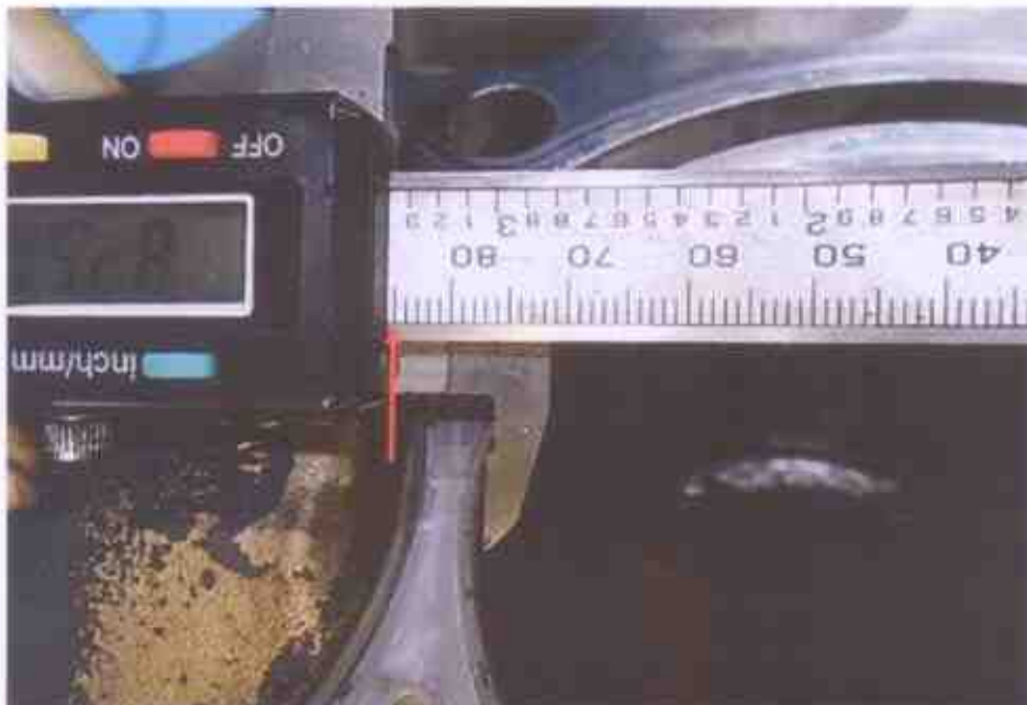
Photo 20 shows the bore measurement of cylinder 4, which was recorded to be 85.00mm.
