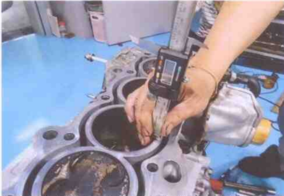
Photo 17 shows measurement of the stroke for cylinder 3 of the Honda engine that I had inspected.
