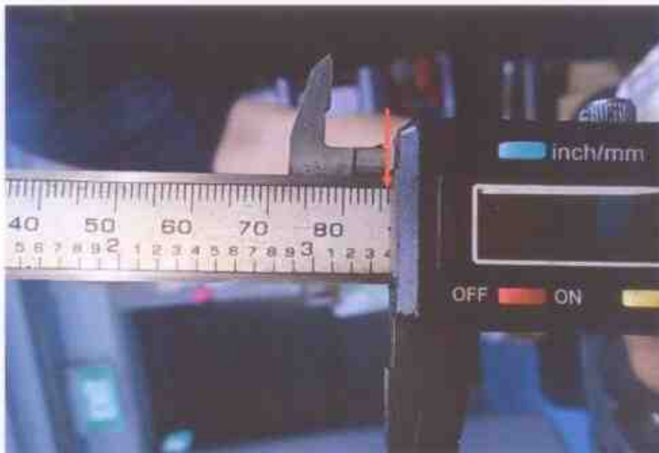
Photo 18 shows the stroke measurement of cylinder 3, which was recorded to be 86.00mm.
