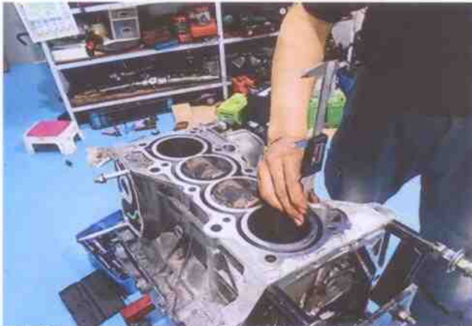
Photo 21 shows measurement being carried out to the stroke of cylinder 4 of the Honda engine. The bore and stroke measurements of the Honda engine were carried out using a Vernier Caliper.
