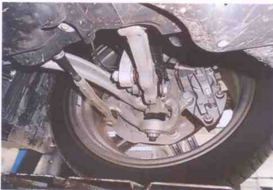
Photo 11 shows the various undercarriage components at the front right wheel of the Motor Car. The mechanical components, control arms and linkages were all found to be intact and secured in an appropriate manner. There was also no fluid leak and/or fluid stain observed on the underside of the Motor Car.
