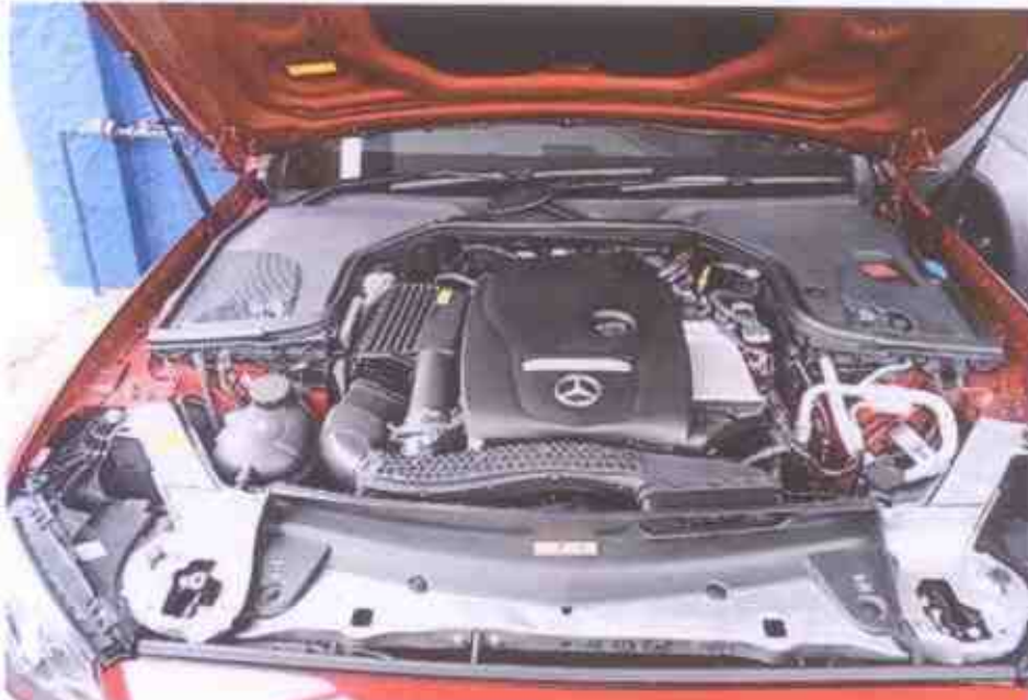
Photo 4 shows the engine compartment of the Motor Car. The various parts and components inside the engine compartment were all observed to be intact and properly fitted. There was also no sign(s) or indication(s) of fluid leak and/or fluid stain found inside the engine compartment. The engine oil, brake fluid and engine coolant were all checked and found to be of sufficient level for operating purposes. Visually, there was also no contamination found to these fluids.
