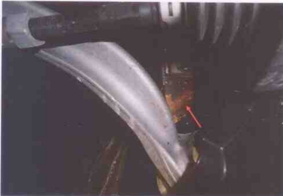
Photo 16 shows the structural body at the front left of the Motor Car. Visually, I did not find any weld marks, other than original spot weld marks on the body panels of the Motor Car. The joints (arrowed) along the body panels were also untouched, indicating no work was done on the body panels of the Motor Car and that the structural body was originally fitted.
