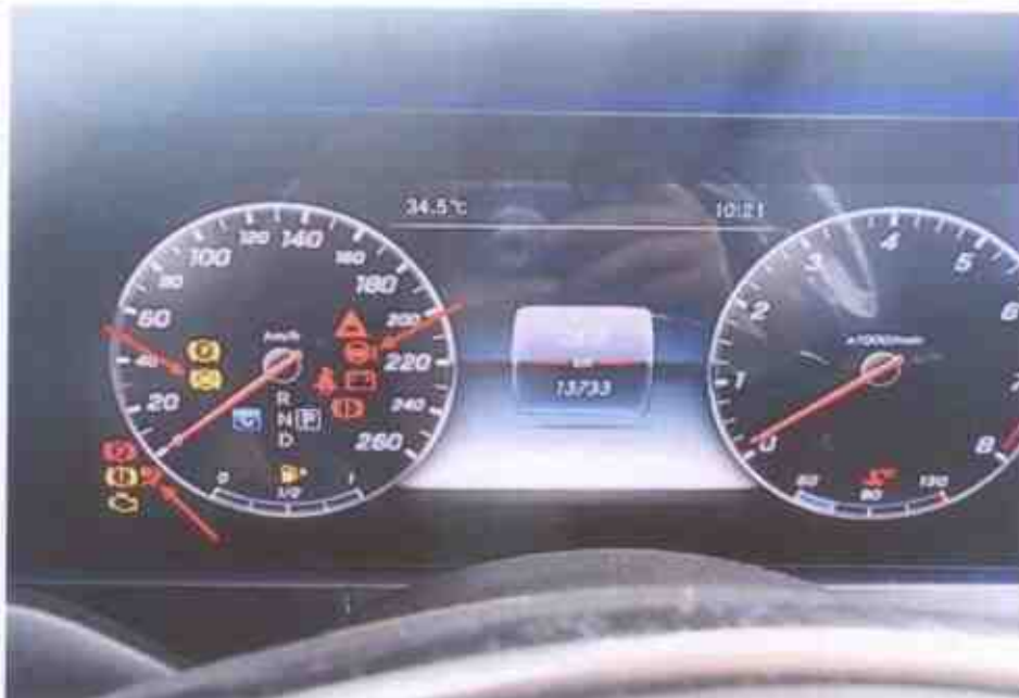
Photo 6 shows the warning lights for the various electronic safety features appearing on the instrument panel of the Motor Car during its self-test when the engine is cranked, in particular the Anti-Brake Lock System (ABS), Supplemental Restraint System (SRS) and Power Steering Assist (PSA) (arrowed).
