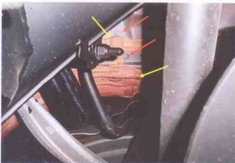
Photo 15 shows a closer view of the structural body/floor panel at the rear right of the Motor Car. I did not find any weld marks, other than original spot weld marks (red arrow), on the body panels of the Motor Car. The original factory sealant (yellow arrow) at the joints along the body panels were also untouched, indicating no work was done on the body panels of the Motor Car.
