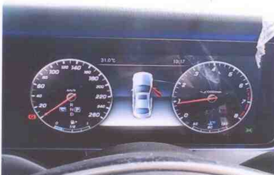
Photo 7 shows the respective warning lights no longer illuminated, indicating that there is no fault detected to the ABS, SRS and PSA systems of the Motor Car during the self-test. These electronic safety features were hence in working condition at the time of my inspection.
