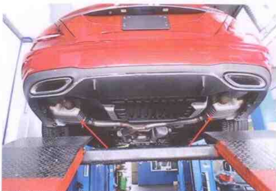
Photo 9 shows the Motor Car hoisted up for checks on its undercarriage. My examination of the Motor Car's exhaust system revealed no sign(s) or indication(s) of any cut or weld marks along its exhaust pipes and on its rear muffler (arrowed).
