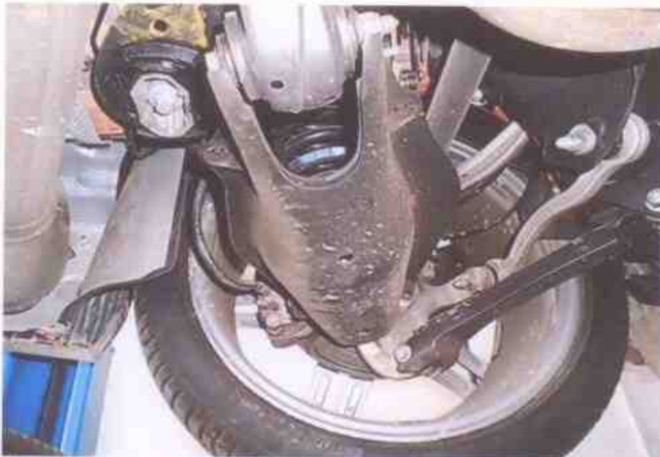
Photo 10 shows the various undercarriage components at the rear left wheel of the Motor Car. The mechanical components, control arms and linkages were all found to be intact and secured in an appropriate manner. There was also no sign(s) or indication(s) of fluid leakage and/or fluid stain(s).
