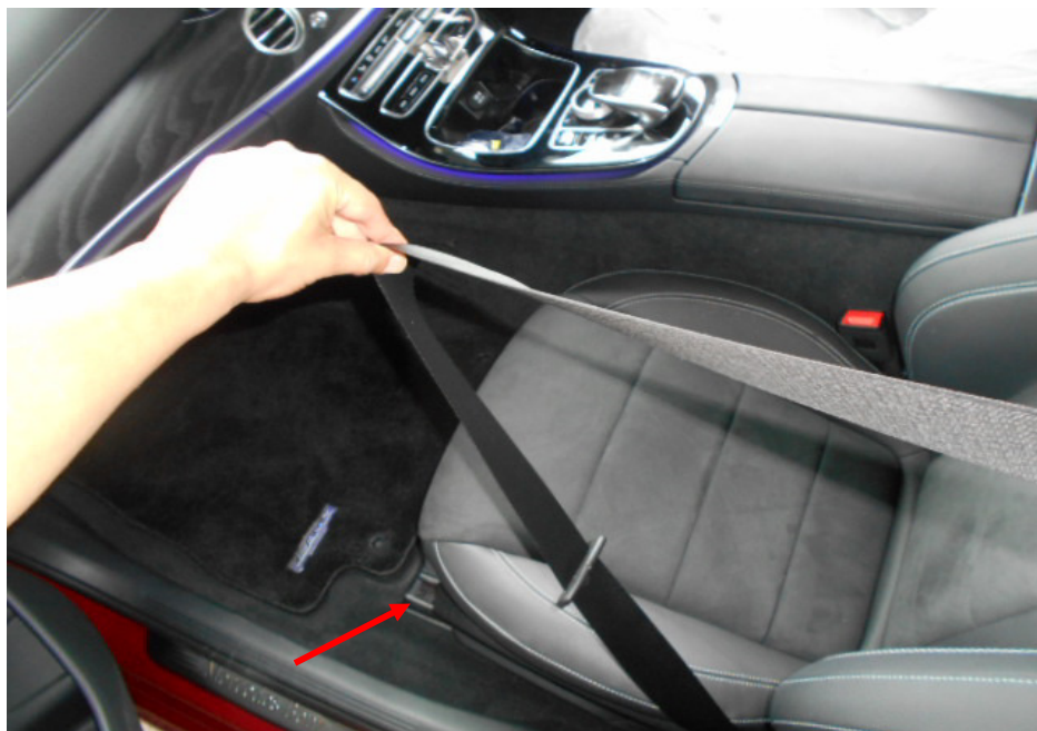
Photo 8 shows the interior compartment of the Motor Car. The seats of the Motor Car were found to be secured to the floor panel of the Motor Car via seat rails (arrowed) that were bolted onto the floor board. Retractable seat belt reels and pre-tensioners were fitted on all seats of the Motor Car. The seat belt reels were able to be fastened securely to the respective pre-tensioner that is fixed to the side of all the seats.
