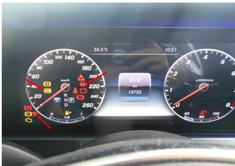
Photo 6 shows the warning lights for the various electronic safety features appearing on the instrument panel of the Motor Car during its self-test when the engine is cranked, in particular the Anti-Brake Lock System (ABS), Supplemental Restraint System (SRS) and Power Steering Assist (PSA) (arrowed).
