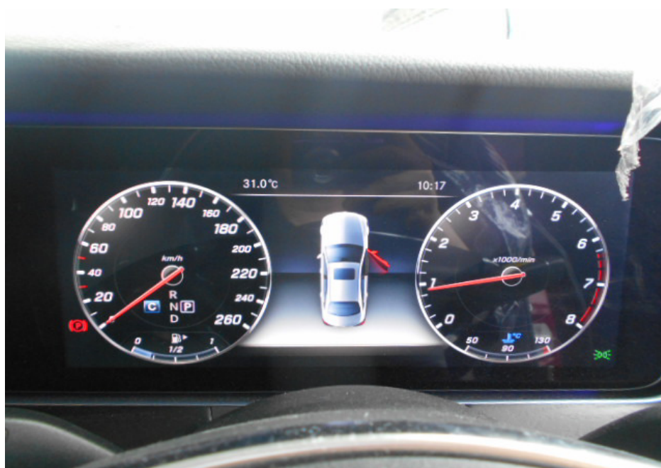
Photo 7 shows the respective warning lights no longer illuminated, indicating that there is no fault detected to the ABS, SRS and PSA systems of the Motor Car during the self-test. These electronic safety features were hence in working condition at the time of my inspection.
