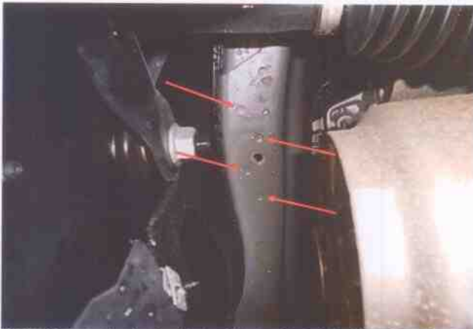
Photo 16 shows the structural body at the front left of the Motor Car. Visually, I did not find any weld marks, other than original spot weld marks (arrowed), on the body panels of the Motor Car. The joints along the body panels were also untouched, indicating no work was done on the body panels of the Motor Car and that the structural body was originally fitted.
