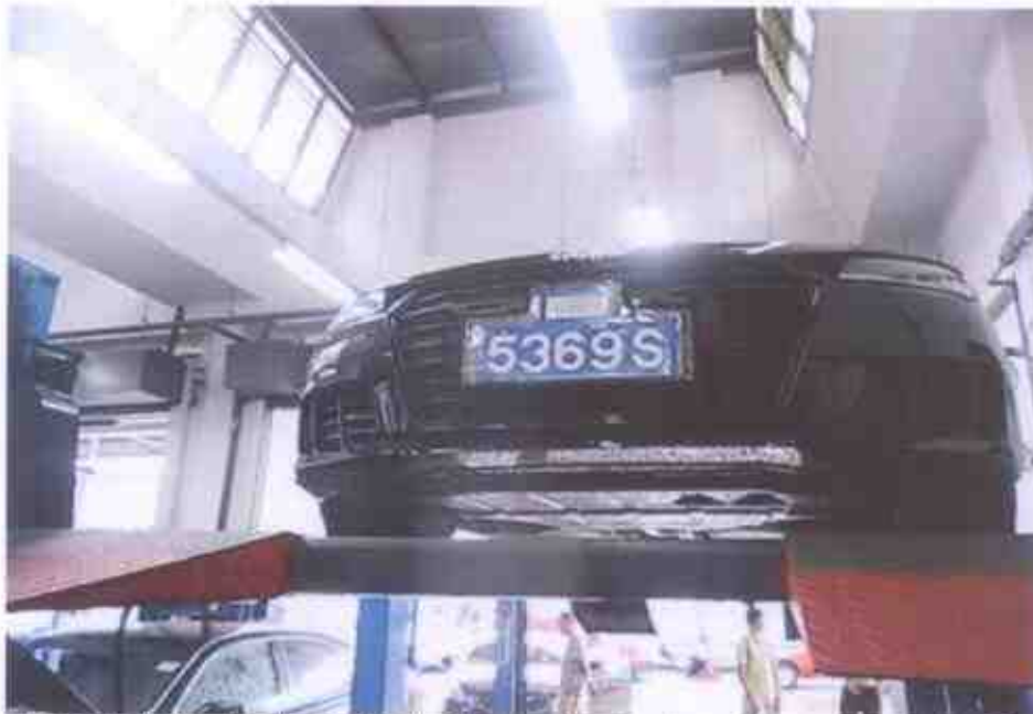
Photo 8 shows the Motor Car hoisted up for checks on its undercarriage. The undercarriage components of the Motor Car were all observed to be intact and secured in an appropriate manner. There was also no sign(s) or indication(s) of fluid leakage and/or fluid stain(s).
