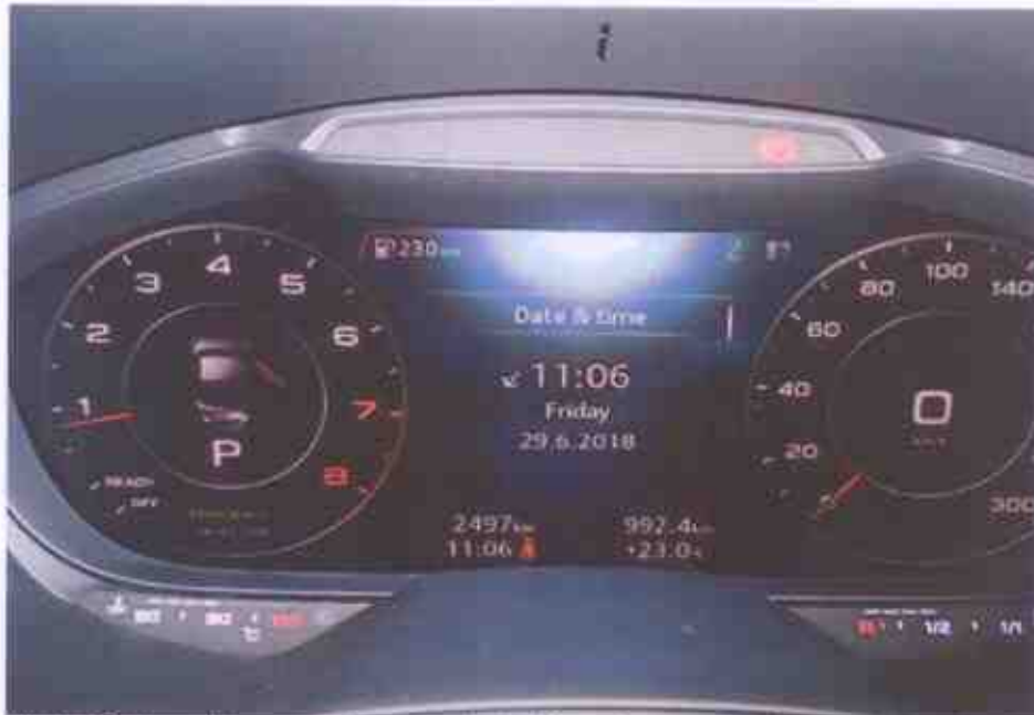
Photo 6 shows the respective warning lights no longer illuminated, indicating that there is no fault detected to the ABS, SRS, EPS and TCS systems of the Motor Car during the self-test. These electronic safety features were hence in working condition at the time of my inspection.
