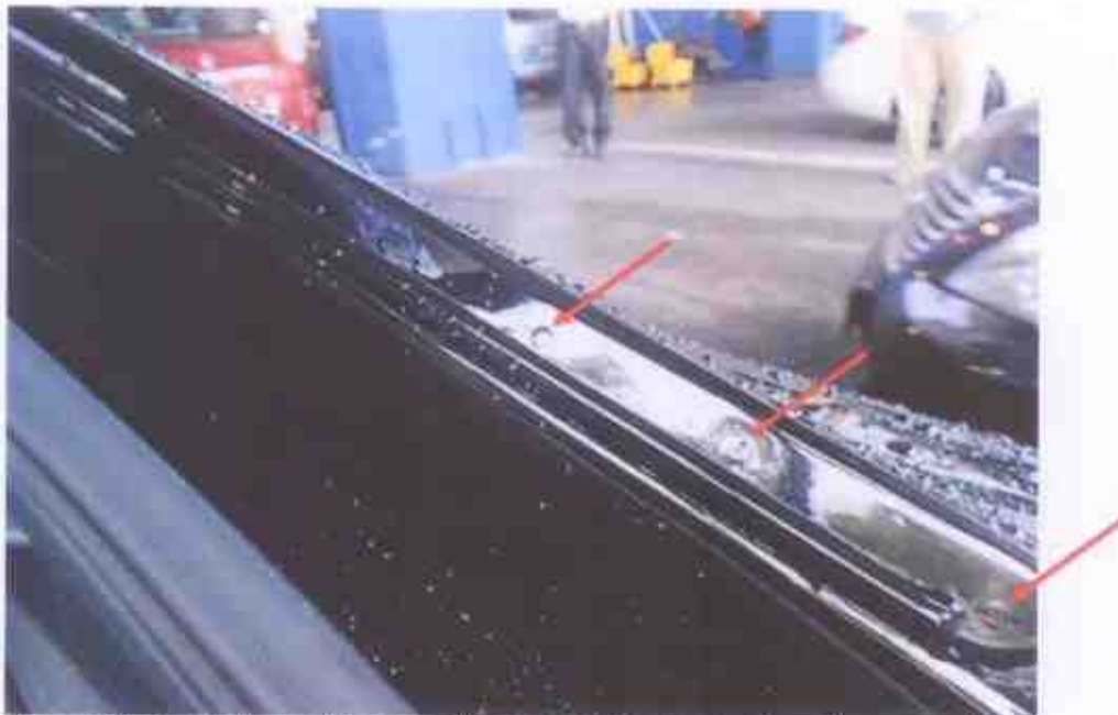
Photo 18 shows the right rear body panel of the Motor Car. The original spot weld marks (arrowed) was found to be untouched, indicating no work was done on the right rear body panel of the Motor Car.
