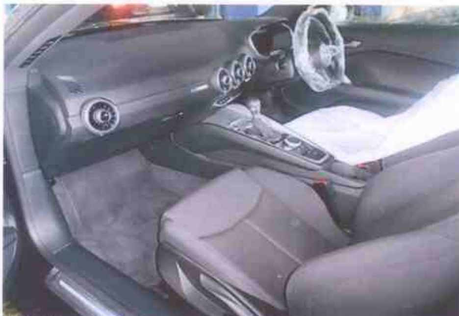
Photo 7 shows the interior compartment of the Motor Car. The seats of the Motor Car were found to be secured to the floor panel of the Motor Car via seat rails bolted onto the floor board. Retractable seat belt reels and pre-tensioners were fitted on all seats of the Motor Car. The seat belt reels were able to be fastened securely to the respective pre-tensioner that is fixed to the side of all the seats.
