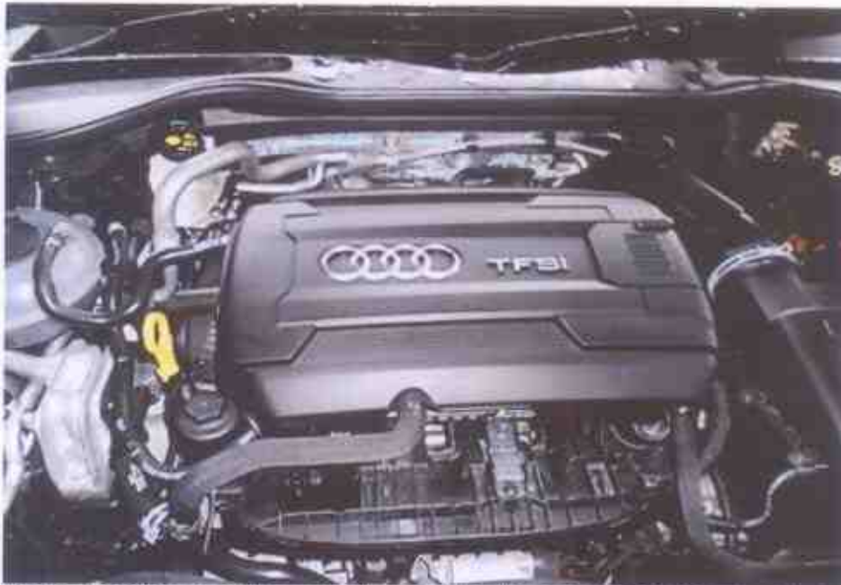
Photo 4 shows the engine compartment of the Motor Car. The various parts and components inside the engine compartment were all observed to be intact and properly fitted. There was no sign(s) or indication(s) of fluid leak and/or fluid stain found inside the engine compartment. The engine oil, brake fluid and engine coolant were all checked and found to be of sufficient level for operating purposes. Visually, there was no contamination found to these fluids.
