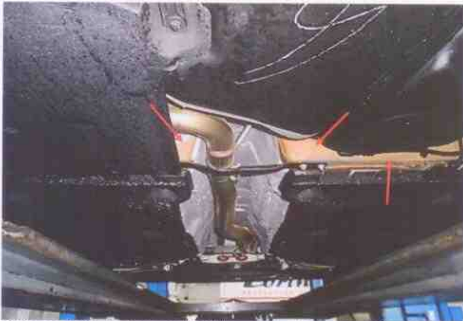
Photo 12 shows the structural body/floor panel at the centre of the Motor Car. Visually, I did not find any weld marks, other than original spot weld marks, on the body panels of the Motor Car. The original factory sealant (arrowed) at the joints along the body panels were also untouched, indicating no work was done on the body panels of the Motor Car and that the structural body was originally fitted.
