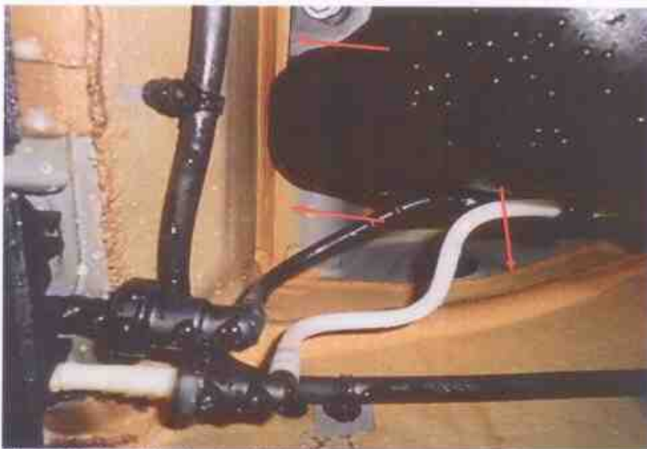
Photo 13 shows the structural body/floor panel at the centre right of the Motor Car. I did not find any weld marks, other than original spot weld marks, on the body panels of the Motor Car. The original factory sealant (arrowed) at the joints along the body panels were also untouched, indicating no work was done on the body panels of the Motor Car and that the structural body was originally fitted.
