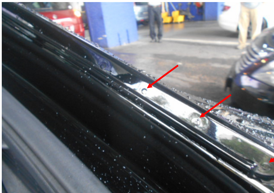
Photo 18 shows the right rear body panel of the Motor Car. The original spot weld marks (arrowed) was found to be untouched, indicating no work was done on the right rear body panel of the Motor Car.
