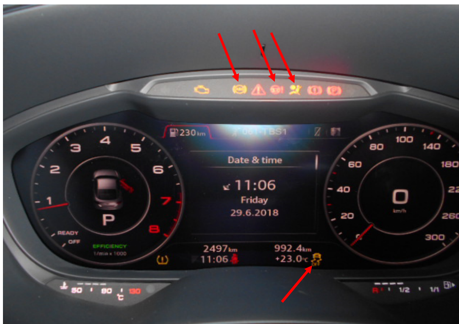
Photo 5 shows the warning lights for the various electronic safety features appearing on the instrument panel of the Motor Car during its self-test when the engine is cranked, in particular the Anti-Brake Lock System (ABS), Supplemental Restraint System (SRS), Electric Power Steering (EPS) and Traction Control System (TCS) (arrowed).
