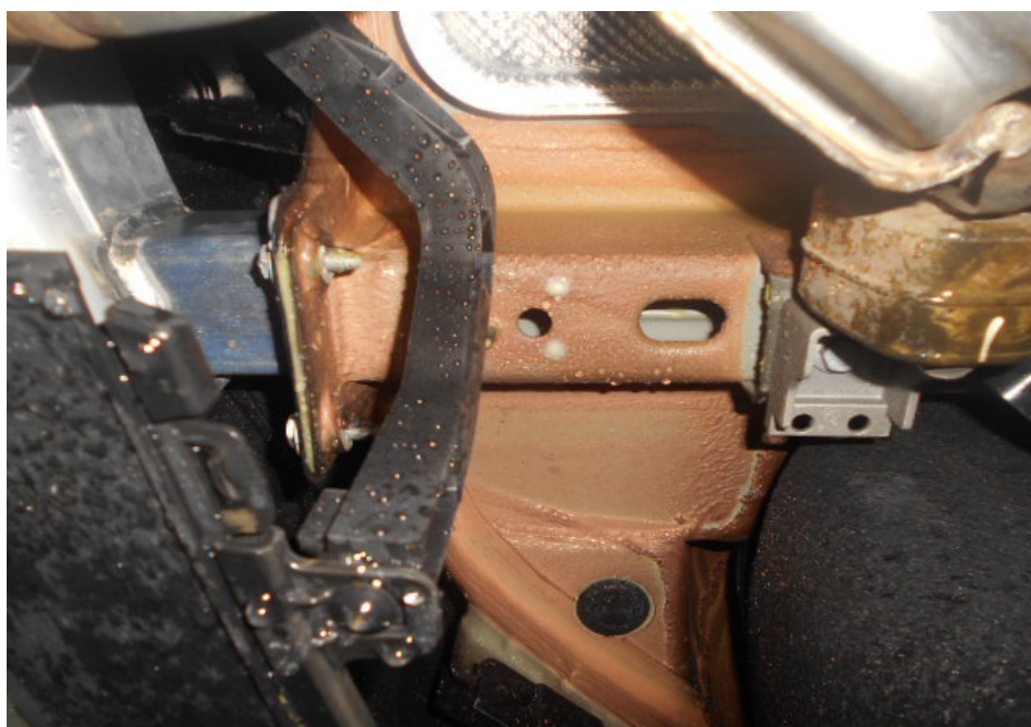
Photo 15 shows the structural body at the rear left of the Motor Car. Visually, I did not find any weld marks, other than original spot weld marks on the body panels of the Motor Car. The joints along the body panels were also untouched, indicating no work was done on the body panels of the Motor Car and that the structural body was originally fitted.
