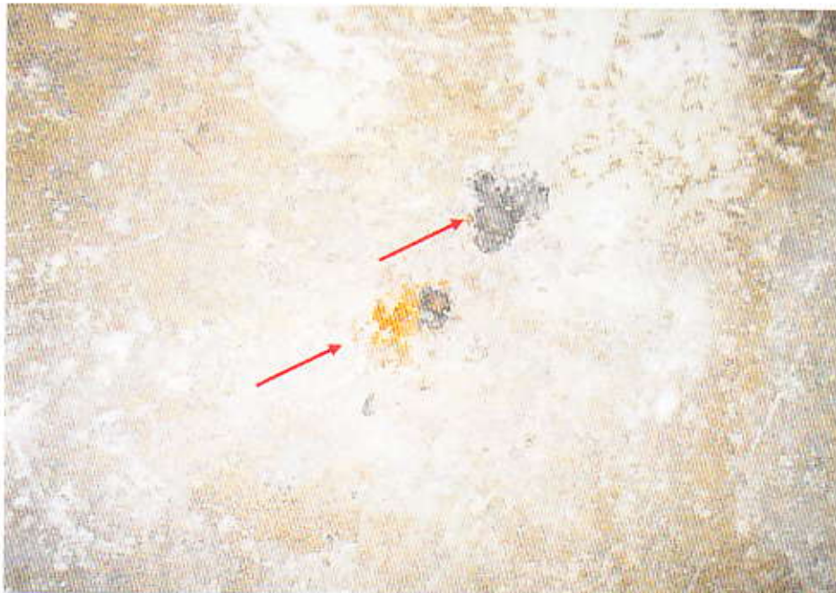
Photo 12 shows the close-up view of the melted burnt substance believed to be from the burnt Insured Vehicle.
