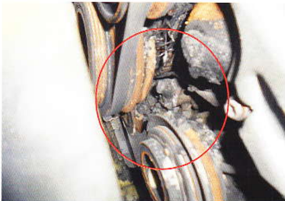
Photo 8 shows the close-up view of the melted rubber materials as a result of the fire incident. This would indicate where the fire had started at time of the fire incident.
