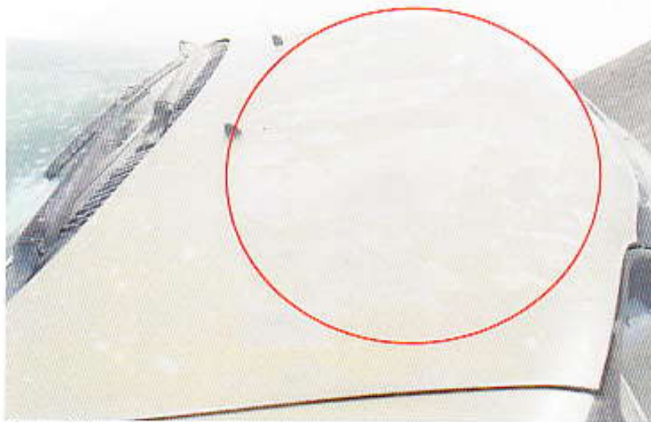
Photo 1 shows the general view of the front portion of the Insured Vehicle at the time of our inspection. The fire damage to the Insured Vehicle was confined to its front top bonnet & at the centre area as a result of the fire.
