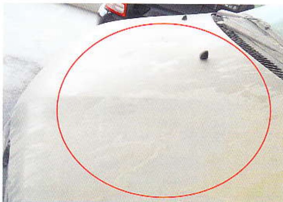
Photo 5 shows the burn pattern and peeling burn marks (circled) that were found on the topside of the front bonnet of the Insured Vehicle. Such peeling burn marks are a result of exposure to prolong heat intensity, which may indicate where the fire had started.
