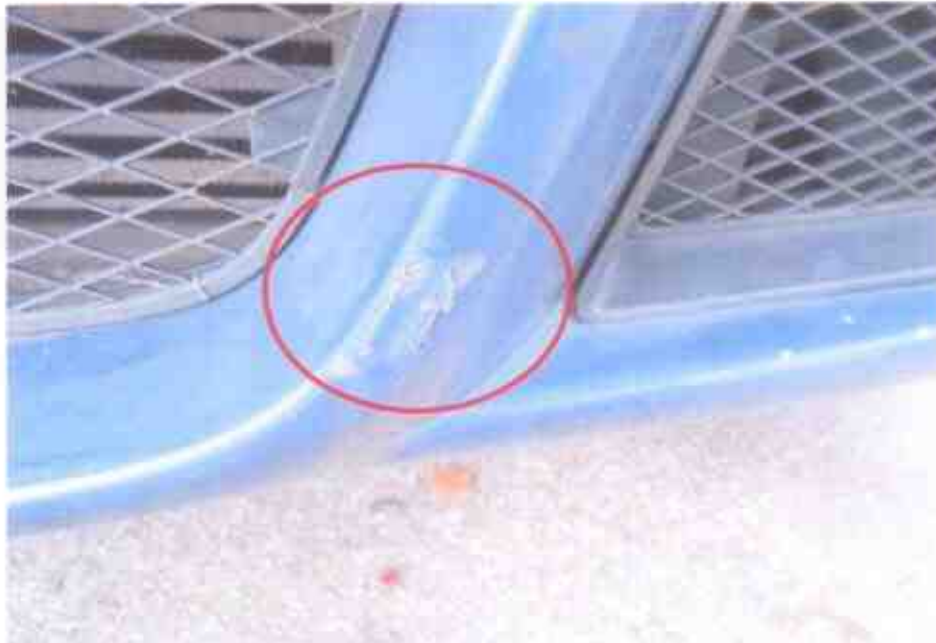
Photo 3 shows a close-up view of the scratches on the front left lower bumper of the Motor Van at the time of our inspection. It was observed to have sustained with minor damage likely due to the accident.
