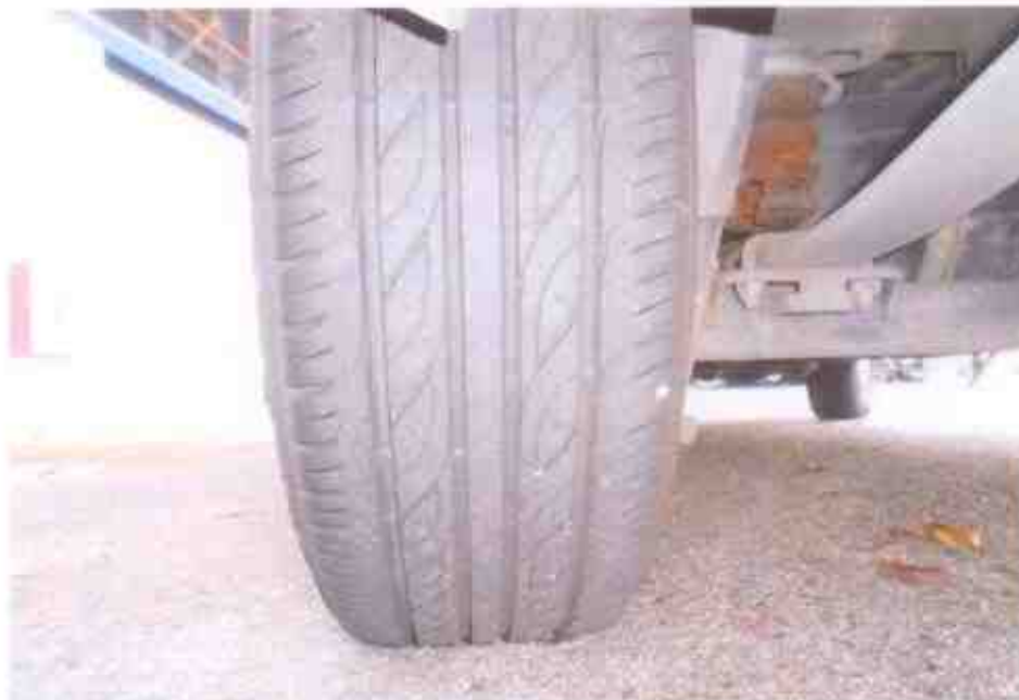
Photo 10 shows the condition of the rear left tyre of the Motor Van, which was observed to be in serviceable condition with remaining tread depth of approximately 6mm. The tyre, which was wrapped around standard wheel rim, was also observed to be sufficiently inflated for vehicular operation. There was also no significant damage found on the 4 wheel rims of the Motor Van.
