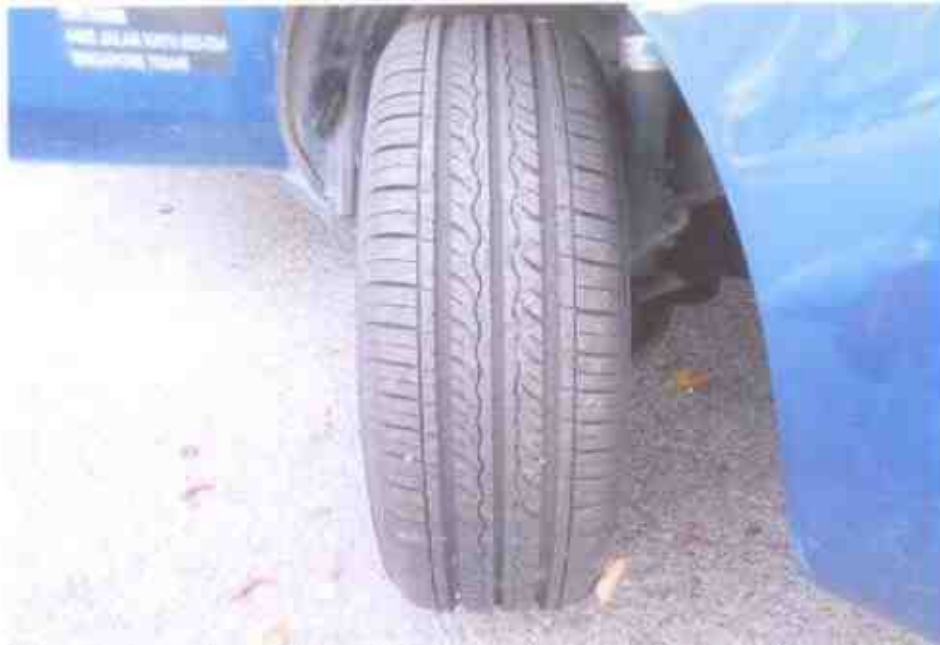
Photo 8 shows the condition of the front right tyre of the Motor Van, which was observed to be in serviceable condition with remaining tread depth of approximately 7mm. The tyres were all observed to be sufficiently inflated for vehicular operation with no tear, cut or burst mark(s) on the outer and the inner sidewalls as well as across the tread.
