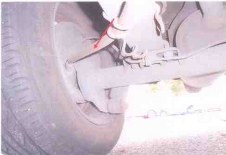
Photo 20 shows the various undercarriage components at the rear right wheel of the Motor Van. The various steering components were all found to be intact, suggesting that the steering system of the Motor Van was likely to be in serviceable condition at the material time of accident. There was also no sign of fluid stain(s) observed on the various undercarriage components at the 4 wheels of the Motor Van.
