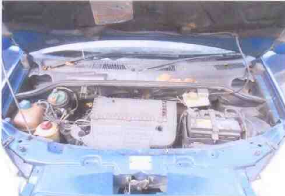
Photo 12 shows a general view of the Motor Van's engine compartment. The various parts and components inside the engine compartment were unaffected by the accident. There was also no sign(s) or indication(s) of fluid leakage and/or fluid stain within the engine compartment.
