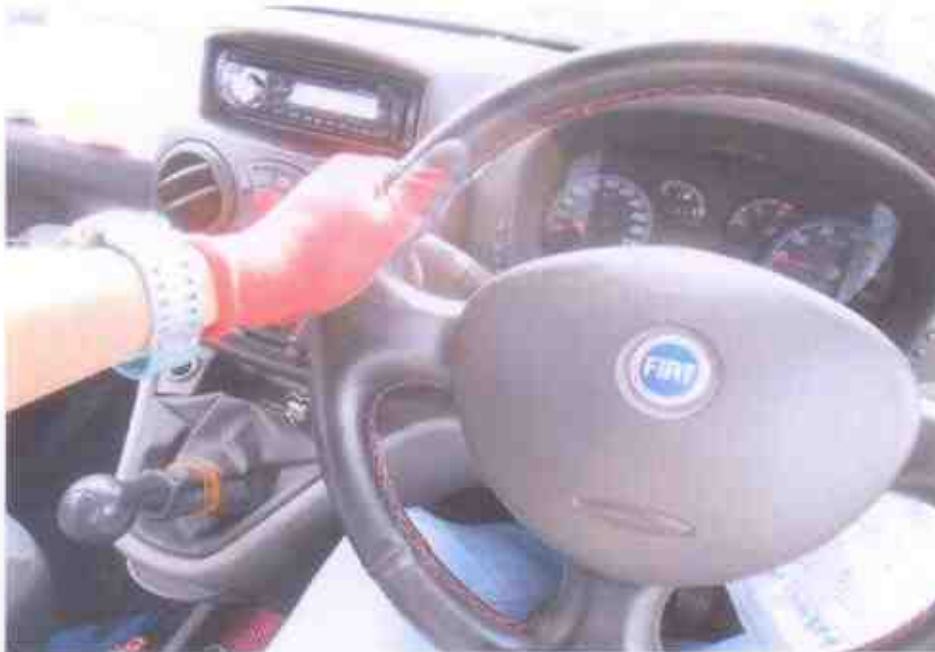
Photo 23 shows a short operational test of the Motor Van, to primarily determine whether there was any abnormality to its various operating systems like its engine system, its transmission system, steering system and braking system was subsequently carried out. The test was conducted by driving the Motor Van forward, stopping, before reversing and coming to a stop again.
