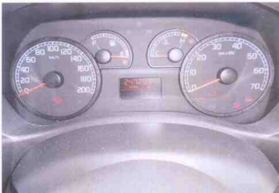
Photo 21 shows the warning lights for the various electronic operating systems of the Motor Car appearing on its instrument panel during the self-test when the engine was cranked.
