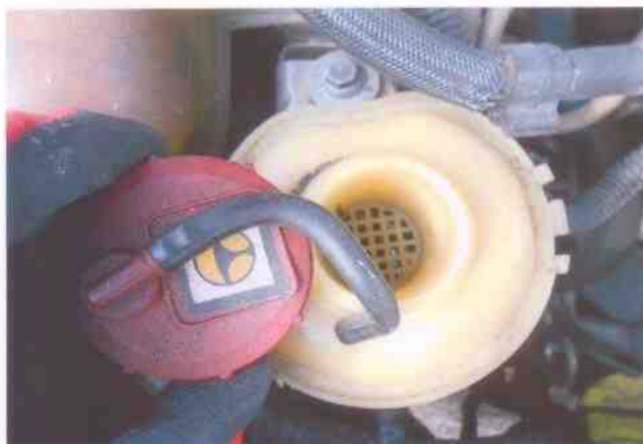
Photo 15 shows the power steering reservoir of the Motor Van at the time of our inspection. It was observed to be of sufficient level and without any visible contamination.
