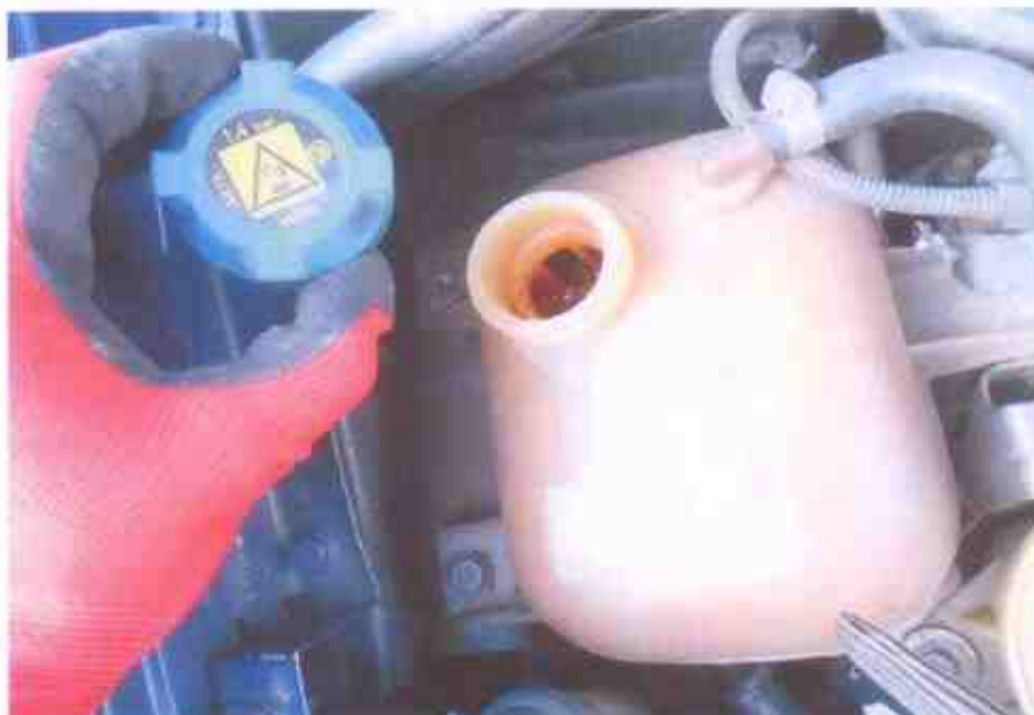
Photo 14 shows the engine coolant reservoir of the Motor Van at the time of our inspection. The engine coolant was observed to be of sufficient level and without any visible contamination.
