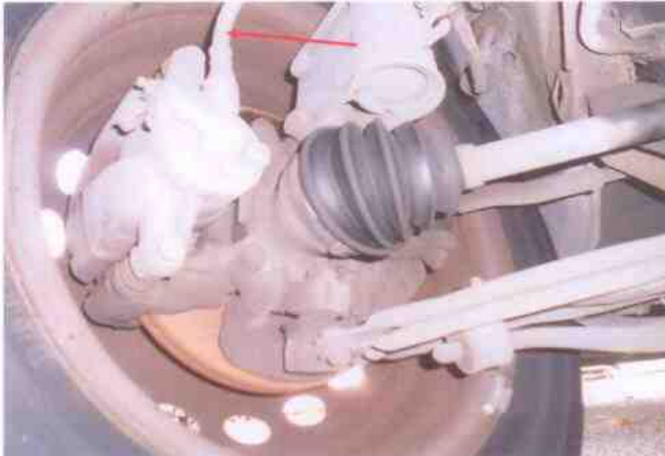
Photo 19 shows the brake hose (arrowed) at the front right wheel of the Motor Van. We did not observe any leakage of brake fluid at the time of our inspection of the Motor Van. Our visual inspection of the various mechanical components of the Motor Van's braking system, including its brake calliper, revealed all to be intact and without visible damage.
