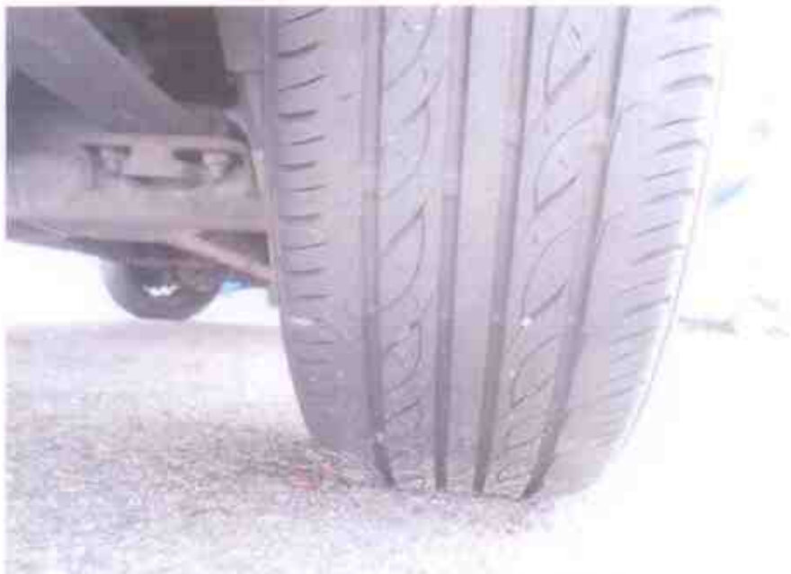
Photo 11 shows the condition of the rear right tyre of the Motor Van, which was observed to be in serviceable condition with remaining tread depth of approximately 6mm. There was also no tear, cut or burst mark(s) on the outer and the inner sidewalls as well as across the tread of the tyre, which was also sufficiently inflated for vehicular operation.
