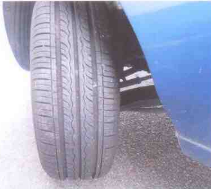
Photo 9 shows the condition of the front left tyre of the Motor Van, which was observed to be in serviceable condition with remaining tread depth of approximately 7mm. The tyre, which was wrapped around standard wheel rim, was also observed to be sufficiently inflated for vehicular operation.
