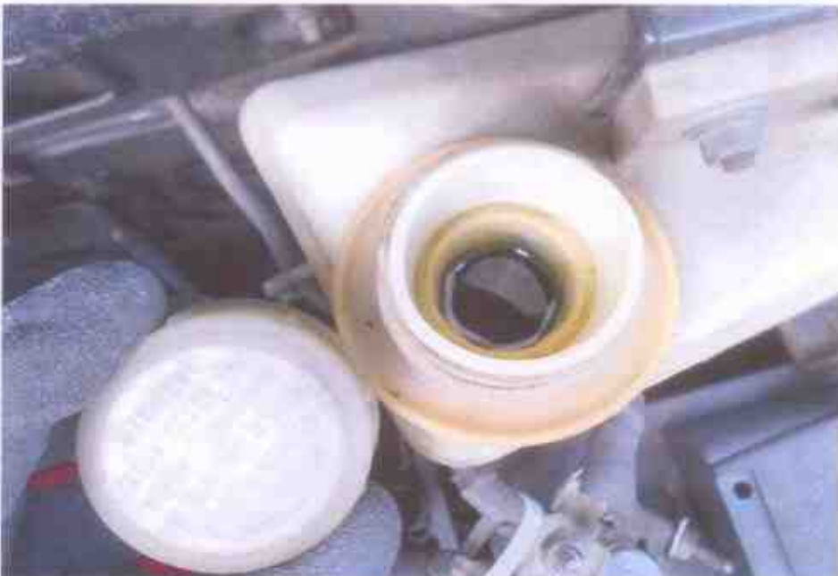
Photo 13 shows the brake fluid reservoir of the Motor Van at the time of our inspection. The brake fluid was observed to be of sufficient level and without any visible contamination.
