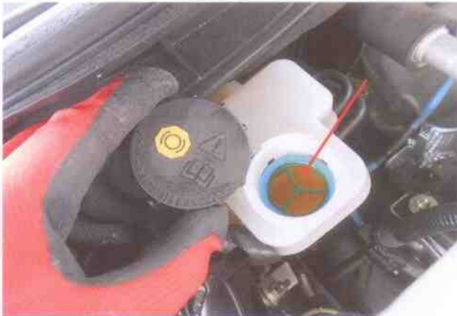
Photo 12 shows the brake fluid reservoir of the Motor Car at the time of our inspection. The brake fluid was observed to be of sufficient level (arrowed) and without any visible contamination.
