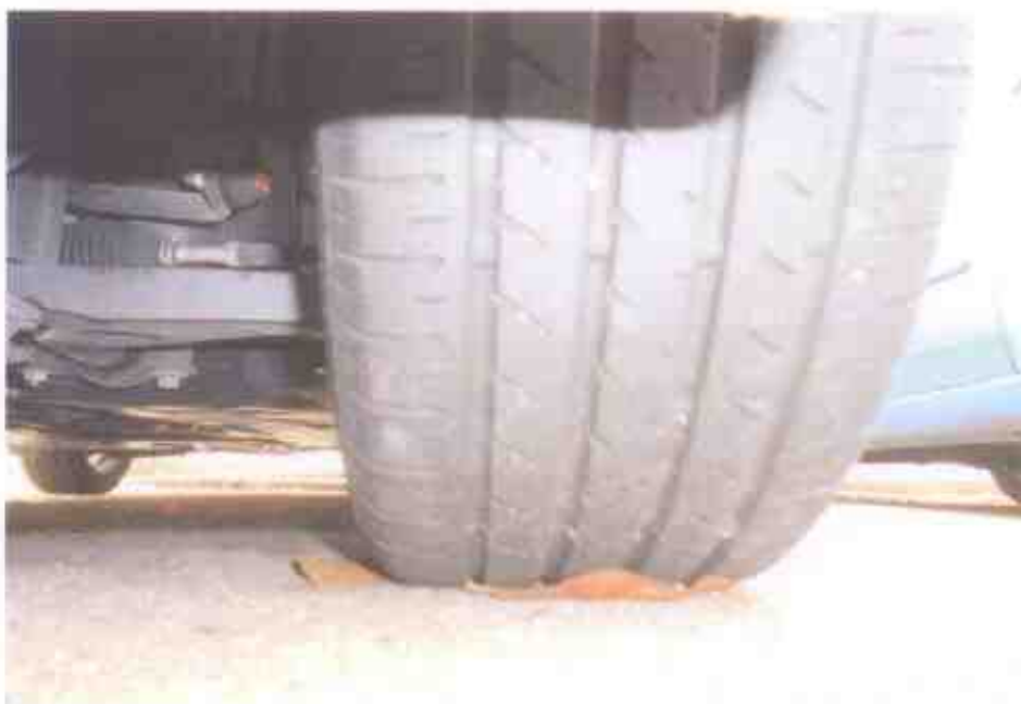
Photo 7 shows the condition of the front left tyre of the Motor Car, which was observed to be in serviceable condition with remaining tread depth of approximately 5mm. The tyre was also observed to be sufficiently inflated for vehicular operation.
