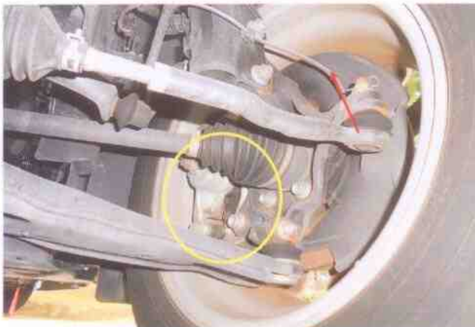
Photo 16 shows the brake hose (arrowed) at the front right wheel of the Motor Car. Our visual inspection of the various mechanical components of the Motor Car's braking system, including its brake calliper (circled), revealed all to be intact and without visible damage, indicating that the braking system was likely to be in serviceable condition at the material time of accident.
