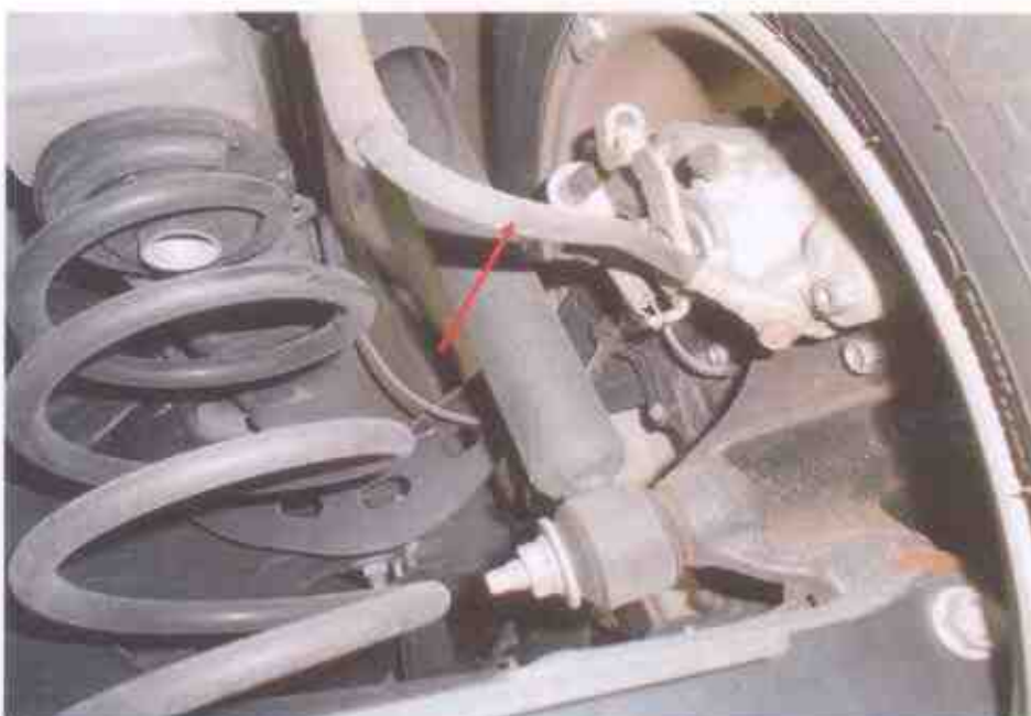
Photo 18 shows the various undercarriage components at the rear right wheel of the Motor Car. We did not observe any leakage of brake fluid at the time of our inspection of the Motor Car. Our visual inspection of the various mechanical components of the Motor Car's braking system revealed all to be intact and without visible damage, indicating that the braking system was likely to be in serviceable condition at the material time of accident.
