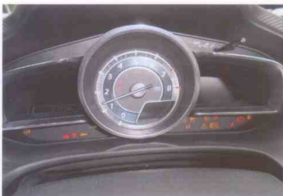
Photo 19 shows the warning lights for the various electronic operating systems of the Motor Car appearing on its instrument panel during the self-test when the engine is cranked, in particular the ABS light and SRS light.
