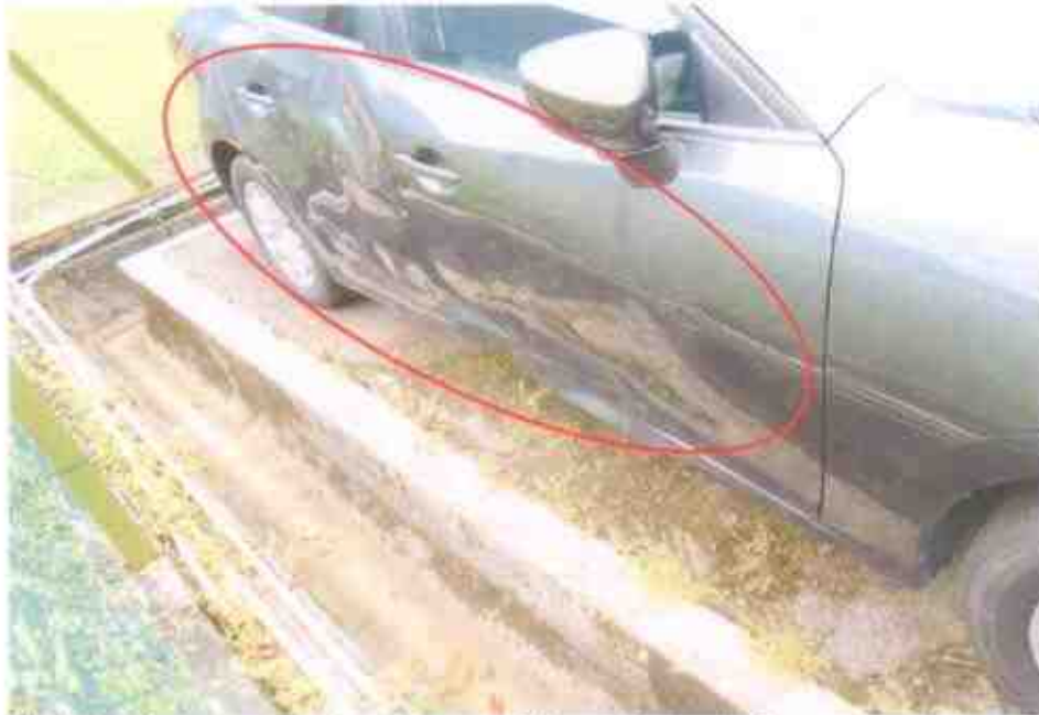
Photo 5 shows a semi-close up view of the right driver's & passenger's door of the Motor Car at the time of our inspection. It had sustained damages due to the accident.
