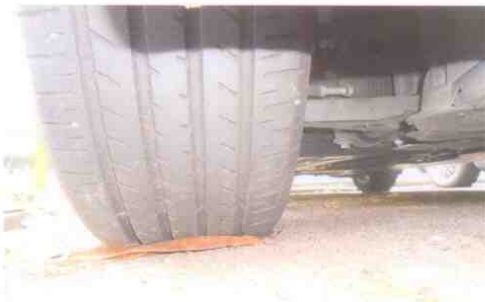
Photo 7 shows the condition of the front left tyre of the Motor Car, which was observed to be in serviceable condition with remaining tread depth of approximately 5mm. The tyre was also observed to be sufficiently inflated for vehicular operation.
