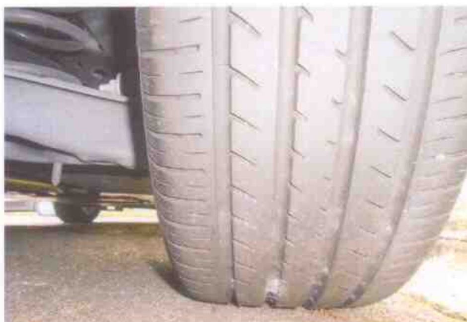
Photo 10 shows the condition of the rear right tyre of the Motor Car, which was observed to be in serviceable condition with remaining tread depth of approximately 7mm.
