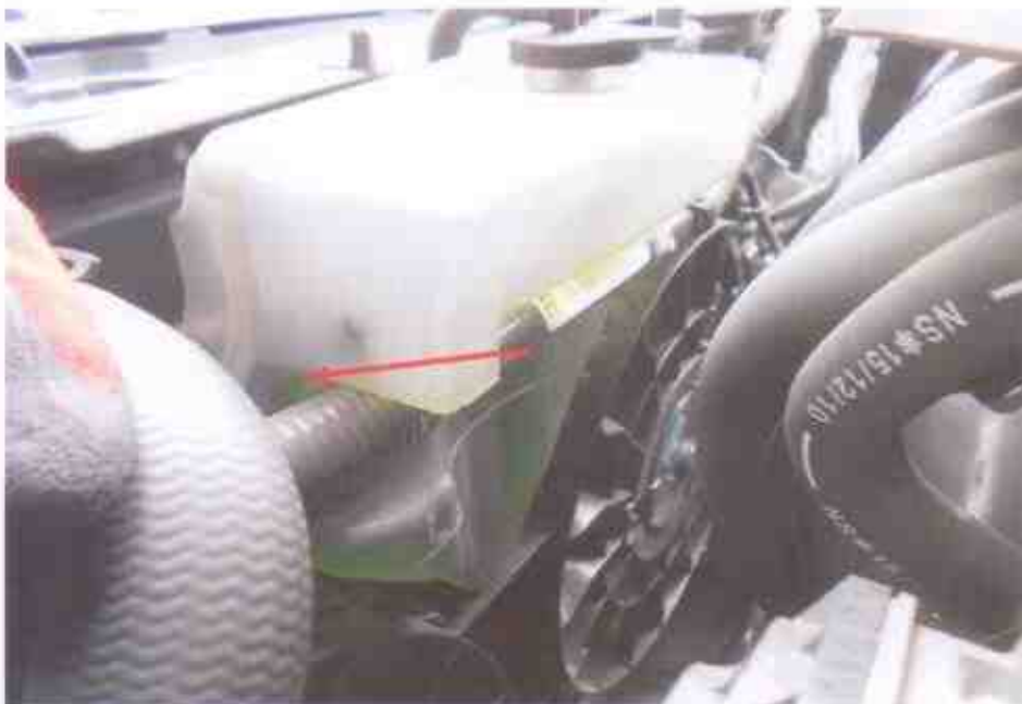
Photo 13 shows the coolant fluid reservoir of the Motor Car at the time of our inspection. The coolant fluid was observed to be of sufficient level and without any visible contamination.
