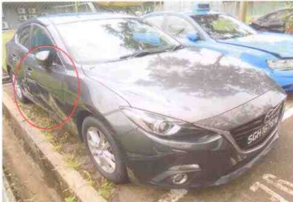
Photo 3 shows a general view of the right front body of the Motor Car at the time of our inspection. The Motor Car was observed to be in good general condition except for minor damages at the right side portion.
