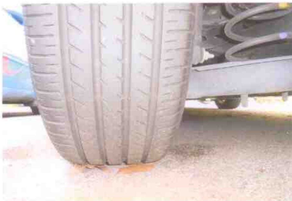
Photo 9 shows the condition of the rear left tyre of the Motor Car, which was observed to be in serviceable condition with remaining tread depth of approximately 7mm. The tyre was also observed to be sufficiently inflated for vehicular operation.
