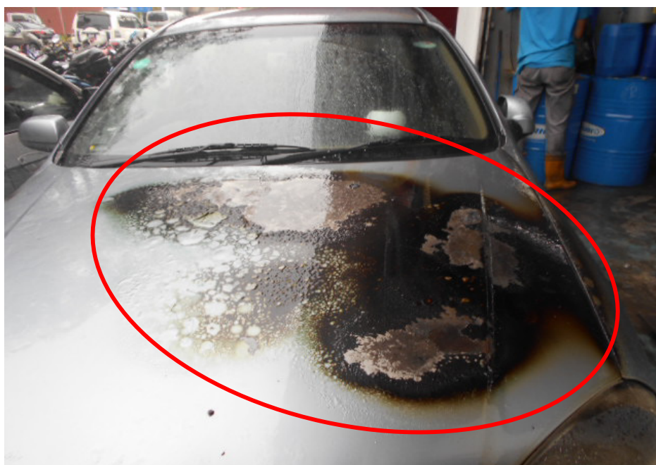
Photo 8 shows the intense burn marks (circled) that were found on the centre left of the front bonnet. Such marks are normally formed on steel/metal material body parts that had been exposed to prolong high heat intensity, and can usually determine the origin of the fire.
