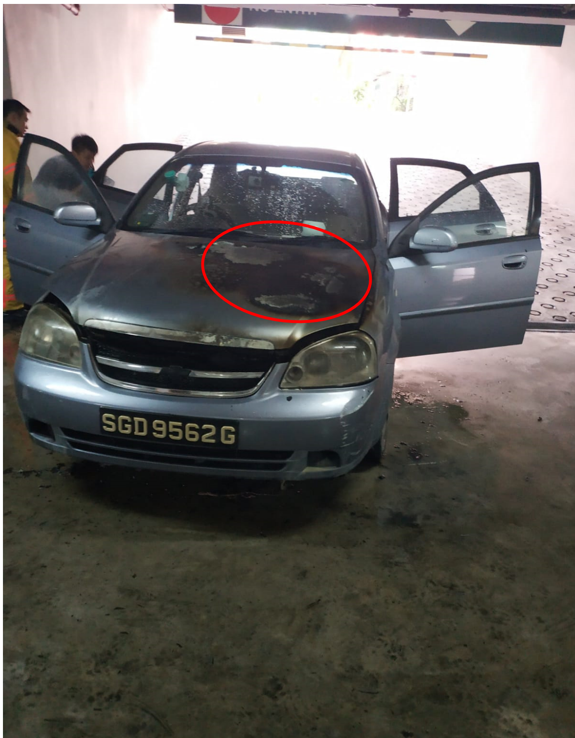
Photo 9 shows the Insured Vehicle at the incident scene after the fire was extinguished. Intense burn marks (circled) were seen on the front bonnet of the Insured Vehicle immediately after the fire was extinguished. Such marks are normally formed on steel/metal material body parts that had been exposed to prolong high heat intensity, and can usually determine the origin of the fire. For this case, the fire had originated at the centre left area of the Insured Vehicle's engine compartment.
