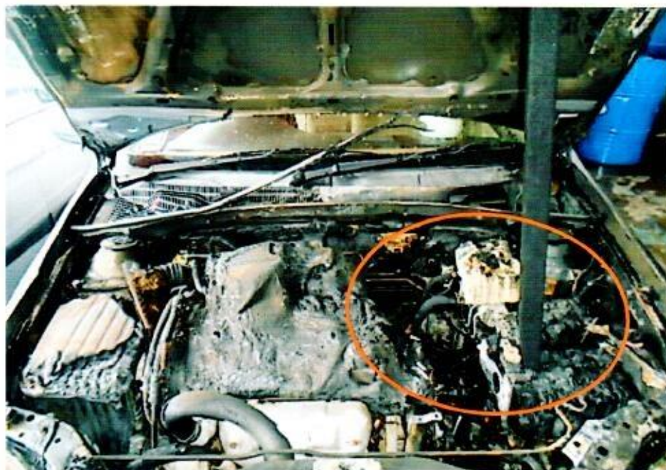
Photo 10 shows the engine compartment of the Insured Vehicle at the time of my inspection. Following the location where intense burn marks were found, the origin of fire was determined to be at the centre left area (circled) of the Insured Vehicle's engine compartment.
