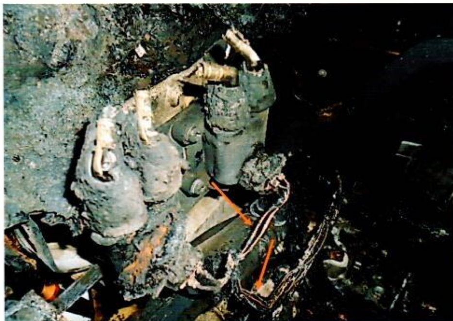
Photo 12 shows another stretch of wiring around the centre left area of the Insured Vehicle's engine compartment. The wirings (arrowed) were found to be completely burned to its bare copper state. Such condition normally indicates internal heating of copper wires, which is a sign of an electrical short circuit occurring. This then indicates that the cause of fire to the Insured Vehicle was of electrical nature.
