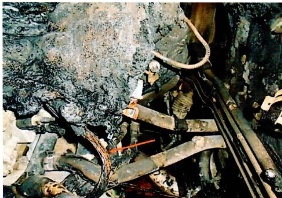
Photo 11 shows the wirings at the centre left area of the Insured Vehicle's engine compartment. Upon closer examination of the area where the fire had originated, I had found wirings (arrowed) that were completely burned to its bare copper state. The bright reddish colour of the copper wires suggest that the wirings were exposed to high heat. Such condition normally indicates internal heating of copper wires, which is a sign of an electrical short circuit occurring.
