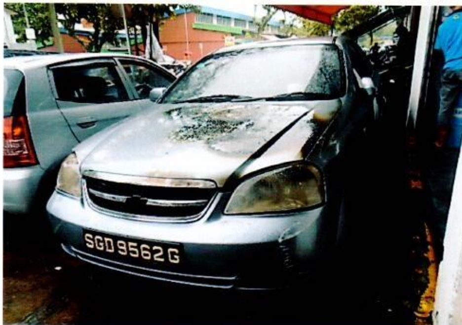
Photo 2 shows a general view of the front left body of the Insured Vehicle at the time of inspection. The Insured Vehicle was observed to have sustained fire damage at its frontal body. Its front left fender, front left headlamp and front bonnet were amongst the body parts that were found to have been burnt as a result of the fire.
