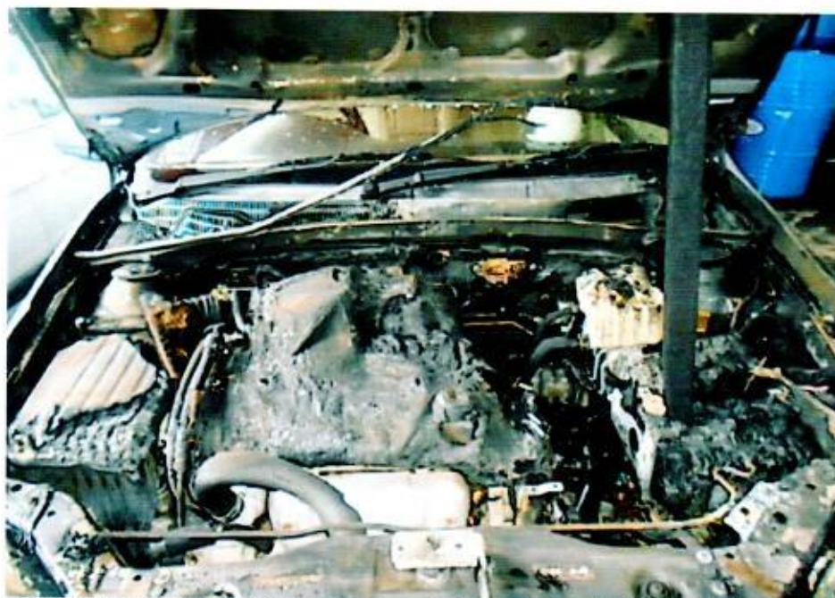
Photo 3 shows the engine compartment of the Insured Vehicle at the time of inspection. Almost all the parts inside the engine compartment were observed to have been burnt and/or melted as a result of the fire. These parts had included its radiator, air condenser, cooling fan, intake manifold, fuse box, battery, air duct, hoses and pipes amongst others.
