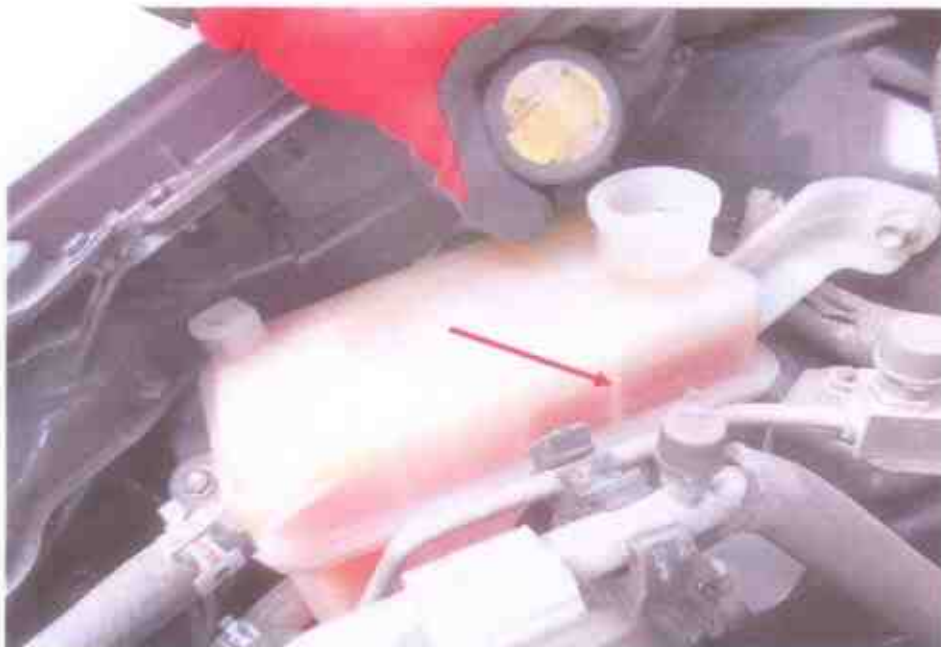
Photo 15 shows the engine coolant fluid reservoir of the Motor Taxi at the time of our inspection. The engine coolant fluid was observed to be of sufficient level and without any visible contamination.
