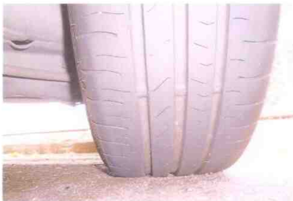
Photo 11 shows the condition of the rear left tyre of the Motor Taxi, which was observed to be in serviceable condition with remaining tread depth of approximately 5mm. The tyre, which was wrapped around alloy wheel rim, was also observed to be sufficiently inflated for vehicular operation.
