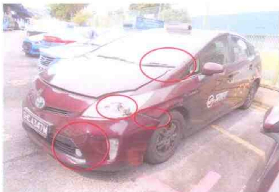
Photo 4 shows a general view of the front left body of the Motor Taxi at the time of our inspection. The Motor Taxi was observed to be in good general condition except for minor damages at the front left portion.
