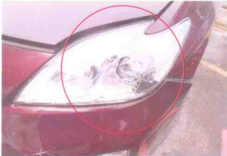
Photo 7 shows a close up view of the front left headlamp of the Motor Taxi at the time of our inspection. The Motor Taxi had sustained relatively minor impact at the front left headlamp as a result of the accident.
