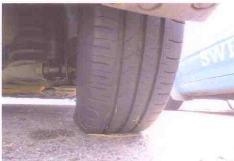
Photo 12 shows the condition of the rear right tyre of the Motor Taxi, which was observed to be in serviceable condition with remaining tread depth of approximately 5mm. There was also no tear, cut or burst mark(s) on the outer and the inner sidewalls as well as across the tread of the 4 tyres.
