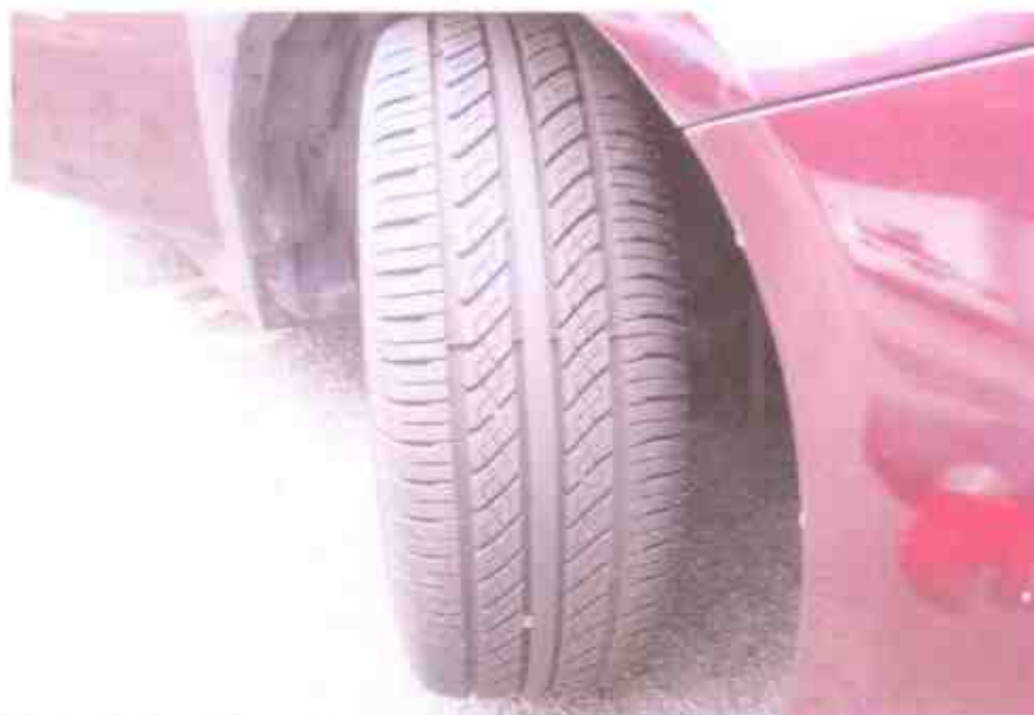
Photo 9 shows the condition of the front right tyre of the Motor Taxi, which was observed to be in serviceable condition with remaining tread depth of approximately 6mm. There was no tear, cut or burst mark(s) on the outer and the inner sidewalls.
