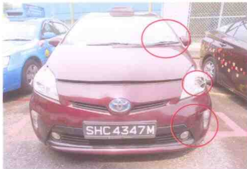
Photo 2 shows a general view of the front body of the Motor Taxi at the time of our inspection. The Motor Taxi was observed to be in good general condition except for minor damages at the frontal left portion.
