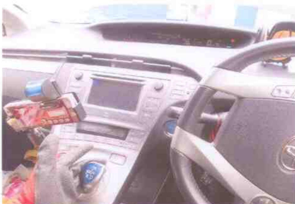
Photo 24 shows neutral mode on the LCD panel of the Motor Taxi while performing operational test. This would suggest that it was able to move forward and backward normally
