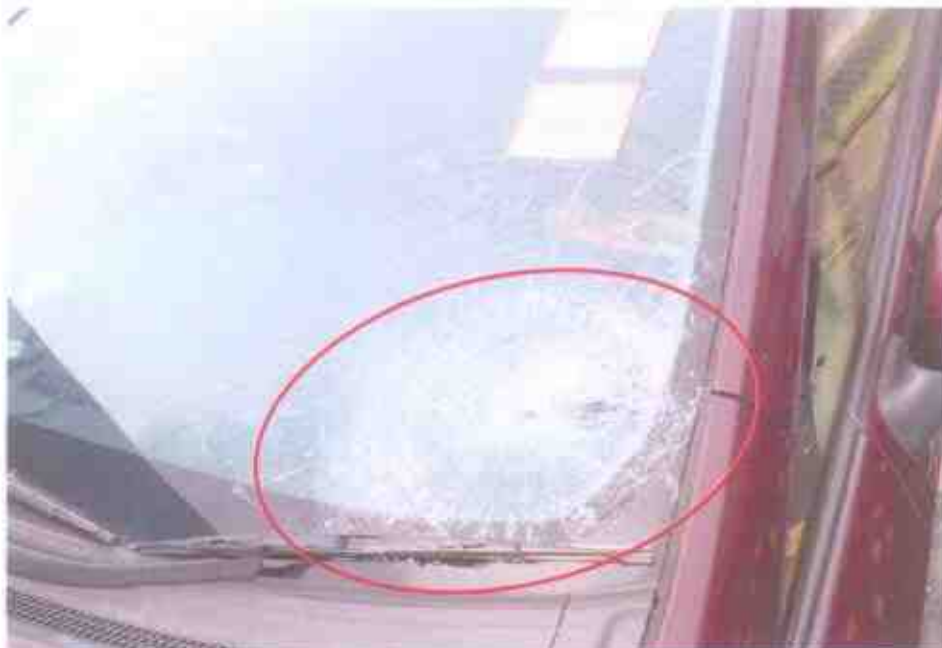
Photo 6 shows a close up view of the front left windshield of the Motor Taxi at the time of our inspection. The Motor Taxi had sustained shattering cracks on its lower left of the windshield.
