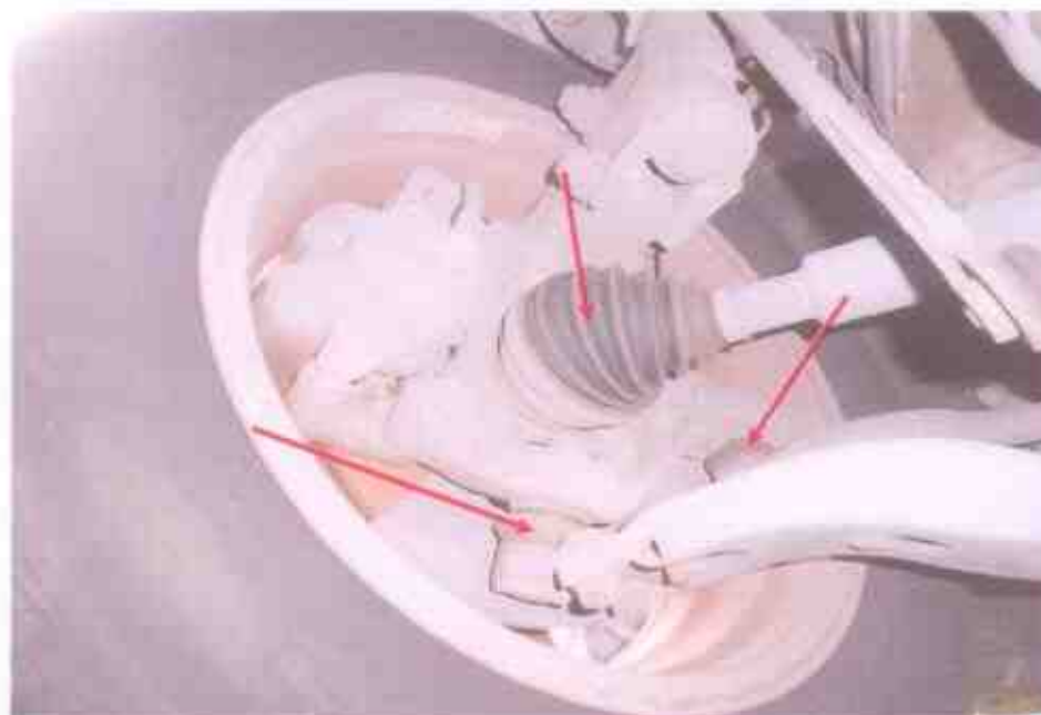
Photo 19 shows the various undercarriage components at the front right wheel of the Motor Taxi, in particular the steering tie rod (arrowed). The various steering components were all found to be intact, suggesting that the steering system of the Motor Taxi was likely to be in serviceable condition.
