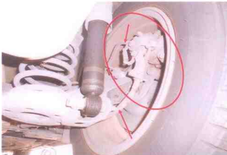
Photo 18 shows the brake hose (arrowed) at the rear right wheel of the Motor Taxi. We did not observe any leakage of brake fluid at the time of our inspection of the Motor Taxi. Our visual inspection of the various mechanical components of the Motor Taxi's braking system, including its brake calliper (circled), revealed all to be intact and without visible damage.
