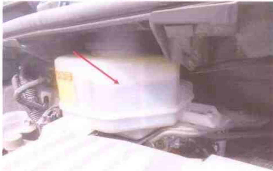
Photo 14 shows the brake fluid reservoir of the Motor Taxi at the time of our inspection. The brake fluid was observed to be of sufficient level (arrowed) and without any visible contamination.
