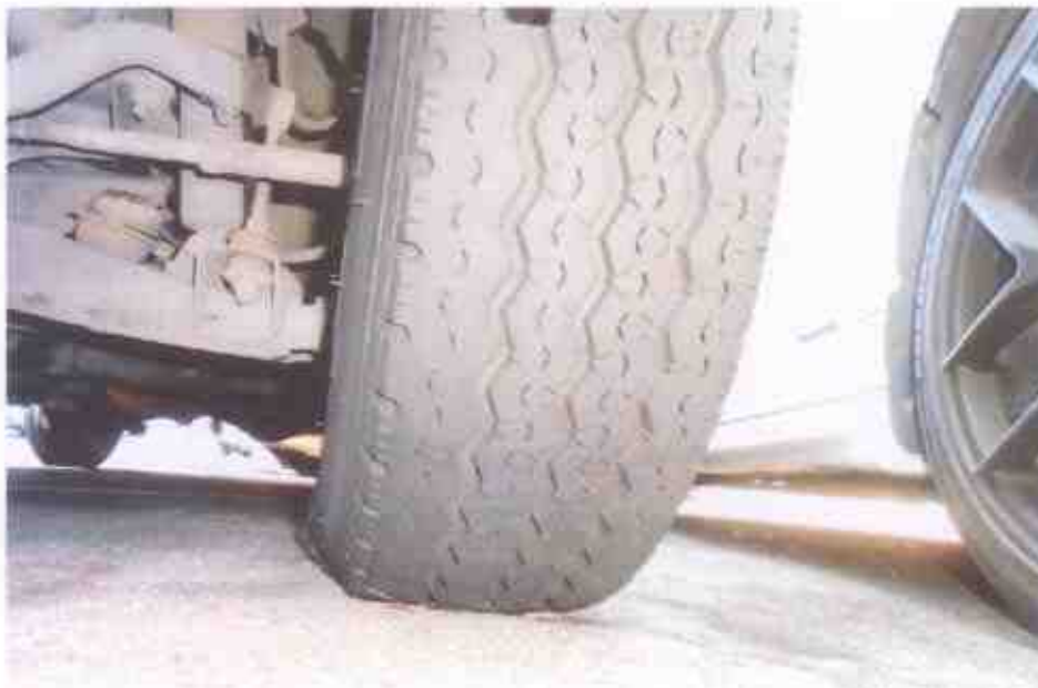
Photo 11 shows the condition of the front left tyre of the Motor Bus, which was observed to be in serviceable condition with remaining tread depth of approximately 7mm. The tyre, which was wrapped around standard wheel rim, was also observed to be sufficiently inflated for vehicular operation.
