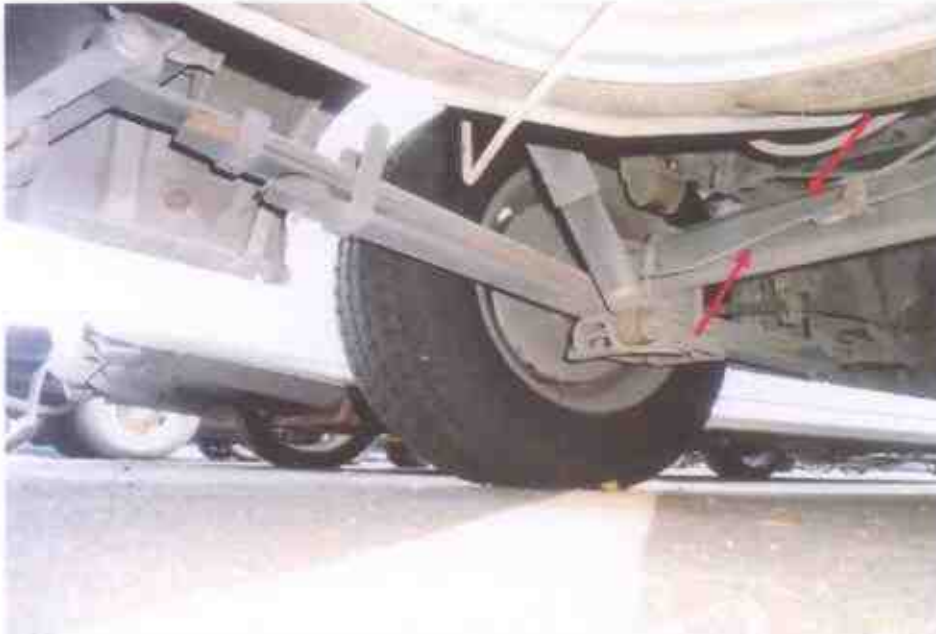
Photo 22 shows the various undercarriage components at the rear left wheel of the Motor Bus, in particular the brake hose (arrowed). We did not observe any leakage of brake fluid at the time of our inspection of the Motor Bus.
