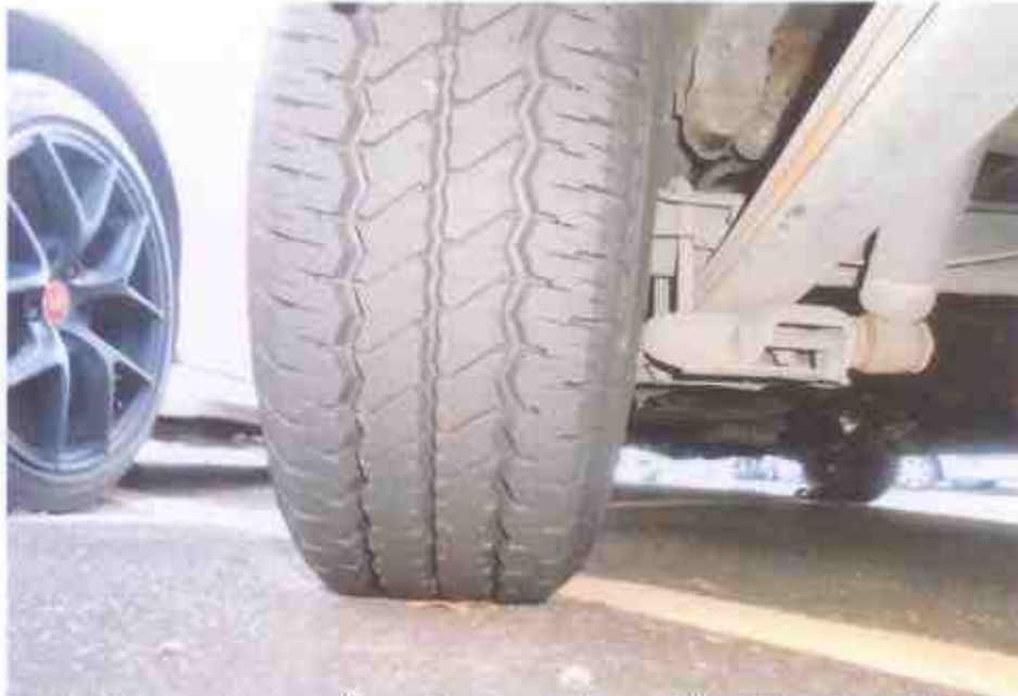
Photo 12 shows the condition of the rear left tyre of the Motor Bus, which was observed to be in serviceable condition with remaining tread depth of approximately 8mm. The tyre, which was wrapped around standard wheel rim, was also observed to be sufficiently inflated for vehicular operation. There was also no significant damage found on the 4 wheel rims of the Motor Bus.
