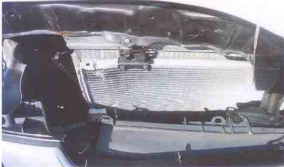
Photo 19 shows the damaged radiator as a result of the accident.
