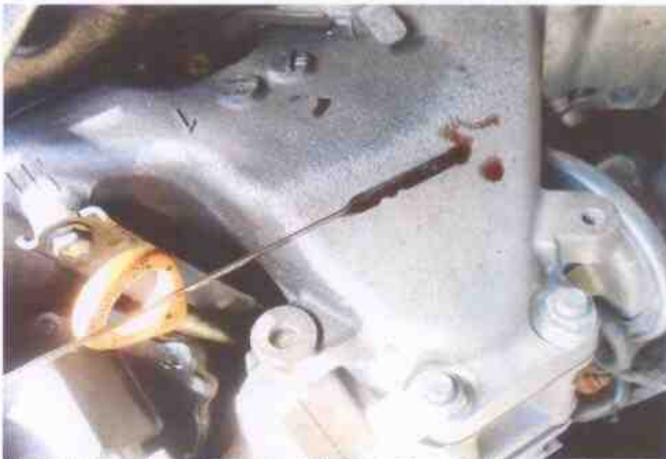
Photo 18 shows the ATF dip stick of the Motor Bus at the time of our inspection. The ATF was observed to be of sufficient level and without any visible contamination.
