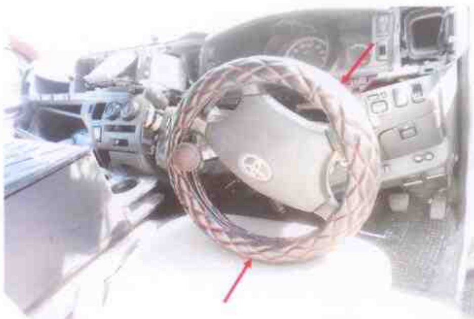
Photo 20 shows the damaged steering wheel at the time of our inspection of the Motor Bus. It was observed to be pushed inwards from the front portion.
