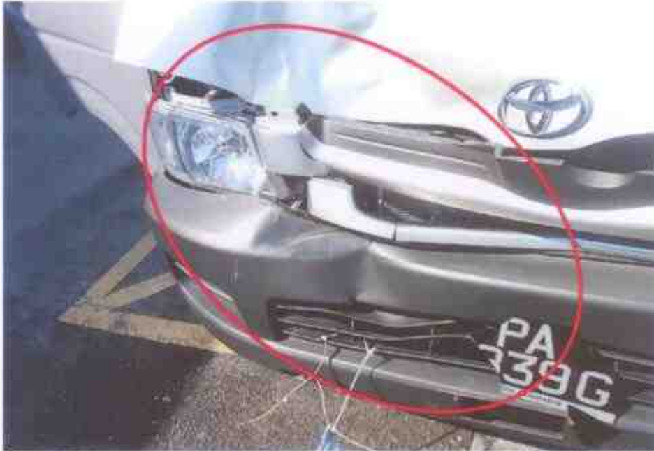
Photo 5 shows a close-up view of the damages on the right portion of the Motor Bus at the time of our inspection. It was likely due to the accident's impact collision.
