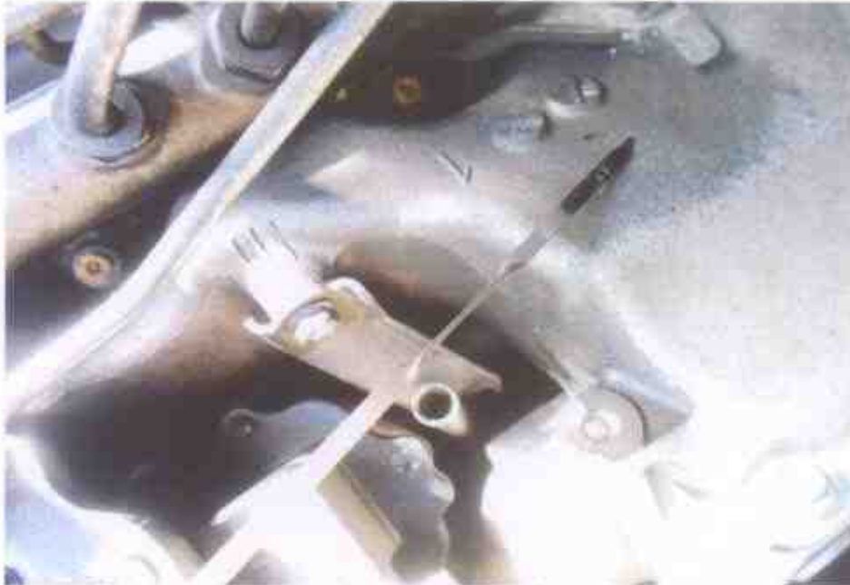
Photo 17 shows the engine dip stick of the Motor Bus at the time of our inspection. The engine oil was observed to be of sufficient level and without any visible contamination.
