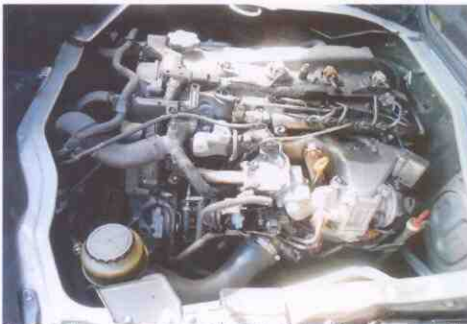
Photo 14 shows a general view of the Motor Bus's engine compartment. The various parts and components inside the engine compartment were unaffected by the accident. There was also no sign(s) or indication(s) of fluid leakage and/or fluid stain within the engine compartment.
