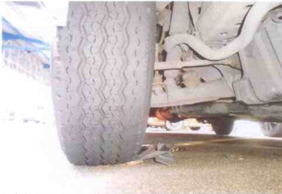
Photo 10 shows the condition of the front right tyre of the Motor Bus, which was observed to be in serviceable condition with remaining tread depth of approximately 7mm. The tyres were all observed to be sufficiently inflated for vehicular operation with no tear, cut or burst mark(s) on the outer and the inner sidewalls as well as across the tread.
