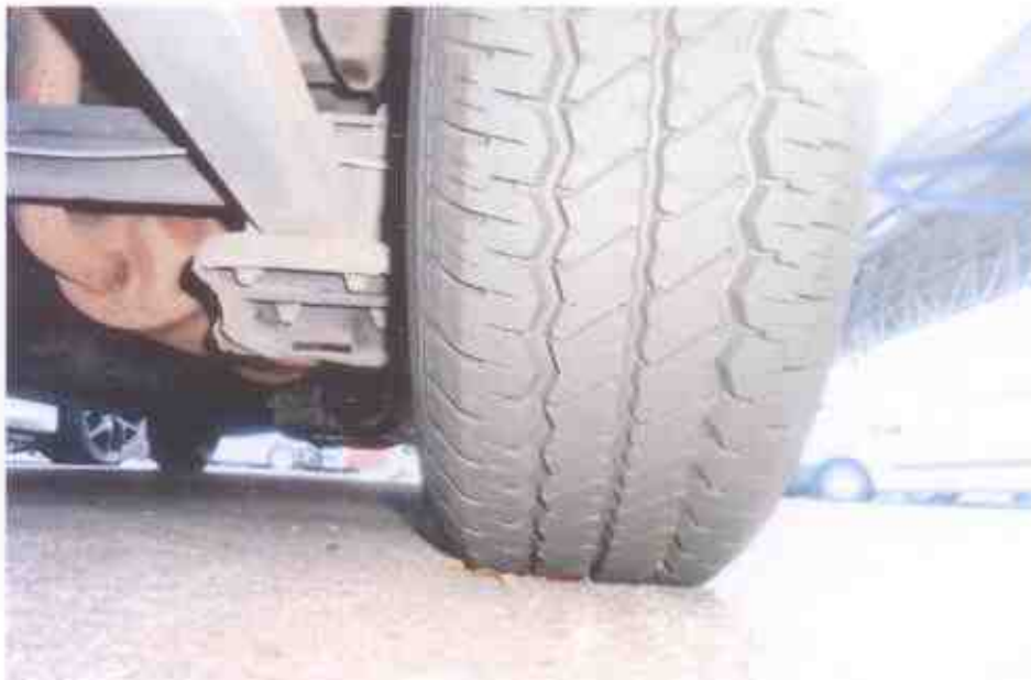
Photo 13 shows the condition of the rear right tyre of the Motor Bus, which was observed to be in serviceable condition with remaining tread depth of approximately 8mm. There was also no tear, cut or burst mark(s) on the outer and the inner sidewalls as well as across the tread of the tyre, which was also sufficiently inflated for vehicular operation.
