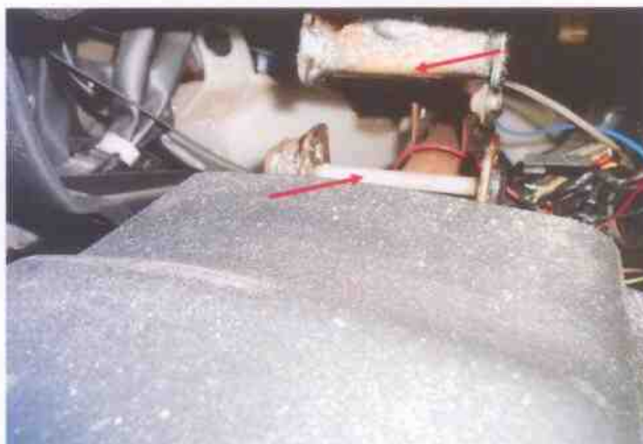
Photo 21 shows the damaged steering wheel supporting component at the time of our inspection of the Motor Bus. It was observed to be dislodged from the original installation.
