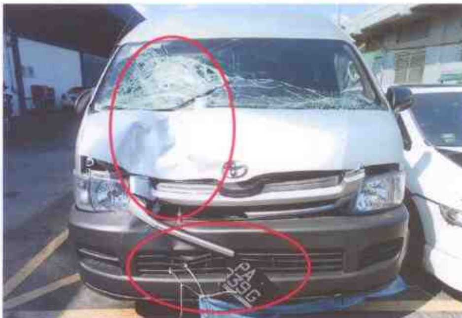
Photo 2 shows a general view of the front body of the Motor Bus at the time of our inspection. The Motor Bus was observed to sustained damages at the front right portion due to the accident's impact.
