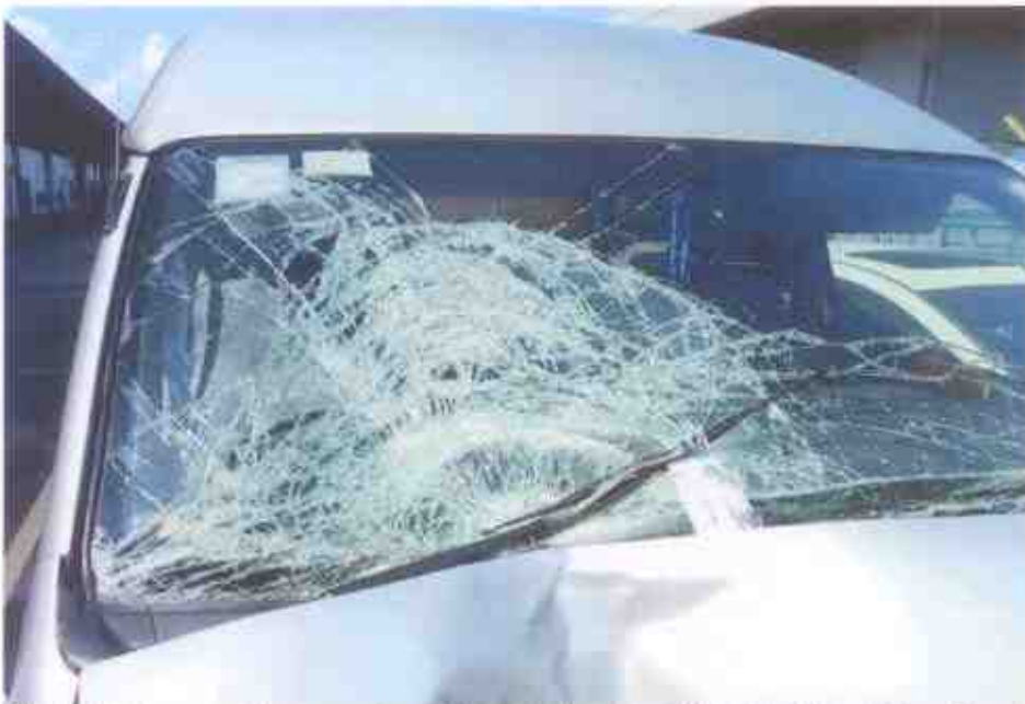
Photo 6 shows a close-up view of the shattered windshield of the Motor Bus at the time of our inspection. It was likely due to the accident's impact collision.
