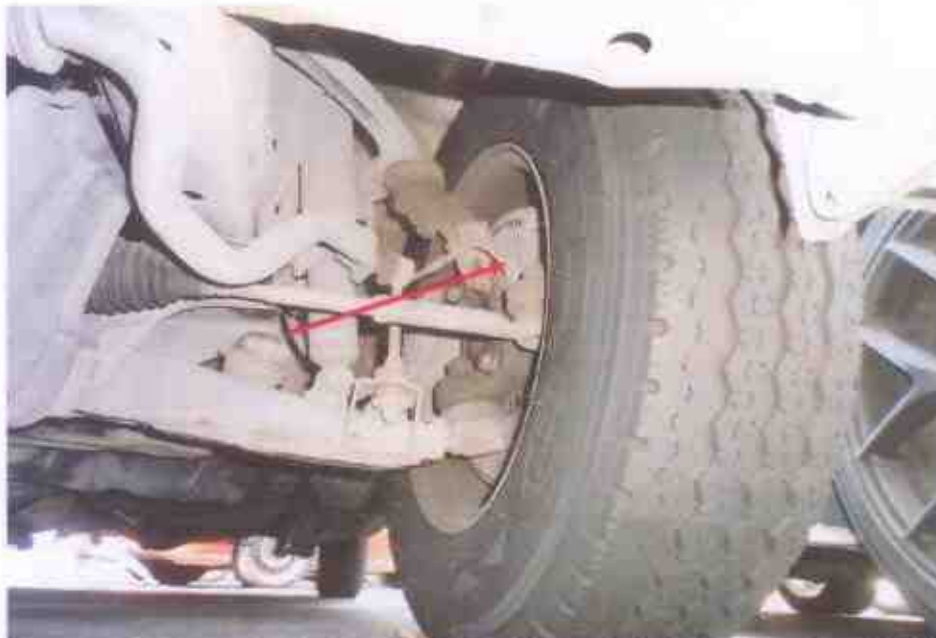
Photo 23 shows the brake hose at the front left wheel of the Motor Bus. We did not observe any leakage of brake fluid. Our visual inspection of the various mechanical components of the Motor Bus's braking system revealed all to be intact and without visible damage, indicating that the braking system was likely to be in serviceable condition at the material time of accident.
