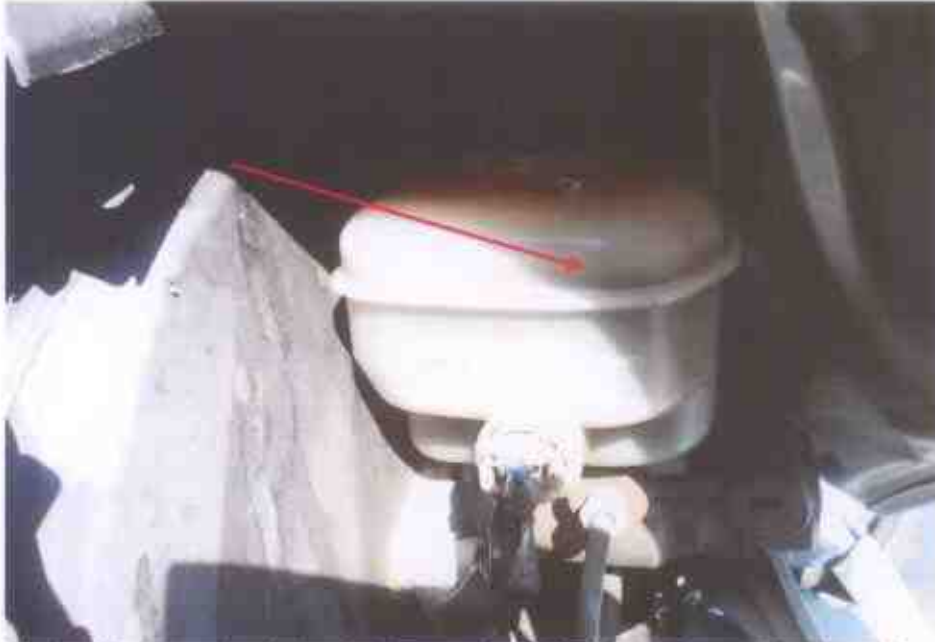
Photo 15 shows the brake fluid reservoir of the Motor Bus at the time of our inspection. The brake fluid was observed to be of sufficient level and without any visible contamination.
