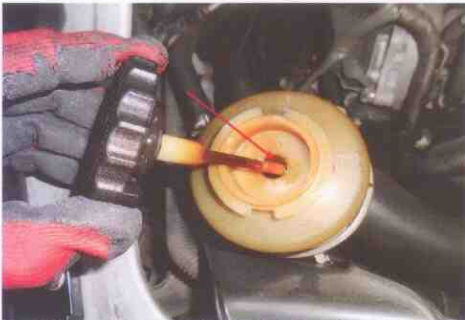
Photo 16 shows the power steering fluid of the Motor Bus at the time of our inspection. It was observed to be of sufficient level and without any visible contamination.
