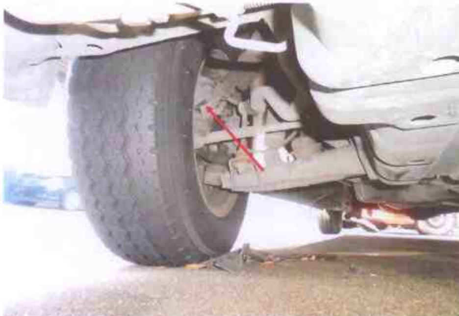
Photo 24 shows the brake hose (arrowed) at the front right wheel of the Motor Bus. We did not observe any leakage of brake fluid at the time of our inspection of the Motor Bus. Our visual inspection of the various mechanical components of the Motor Van's braking system, including its brake calliper, revealed all to be intact and without visible damage.
