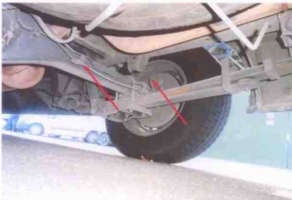
Photo 25 shows the various undercarriage components at the rear right wheel of the Motor Bus. The various steering components were all found to be intact, suggesting that the steering system of the Motor Bus was likely to be in serviceable condition at the material time of accident. There was also no sign of fluid stain(s) observed on the various undercarriage components at the 4 wheels of the Motor Bus.
