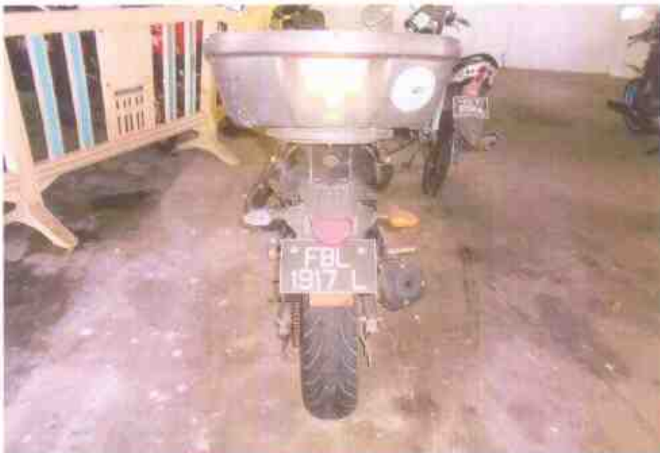
Photo 4 shows a general view of the rear portion of the Motorcycle at the time of our inspection. The Motorcycle was observed to have sustained with relatively minor impact due to the accident collision. This includes damages on its left signal lamp & rear compartment box.
