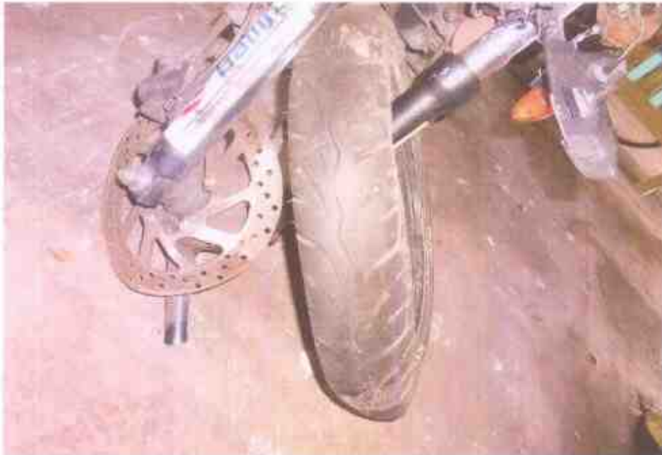
Photo 11 shows the Motorcycle's front tyre, it was observed to be dislodged from the broken wheel rim & deflated due to the accident's impact collision. However, the tread pattern of the front tyre was clearly visible. We did not observe any tear, burst mark(s) and/or punctured hole(s) on the sidewalls as well as across the tread of the rear tyres
