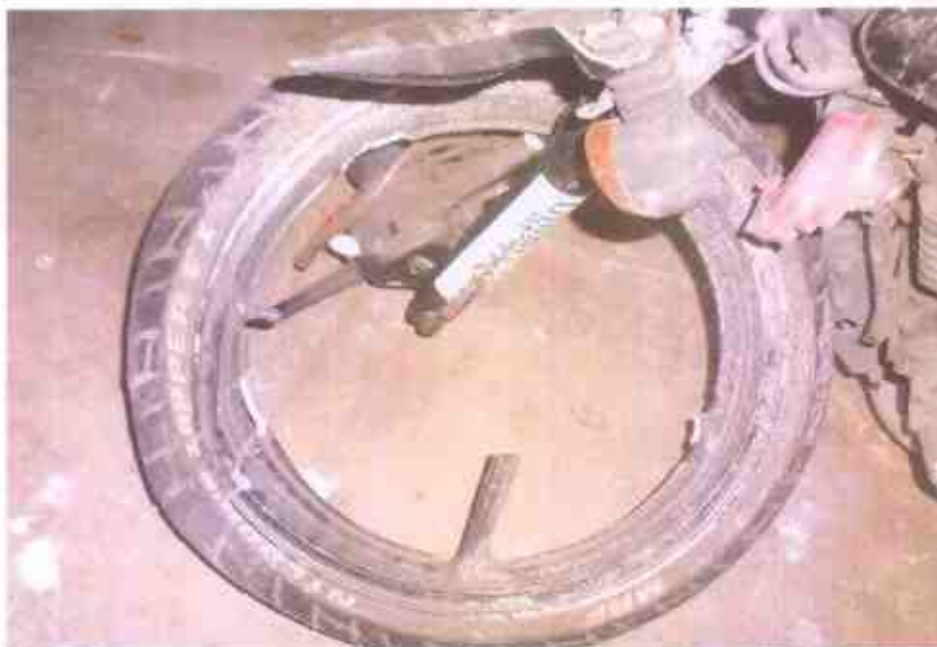
Photo 6 shows a close-up view of the broken front wheel rim of the Motorcycle due to the accident collision.
