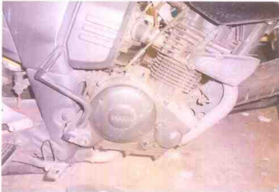
Photo 14 shows the engine area view. There was also no sign(s) or indication(s) of fluid leak observed around the engine area of the Motorcycle.
