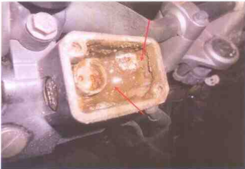
Photo 20 shows after opening of the front brake fluid reservoir of the Motorcycle (arrowed). We found that the brake fluid turned into sludge like substance. Hence, indicates it had been contaminated prior to the accident.
