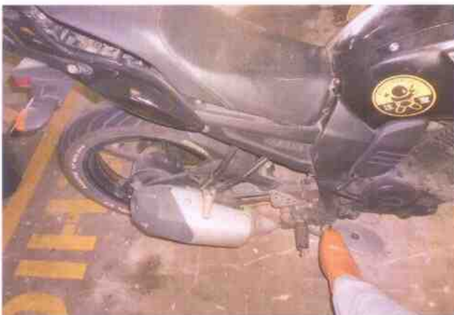
Photo 22 shows the rear brake static test of the Motorcycle. The type of brake system for the rear wheel was of mechanical type, controlled by the brake foot pedal of the Motorcycle. Our static brake test revealed that the rear brake system of the Motorcycle was in serviceable condition without damage.
