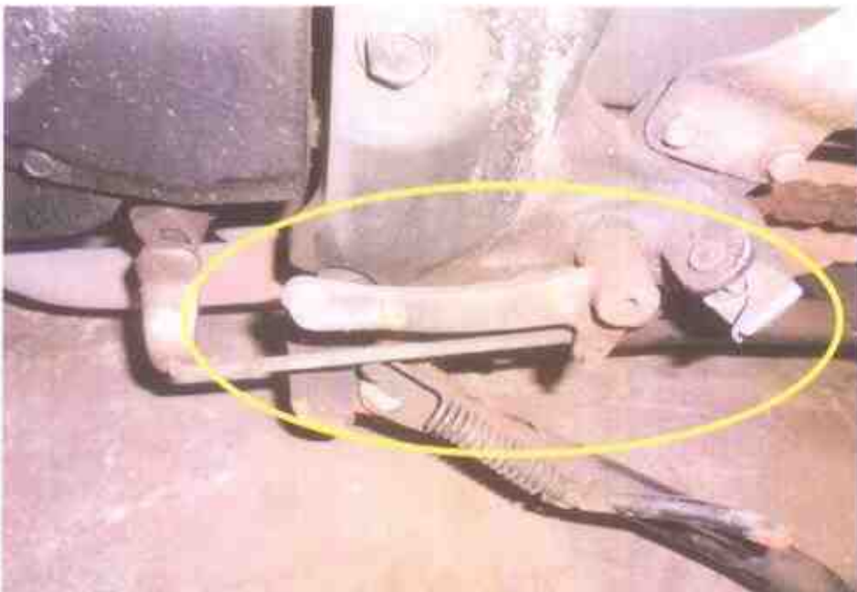
Photo 8 shows a close-up view of the damages on the foot rest & gear shift pedal of the Motorcycle due to the accident collision.
