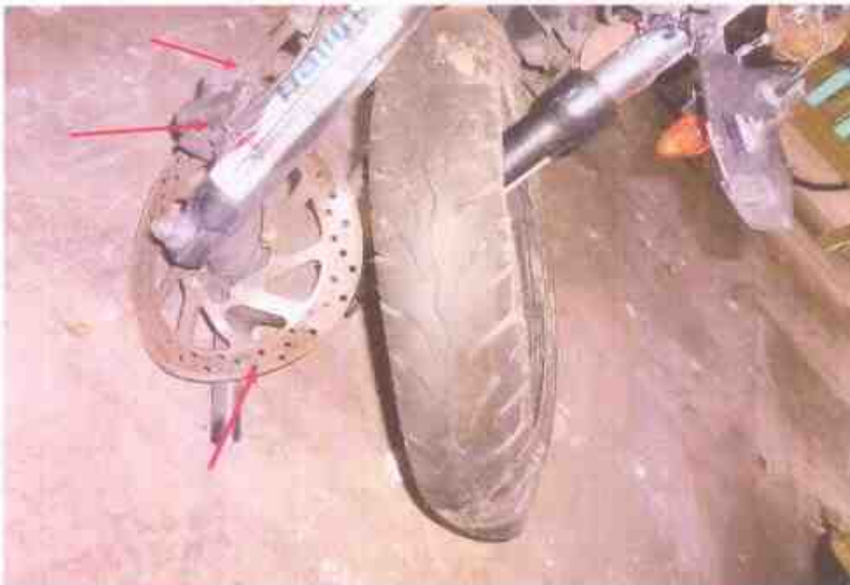
Photo 18 shows the front brake calliper, front brake disc and front brake hose of the Motorcycle (arrowed), which are all part of the components in the front brake system of the Motorcycle. Our visual checks of these various components had revealed that only the brake disc was damaged due to the accident. No leakage of brake fluid was also observed.
