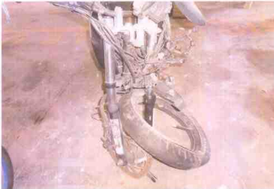
Photo 17 shows the front fork was observed to have sustained with severe damages as a result of the accident. Hence, we are not able to conduct any tests on the steering system of the Motorcycle.
