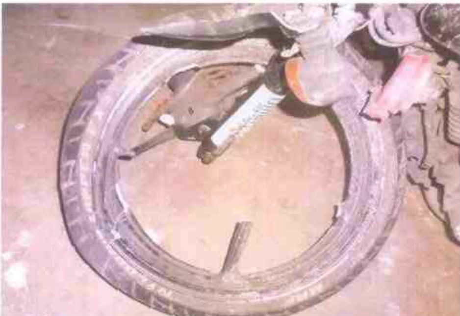
Photo 12 shows the Motorcycle's front wheel rim, it was observed to be broken due to the accident's impact collision. However, the tread pattern of the front tyre was clearly visible. We did not observe any tear, burst mark(s) and/or punctured hole(s) on the sidewalls as well as across the tread of the rear tyres
