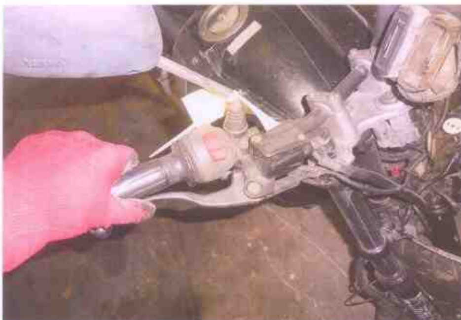
Photo 21 shows the front brake static test. It was observed to be not in serviceable condition at time of our inspection. The brake lever was found to be without resistance (spongy like feel). However, no brake fluid leakage was observed at time of our inspection.
