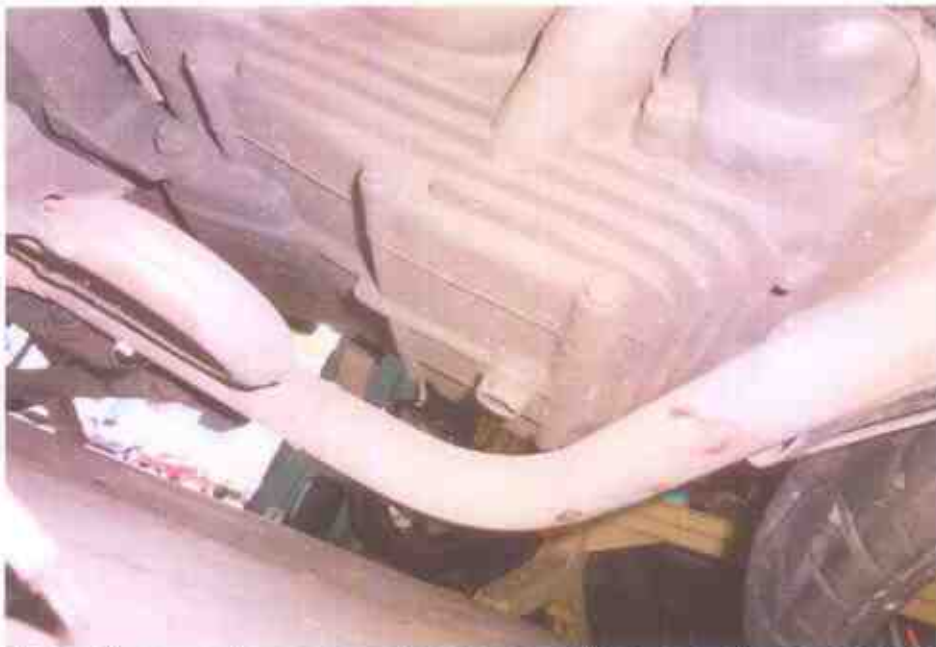
Photo 13 shows the engine underside view. There was also no sign(s) or indication(s) of fluid leak observed around the engine area of the Motorcycle.
