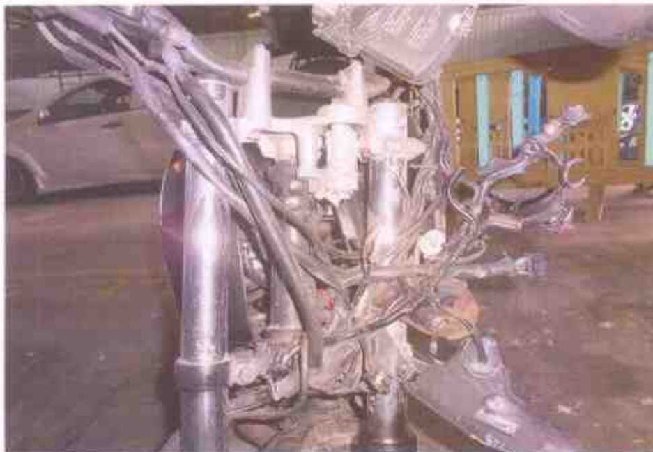
Photo 5 shows a close-up view of the missing headlamp & missing speedometer of the Motorcycle due to the accident collision.
