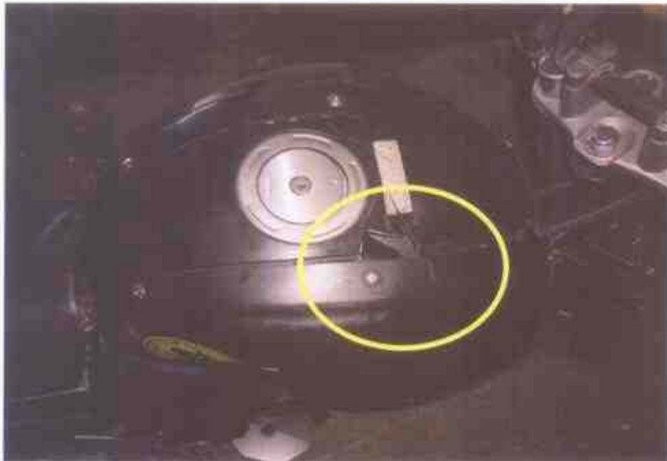
Photo 7 shows a close-up view of the crack mark on the fuel tank of the Motorcycle due to the accident collision.
